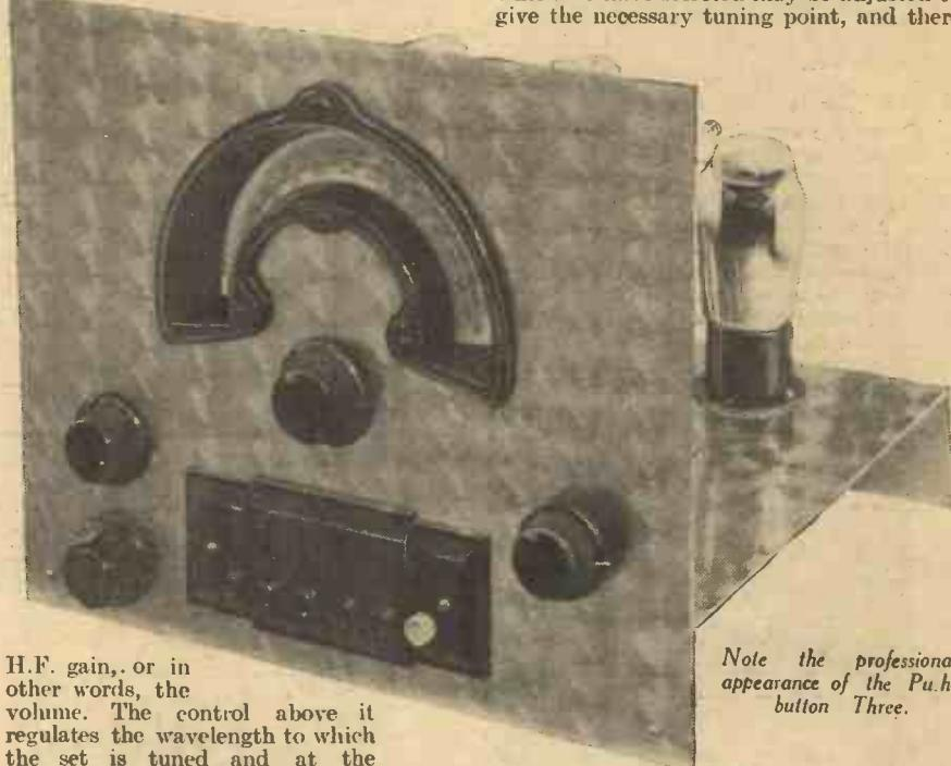
H.F. gain, or in other words, the volume. The control above it regulates the wavelength to which the set is tuned and at the same time switches the set on and off. The right-hand control is merely for reaction, and is only used when a weak station is required and the signal strength has to be augmented. Run round the dial on both wavebands, and note the stations which may be received. There should be quite a wide selection available providing that a good aerial and earth are being employed.
