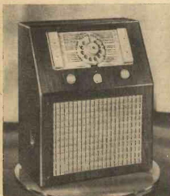
The Cossor auto-tuning system operates direct on the tuning condenser without trimmers.
