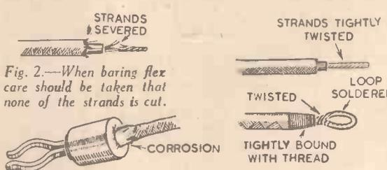
Fig. 5.—Some methods of making good connections to wander plugs and other types of connecting device.
