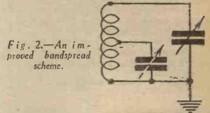
Fig. 2.—An improved bandspread scheme.
