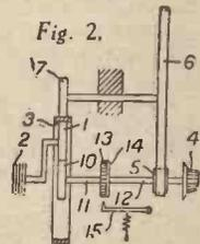
tune position, when a control voltage actuates an electromagnet device 15 which engages the toothed periphery of clutch member 13 thereby arresting shaft 11 and the sun wheel 10. Continued rotation of knob 4 now drives the condenser 2 through the gear train 6, 7, 3, 1 the ratio of which may be ten times that of the other planetary system. The wheels 7 and 1 may both engage the inner surface of the wheel 3.
