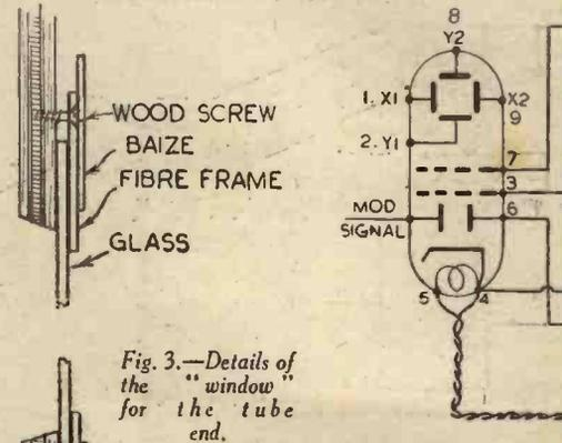
Fig. 3.—Details of the "window" for the tube end.
