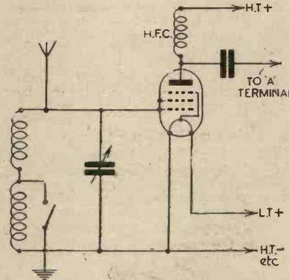
Fig. 3.—An H.F. or pre-selector stage for addition to a standard superhet circuit.
