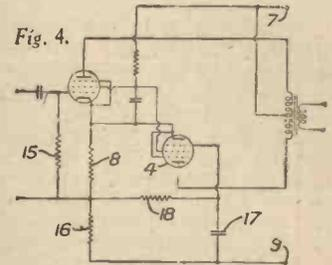
negative high tension terminal. The input to the first valve may be directly between the grid and the cathode, and the input to the second valve may include a resistance in the common anode circuit.
