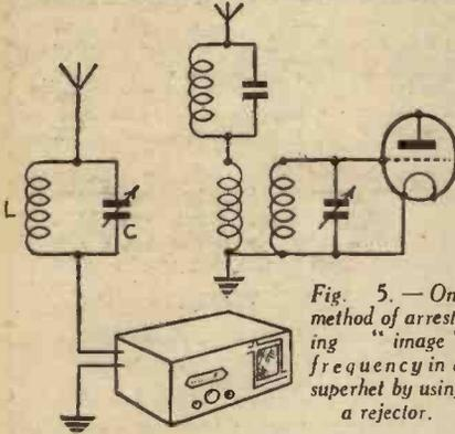
Fig. 5. — One method of arresting "image" frequency in a superhet by using a rejector.
