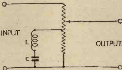
Fig. 10.—Tone-compensated volume control giving uniform frequency response. L.C. is an acceptor tuned broadly to 1000 cycles.
