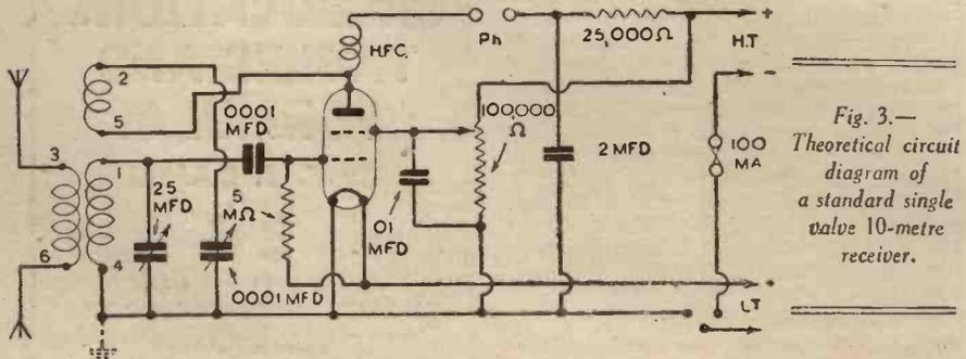
Fig. 3.—Theoretical circuit diagram of a standard single valve 10-metre receiver.
