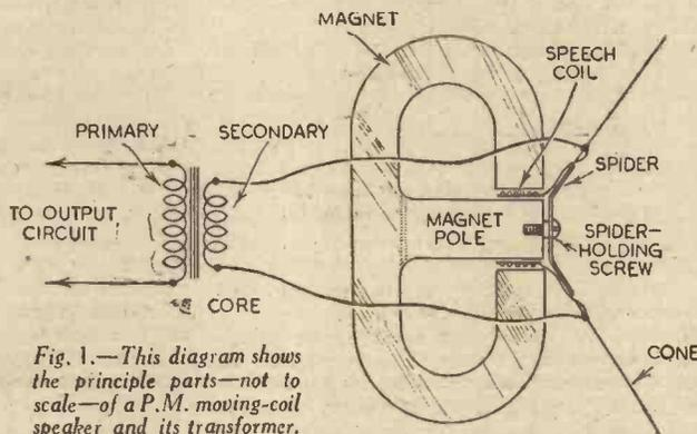
Fig. 1.—This diagram shows the principle parts—not to scale—of a P.M. moving-coil speaker and its transformer.
