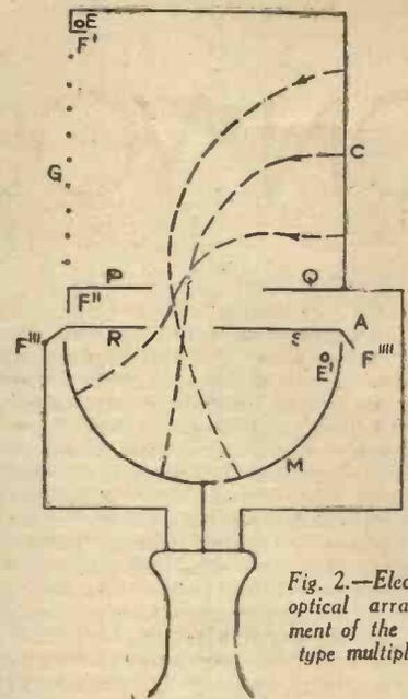
Fig. 2.—Electron optical arrangement of the new type multiplier.
