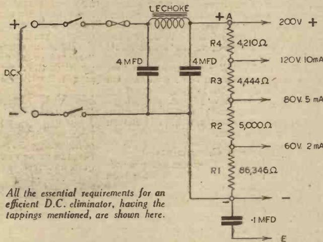
All the essential requirements for an efficient D.C. eliminator, having the tappings mentioned, are shown here.
