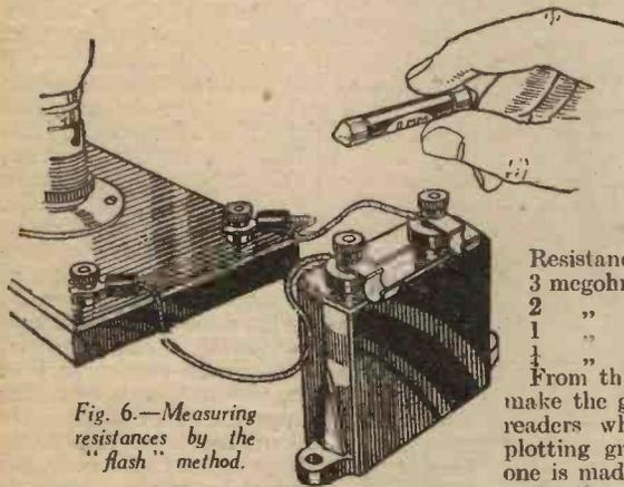
Fig. 6.—Measuring resistances by the "flash" method.
