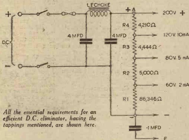
500 volts at 120 mA's, then a suitable value for the bleeder would be:
