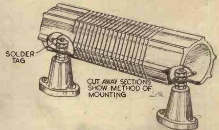
Fig. 4.—Showing the method of mounting the tuning coil.
