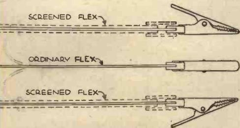
The flex and Fig. 5.—Details of screened flex leads with plugs and clips.
