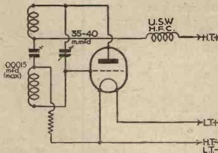
Fig. 2.—Circuit diagram of a conventional ultra-short-wave oscillator.
