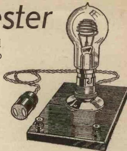
Fig. 1.—The completed neon lamp tester.
