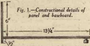
Fig. 1.—Constructional details of panel and baseboard.
