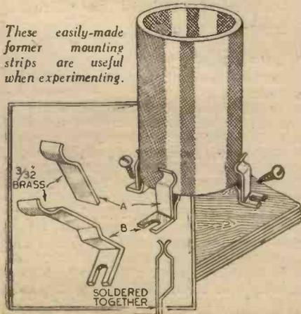
These easily-made former mounting strips are useful when experimenting.
