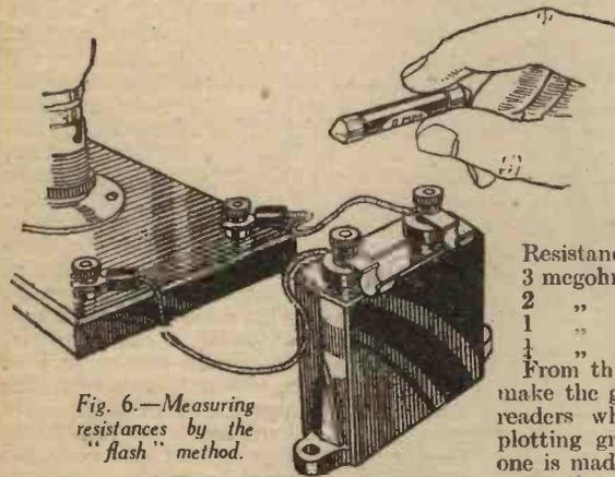
Fig. 6.—Measuring resistances by the "flash" method.
