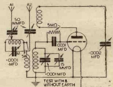
Fig. 2.—Circuit diagram showing an alternative method of aerial resonance tuning.
