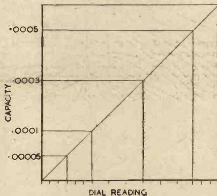
Fig. 6.—A graph of condenser readings.
