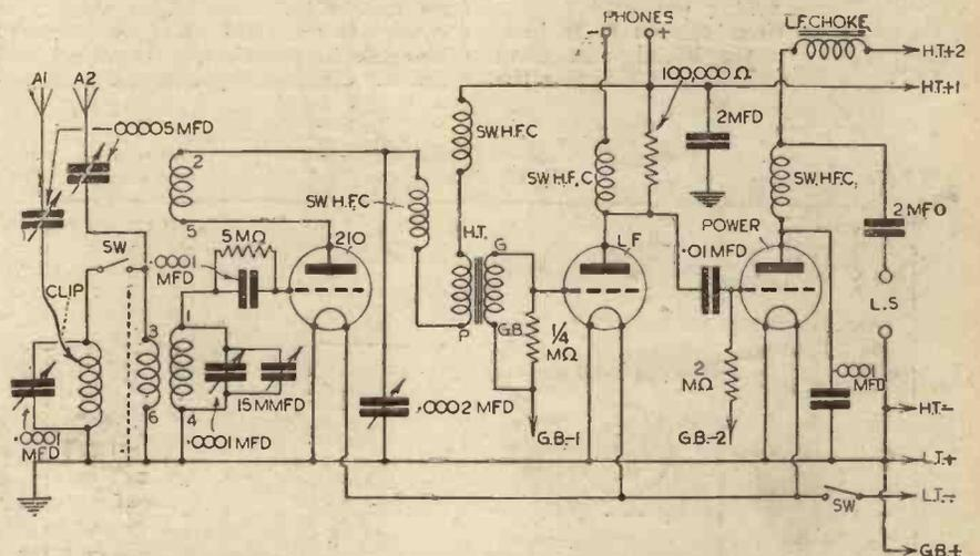
Fig. 1.—Theoretical circuit diagram of an experimental three-valve S.W. receiver. Aerial tuner consists of 26 turns of 22-gauge tinned copper wire spaced 1/4 in. on a 1 1/2 in. diameter ebonite ribbed former.
