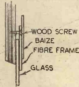
Fig. 3.—Details of the "window" for the tube end.
