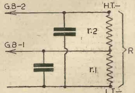
Fig. 3.—Shows how the resistance R has to be tapped to allow more than one G.B. supply to be obtained.
