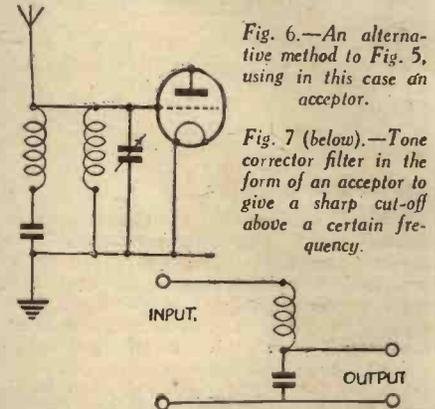
Fig. 6. — An alternative method to Fig. 5, using in this case an acceptor.
