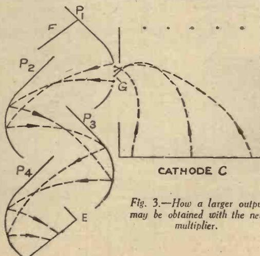
Fig. 3.—How a larger output may be obtained with the new multiplier.
