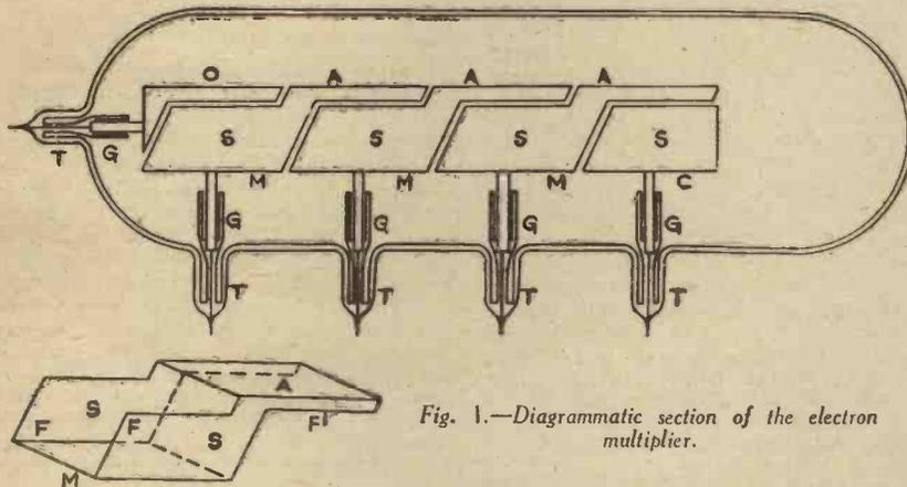
Fig. 1.—Diagrammatic section of the electron multiplier.
