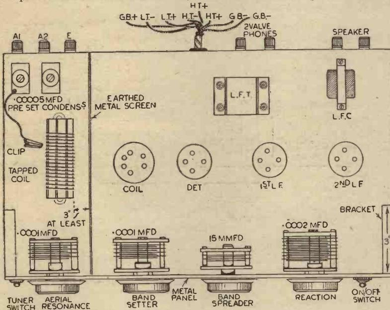
Fig. 3.—The layout of components for the three-valve receiver described in the text.
