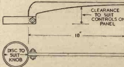
Fig. 7.—Details of extension handle for condenser.
