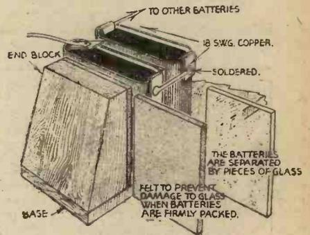
A method of assembling flash-lamp batteries for forming an H.T. unit.
