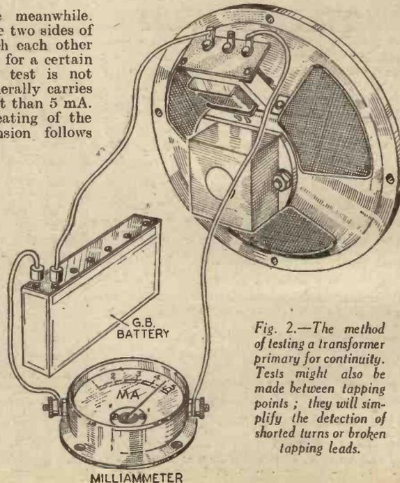
Fig. 2.—The method of testing a transformer primary for continuity. Tests might also be made between tapping points; they will simplify the detection of shorted turns or broken tapping leads.
