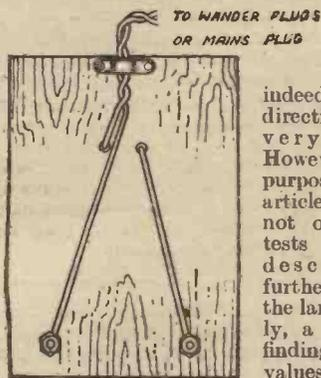
Fig. 2.—The simple wiring below the test board.
