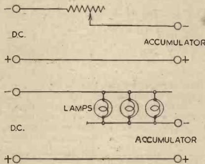
Fig. 4.—Two arrangements for limiting the current flowing in the accumulator circuit.
