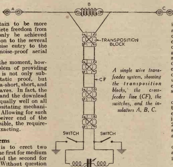
A single wire trans-feeder system, showing the transposition blocks, the cross-feeder line (CF), the switches, and the insulators A, B, C.
