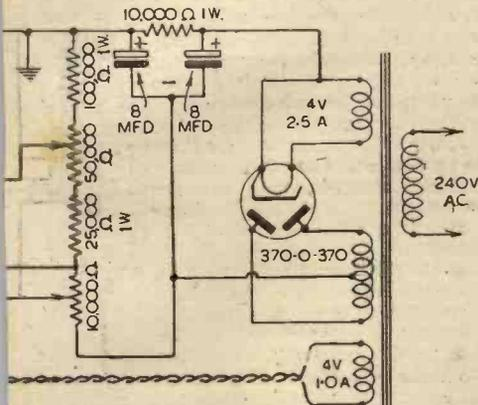
Fig. 3.—Circuit diagram of the monitor tube and power-pack unit.
