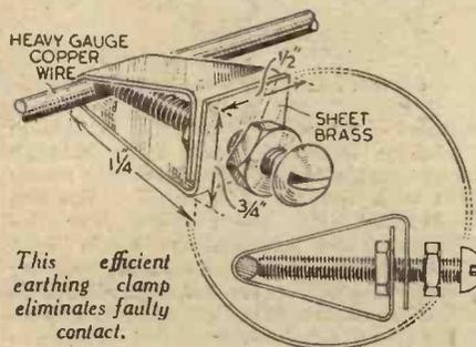
This efficient earthing clamp eliminates faulty contact.
