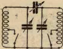
Fig. 1.—The standard bandpass tuning circuit.
