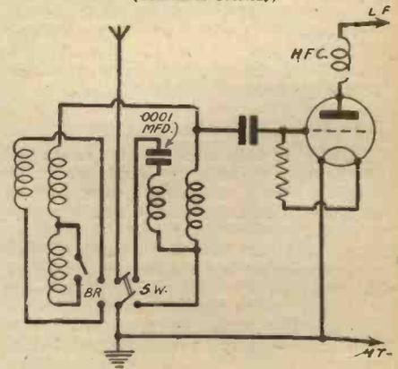
Fig. 4.—This circuit shows connections which can be used when both S.W. and broadcast coils have separate aerial windings. Tuning condensers and reaction circuits are omitted for simplicity.
