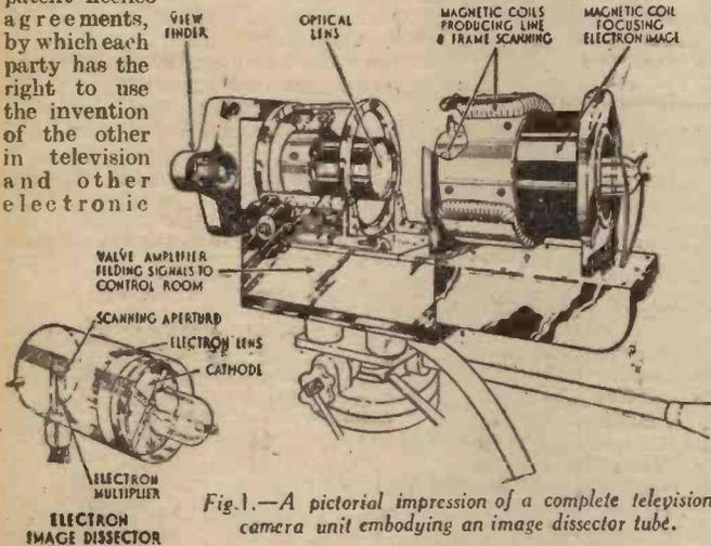
Fig. 1.—A pictorial impression of a complete television camera unit embodying an image dissector tube.
