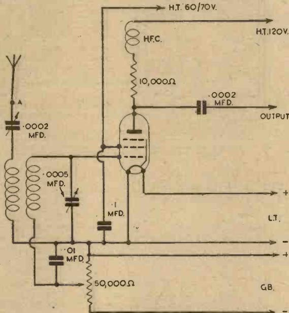
Fig. 1.—The circuit employed for this unit, showing how the variable bias is applied.
