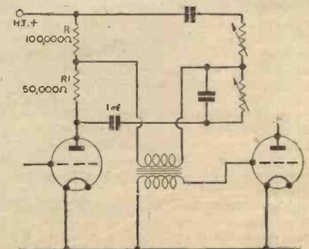
Fig. 5.—The filter used for intervalve coupling.
