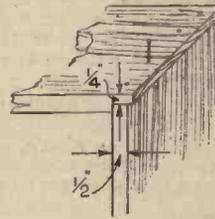
Fig. 2 (Right).—How a corner halving joint is made.
