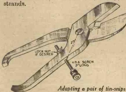
Adapting a pair of tinman's shears for insulation stripping.
