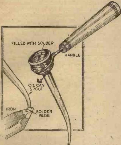
A useful soldering accessory contrived from an old oil-can spout.
