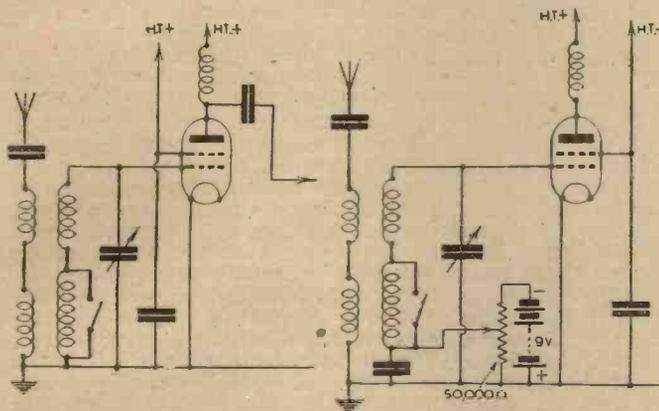
Fig. 1.—The diagram on the left shows an ordinary H.F. grid circuit while that on the right indicates connections for a variable-mu.
