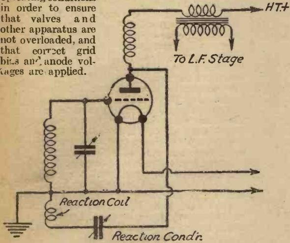
Fig. 1.—The conventional form of capacity reaction control.
