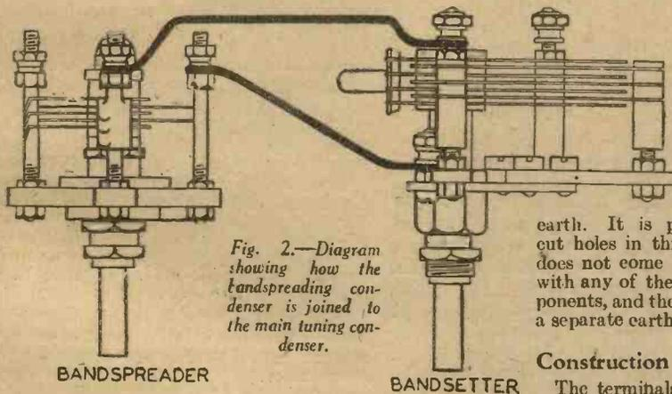
Fig. 2.—Diagram showing how the handspreading condenser is joined to the main tuning condenser.
