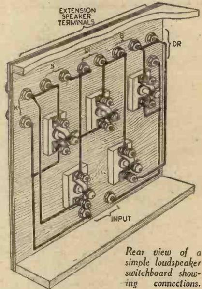
use individually or collectively. By operating the switches when two or more speakers are joined rapid comparisons are possible for test purposes, or if the speakers are fed from a distant point individual rooms may be switched in and out as required.—W. CLOUTING (Bayton, nr. Woodbridge).
