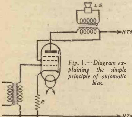
Fig. 1.—Diagram explaining the simple principle of automatic bias.
