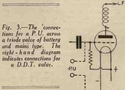
Fig. 3.—The connections for a P.U. across a triode valve of battery and mains type. The right-hand diagram indicates connections for a D.D.T. valve.
