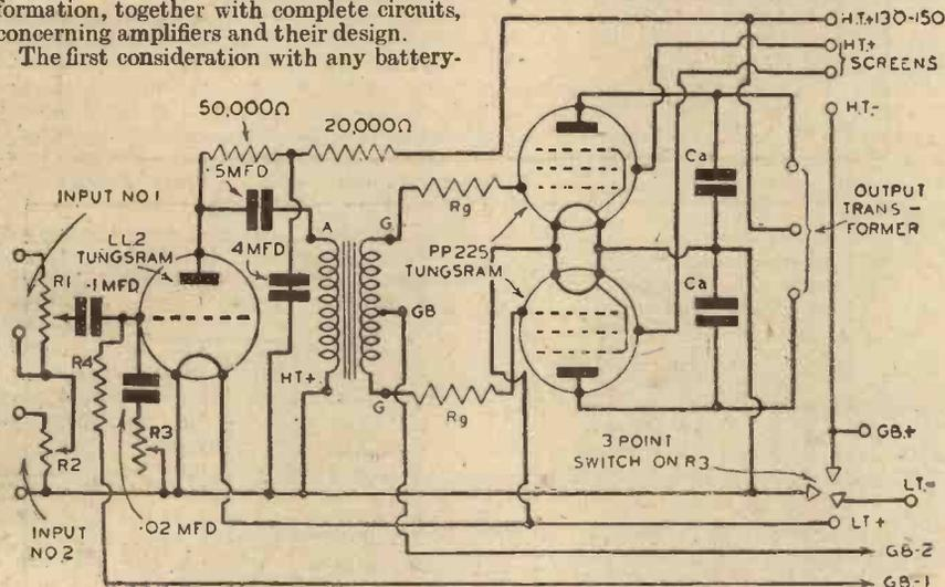
Fig. 1.—Theoretical circuit of the 2½-watt battery amplifier.
