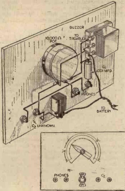
A simple but efficient capacity bridge.
