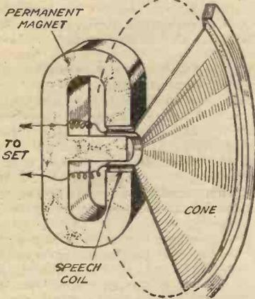
Fig. 1.—Main details of a permanent magnet speaker.
