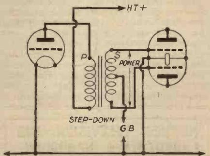
*A class B transformer steps down, because the valve is power operated; an ordinary L.F. transformer steps up because the*
