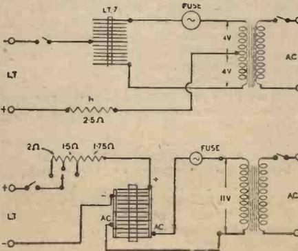
Fig. 2.—The upper circuit is suitable for a trickle charger, while the one below is recommended for greater outputs.
