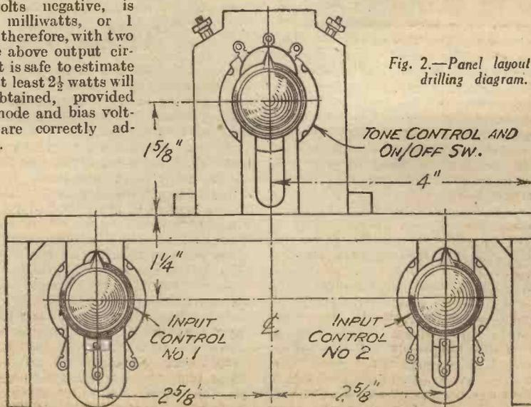
Fig. 2.—Panel layout and drilling diagram.
