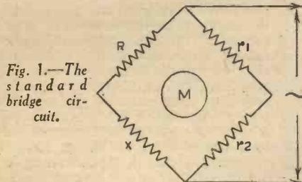
Fig. 1.—The standard bridge circuit.
