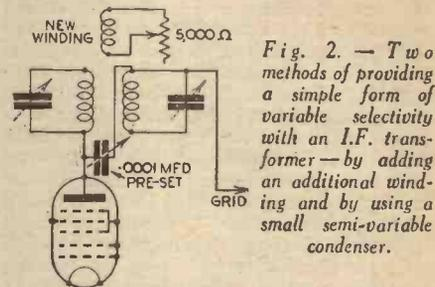
Fig. 2.—Two methods of providing a simple form of variable selectivity with an I.F. transformer—by adding an additional winding and by using a small semi-variable condenser.
