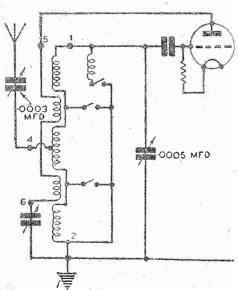
Fig. 1.—Circuit of the Lissen 4-range luner.
