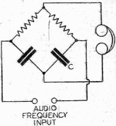
Fig. 2.—Main details of a capacity bridge, C being the capacity under dest.
