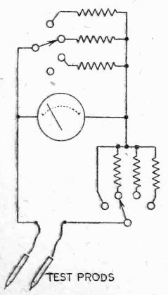
Fig. 1.—Basic principles of a general-purpose lest meter.
