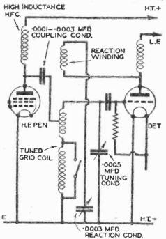
Fig. 1.—The simplest form of H.F. coupling the tuned-grid circuit.
