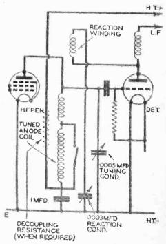
Fig. 3.—Parallel tuned-anode coupling.
