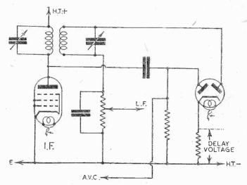
Fig. 3.—These skeleton diagrams show two simple methods of providing delayed A.V.C. action.
