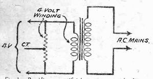
Fig. 1.—Providing an artificial centre-tap on the heater winding of a mains transformer.
