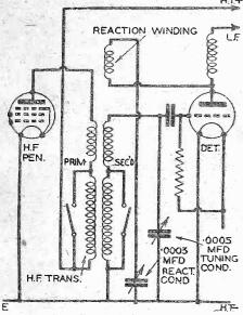
Fig. 4.—H.F. transformer coupling is shown here.
