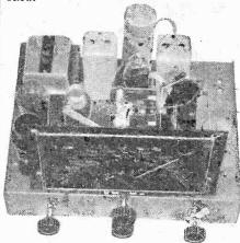
MODEL AW38. S-valve All-wave Superheterodyne chassis. This All-wave Radiogram chassis has resistance capacity coupled push-pull output capable of handling 6 watts, and gives good quality reproduction on both radio and gramophone, for an economical price of 8 gns. Plus 5% war increase.
