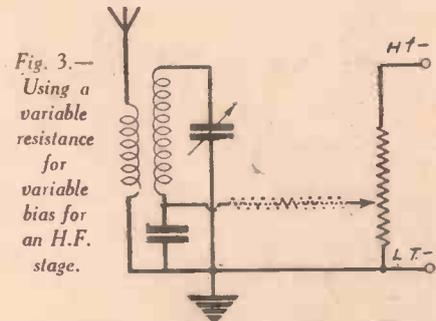
Fig. 3.—Using a variable resistance for variable bias for an H.F. stage.
