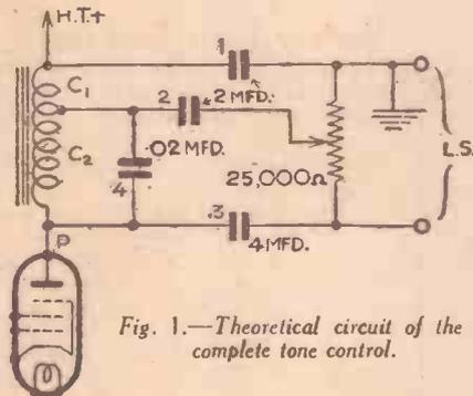
Fig. 1.—Theoretical circuit of the complete tone control.
