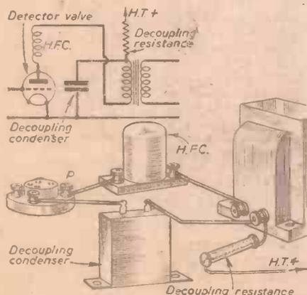
Fig. 2.—Adequate decoupling helps to eliminate distortion due to feed-back.
