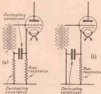
Fig. 4.—The effectiveness of a decoupling arrangement can be increased by adding another condenser in parallel.
