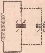
Fig. 1.—The standard signal-frequency tuned circuit.
