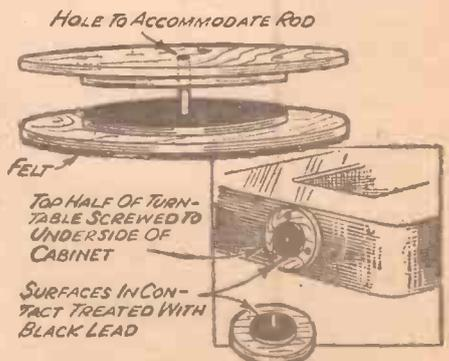
Fig. 4.—Turntables are simple to add to portable receivers.
