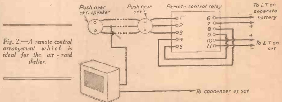
Fig. 2.—A remote control arrangement which is ideal for the air-raid shelter.
