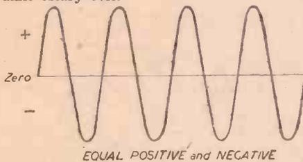
Fig. 1.—Curve of a radio-frequency wave representing an unmodulated signal.
