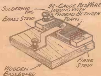
Fig. 3.—This illustration shows the constructional details of the 10 ohm variable resistance described.
