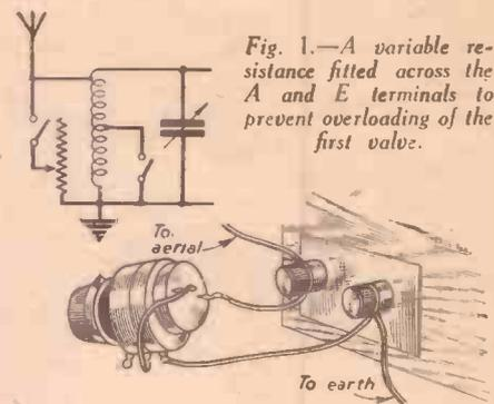
Fig. 1.—A variable resistance fitted across the A and E terminals to prevent overloading of the first valve.
