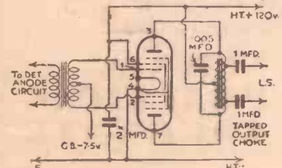
Fig. 4.—A Q.P.P. stage which can be used in a portable with good results.
