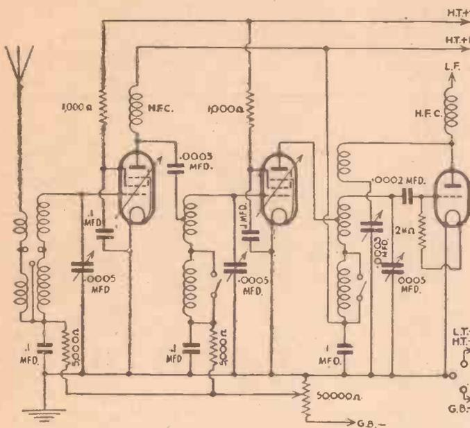
Fig. 1.—Skeleton circuit of a 2 H.F. amplifier with asymmetrical tuning circuits.
