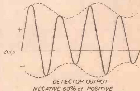
Fig. 6.—Rectified signal curve having a component as shown in Fig. 2.
