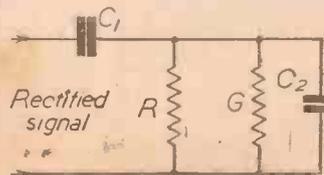
Fig. 2.—The elements of R.C. coupling shown as a network.
