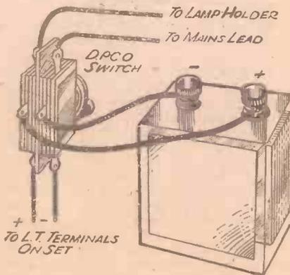
Fig. 2.—The switching system for transferring the accumulator leads from the set to the charger when the former is out of use.
