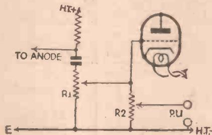
Fig. 3.—In this arrangement signals may be superimposed on those present at the grid.
