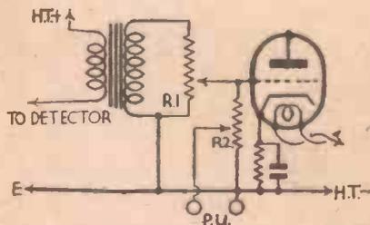
Fig. 1.—A simple fading circuit for radio and gramophone.
