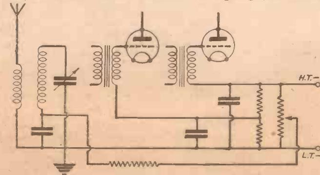
Fig. 4.—Complete biasing scheme, one variable H.F. bias circuit, and 2 L.F. circuits.
