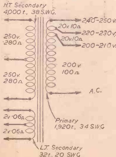
Fig. 2.—Approximate figures relating to a typical transformer of good design.
