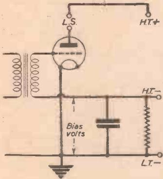
Fig. 1.—The normal method of providing auto-bias for an output stage.
