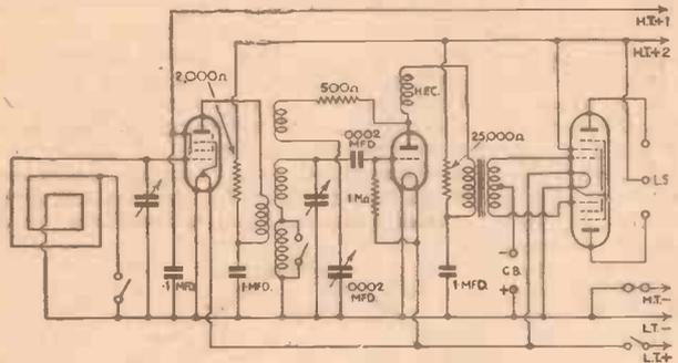
Fig. 5.—Circuit of a 3-valve portable. An H.F. pentode, detector and double output pentode are used.
