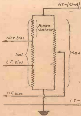
Fig. 5.—Using a ballast resistance to simplify calculations in the bias circuit.
