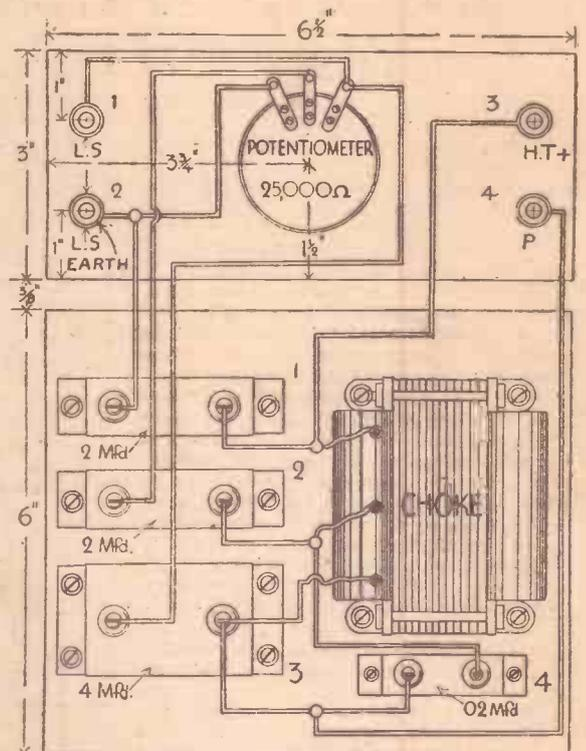
Fig. 2.—Wiring diagram showing components and layout.
