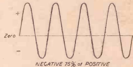
Fig. 3.—In this curve the negative voltage is 75% of the positive.
