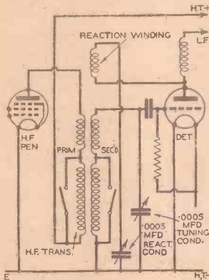
Fig. 4.—An intervalve coupling circuit which combines the advantage of tuned-grid and tuned-anode—the tuned H.F. transformer arrangement.
