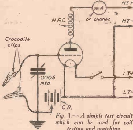
Fig. 1.—A simple test circuit which can be used for coil testing and matching.
