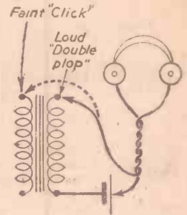
Fig. 1.—Method of making preliminary tests with an L.F. transformer.
