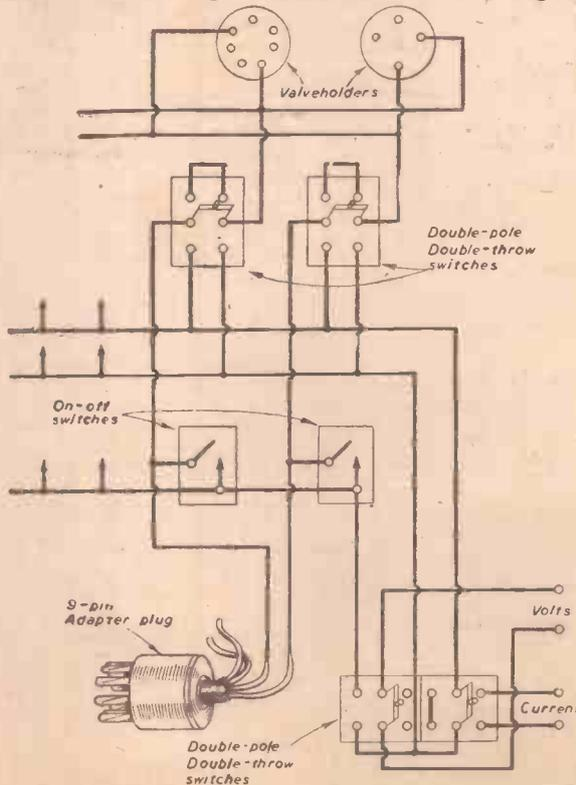
Skeleton circuit of the set analyser. Other valveholders to complete the range are added in parallel, with additional switches.
