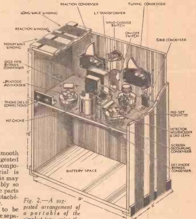
Fig. 2.—A suggested arrangement of a portable of the simplest type using the circuit given in Fig. 1. Dimensions are approximate and will have to be modified according to the batteries employed and if a speaker is to be accommodated.
