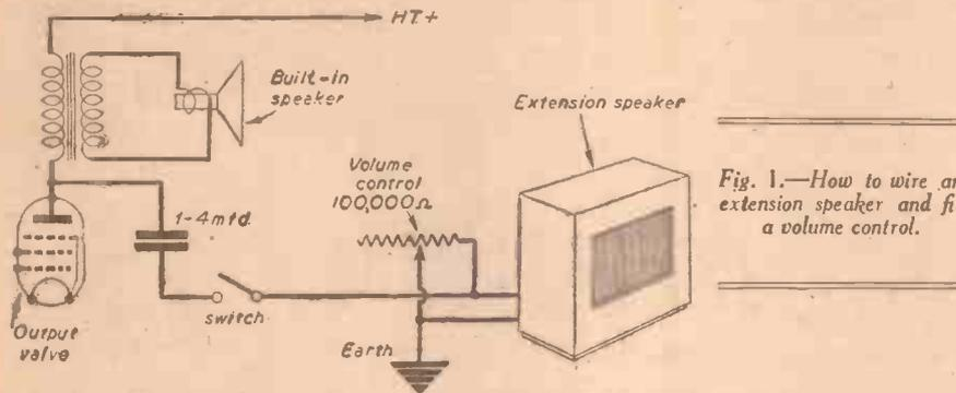
Fig. 1.—How to wire an extension speaker and fit a volume control.
