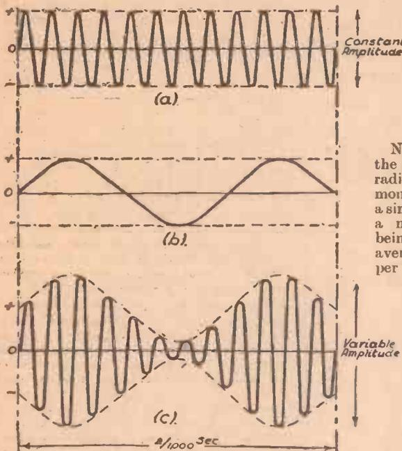
Fig. 1.—Diagrams illustrating the combination of L.F. and H.F. waves to give a modulated H.F. wave.
