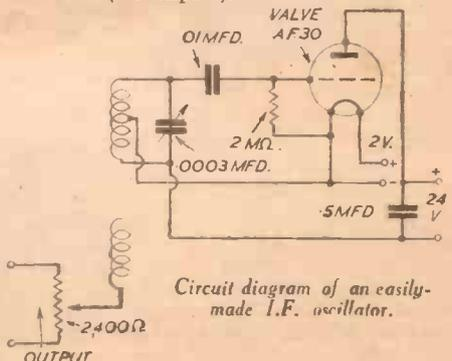
Circuit diagram of an easily-made I.F. oscillator.
