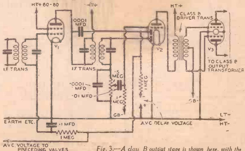
Fig. 3.—A class B output stage is shown here, with the triode section of a D.D.T. valve acting as driver
