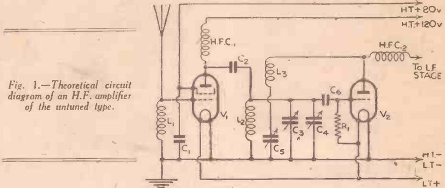
Fig. 1.—Theoretical circuit diagram of an H.F. amplifier of the untuned type.
