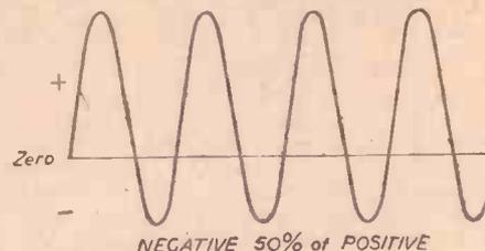
Fig. 2.—This curve represents a signal which has a negative voltage 50% of the positive.
