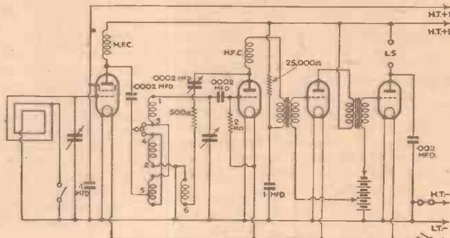
Fig. 6.—A 4-valve portable which can be built from spare parts.
