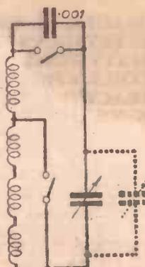
Fig. 4.—The oscillator circuit when a special shaped-plate tuning condenser is used.
