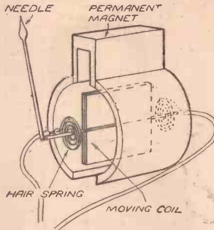
The essential parts of a moving-coil meter are shown here. Note hair-spring connections to coil.
