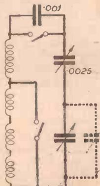
Fig. 3.—This is an oscillator circuit employing a standard tuning condenser.
