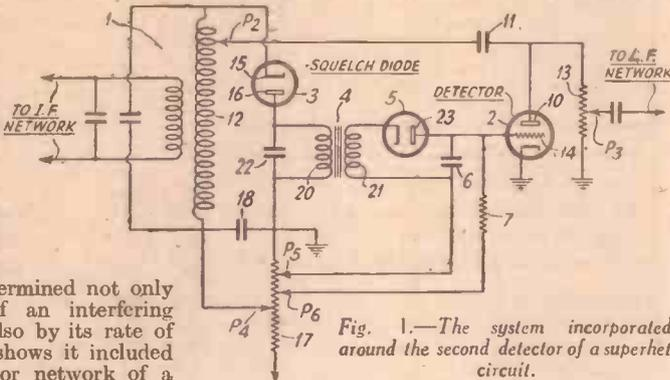
Fig. 1.—The system incorporated around the second detector of a superhet circuit.
