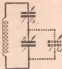
Fig. 2.—This is the equivalent oscillator tuned circuit.
