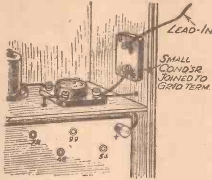
Fig. 1.—A series aerial condenser and an add-on aerial for a portable.
