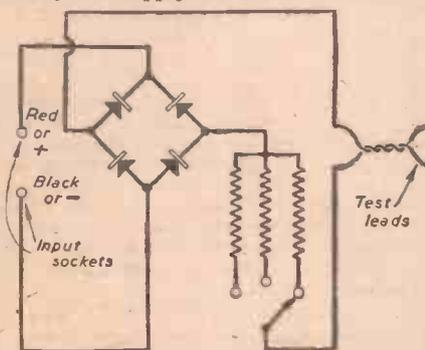
Fig. 1.—Theoretical circuit of the A.C. unit.
