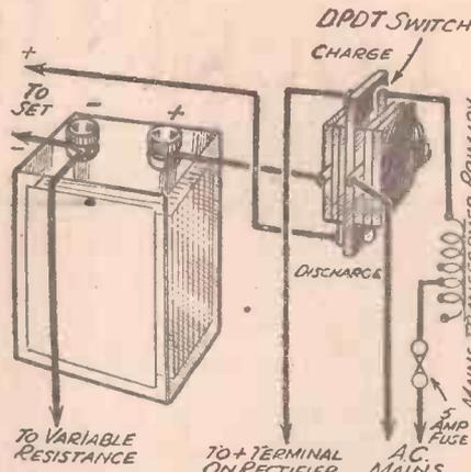
Fig. 5.—The switching system required when using an A.C. trickle charger.
