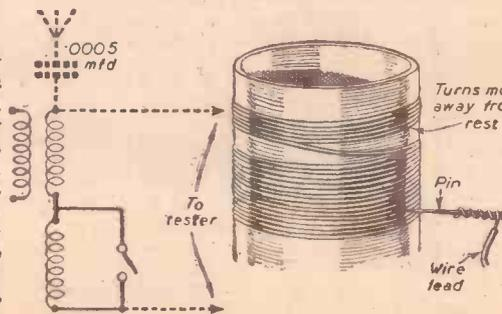
Fig. 2.—Method of connecting the coils to the test circuit.
