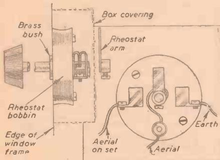
An improvised semi-rotary aerial-earthing switch.
