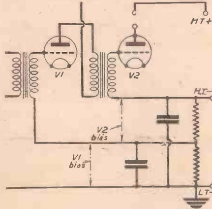
Fig. 2.—Bias for two stages may be obtained as shown above. Two resistors or a tapped component may be used.
