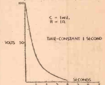
Fig. 2.—Discharge curve of the grid circuit.
