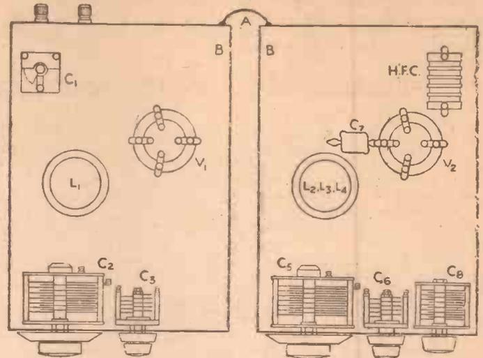
Fig. 3.—A suggested layout capable of providing efficient screening.
