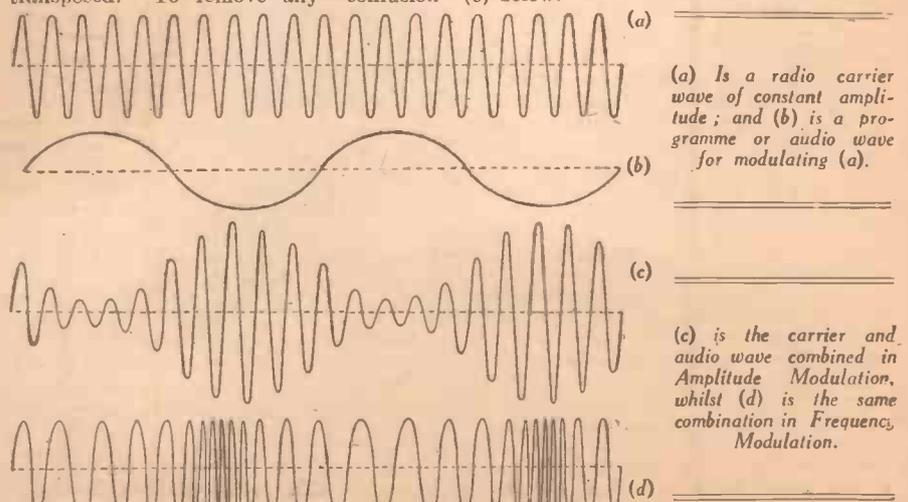
(a) Is a radio carrier wave of constant amplitude; and (b) is a programme or audio wave for modulating (a).
