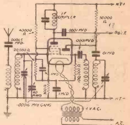
Fig. 2.—A triode-hexode frequency-changing stage for A.C. mains use.
