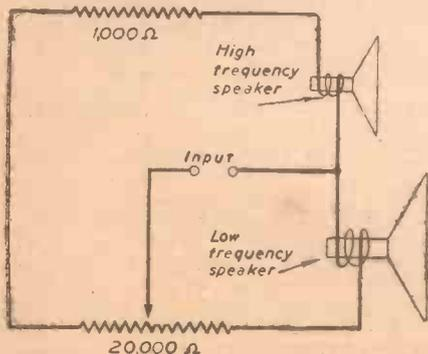
A tone control circuit for two loudspeakers.
