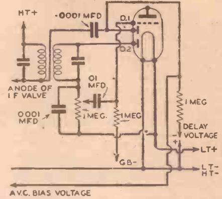
Fig. 2.—This is a delayed A.V.C. circuit.
