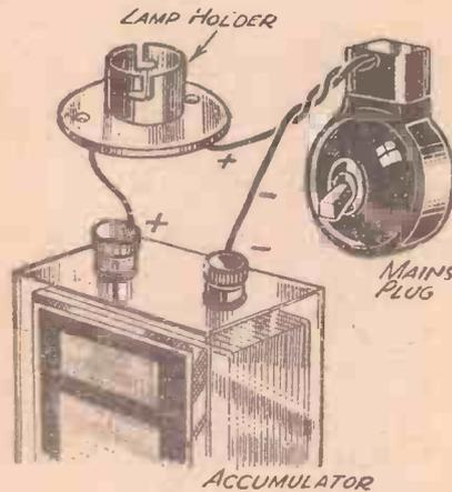
Fig. 1.—Showing the simple arrangement of a trickle charger for use on D.C. mains.
