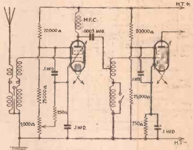
Fig. 4.—An alternative scheme with control of the first valve only.
