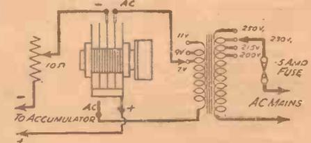
Fig. 4.—The circuit required when using the Westinghouse L.T. 2 rectifier.
