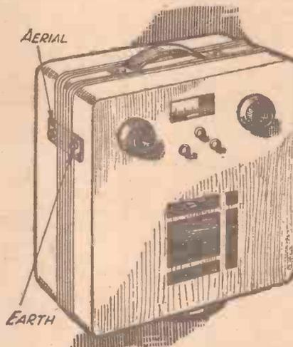
Fig. 2.—Another way of adding an external aerial to a portable.
