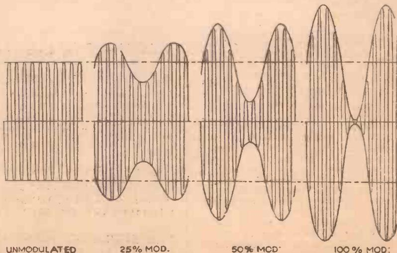
Fig. 2.—Curves illustrating the different degrees of modulation.
