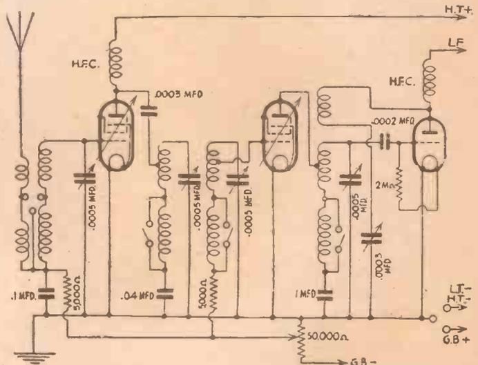
Fig. 2.—Band-pass tuning is here incorporated between the H.F. stages.
