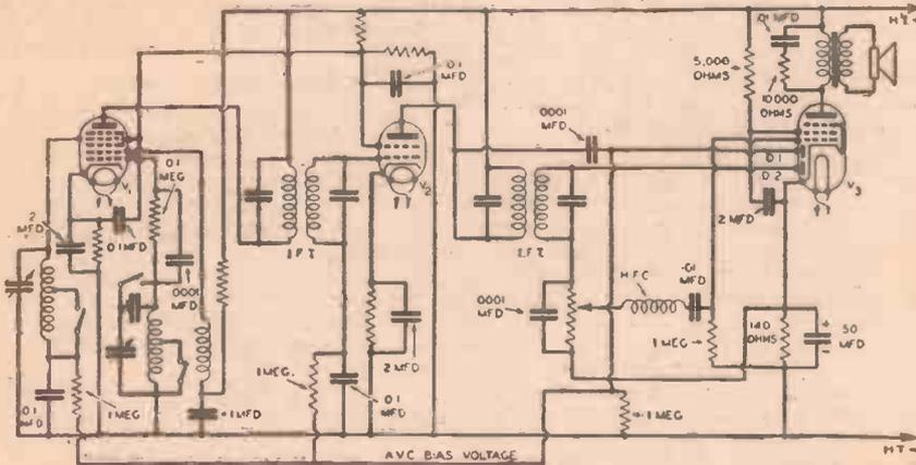
Fig. 1.—An A.C. three-valve superhet circuit with A.V.C.
