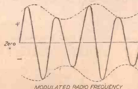
Fig. 5.—The curve of a modulated R.F. signal.
