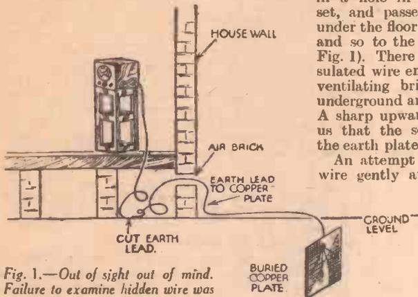
Fig. 1.—Out of sight out of mind. Failure to examine hidden wire was responsible for this unusual fault.
