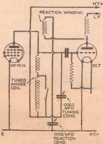
Fig. 2.—The simplest form of tuned-anode circuit in which the tuning condenser is connected in parallel with the anode coil (the same type may be used as in a tuned-grid circuit).
