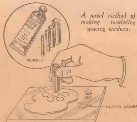
A novel method of making insulating spacing washers.
