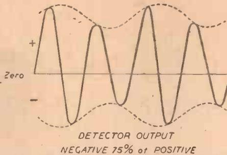
Fig. 7.—Curve of the detector output with a 75% negative voltage.
