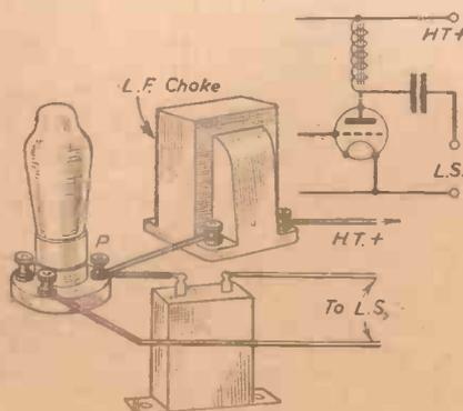
Fig. 3.—Showing how a simple choke-filter system provides decoupling for the output stage.
