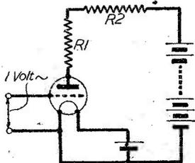
Fig. 1.—The resistance  $R_1$  represents the valve resistance and  $R_2$  the external load.
