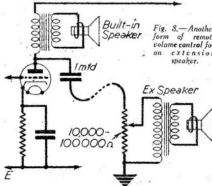
Fig. 8.—Another form of remote volume control for an extension speaker.
