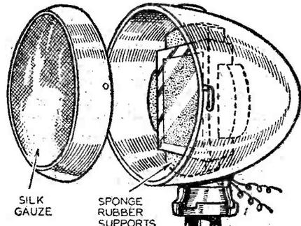
Fig. 3.—The method of housing the microphone used by the designer.
