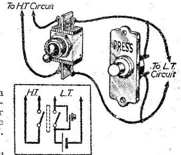
An efficient arrangement of H.T. and L.T. switching.
