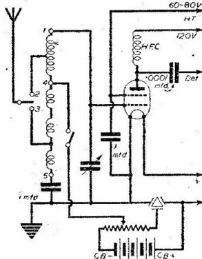
Fig. 14.—The circuit of an H.F. stage using a variable- $\mu$  valve. An H.F. pentode can be substituted for the S.G. valve if desired.
