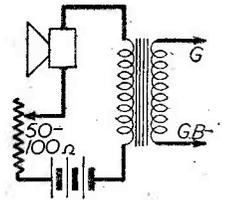
Fig. 3.—A method of L.F. volume control which can sometimes be used conveniently with a microphone.
