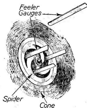
Fig. 2.—The method of centring a speaker cone by the use of three feeler gauges of equal thickness. The screw in the centre of the "spider" is tightened only when the feelers have been inserted between the inside of the speech coil and the pole-piece.
