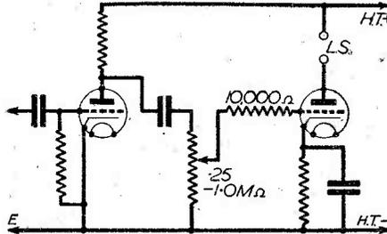
Fig. 2.—A form of volume control similar to that shown in Fig. 1, but for an R.C.C. stage. A grid stopper resistor is also shown.
