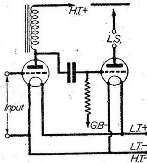
Fig. 2.—By using L.F. choke coupling excessive voltage drop in the anode circuit is avoided.
