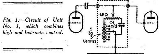
Fig. 1.—Circuit of Unit No. 1, which combines high and low-note control.
