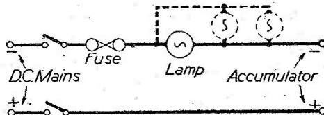
Fig. 2.—A standard L.T. charging circuit and layout suitable for use with D.C. mains. The double-pole on-off switch is essential.
