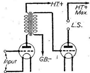
Fig. 3.—A normal transformer coupling which offers low D.C. resistance to the H.T.
