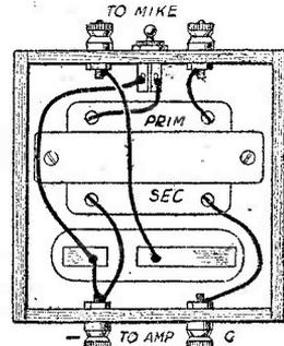
Fig. 5.—The transformer and battery can be housed in a neat case as shown here.
