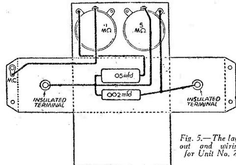
Fig. 5.—The layout and wiring for Unit No. 2.
