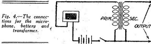
Fig. 4.—The connections for the microphone, battery and transformer.
