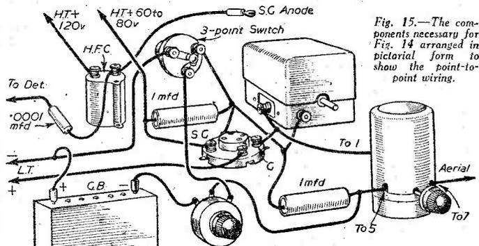
Fig. 15.—The components necessary for Fig. 14 arranged in pictorial form to show the point-to-point wiring.
