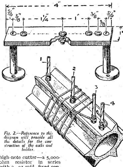
Fig. 2.—Reference to this diagram will provide all the details for the construction of the coils and holder.
