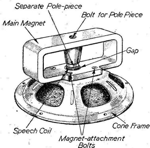
Fig. 1.—Some details of a representative permanent-magnet moving-coil speaker which are referred to in the text.
