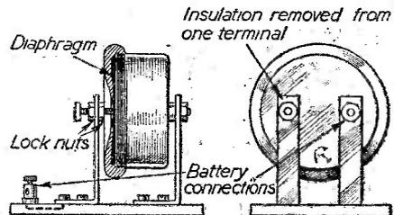
Two views of a simple buzzer made with an old earphone.
