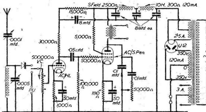
Circuit diagram of J. Richardson's two-valve amplifier.
