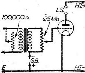
Fig. 1.—Two methods of L.F. volume control. That shown in full lines is often better than that indicated by broken lines.
