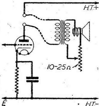
Fig. 7.—Remote volume control for a M.C. speaker.
