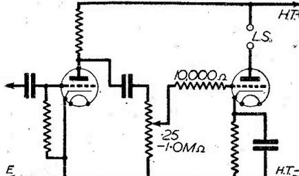
Fig. 2.—A form of volume control similar to that shown in Fig. 1, but for an R.C.C. stage. A grid stopper resistor is also shown.
