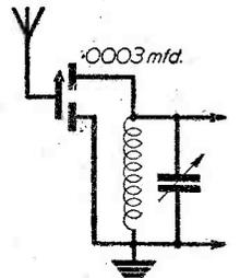
Fig. 5.—Input H.F. volume control by means of a differential condenser.
