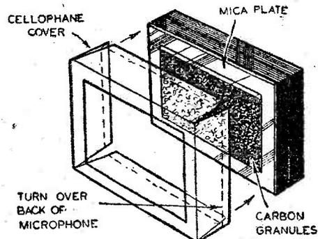
Fig. 2.—Showing how the protective cover of cellophane is cut and lapped over the unit after the granules are in position.
