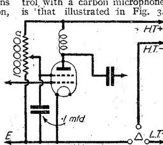
Fig. 4.—H.F. control by varying the voltage on the screening grid of an S.G. valve.
