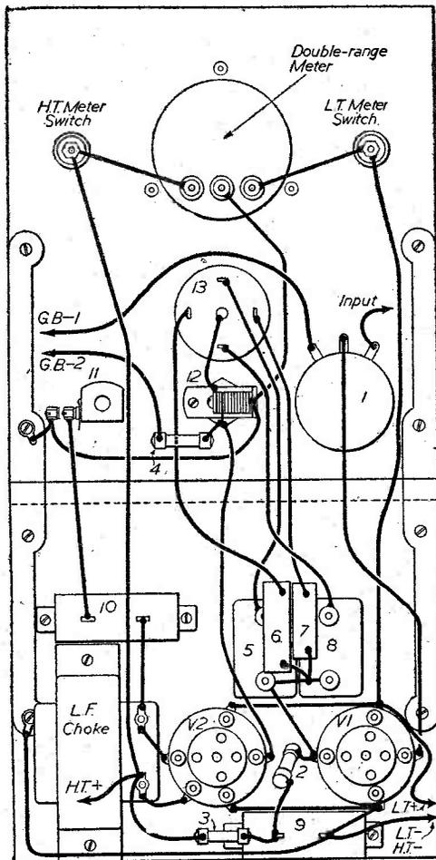
Layout and wiring plan of amplifier. Components are: 1. 0.5 meg. potentiometer; 2. 50,000 ohm resistor; 3. 15,000 ohm ditto; 4. 1 meg. grid-leak; 5, 6, 7, 8. 0.001 mfd., 0.005 mfd., 0.01 mfd. and 0.05 mfd. fixed condensers; 9 and 10. 2 mfd. condensers; 11. Single-circuit jack; 12. Double-circuit ditto; 13. Suitable rotary switch. L.F. choke 25-30 henries.
