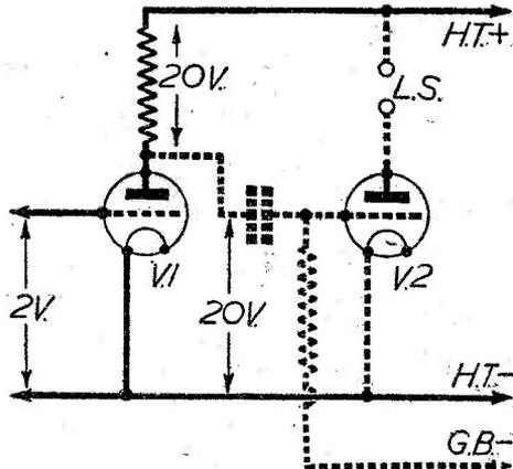
Fig. 1.—This simplified diagram shows how voltage amplification is provided by the triode marked V.1; the amplified signal voltage is passed on to the grid-filament circuit of V.2.
