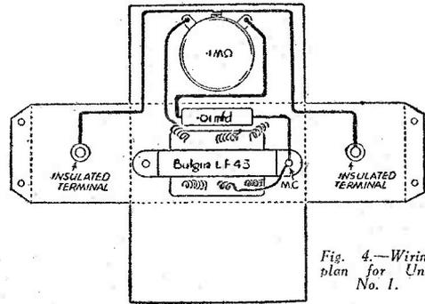
Fig. 4.—Wiring plan for Unit No. 1.
