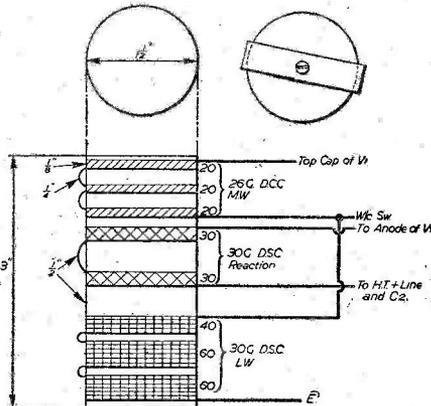
Fig. 1.—Details of the coil for the Universal Oscillator.
