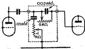
Fig. 2.—This is Unit No. 2's circuit, where separate controls are provided for high and low notes.
