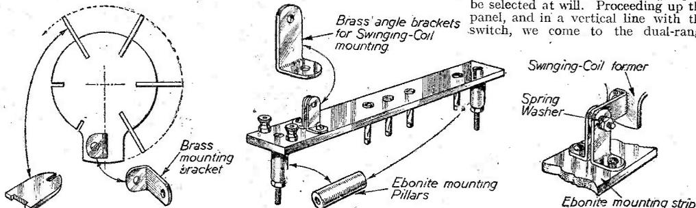
Fig. 3.—(Left) General details of the swinging-coil, for which 9 turns of 24 S.W.G. wire are required. (Right) Shows how the coilholder and the swinging-coil movement is made.
