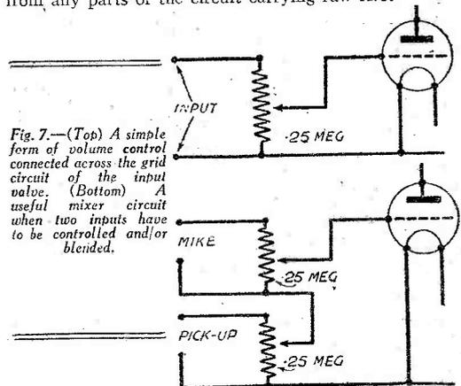
Fig. 7.—(Top) A simple form of volume control connected across the grid circuit of the input valve. (Bottom) A useful mixer circuit when two inputs have to be controlled and/or blended.
