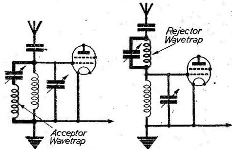
Fig. 2.—An acceptor circuit wave-trap is shown on the left, and a rejector circuit wave-trap on the right. In both cases the wave-trap is shown in heavy lines.
