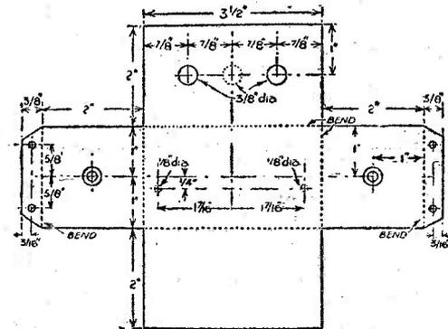
Fig. 3.—Cutting, drilling and bending dimensions for the cases.
