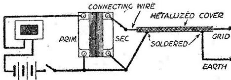
Fig. 6.—The method adopted when a screened connecting cable is used to provide a common negative earth return by means of the metallized covering.
