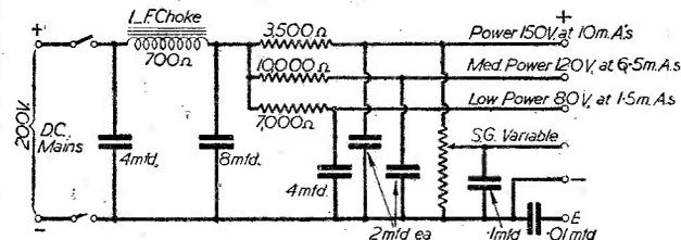
Fig. 1.—An H.T. eliminator for D.C. mains. The values shown are suitable when the unit is to be used with a 3 or 4 valve receiver off 200-220 volts D.C. supplies.
