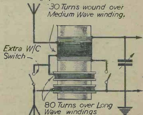
Fig. 7.—How a normal two-range coil, without separate aerial windings, can be modified for use with a doublet.
