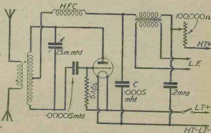
Two super-regenerative circuits. In the top circuit a separate quenching valve is used; this circuit resembles the original Armstrong super-regenerative circuit and is nowadays regarded as obsolete.
