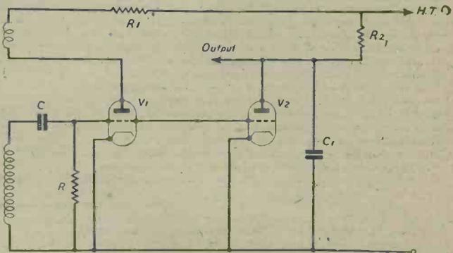
Fig. 16.—An improved circuit designed to overcome the time increase of the fly-back due to the resistance of the coils.
