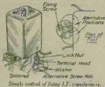
Simple method of fixing I.F. transformers.
