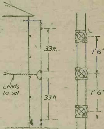
Fig. 3 (left).—Flat-dwellers or those living in a room above ground level in a high building will find that this arrangement of dipole can often be used successfully. It is not ideal as an anti-interference aerial, but is satisfactory for all-wave reception, and sensibly non-directional.
