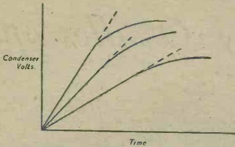
Fig. 10.—Charging curves showing departure from linearity.
