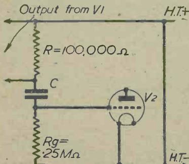
Fig. 4.—This diagram shows that only a percentage of the voltage appearing across the load resistance of  $V_1$  is applied to the grid of  $V_2$ .
