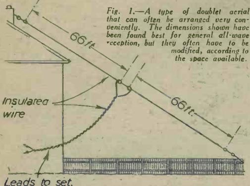
Fig. 1.—A type of doublet aerial that can often be arranged very conveniently. The dimensions shown have been found best for general all-wave reception, but they often have to be modified, according to the space available.
