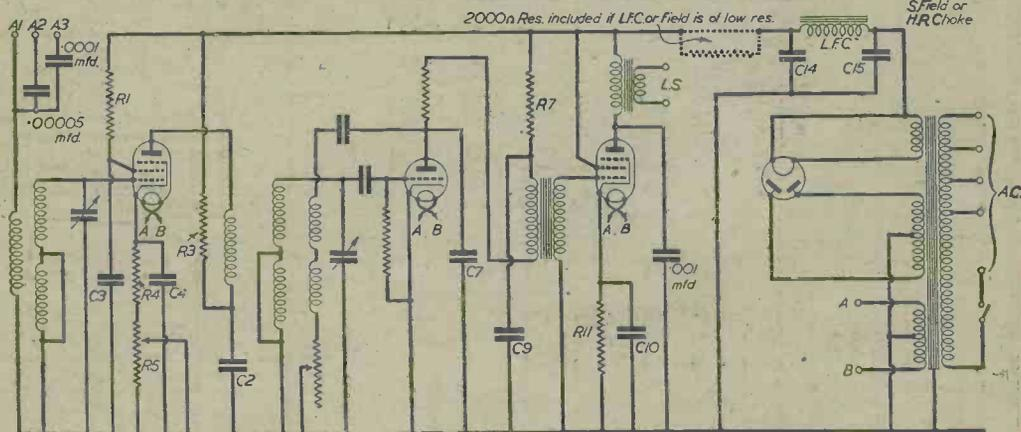
Fig. 2.—Although the basic principles of Fig. 1 have been retained, this circuit is much more simple.
