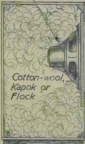
Fig. 4.—"Killing" the air column contained within the cabinet.
