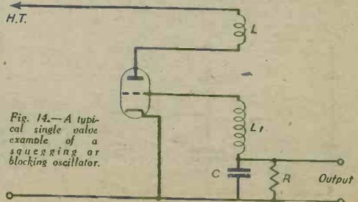
Fig. 14.—A typical single valve example of a squagging or blocking oscillator.
