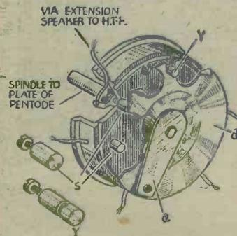
A novel switching arrangement for use with pentodes and extension speakers.
