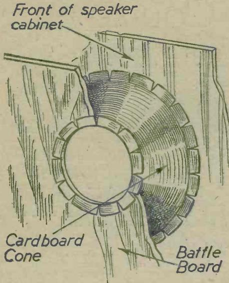
Fig. 6.—The method used for fixing the flare, which the writer made of cardboard.
