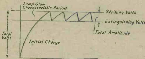
Fig. 13.—Showing the difference between striking and extinguishing volts for a neon lamp.
