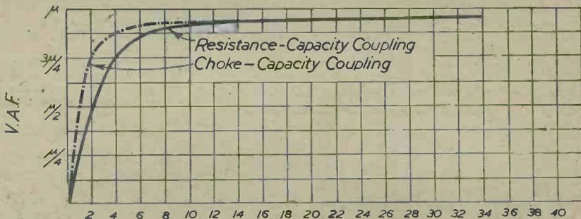
Fig. 3.—Curves which show how the amplification  $R/R_a$  provided by a valve varies with the resistance or reactance of the anode load.
