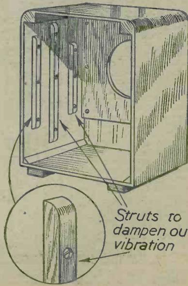
Fig. 2.—Using struts to damp out or eliminate case vibration. They should be fixed firmly in position by screws and glue. Note uneven lengths.
