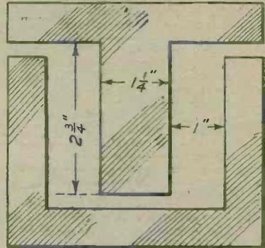
Fig. 1.—The dimensions and pattern of No. 33 stampings as used in the making of the transformer.
