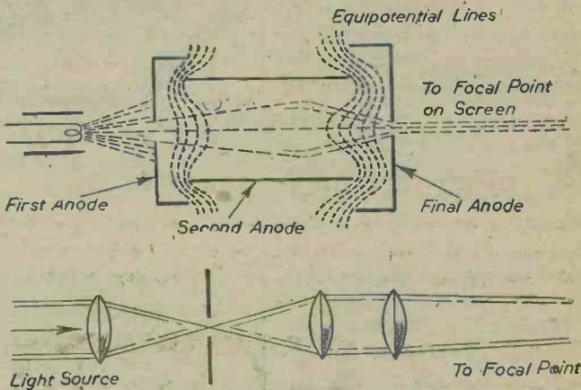
Diagrams illustrating the function of a cathode-ray tube focusing system. (See letter from S. A. Knight.)
