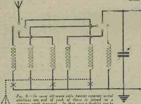
Fig. 6.—In some all-wave coils having separate aerial windings one end of each of these is joined to a common earth terminal. In that case a doublet can be used by breaking the leads marked X and connecting them together, as indicated by the broken line, and to earth.
