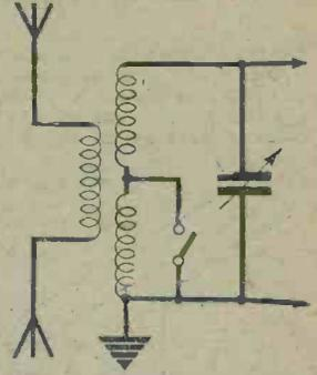
Fig. 5. The two leads from the dipole or doublet should be joined one to each end of a separate winding on the aerial coil, as shown here.
