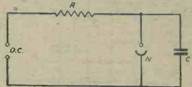
Fig. 12.—A simple electrically controlled oscillator using a neon lamp.
