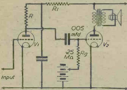
Fig. 1.—Simplified circuit of a two-valve amplifier with R.C. coupling.
