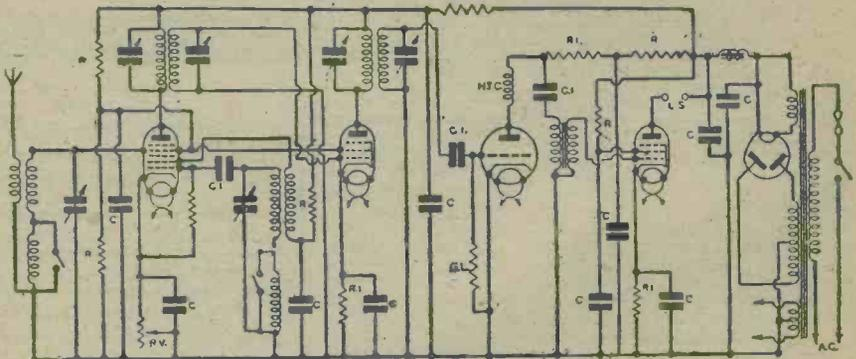
This skeleton circuit of a typical four-valve superhet, with rectifier, is used to show in which parts of the circuit values are most critical.
