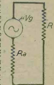
Fig. 2.—The equivalent circuit for  $V_1$  in Fig. 1.  $R_a$  is the internal resistance of the valve,  $R$  is the anode load resistance and  $\mu V_g$  the theoretical output voltage from  $V_1$ .
