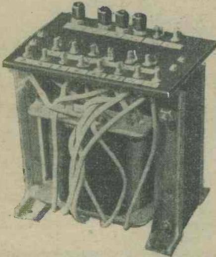
The completed component, showing how the tapping leads are taken to the terminal board.
