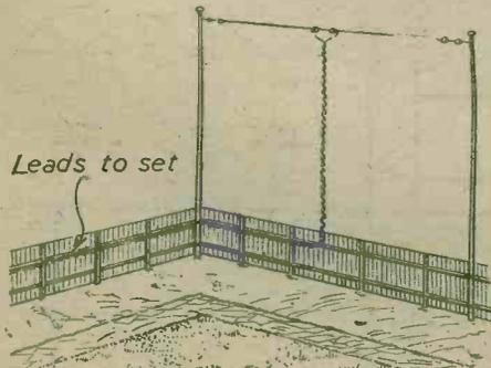
Fig. 2.—How a doublet can sometimes be erected between two masts at the end of the garden so that it is well away from the source of interference. In this case the aerials' span can rarely be more than 33ft. each, the total length of the lead-in being 66ft.
