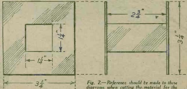
Fig. 2.—Reference should be made to these diagrams when cutting the material for the construction of the bobbin.
