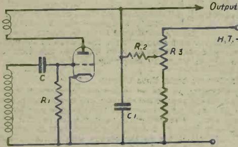
Fig. 15.—Another form of squegging oscillator, having a slightly different operation to Fig. 14.
