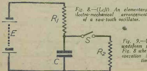
Fig. 8.—(Left) An elementary electro-mechanical arrangement of a saw-tooth oscillator.
