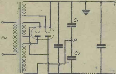
Fig. 7.—A valve voltage doubling rectifier circuit, using a Cossor 225D.U.
