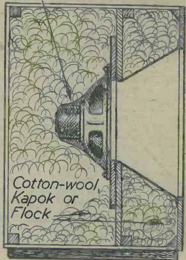
Fig. 5.—A recessed baffle-board plus short horn is very effective, as better loading of the cone is obtained and cabinet troubles are reduced.
