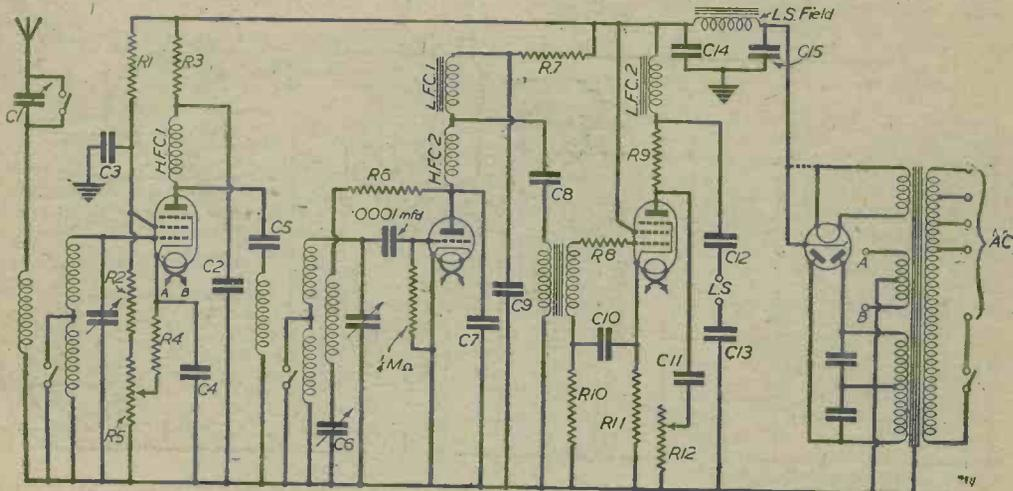
Fig. 1.—A typical four-valve A.C. circuit; but many refinements have been added in order to illustrate points in this article.
