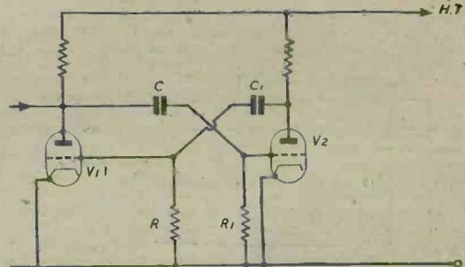
Fig. 17.—Simplified circuit of the Multi-vibrator or Kipp Relay.
