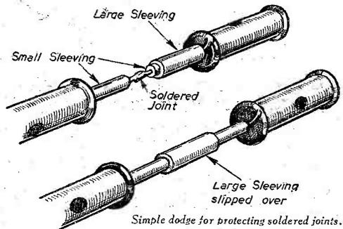
Simple dodge for protecting soldered joints.
