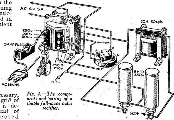
Fig. 4.—The components and wiring of a simple full-wave valve rectifier.
