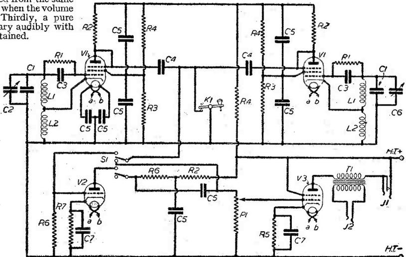
Fig. 1.—The theoretical circuit of the unit in which V1 and V1 are the two electron-coupled oscillators responsible for the audible note.
