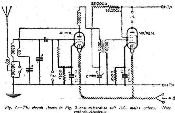
Fig. 3.—The circuit shown in Fig. 2 now altered to suit A.C. mains valves. Note cathode circuits.
