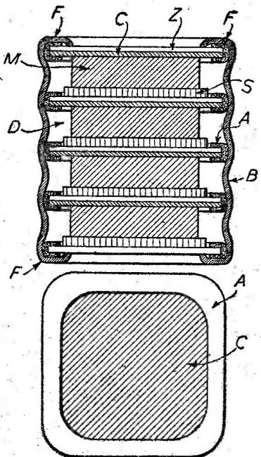
Figs. 1 and 2.—Sectional elevation and plan of an improved dry battery, showing how effective inter-cell sealing is obtained.
