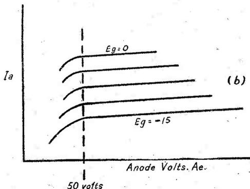
Fig. 19. (a) A pentode used as a constant current device; (b) Showing how the anode current remains reasonably constant independent of voltage.
