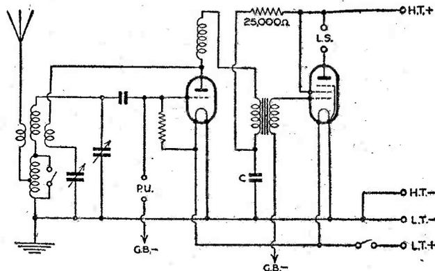
Fig. 2.—A typical 2-valve battery-operated circuit which lends itself to easy conversion.
