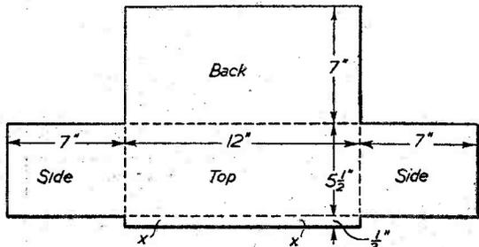
Fig. 13.—The perforated zinc used for the cover should be marked out as shown here.
