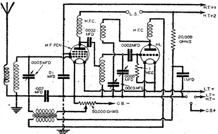
Fig. 2.—The above circuit is a suggestion for a reflex circuit employing modern components. Broken line shows an alternative earth connection, which should be tried.
