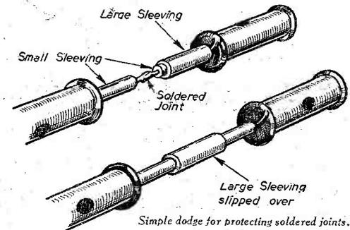
Simple dodge for protecting soldered joints.
