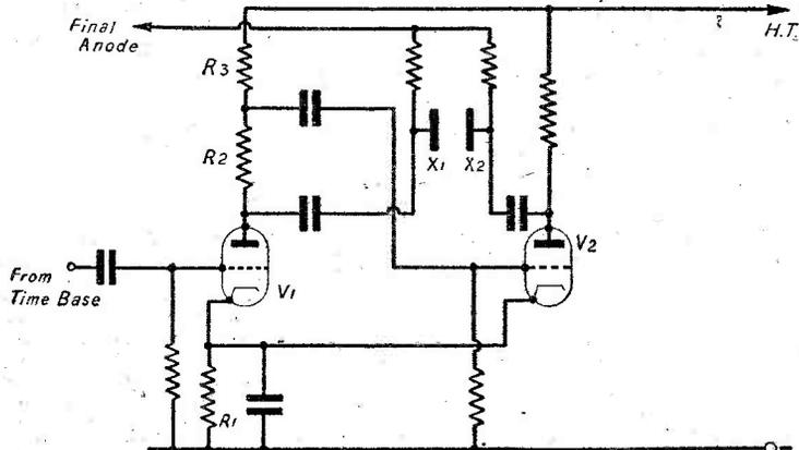
Fig. 23.—An amplifier circuit which can be introduced between the time base output and the X plates of the tube.
