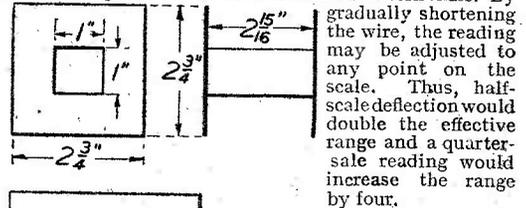
Fig. 2 (Top left).—The measurements of the parts required for the bobbin.
