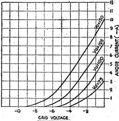
Fig. 1.—Static characteristics of a typical general purpose battery-operated valve.
