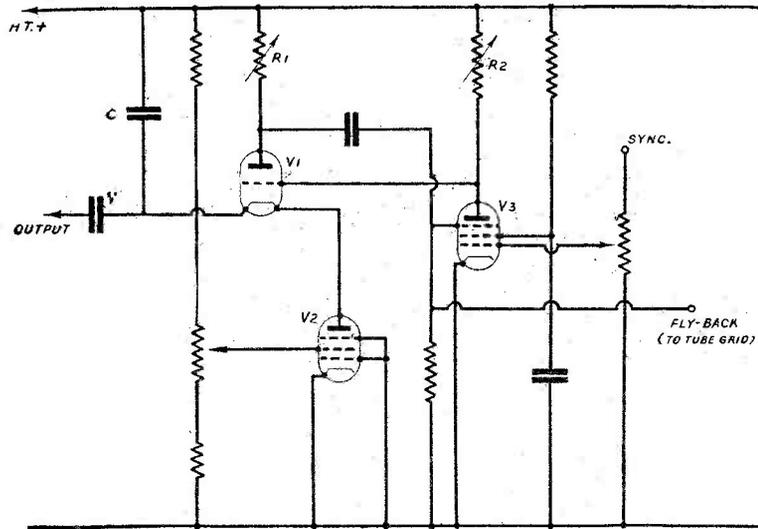
Fig. 21.—The Puckle hard-valve time-base circuit capable of providing stable operation over a very wide frequency range.
