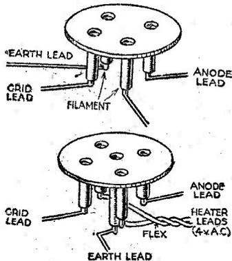
Fig. 1.—Shows how the valve-holder connections have to be altered to suit A.C. mains valves.
