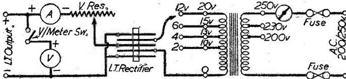
Fig. 1.—The complete circuit of the charger, showing the secondary voltages for accumulators of various voltages.
