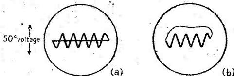
Fig. 20.—The effect produced if steps are not taken to suppress the cathode beam during discharge.
