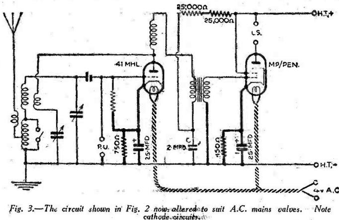
the G.B.— terminal on the L.F. transformer and the earth line, the cathode by-pass condenser being connected between one end of the decoupling resistance and the cathode of the valve.
