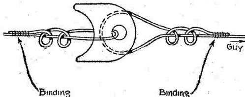
This shows the correct method of connecting the halyard and aerial to a shell-type insulator
