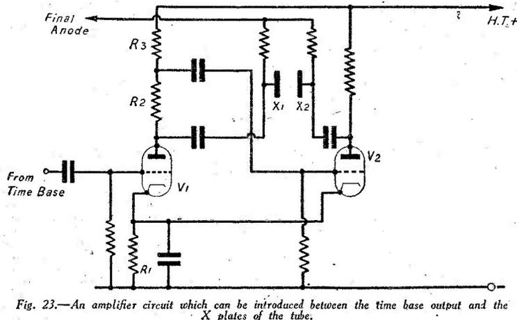
Fig. 23.—An amplifier circuit which can be introduced between the time base output and the X plates of the tube.
