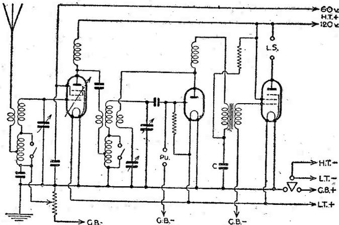
Fig. 5.—This is representative of 3-valve battery circuits of the 1-V-1 type. Compare it with Fig. 6.
