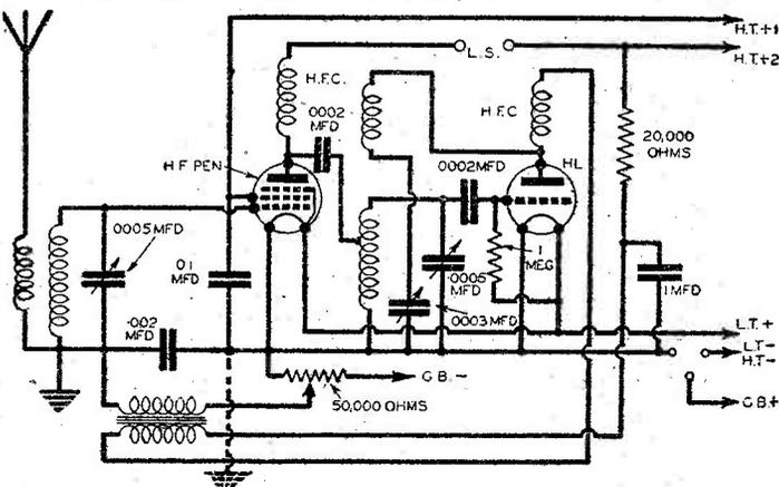
Fig. 2.—The above circuit is a suggestion for a reflex circuit employing modern components. Broken line shows an alternative earth connection, which should be tried.
