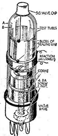
A novel coil assembly, using test tubes.
