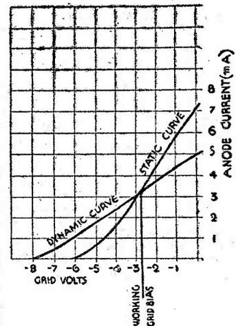
Fig. 2.—Static and dynamic curve forms.
