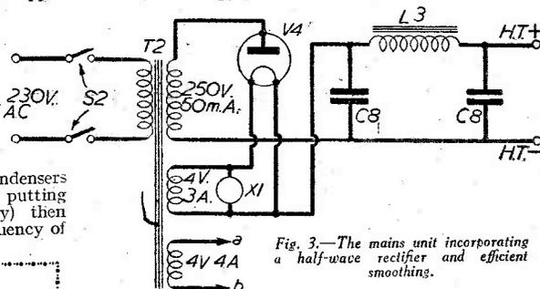
Fig. 3.—The mains unit incorporating a half-wave rectifier and efficient smoothing.
