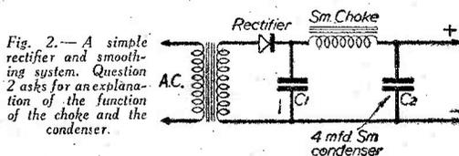
Fig. 2.—A simple rectifier and smoothing system. Question 2 asks for an explanation of the function of the choke and the condenser.
