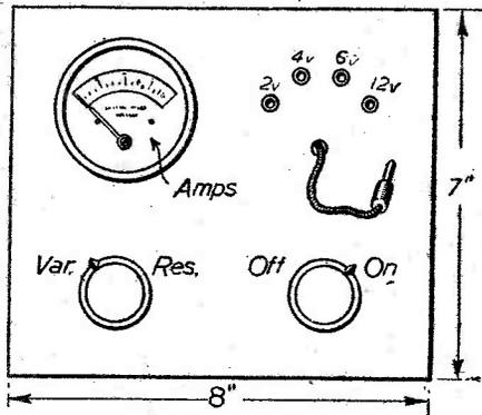
Fig. 4.—Dimensions and layout of the panel if the voltmeter is not used.
