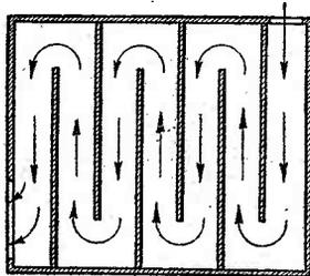
Fig. 7.—The fundamental arrangement to secure a folded back air column.
