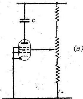
Fig. 19. (a) A pentode used as a constant current device; (b) Showing how the anode current remains reasonably constant independent of voltage.
