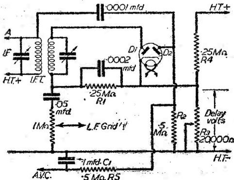
Fig. 1.—A double-diode used for second detection and to provide delayed A.V.C. for the preceding H.F. and I.F. stages.
