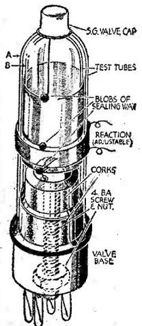
A novel coil assembly, using test tubes.
