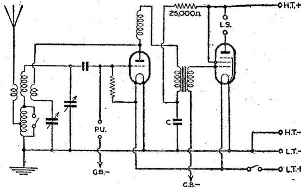
Fig. 2.—A typical 2-valve battery-operated circuit which lends itself to easy conversion.
