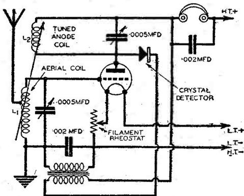
Fig. 1.—An early type of reflex circuit, in which use was made of a crystal as the detector.
