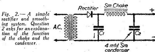
Fig. 2.—A simple rectifier and smoothing system. Question 2 asks for an explanation of the function of the choke and the condenser.
