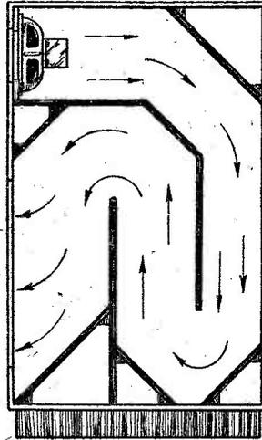
Fig. 9.—The system applied to a large cabinet. Note the gradual increase in width of the air column.
