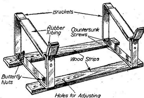
A radio-chassis cradle of simple construction.
