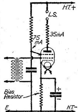
Fig. 4.—The circuit of an output tetrode using cathode biasing. It is required to find the correct value for the bias resistor.
