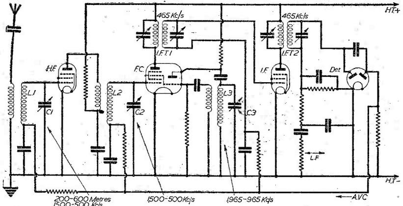
This skeleton circuit of the first four valves of a typical good-class superhet shows the frequency ranges of the tuning circuits. L<sub>1</sub> and C<sub>1</sub>, and L<sub>2</sub> and C<sub>2</sub> cover the signal-frequency range, while L<sub>3</sub> and C<sub>3</sub> cover the corresponding oscillator frequency range. The two 465 kc/s I.F. transformers are marked I.F.T.1 and I.F.T.2.
