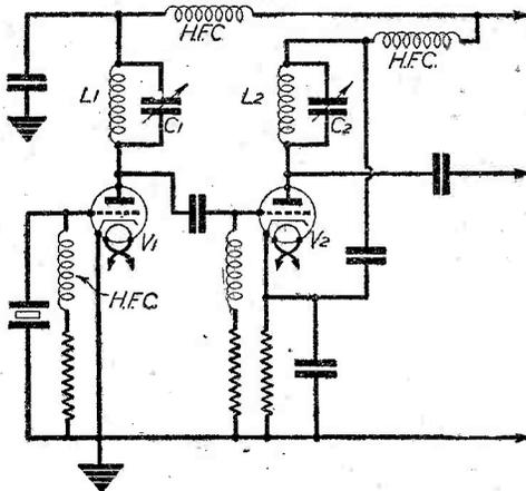
Fig. 3.—A simple frequency-doubling circuit. V.1 is a crystal oscillator, the anode circuit of which is tuned to the crystal frequency by L.1 and C.1. V.2 is the doubler, and L.2 and C.2 tune to twice the crystal frequency.
