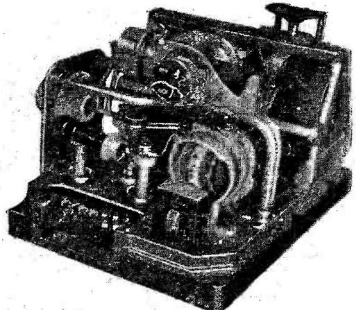
*Top view of aerial tuning unit, showing one of the variometers and the sturdy method of construction.*
