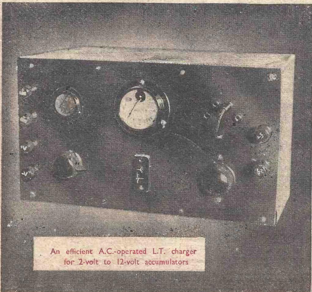
An efficient A.C.-operated L.T. charger
