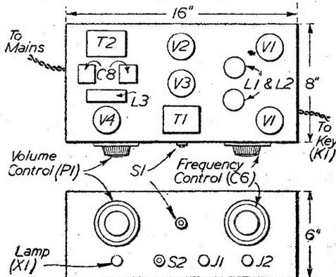
Fig. 2.—The actual layout, as used by the writer of the article. Note positions of V1 and V1.
