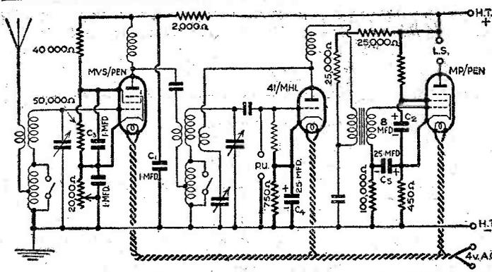
Fig. 6.—The circuit modified for A.C. supplies, variable bias being provided for the H.F. valve.
