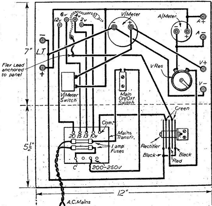
The detailed wiring diagram of the charger, showing the location of the component parts.
