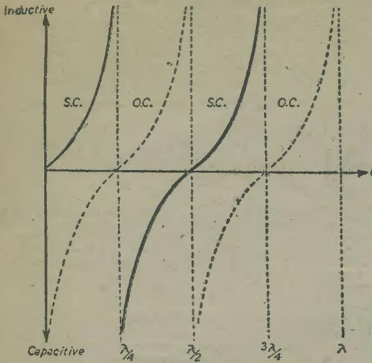
Fig. 16.—Curves showing variations of  $z_i$  as length of line is varied, for open- and short-circuited cases.
