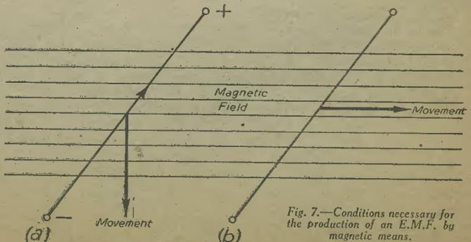
Fig. 7.—Conditions necessary for the production of an E.M.F. by magnetic means.
