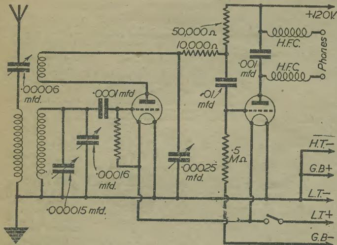
Here is the circuit of the receiver. Quite simple and very efficient.
