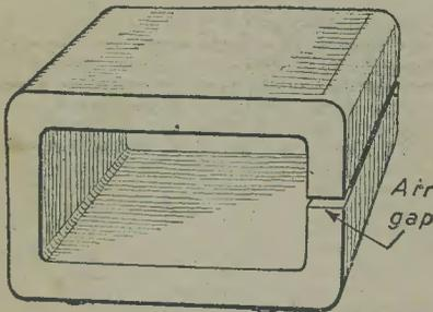
Fig. 1.—A typical meter magnet.
