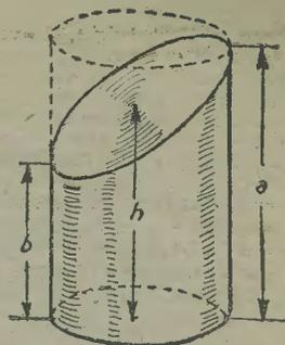
Fig. 15.—Cylinder and frustum of cylinder.
