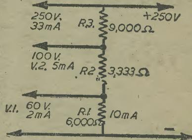
Fig. 5.—A potential divider made up from three separate fixed resistors, and used for regulating a H.T. supply from a rectifier.
