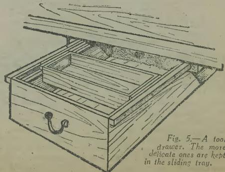
Fig. 5.—A tool drawer. The more delicate ones are kept in the sliding tray.
