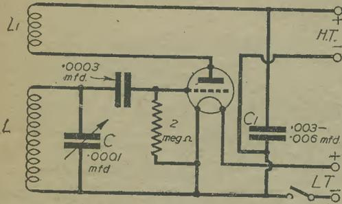
Fig. 1.—A simple heterodyne circuit utilising a triode valve and fixed "throttle" control.
