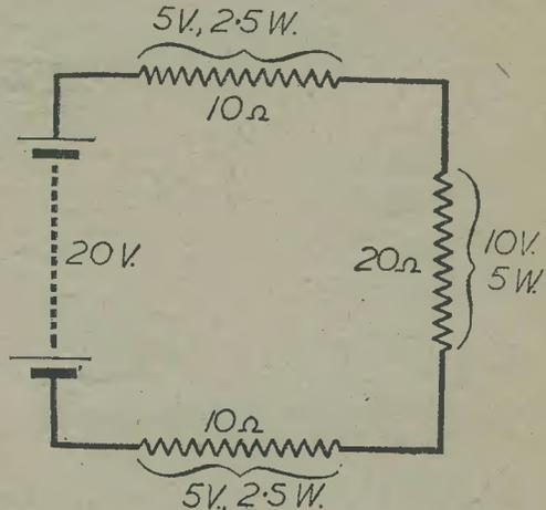
Fig. 2.—An "equivalent" circuit to that in Fig. 1, showing the distribution of voltage and power dissipation.
