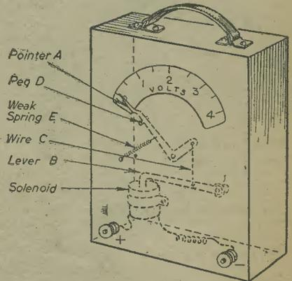
A useful voltmeter made from odd parts.
