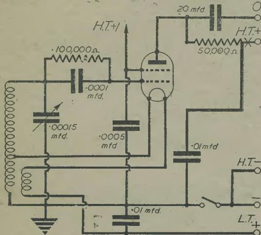
Fig. 3.—The battery operated counterpart of Fig. 2. Note the filament circuit.
