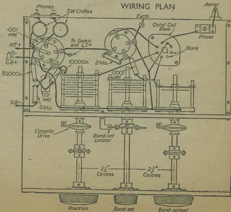
it can only be regarded as a substitute. The method of arranging the bandspread condenser's pointer and dial is not shown, as this is a matter for individual preference. The band-set condenser should be equipped with one of the small knobs supplied with the epicyclic drives and a scale marked from 1-14. These details will become apparent when the actual components are to hand.
