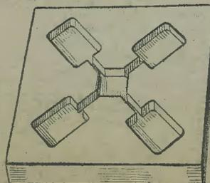
Fig. 2.—Mould base.
