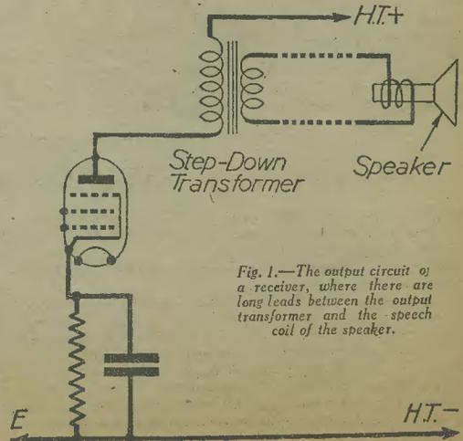
Fig. 1.—The output circuit of a receiver, where there are long leads between the output transformer and the speech coil of the speaker.
