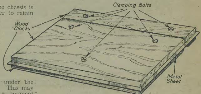
Fig. 3.—Showing how the metal is clamped between pieces of hard wood prior to bending.
