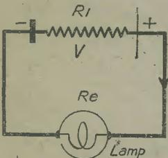
Fig. 8.—The effect of the internal resistance of a cell.
