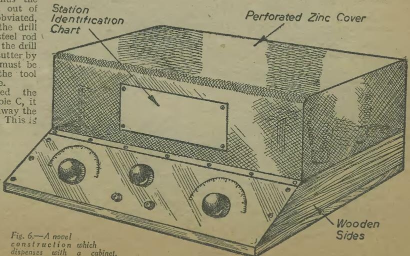
Fig. 6.—A novel construction which dispenses with a cabinet.
