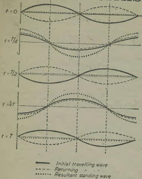
Fig. 8.—Voltage standing waves set up by the travelling and reflected components.
