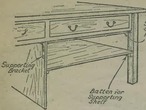
Fig. 1.—A shelf enables the batteries and/or mains unit to be kept out of harm's way. A curtain covers the front to protect them from dust, etc.
