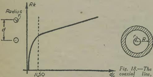
Fig. 18.—The coaxial line, where  $Rk = 138 \log_{10} R/r$ .
