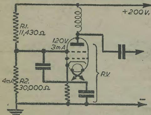
Fig. 1.—A fixed potentiometer, comprising R.1 and R.2, used to supply the screening-grid voltage to an H.F. tetrode.
