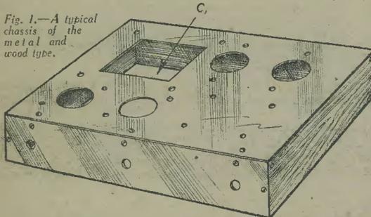
Fig. 1.—A typical chassis of the metal and wood type.
