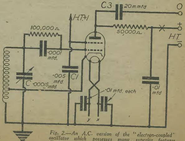
Fig. 2.—An A.C. version of the "electron-coupled" oscillator which possesses many superior features. For most satisfactory adjustment, the screening-grid voltage should be obtained via a potentiometer.
