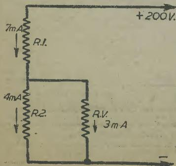
Fig. 2.—(Left) An equivalent circuit to that in Fig. 1. It shows how the current is distributed.
