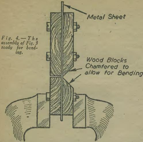
Fig. 4.—The assembly of Fig. 3 ready for bending.
