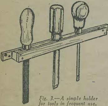
Fig. 3.—A simple holder for tools in frequent use.
