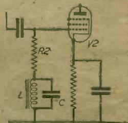
Fig. 2.—Bass-boost is obtained by connecting an oscillatory circuit in series with the grid leak.
