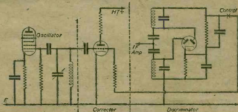
Fig. 4.—Skeleton diagram showing the general arrangement of a simple system of automatic frequency correction.
