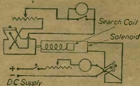
Fig. 5.—Circuit details and connections for the ballistic galvanometer test.
