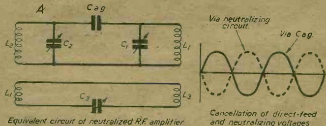
Fig. 26.—Neutralising principle, equivalent circuit and graphical form.
