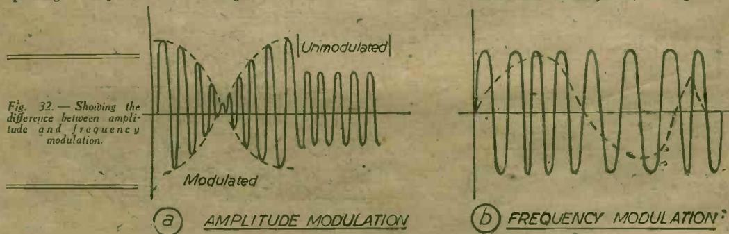
Fig. 32.—Showing the difference between amplitude and frequency modulation.
