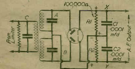
Fig. 5.—Circuit of amplitude discriminator.
