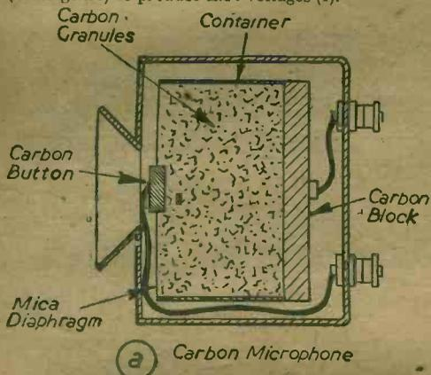
of the carbon button upon the carbon granules, thereby reducing and increasing the contact area of the instrument.
