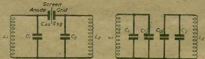
(a) Triode with Screen (b) Triode with 'Earthed' Screen
