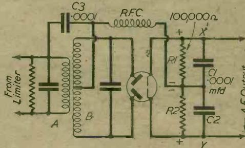
Fig. 6.—The arrangement of a phase discriminator circuit.
