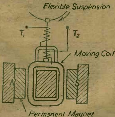
Fig. 6.—The fundamental details of the Grassot fluxmeter.
