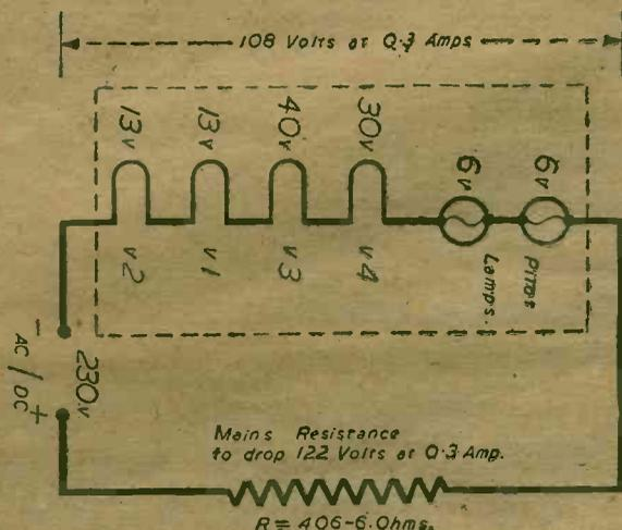
Showing how the heater chain is virtually "across" the mains supply.
