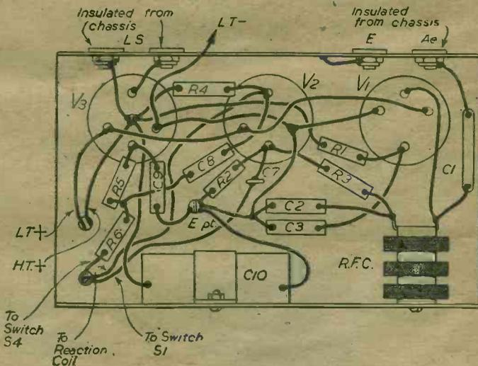
Fig. 2.—Underside of chassis showing wiring, etc.
