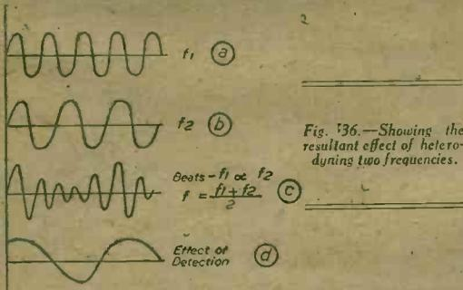
Fig. 36.—Showing the resultant effect of heterodyning two frequencies.
