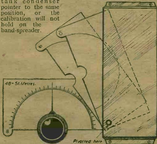
Fig. 2.—The 49 m. card in position ready for calibrating. Remaining card swung back into pocket as shown.
