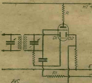
Fig. 3.—Simplified circuit of a second detector providing delayed and amplified A.V.C.
