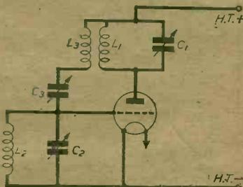
Fig. 27.—A typical neutralising circuit.
