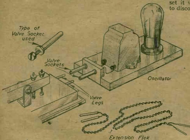
A simple arrangement for a detachable morse key and oscillator.
