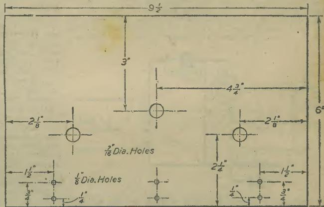
Fig. 2.—Panel and drilling dimensions.
