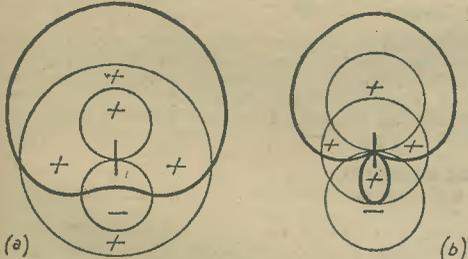
Fig. 104.—Loop voltages smaller (a) and greater (b) than the straight aerial voltages.
