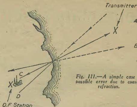
Fig. 111.—A simple case of possible error due to coastal refraction.
