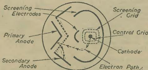
Fig. 1.—The diagram on the left shows the general form of construction for an electron-multiplier. On the right are shown the connections to the valve electrodes.
