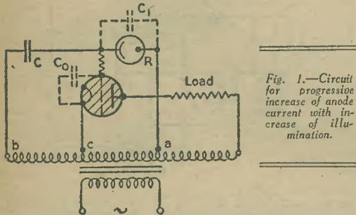
Fig. 1.—Circuit for progressive increase of anode current with increase of illumination.
