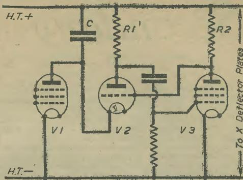
Fig. 30.—A hard valve time base circuit.
