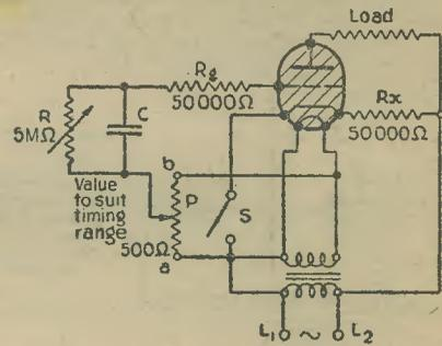
*Fig. 3.—Basic time-delay circuit*
