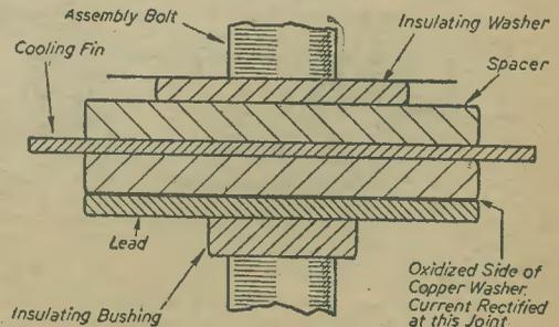
Fig. 2.—A metal rectifier unit assembly.
