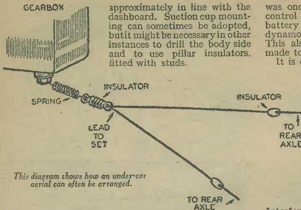
This diagram shows how an under-car aerial can often be arranged.
