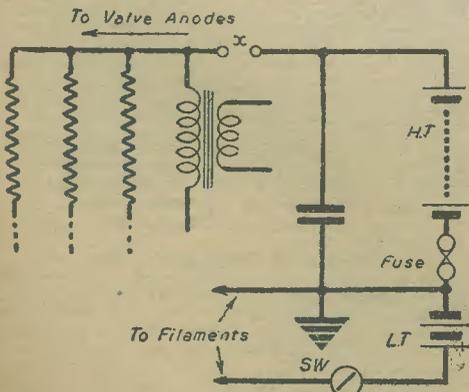
Fig. 1.—In the case of battery-operated receivers, the power supply takes the simplest form as shown here.
