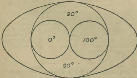
Fig. 106.—Effect of combining loop and straight aerial voltages having a phase difference of 90 deg.
