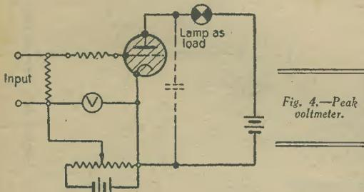
Fig. 4.—Peak voltmeter.
