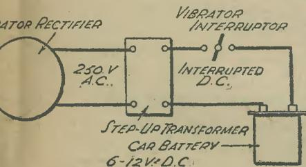
Diagrammatic arrangement for the power supply.
