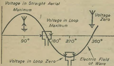
Fig. 105.—Phase difference between loop and straight aerial voltages.
