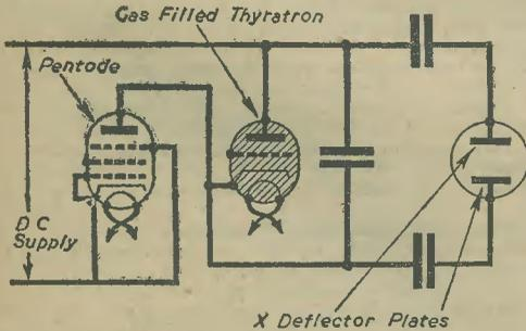
Fig. 29.—The circuit of a thyatron time base.
