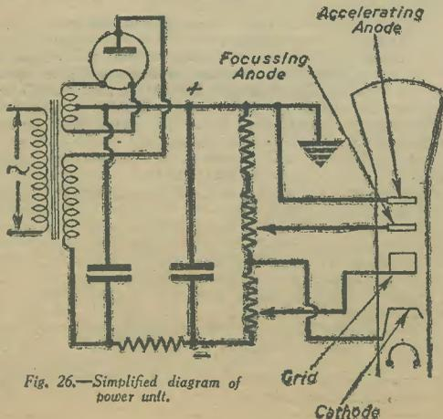
Fig. 26.—Simplified diagram of power unit.
