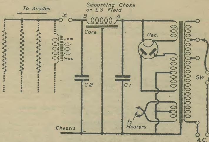
Fig. 2.—A typical arrangement of a power supply for an A.C. operated receiver.
