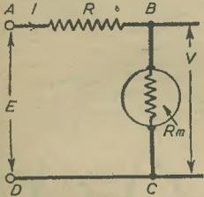
Fig. 1.—In which the voltage across  $B.C.$  is being measured.
