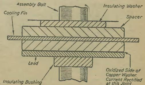
Fig. 2.—A metal rectifier unit assembly.
