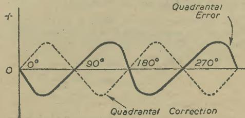
Fig. 109.—Quadrantal error and correction curves.
