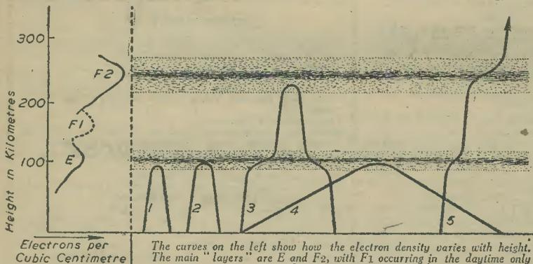
The curves on the left show how the electron density varies with height. The main "layers" are E and F<sub>2</sub>, with F<sub>1</sub> occurring in the daytime only and mainly in summer.
