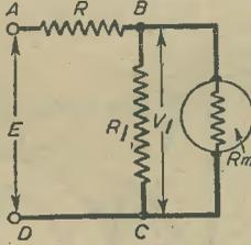
Fig. 2.—In this case we are concerned with the voltage across the load  $R_1$ .
