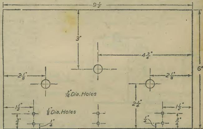
Fig. 2.—Panel and drilling dimensions.
