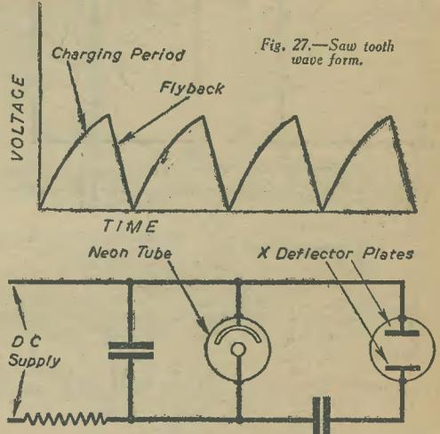
Fig. 28.—Neon tube time base.
