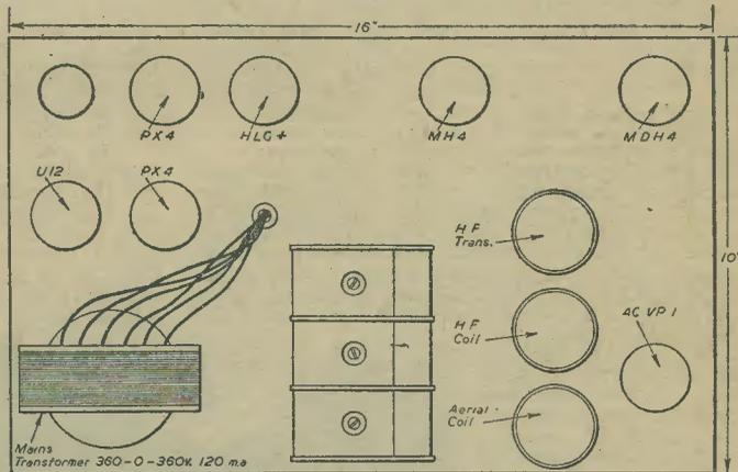
Fig. 4.—Plan view of chassis. A neat and symmetrical layout.
