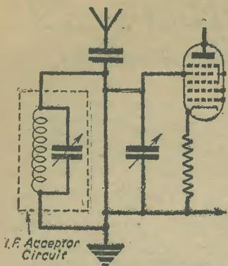
Fig. 2.—An I.F.-tuned acceptor circuit connected between aerial and earth terminals of a "superhet" to prevent "birdies."
