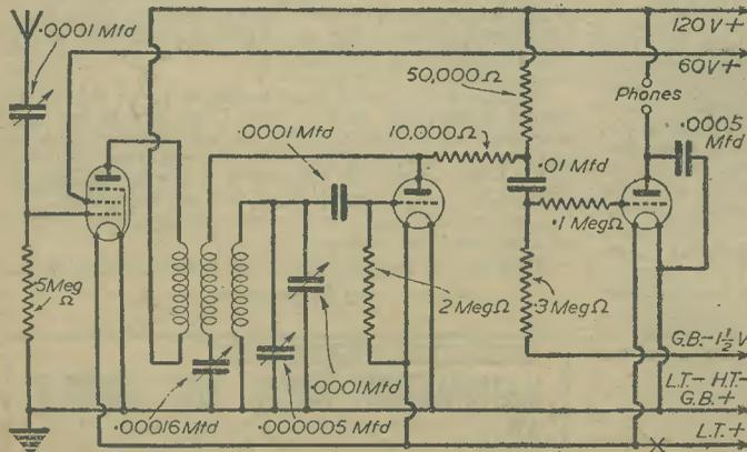
Fig. 1.—The simplicity of the circuit is emphasized by this diagram.
