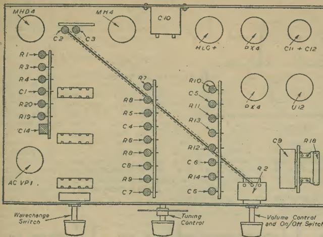
Fig. 2.—Layout of underside of chassis showing use of component panels.
