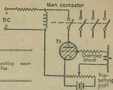
Fig. 5.—Self-resetting overload relay.
