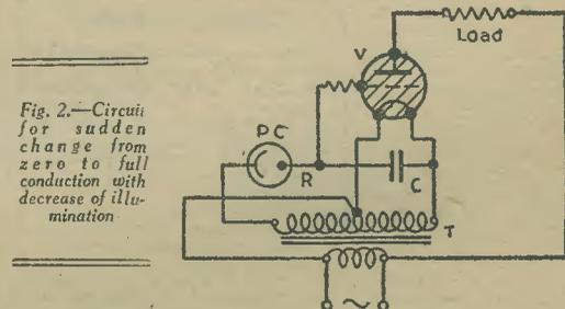
Fig. 2.—Circuit for sudden change from zero to full conduction with decrease of illumination.
