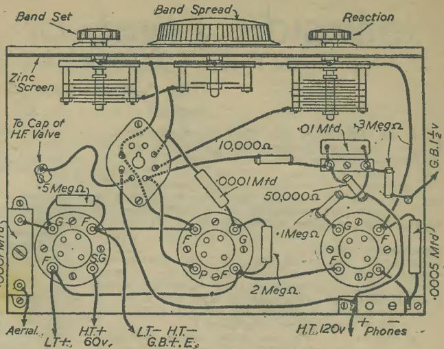
Fig. 3.—Component layout and wiring plan.
