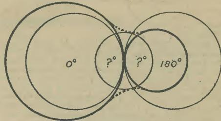
Fig. 107.—Aerial effect produces resultant polar diagram depending on relative phase of loop and aerial voltages.
