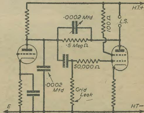
Fig. 3.—Methods of preventing instability with a high-gain output tetrode. They include: the use of a grid stopper; screen decoupler; current feedback, by omission of cathode by-pass condenser; and voltage negative feedback, by connecting a resistor between the anodes of the output and penultimate valves.
