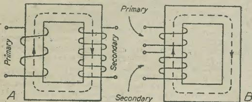
Fig. 1.—Core-type construction.
