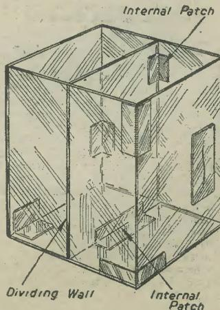
Fig. 2.—Method of repairing leaky containers.
