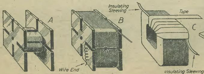
Fig. 6.—Three stages in the winding of coils.
