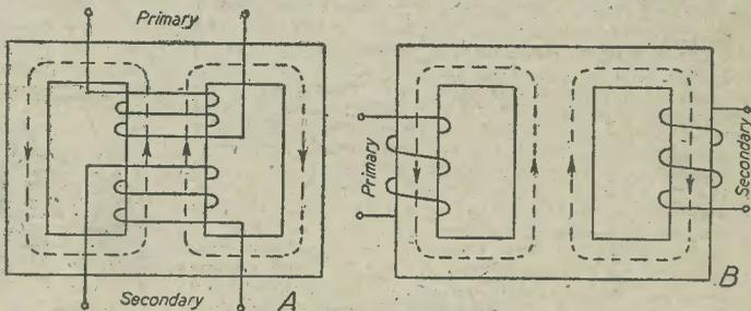
Fig. 2.—Shell-type construction.
