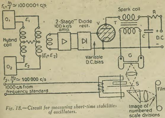
Fig. 18.—Circuit for measuring short-time stabilities of oscillators.
