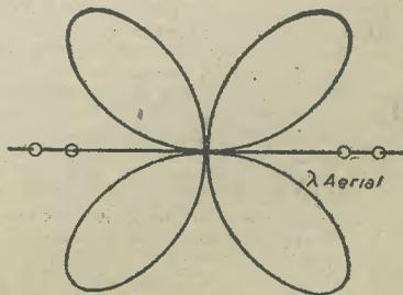
Fig. 3.—Polar diagram of full-wave aerial.
