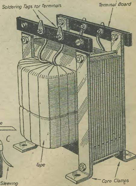
Fig. 7.—Typical shell type transformer.
