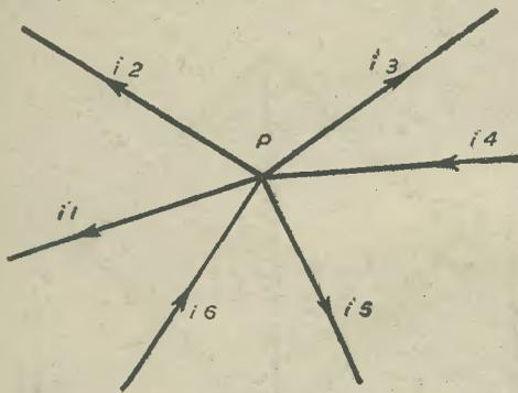
Fig. 3.—Currents flowing to and from a point, demonstrating the first law.
