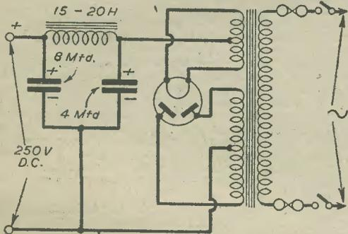
Fig. 1.—A standard full-wave rectifier complete with smoothing arrangements.
