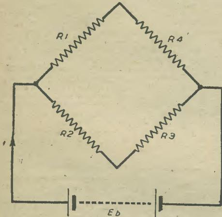
Fig. 1.—A simple series-parallel circuit, involving only an application of Ohm's Law.
