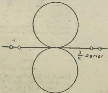
Fig. 2.—Polar diagram of a free-spaced (no earthed) half-wave aerial.
