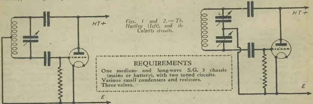
Figs. 1 and 2.—The Hartley (left), and the Colpitts circuits.
