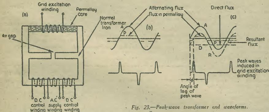
Fig. 23.—Peak-wave transformer and waveforms.
