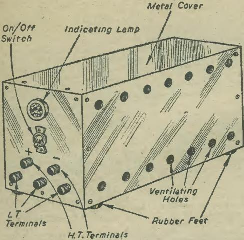
Fig. 3.—The completed mains unit as assembled by the writer. Note the well-ventilated protecting metal cover.
