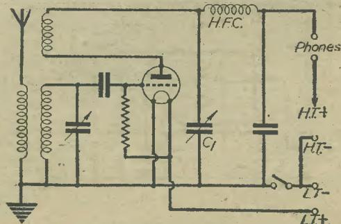
Fig. 2. In this "throttle"-controlled reaction circuit, C<sub>1</sub> varies the degree of feed-back.
