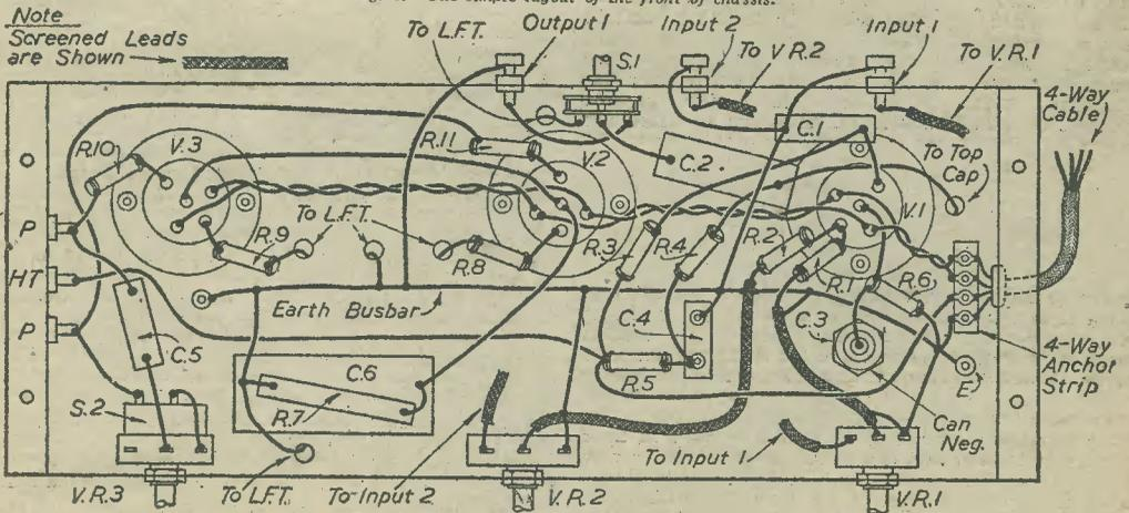
Fig. 5.—Under-chassis wiring diagram and layout.
