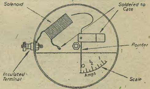
A useful ammeter made from odds and ends.
