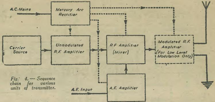
Fig. 4.—Sequence chain for various units of transmitter.
