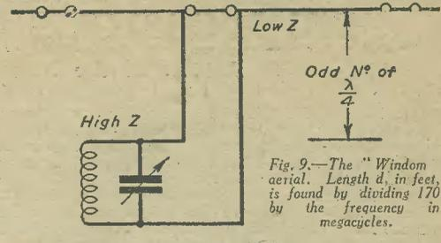
Fig. 9.—The "Windom aerial. Length  $d$ , in feet, is found by dividing 170 by the frequency in megacycles.
