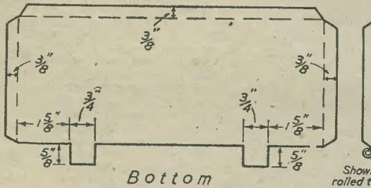
Fig. 6.—Pattern for bottom plate.
