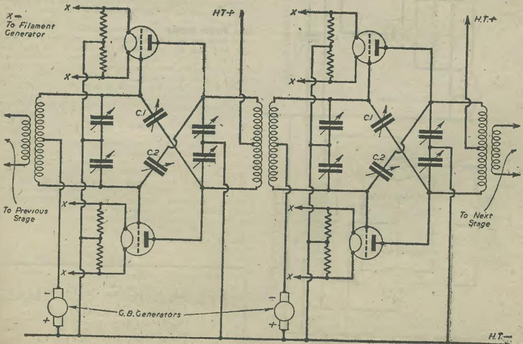
Fig. 2.—Typical circuit for carrier section of transmitter. R.F. valves are used in push-pull.
