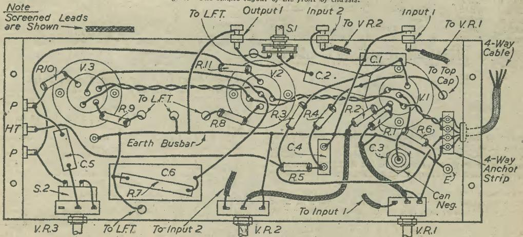
Fig. 5.—Under-chassis wiring diagram and layout.
