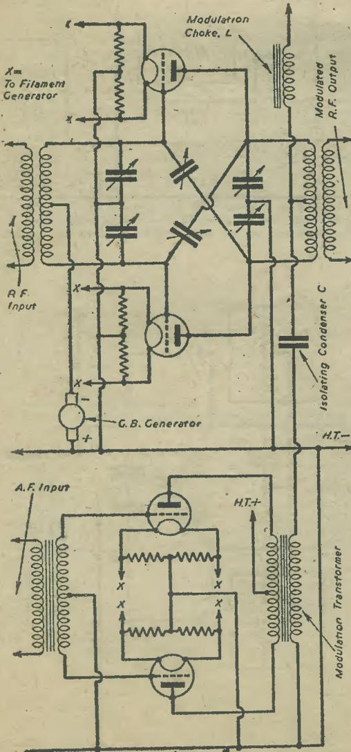
Fig. 3.—The Heising modulation circuit, employing R.F. amplifiers following the modulation.
