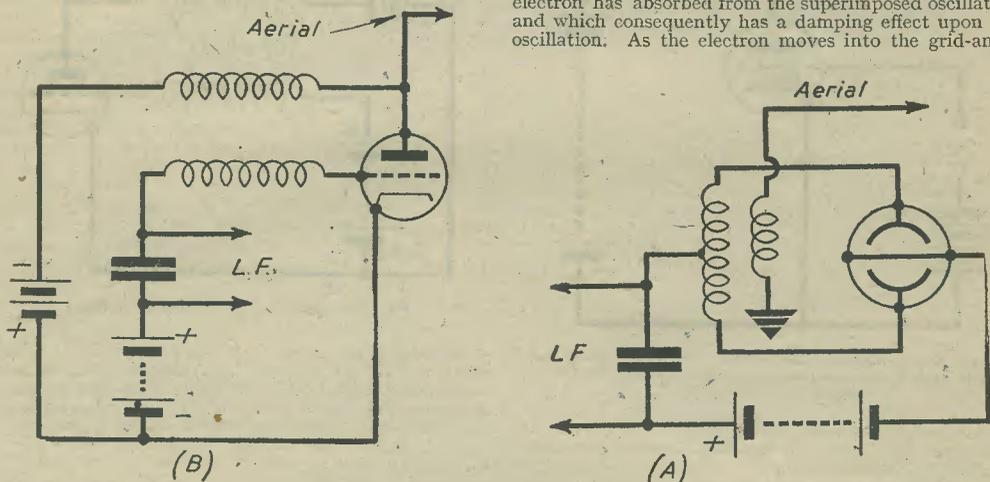
Fig. 4.—Magnetron and Backhausen detectors respectively.
