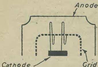
Fig. 3.—How electrons oscillate about the grid in a Backhausen oscillator before being trapped by it.
