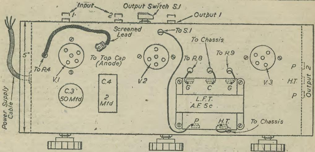
Fig. 3.—Top of chassis layout.
