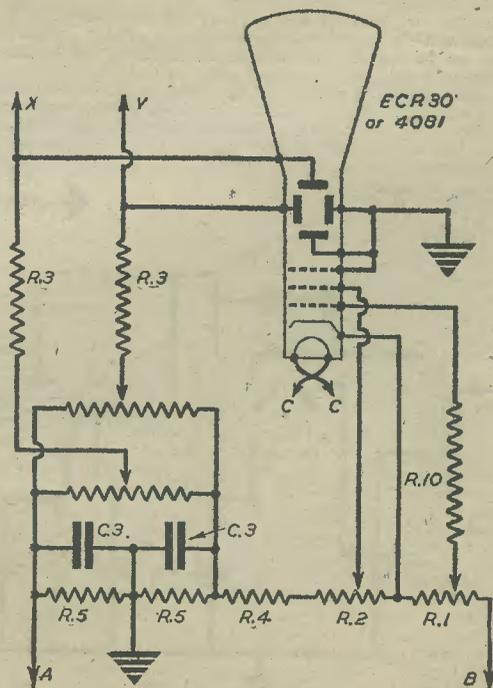
Fig. 2.—Connections to the tube, and resistance network.
