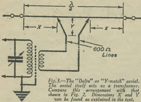
Fig. 3.—The "Delta" or "Y-match" aerial. The aerial itself acts as a transformer. Compare this arrangement with that shown in Fig. 2. Dimensions X and Y can be found as explained in the text.
