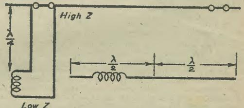
Fig. 5.—The "Zep" aerial with a quarter-wave feeder. The inset diagram explains how a low impedance source is matched into the (high impedance) end of a half-wave aerial.
