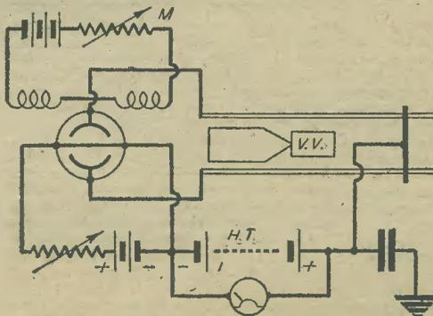
Fig. 6.—A magnetron set up in the electronic mode for experiment to be carried out on oscillating conditions.
