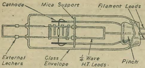
Fig. 5.—Sectional view of typical magnetron.
