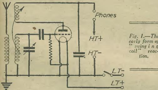
Fig. 1.—The early form of "swing in Q coil" reaction.
