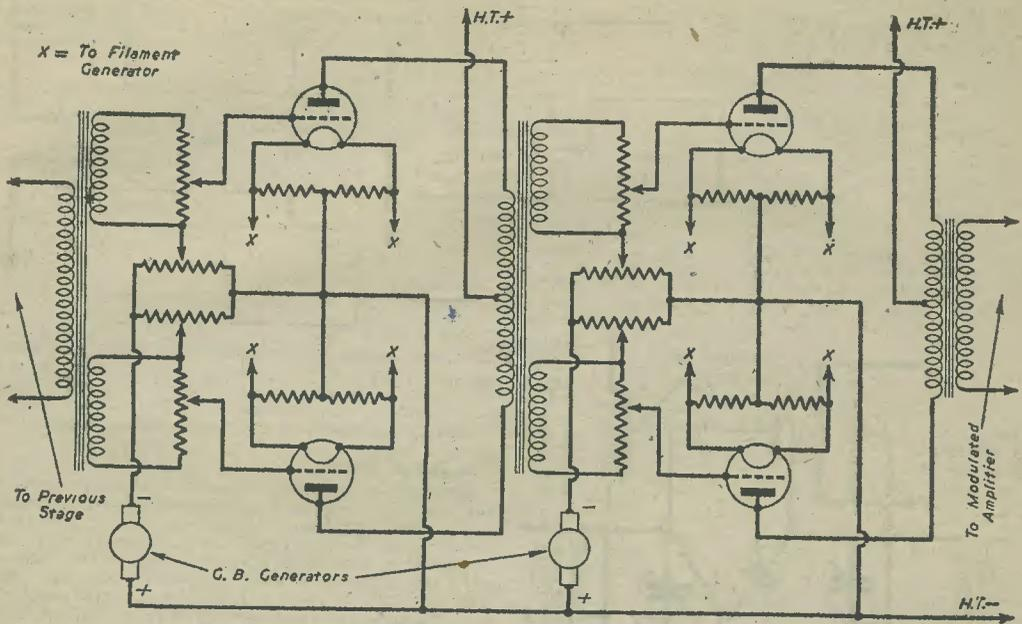
Fig. 1.—Circuit for control of magnitude of audio-frequency input to each valve by means of potential dividers, permitting differences of amplification factors. The two halves of the class B output stage are given independent grid bias supplies.
