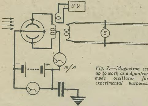
Fig. 7.—Magnetron set up to work as a dynatron mode oscillator for experimental purposes.
