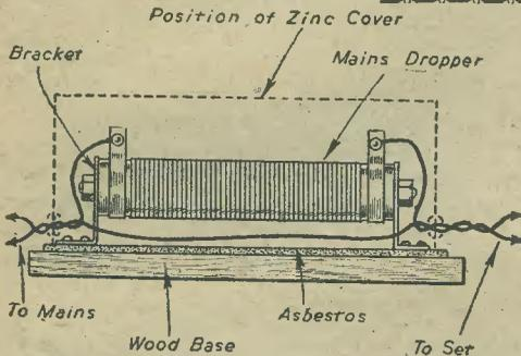
Method of using a mains dropper as a line-cord resistance.
