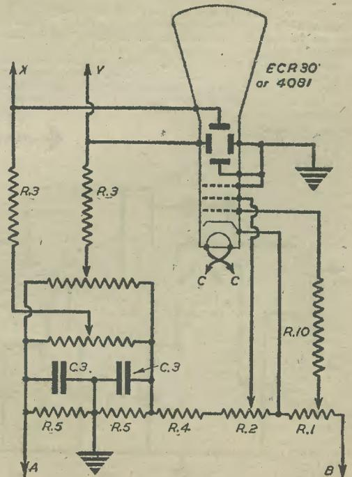
Fig. 2.—Connections to the tube, and resistance network.
