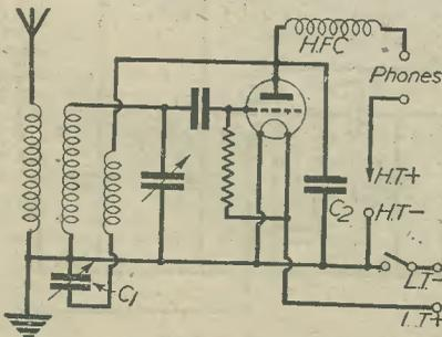
Fig. 3.—The "Reinartz" circuit also has a fixed reaction coil and capacity control.
