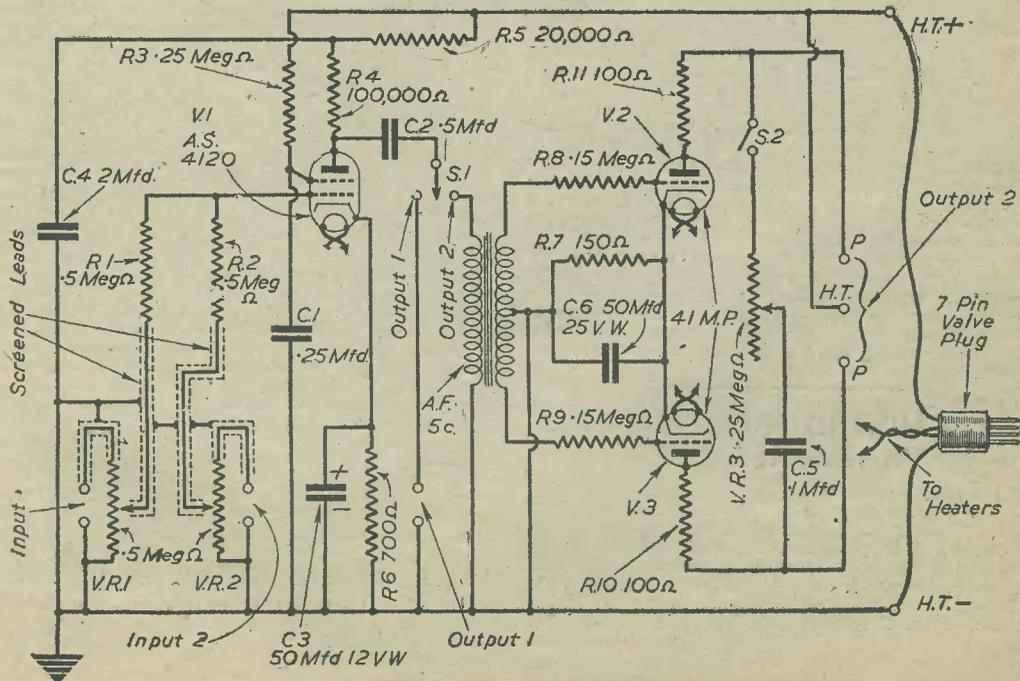
Fig. 1.—The circuit diagram of the push-pull amplifier.
