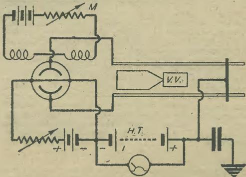
Fig. 6.—A magnetron set up in the electronic mode for experiment to be carried out on oscillating conditions.
