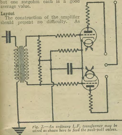
Fig. 2.—An ordinary L.F. transformer may be wired as shown here to feed the push-pull valves.
