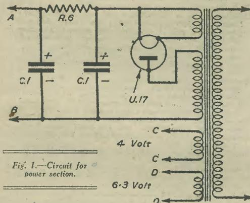
Fig. 1.—Circuit for power section.
