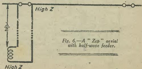
Fig. 6.—A "Zep" aerial with half-wave feeder.
