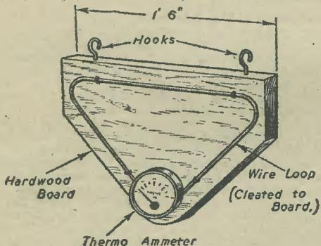
Fig. 4.—A simple device for checking aerial matching and for detecting standing waves and feeders.
