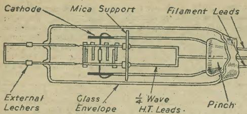
Fig. 5.—Sectional view of typical magnetron.
