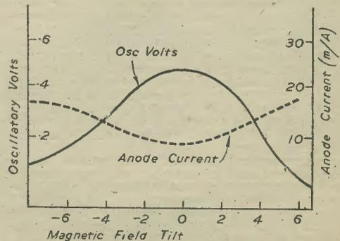
Fig. 8.—A graph depicting the change in oscillator voltage (and d.c. anode current) for variation of the magnetic field.
