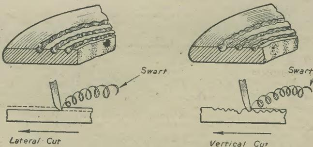
Fig. 4 (Left)—Lateral cut, constant movement; and (Right) Vertical cut constant pitch lateral contour, but cut up and down, giving variable depth.
