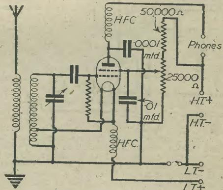
Fig. 4.—A battery version of the "electron-coupled" system of regeneration.
