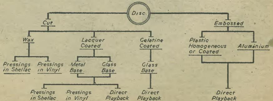
Fig. 2.—Types of disc recording and relationship between cut and embossed records.
