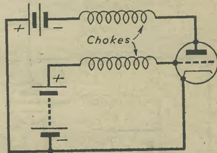
Fig. 2.—Simple form of Backhausen oscillator.
