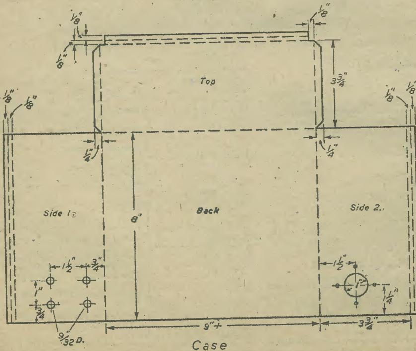
Fig. 4.—Developed plan of the metal box.
