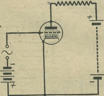
Fig. 1.—Transit-time causes the electrons to be unequally distributed on either side of the grid; hence, a current flows into the grid in spite of its negative bias.
