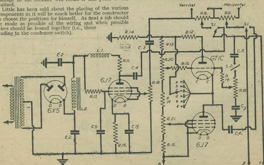
Fig. 3.—A satisfactory oscilloscope circuit: a=c5, b=c4, c=c3, d=c8, e=c7, f=c6.
