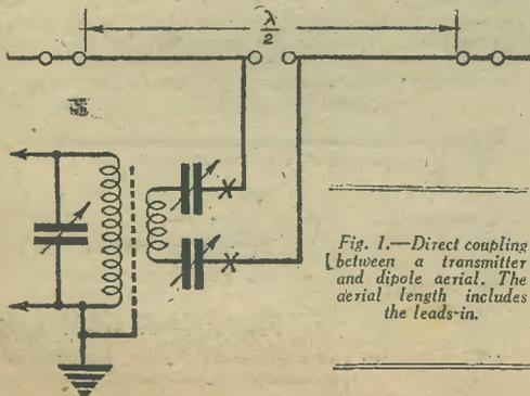
Fig. 1.—Direct coupling between a transmitter and dipole aerial. The aerial length includes the leads-in.
