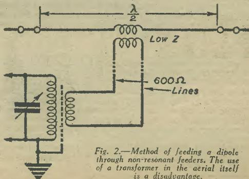
Fig. 2.—Method of feeding a dipole through non-resonant feeders. The use of a transformer in the aerial itself is a disadvantage.
