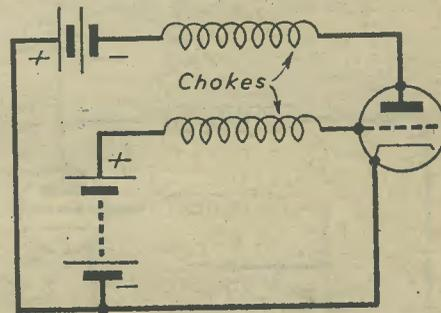
Fig. 2.—Simple form of Backhausen oscillator.
