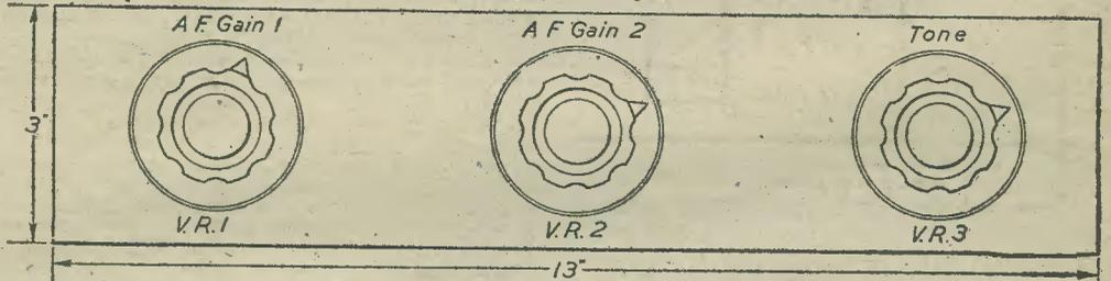
Fig. 4.—The simple layout of the front of chassis.
