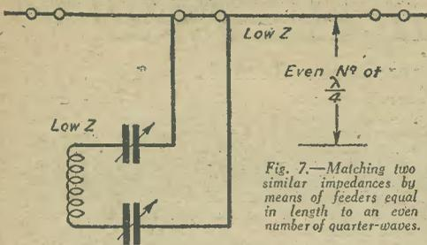
Fig. 7.—Matching two similar impedances by means of feeders equal in length to an even number of quarter-waves.
