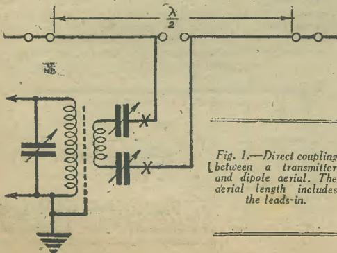
The number of turns required on the secondary can be found by calculating the necessary step-down ratio, having a knowledge of optimum load of the valve which feeds the tuned tank circuit, from the formula:
