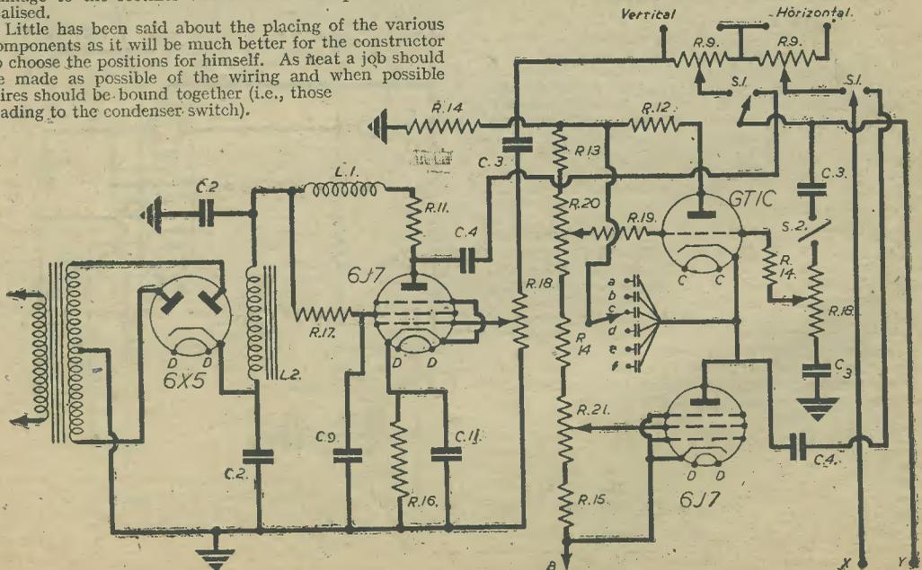
Fig. 3.—A satisfactory oscilloscope circuit: a=c5, b=c4, c=c3, d=c8, e=c7, f=c6.
