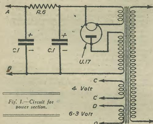
Fig. 1.—Circuit for power section.
