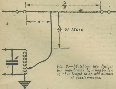
Fig. 8.—Matching two dissimilar impedances by using feeders equal in length to an odd number of quarter-waves.
