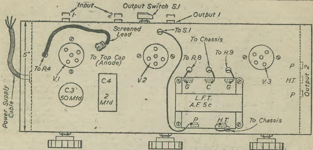
Fig. 3.—Top of chassis layout.
