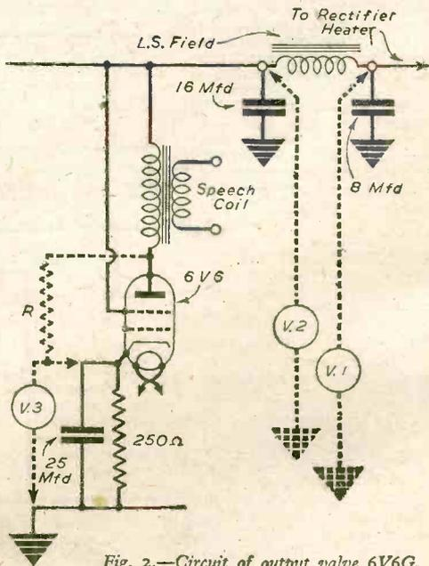
Fig. 2.—Circuit of output valve 6V6G.
