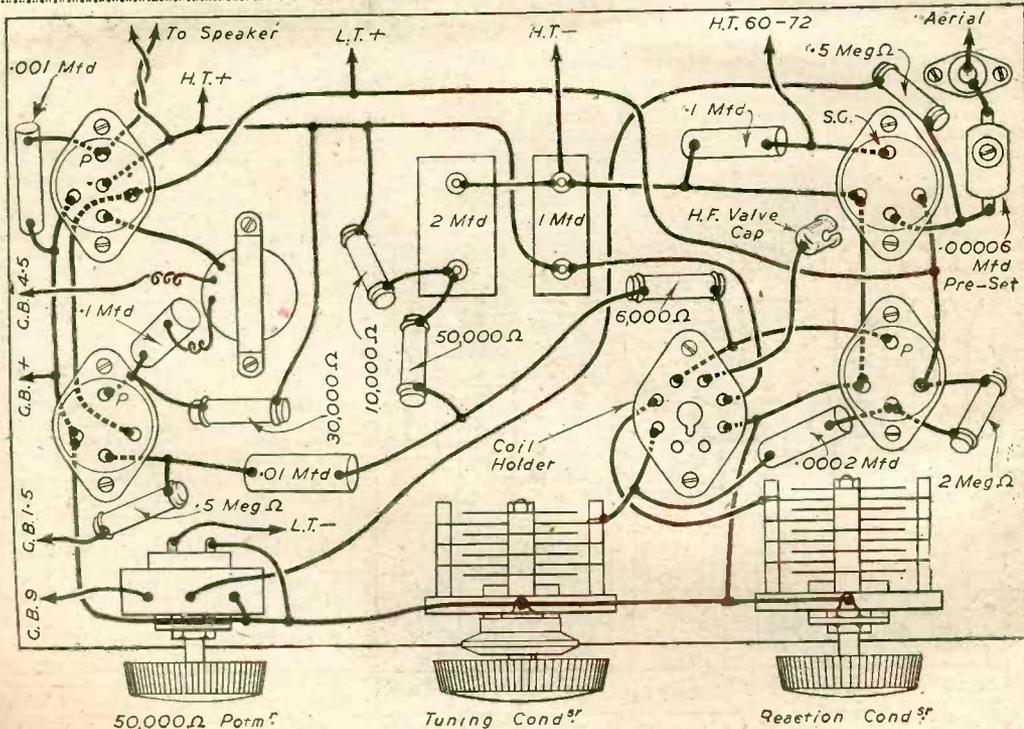
Fig. 2.—Layout of components and wiring diagram.
