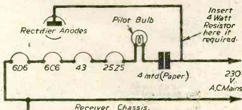
Using a voltage-dropping condenser in a heater circuit.
