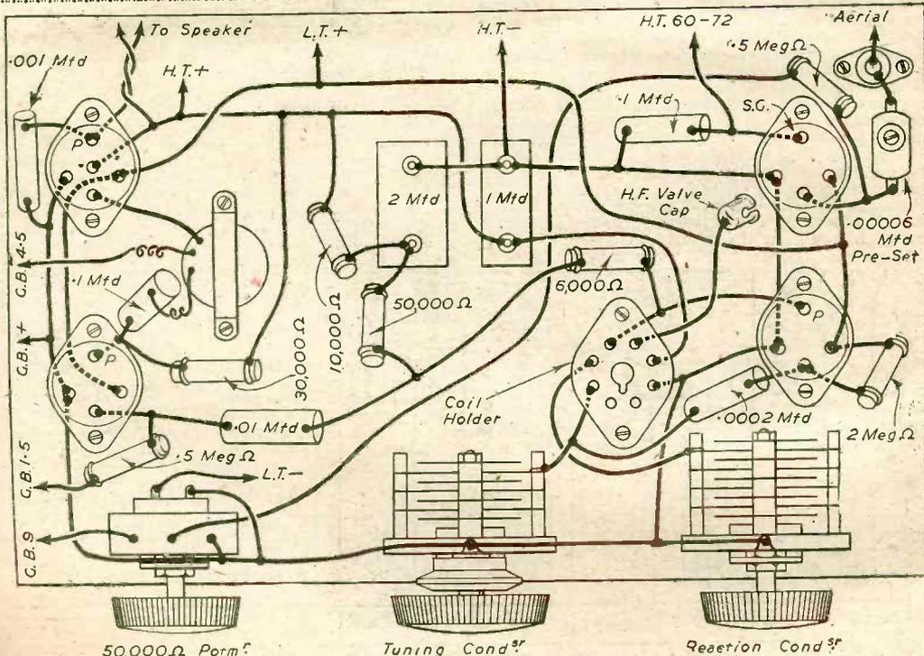
Fig. 2.—Layout of components and wiring diagram.
