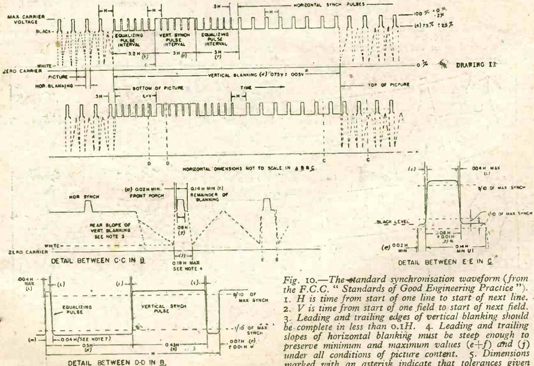
Fig. 10.—The standard synchronisation waveform (from the F.C.C. "Standards of Good Engineering Practice").
