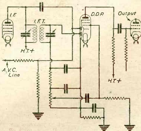
Fig. 9.—Delayed A.V.C. circuit.
