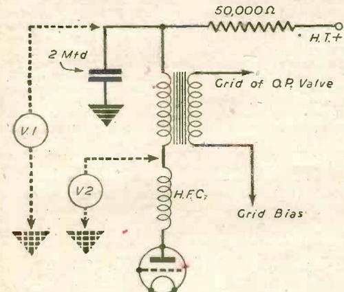
Fig. 1.—Detector anode and grid circuit.
