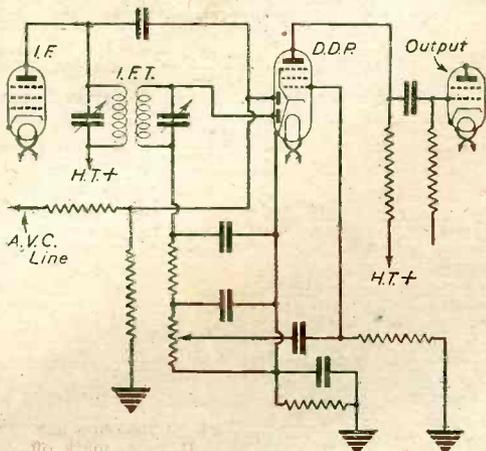
Fig. 9.—Delayed A.V.C. circuit.
