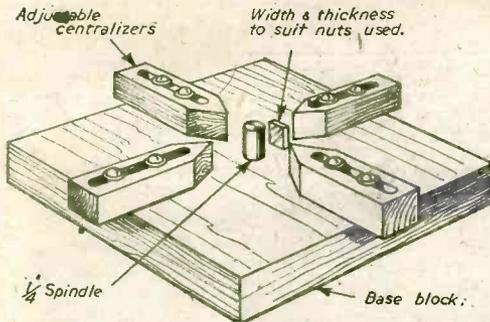
Jig for filling screw-caps with plastic material for making small knobs.
