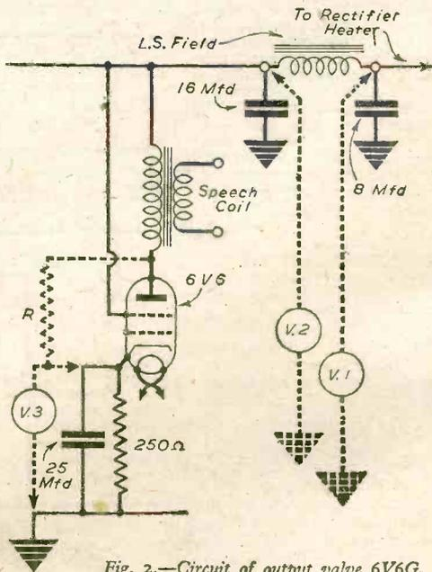
Fig. 2.—Circuit of output valve 6V6G.
