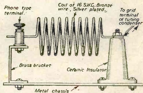
A simple method of varying the inductance of an H.F. coil.
