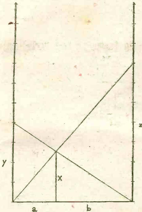
Fig. 1.—Abac for calculating total value of total resistances.
