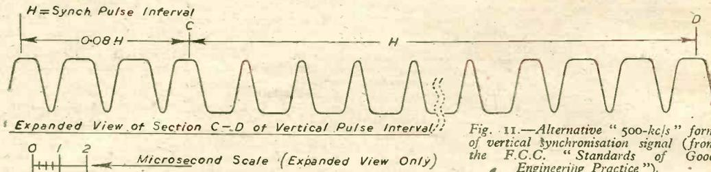
Fig. 11.—Alternative "500-kc/s" form of vertical synchronisation signal (from the F.C.C. "Standards of Good Engineering Practice").
