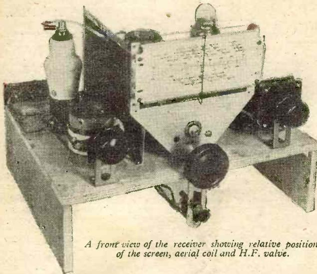
*A front view of the receiver showing relative positions of the screen, aerial coil and H.F. valve.*
