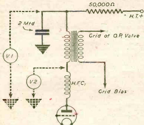
Fig. 1.—Detector anode and grid circuit.
