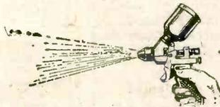
No one can dispute that for speed the spray gun will beat the paint brush every time. But when spraying small objects a lot of paint is inevitably wasted. Further, unless the gun is skilfully used, 'runs' and 'tears' will form, necessitating rubbing down and a re-spray.
