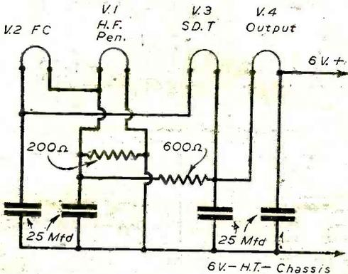
Fig. 1.—Circuit diagram showing filament resistance.
