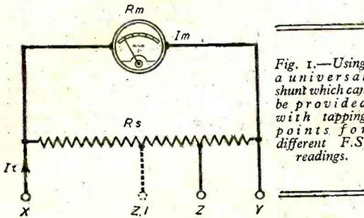
Fig. 1.—Using a universal shunt which can be provided with tapping points for different F.S. readings.
