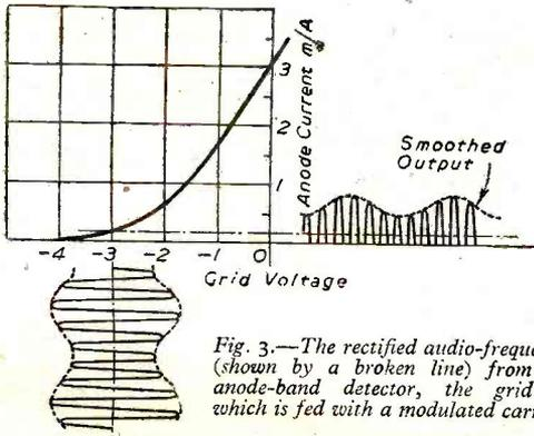
Fig. 3.—The rectified audio-frequency (shown by a broken line) from an anode-band detector, the grid of which is fed with a modulated carrier.
