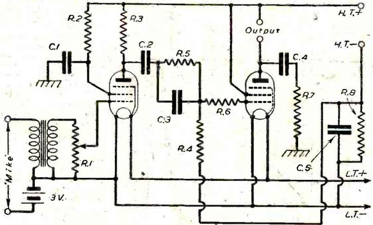
Fig. 1.—Theoretical circuit showing high- and low-note boosters.
