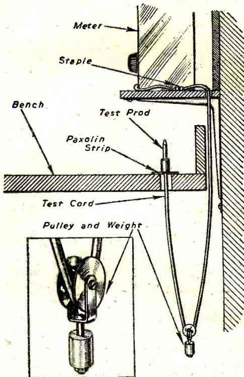
*A good method of arranging the test cords.*
