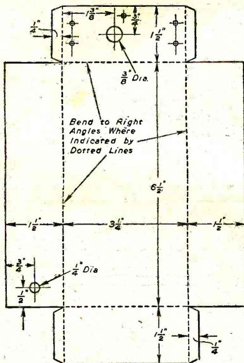
Fig. 3.—Plan and dimensions of case. Fold on dotted lines.
