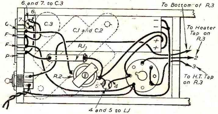
Fig. 9.—Under-chassis wiring.
