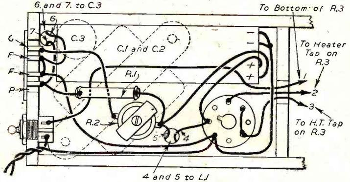
Fig. 9.—Under-chassis wiring.
