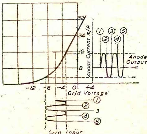
Fig. 2.—This diagram shows how the anode waveform can be projected geometrically from the grid input waveform on an anode current-grid voltage curve.
