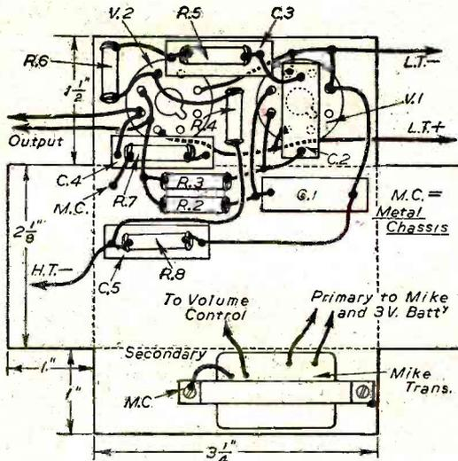
Fig. 4.—Wiring plan and flat shape of valveholder platform.
