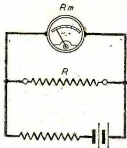
Fig. 3.—This method can be used for measuring resistances of low value, the resistance circuit under test being represented by R.
