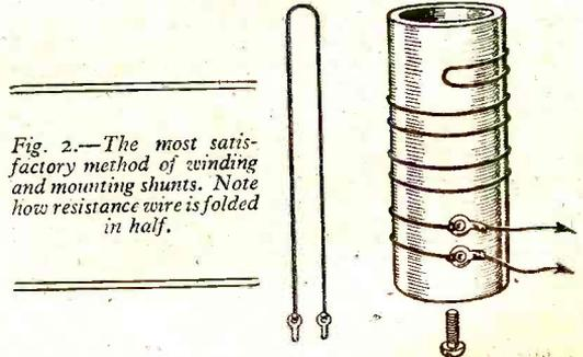
Fig. 2.—The most satisfactory method of winding and mounting shunts. Note how resistance wire is folded in half.
