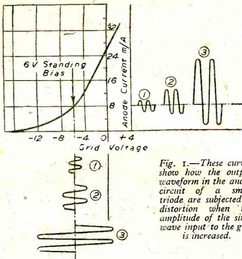
Fig. 1.—These curves show how the output waveform in the anode circuit of a small triode are subjected to distortion when the amplitude of the sine-wave input to the grid is increased.
