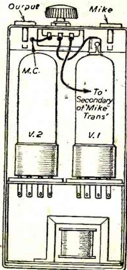
Fig. 2.—General assembly of the amplifier in case.
