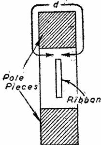
Fig. 2.—The frequency range of a ribbon microphone depends on the distance "d"
