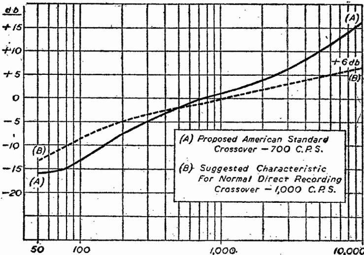
Fig. 1.—Characteristic curves for recording crossovers.
