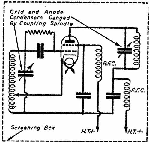
Fig. 4.—Heterodyne frequency meter.
