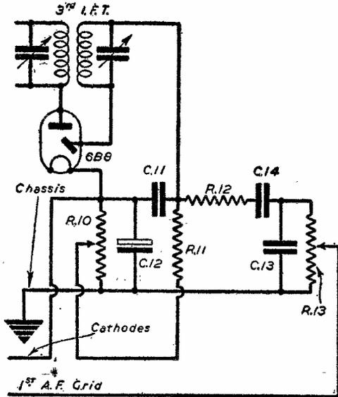
Fig. 1.—Modified circuit for the noise limiter.
