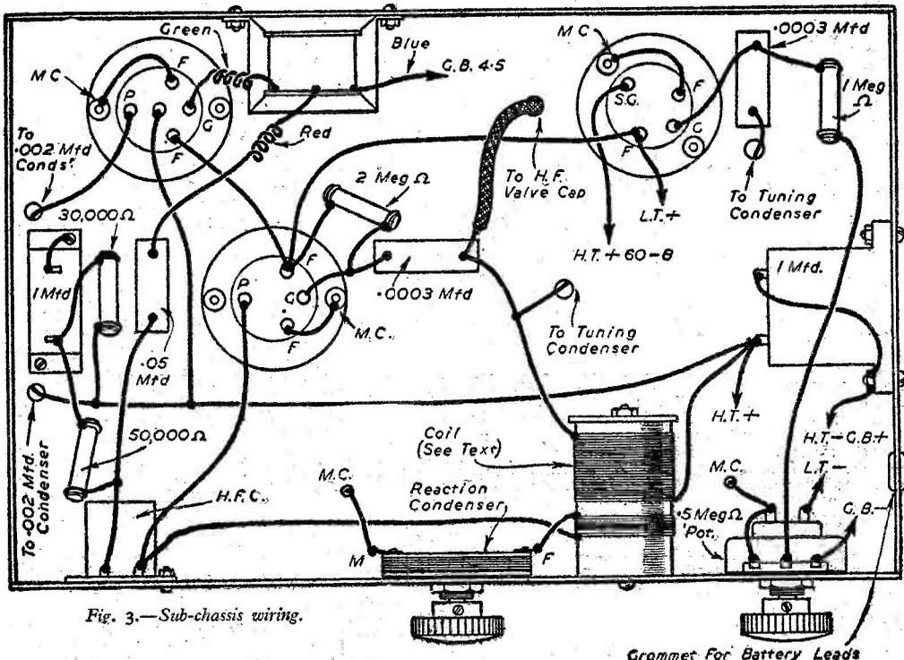
Fig. 3.—Sub-chassis wiring.
