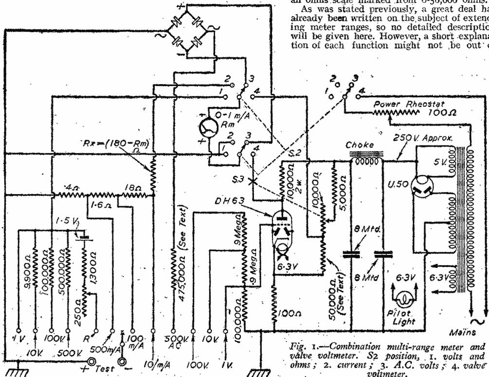
Fig. 1.—Combination multi-range meter and valve voltmeter. S<sub>2</sub> position, 1. volts and ohms; 2. current; 3. A.C. volts; 4. valve voltmeter.
