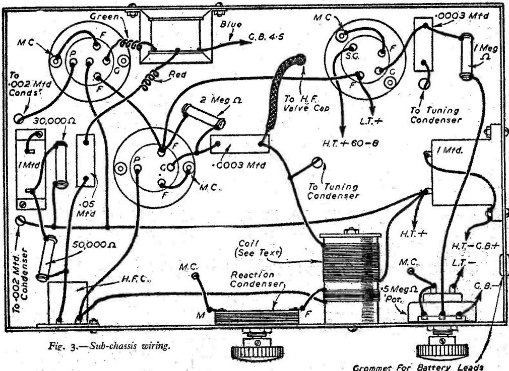
Fig. 3.—Sub-chassis wiring.
