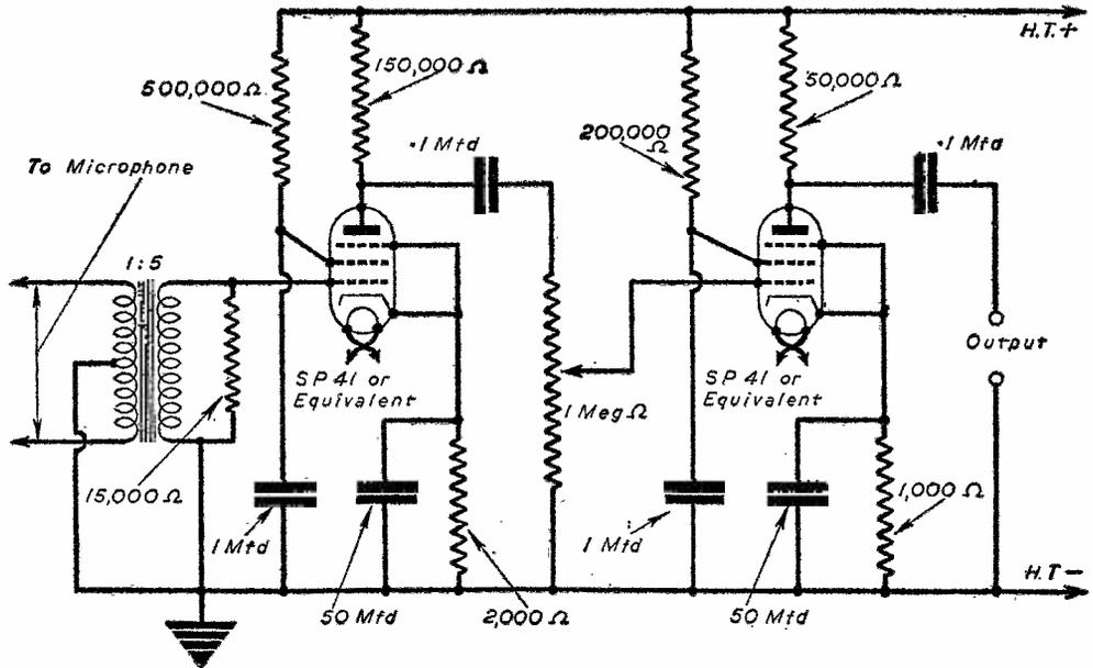
Fig. 7.—Suggested circuit diagram for microphone amplifier.
