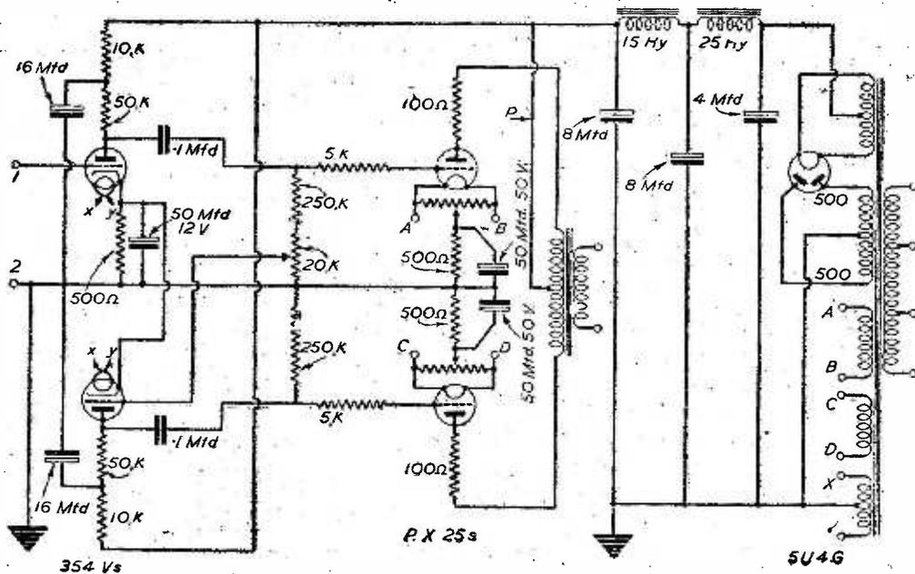
Fig. 3.—Circuit of well-known conventional type amplifier.
