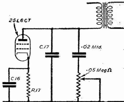
Fig. 2a.—Circuit for "top cut."
