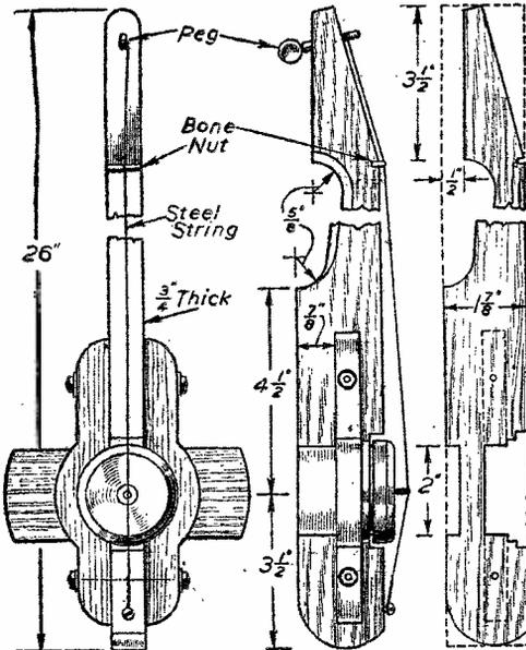
Fig. 1.—Shortened top and side view of instrument and handle.
