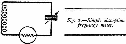
Fig. 1.—Simple absorption frequency meter.
