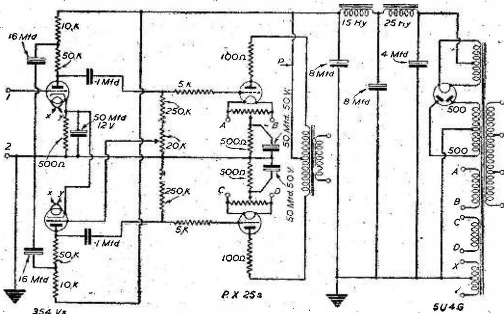
Fig. 3.—Circuit of well-known conventional type amplifier.
