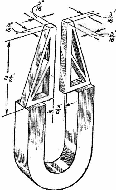
Fig. 4.—Suggested construction of microphone. Essential dimensions are given.
