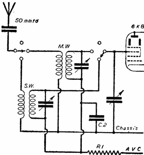
Fig. 4.—Modified R.F. circuit.
