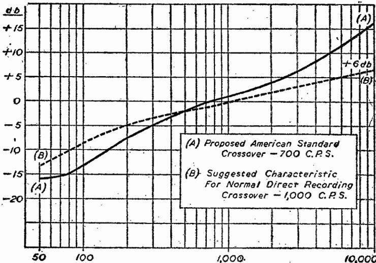
Fig. 1.—Characteristic curves for recording crossovers.
