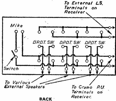
The board is shown wired for three external speakers, but any number can be fitted, an extra D.P.D.T. switch, in parallel with the rest, having to be added for each L.S. A sensitive headphone may be used in place of the microphone, if desired.
