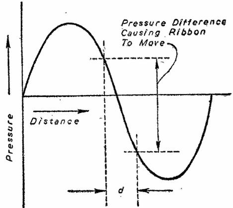
Fig. 3.—Illustrating principle of "Velocity" operation.
