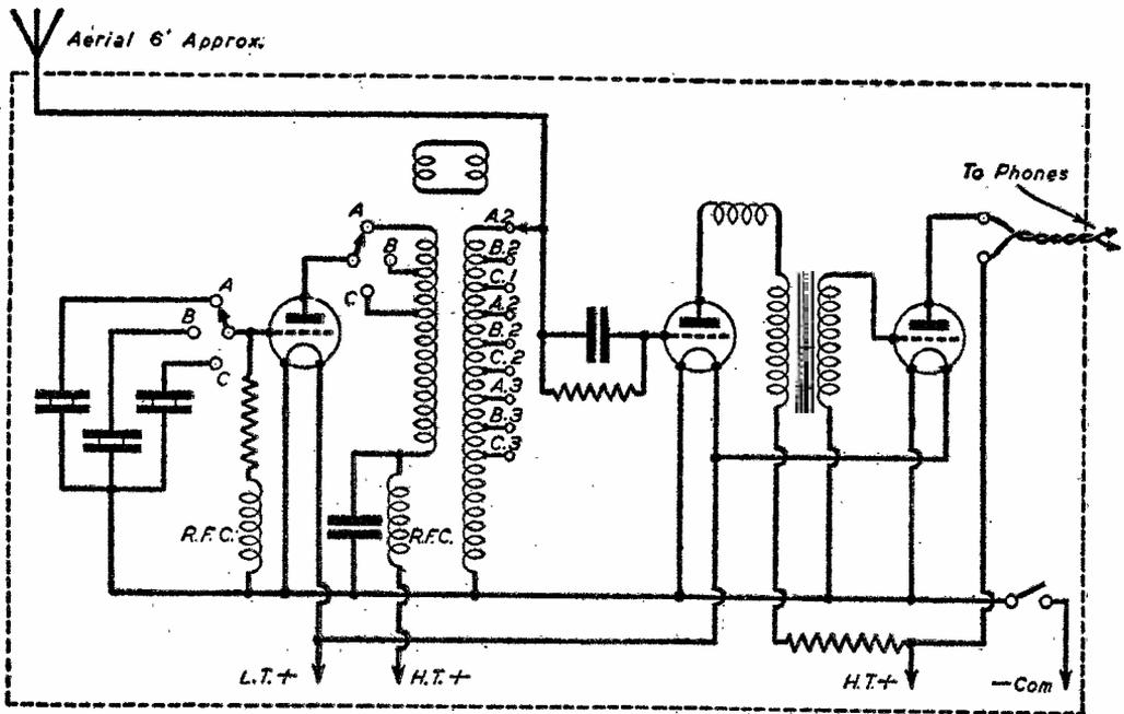
Fig. 5.—Crystal frequency monitor.
