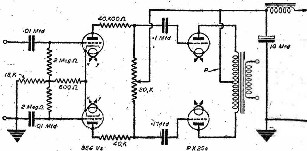
Fig. 4.—Alternative input (Schmitt circuit). To balance, in each case, insert 50 resistor at P. With 1,000 c.p.s. input balance 20 k. potentiometer to minimum signal—with 'phones across P.
