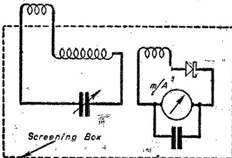
Fig. 2.—Modern absorption wavemeter.
