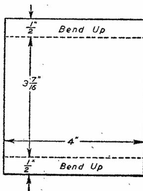
Fig. 5.—The two supporting brackets for the H.F. shelf, and the coil stowage partition.
