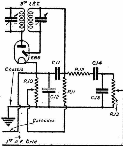
Fig. 1.—Modified circuit for the noise limiter.
