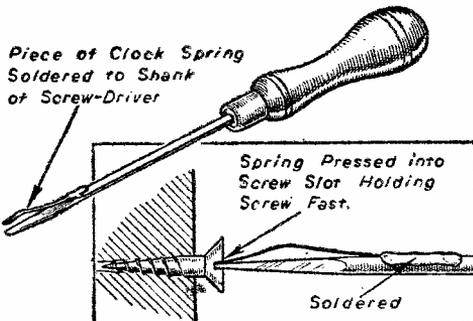
Adapting a screwdriver for holding screws in awkward places.
