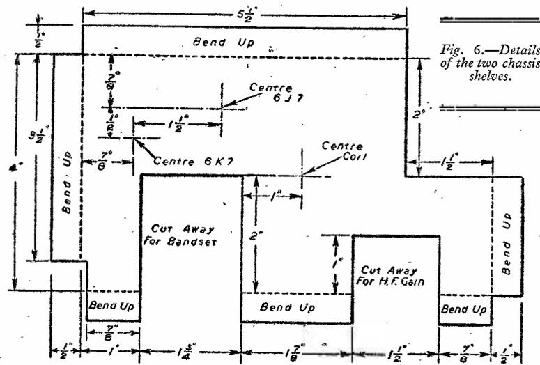
Fig. 6.—Details of the two chassis shelves.
