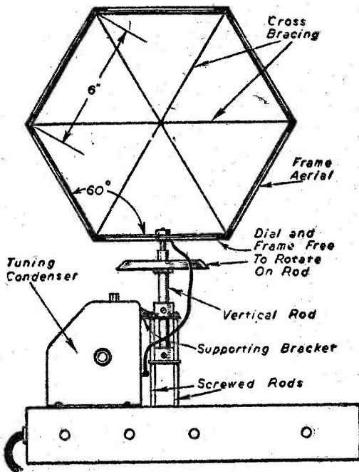
Fig. 4.—Front view, showing location of frame aerial.
