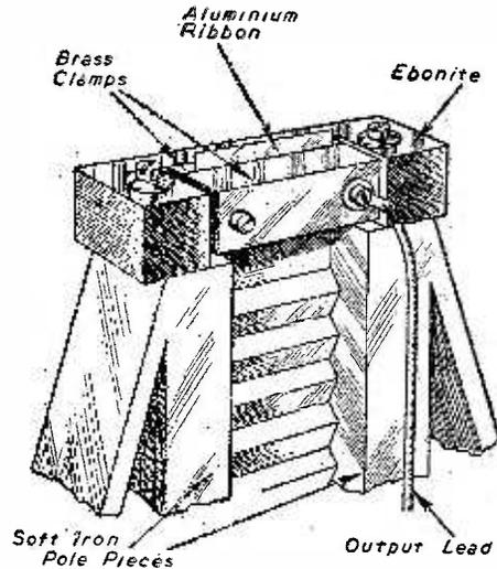
Fig. 5.—Suggested construction of end clamps.
