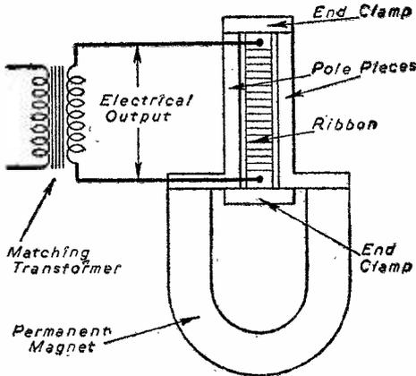
Fig. 1.—General view of the essential working parts of a ribbon microphone.
