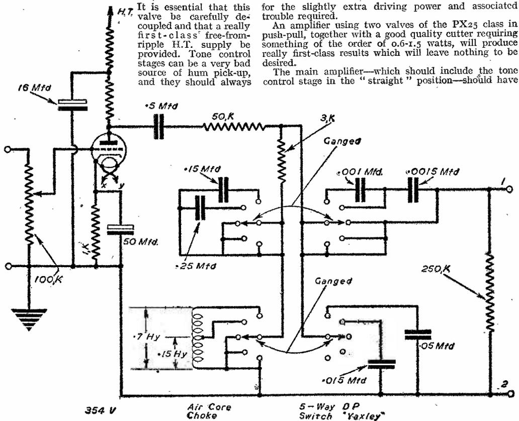
Fig. 2.—Tone control circuit.
