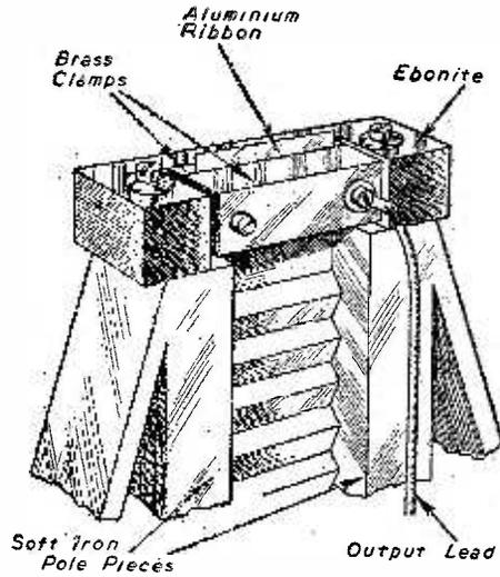
Fig. 5.—Suggested construction of end clamps.
