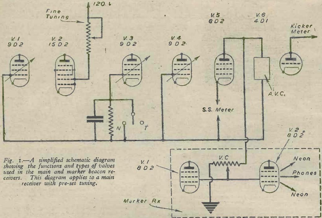
Fig. 1.—A simplified schematic diagram showing the functions and types of valves used in the main and marker beacon receivers. This diagram applies to a main receiver with pre-set tuning.
