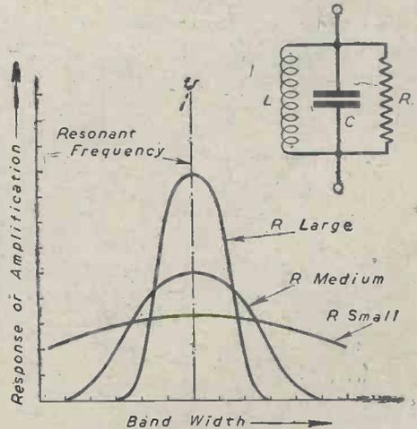
Fig. 5.—Response curves for a loaded tuned circuit.
