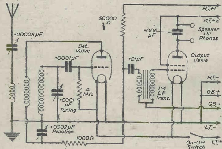
Fig. 1.—Theoretical circuit.
