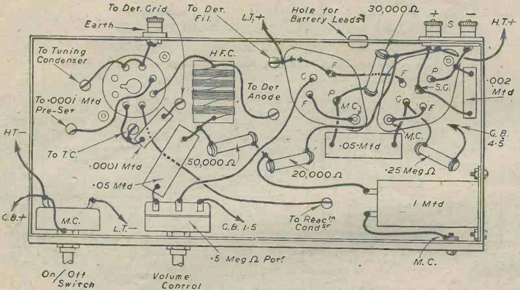
Fig. 3.—Sub-chassis wiring diagrams.
