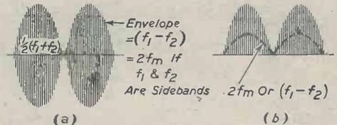
Fig. 2.—Beat resultant of two frequencies  $f_1$  and  $f_2$ , which may be the sidebands ( $f_c + f_m$ ) and ( $f_c - f_m$ ) in Fig. 1. Frequency doubling of the modulation envelope would then occur, i.e.,  $2f_m$
