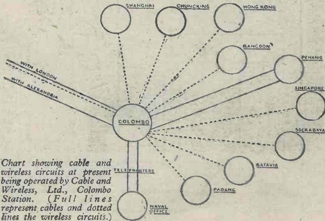
Chart showing cable and wireless circuits at present being operated by Cable and Wireless, Ltd., Colombo Station. (Full lines represent cables and dotted lines the wireless circuits.)
