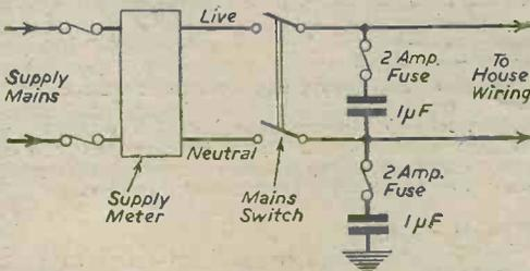
Fig. 2.—Condenser filter to isolate house wiring systems in the case of mains-borne interference.
