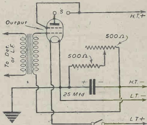
Fig. 6.—Addition to auto-bias circuit.
