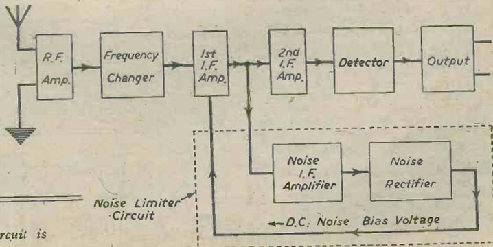
Fig. 8.—How the noise limiter circuit is introduced.
