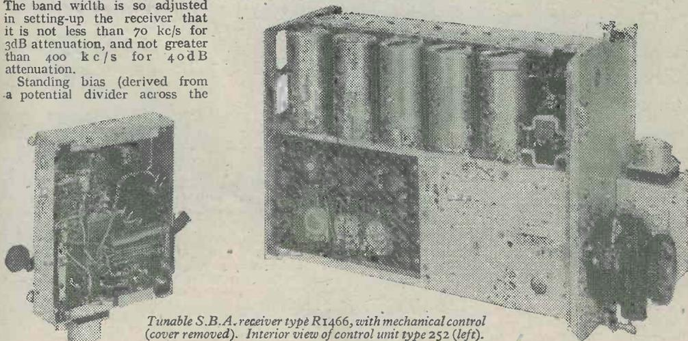
Tunable S.B.A. receiver type R1466, with mechanical control (cover removed). Interior view of control unit type 252 (left).
