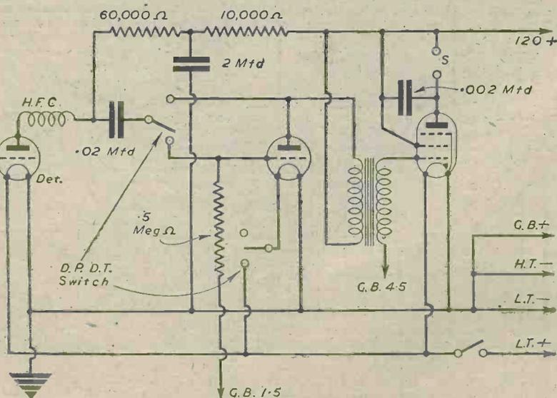
Fig. 5.—Circuit with optional L.F. stage.
