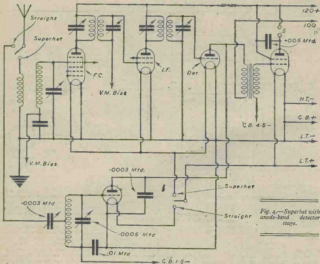
Fig. 4.—Superhet with anode-bend detector stage.
