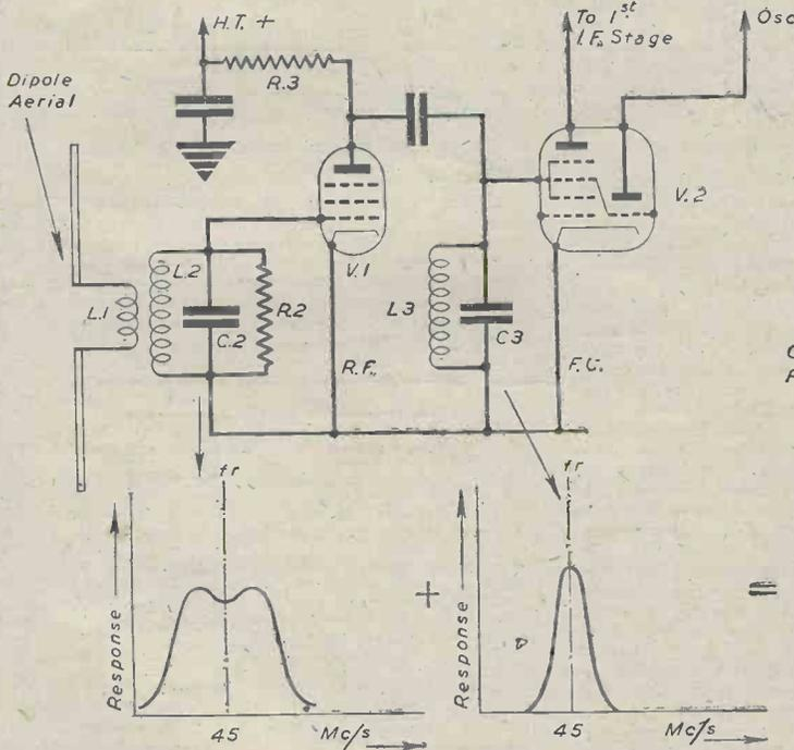
Fig. 1.—R.F. wide-band coupling circuits with response curves.
