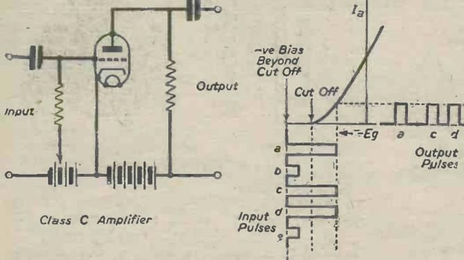
Fig. 8.—If this type of circuit is employed, then only pulses exceeding a certain amplitude will be passed.
