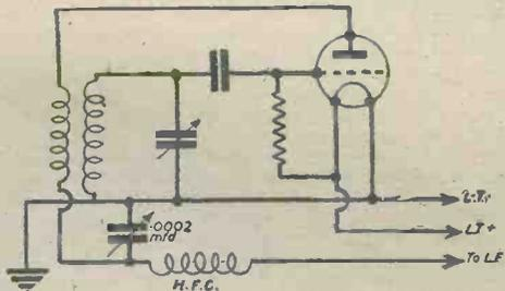
Fig. 4.—This arrangement is known as "throttle-controlled reaction."
