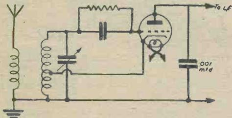
Fig. 6.—With mains valves, this cathode-tap arrangement will be found very effective.
