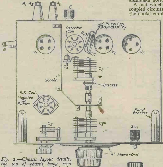
Fig. 2.—Chassis layout details, the top of chassis being seen above, and the underside in the diagram on the right.
