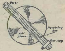
because the ordinary "toggle" switch has a nasty habit of getting turned on when in a confined space. This is impossible with the push-pull switch as it is off in the "in" position.
