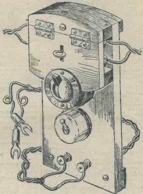
Fig. 6.—The completed charging board.
