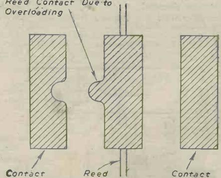
Fig. 4.—A common vibrator fault shown in section.
