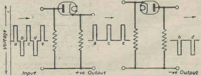
Fig. 7.—A diode separator circuit showing how it may be made to pass either positive or negative pulses.
