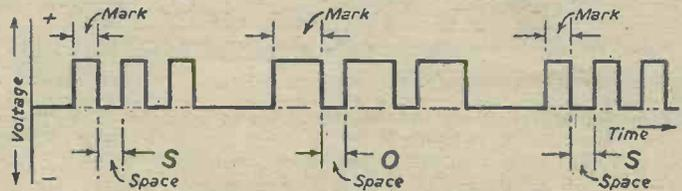
Fig. 2.—The morse letters S O S showing how the mark/space ratio varies with different letters.
