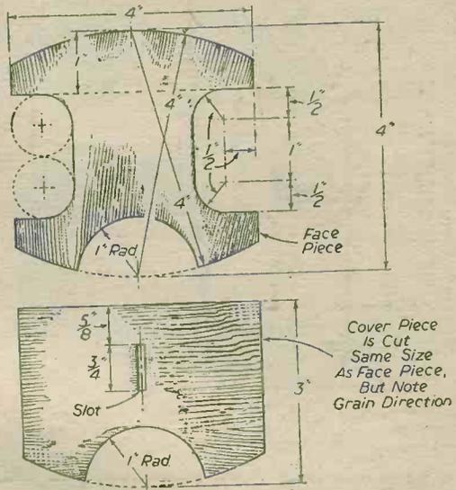
Fig. 2.—Terminal housing piece and part cover piece.
