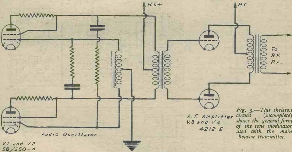
Fig. 3.—This skeleton circuit (incomplete) shows the general form of the tone modulator used with the main beacon transmitter.
