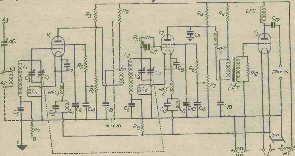
Fig. 1.—Theoretical circuit of the 3-valve short-wave receiver.
