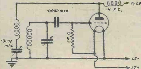
Fig. 1.—The simplest reaction arrangement.
