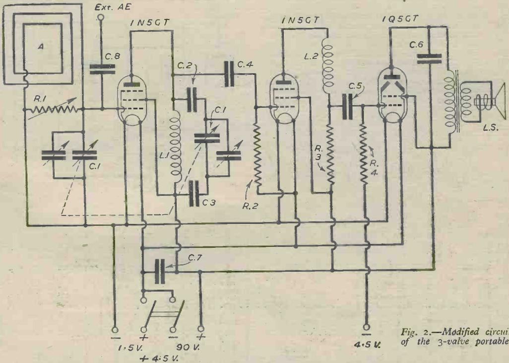
Fig. 2.—Modified circuit of the 3-valve portable.
