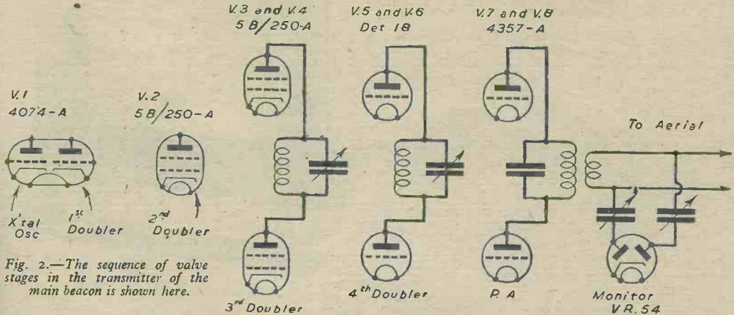
Fig. 2.—The sequence of valve stages in the transmitter of the main beacon is shown here.
