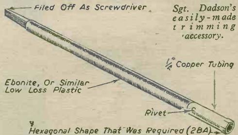
Sgt. Dadson's easily-made trimming accessory.
