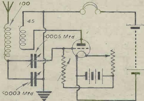
Fig. 1.—The Chitos circuit.
