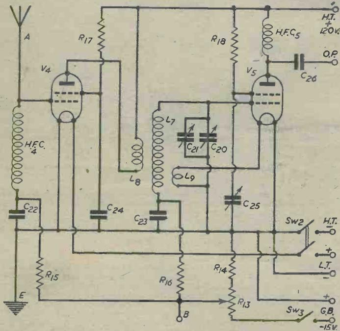
Fig. 1—Circuit of the Preselector.
