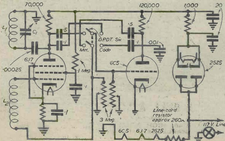
Fig. 2.—The metronome includes a multivibrator and an oscillator. It can be adjusted for widely different frequencies and even acts as a code oscillator. For higher frequencies the 0.1 condensers may be replaced by smaller (.01) units.
