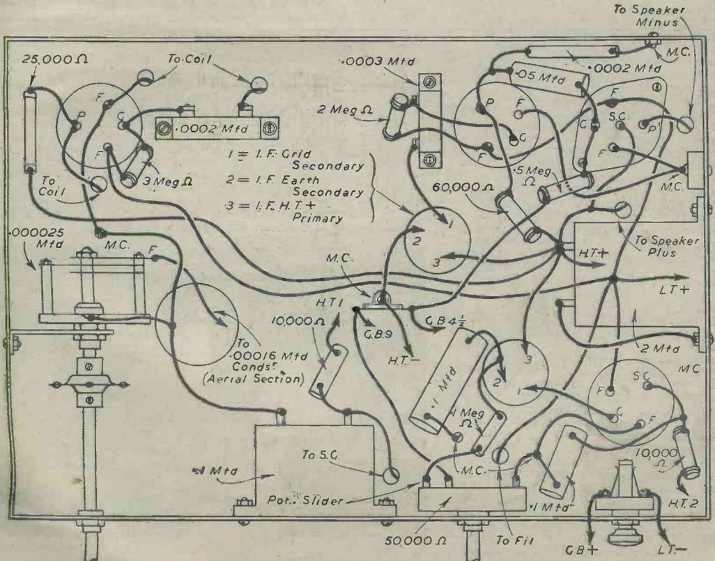
Fig. 5.—Under chassis wiring diagram, which may be compared with the photographic illustration above.
