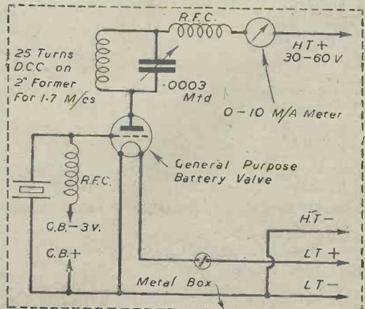
Fig. 2.—Test oscillator for the crystals.
