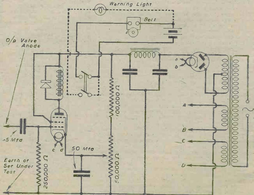
Circuit of the fault detector.
