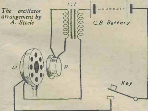
microphone, one low resistance headphone, 1 : 1 transformer, key and a G.B. battery. The pitch of signal can be adjusted by altering the distance (usually about 1/4 in.) between the microphone and receiver.
