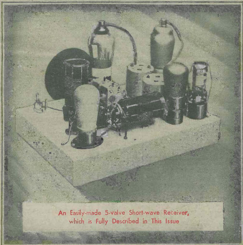
An Easily-made 5-valve Short-wave Receiver,
