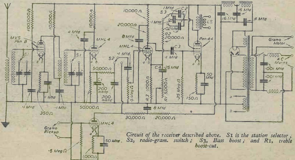
The usual disadvantage of this circuit, in that A.V.C. voltage cannot be obtained as it stands, does not apply in this instance since A.V.C. is not required.
