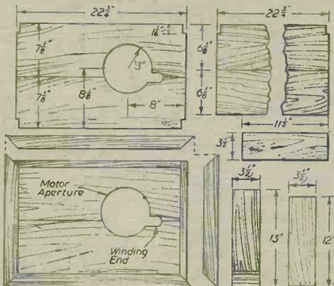
Fig. 5.—Motor board, shelves and divisions, with top plan.
