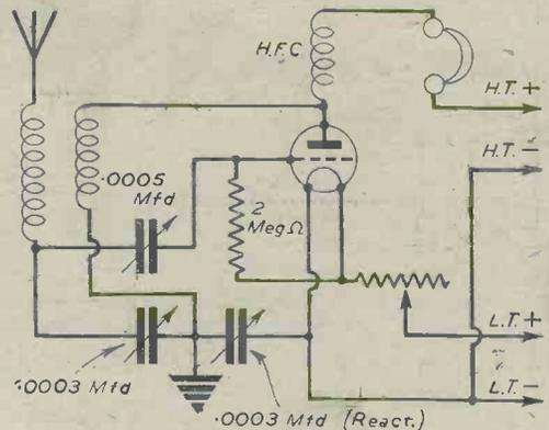
Fig. 2.—A modified Chitos circuit.
