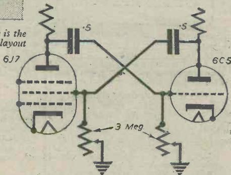
Fig. 4.—Fundamental circuit of the device.
