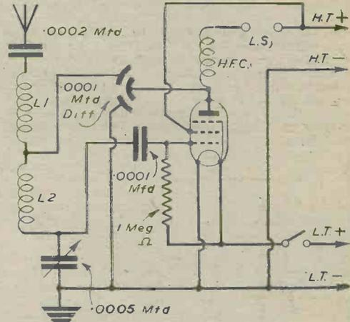
Fig. 4.—A modified Ultra-Audion circuit.
