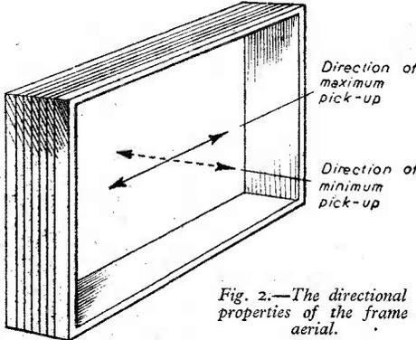
Fig. 2.—The directional properties of the frame aerial.
