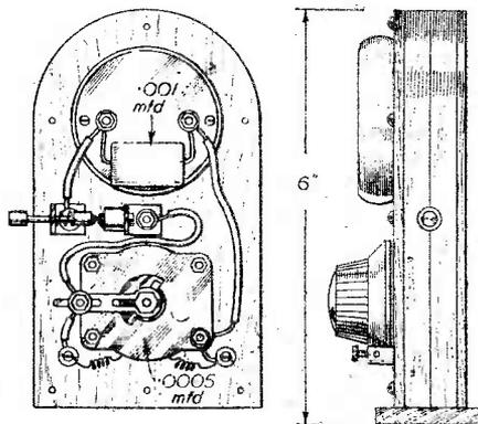
Fig. 3.—Back view showing wiring with side elevation of the completed receiver.
