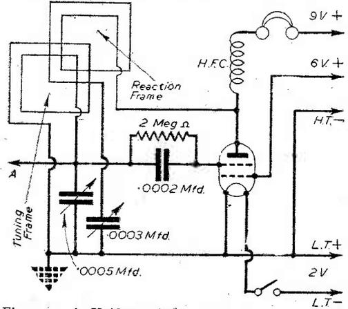
Fig. 23.—A Unidyne circuit adapted as a one-valve portable.
