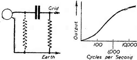
Fig. 3.—An alternative bass cut filter which is more drastic than the arrangement at Fig. 2. If it is desired to provide the pick-up with a D.C. circuit, e.g., when using a crystal pick-up, the resistance shown dotted may be inserted, but must have a high value.
