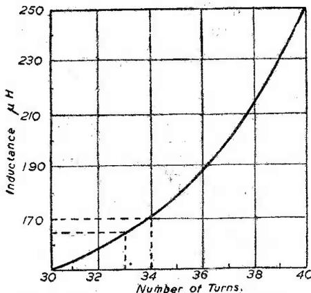
Fig. 5.—An example of inductance calculation.
