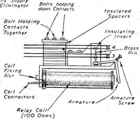
Fig. 2.—The arrangement of the relay, after modification. It should be noted that contacts 1 and 2 are immediately behind contacts 3 and 4; shown in the side view of the relay.
