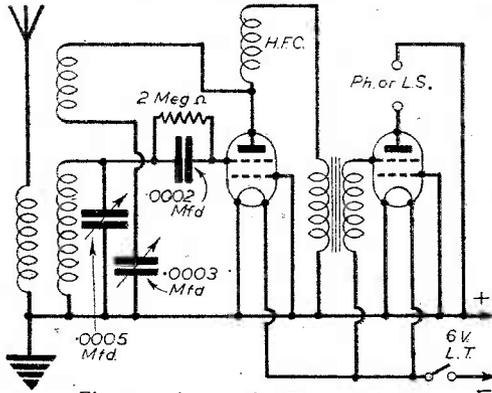
Fig. 22.—A two-valve Unidyne circuit.
