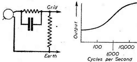
Fig. 2.—A bass cut filter, which has the advantage of setting a minimum limit of attenuation.
