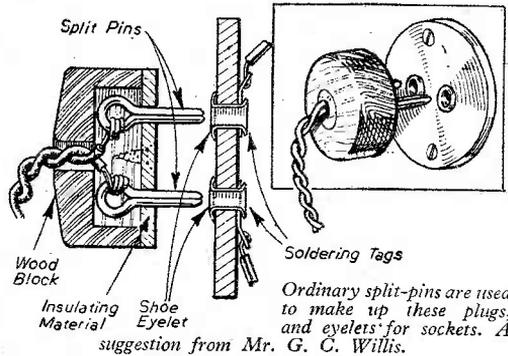
on the protruding portion of the eyelet or alternatively riveting over as illustrated.
