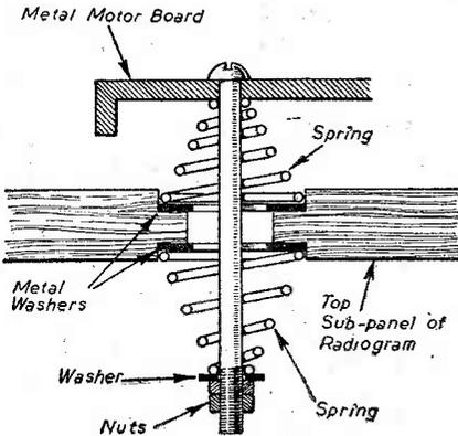
Fig. 1.—A sectional drawing showing a convenient method of spring mounting a gramophone motor assembly.
