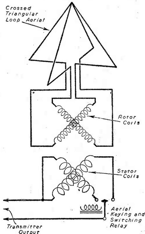
Fig. 6.—The arrangement of a Bellini-Tosi loop aerial system and associated radio-goniometer. The pair of stator and rotor coils are rigidly mounted at right-angles, while the rotor is free to rotate within the stator; a 360 degree scale is provided to indicate the position of the rotor.
