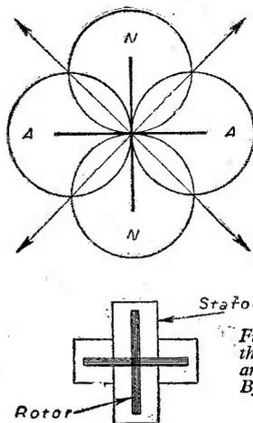
Fig. 9. (above)—When using an Adcock aerial system the polar diagram can be distorted by the introduction and suitable phasing of a fixed aerial, as indicated here. By distorting the polar diagram it is possible to alter the angles between the equi-signal "legs."
