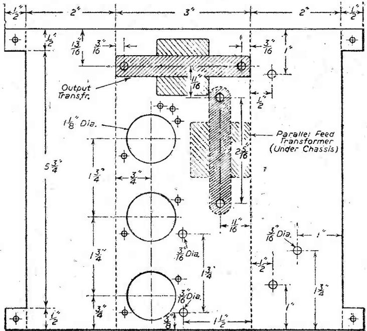
Fig. 3.—Details of the chassis.
