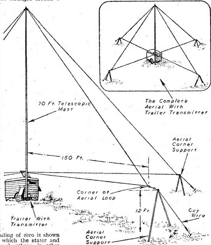
Fig. 5.—This sketch gives an impression of the appearance and set-up of a mobile radio range installation. When a mains supply is not available there is a second trailer which houses a petrol-electric set.
