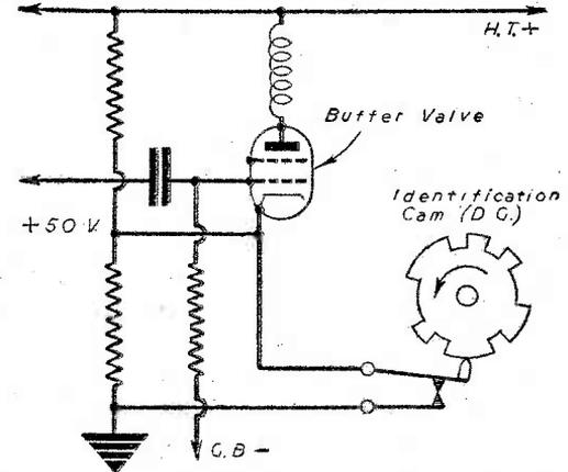
Fig. 11.—The identification cam, which automatically keys the transmitter with a two-letter call sign, operates a pair of contacts which open and close the bias circuit to the buffer valve connected between the R.F. oscillator and the intermediate amplifier stage.
