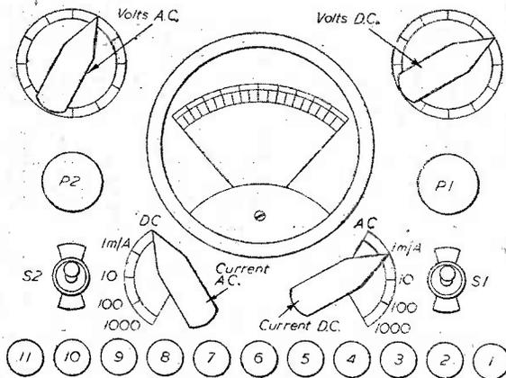
Fig. 3.—Layout of the panel and controls.
