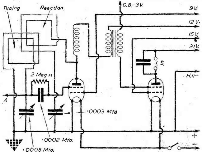
Fig. 24.—A two-valve portable using low values of H.T.
