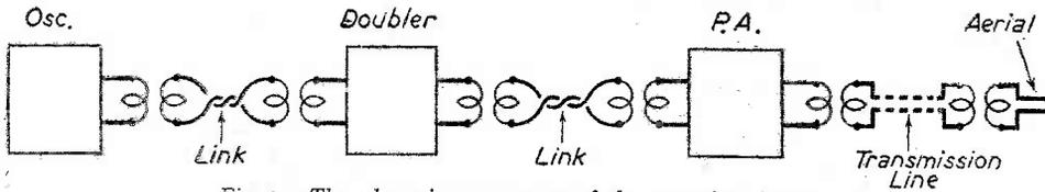
Fig. 2.—The schematic arrangement of the transmitter layout.
