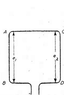
Fig. 1.—The simple loop aerial.
