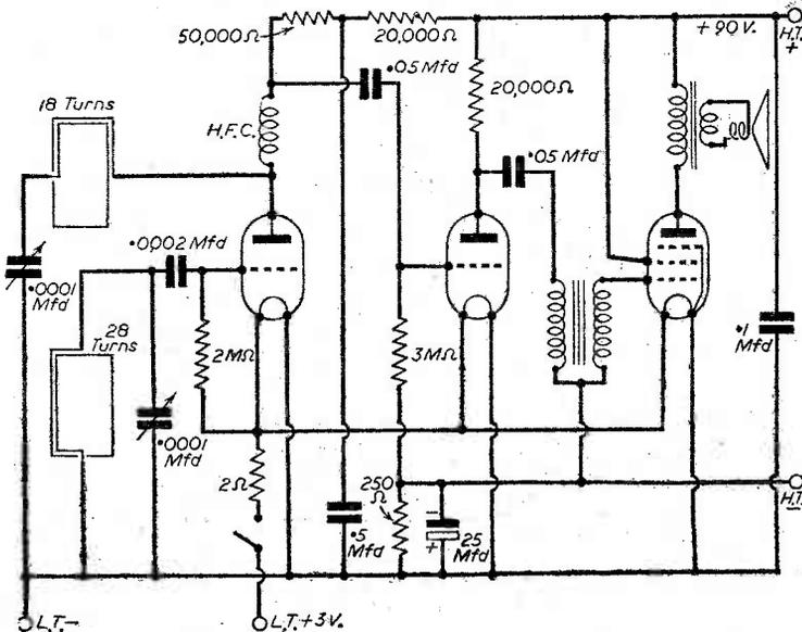
Fig. 1.—Theoretical circuit of the portable.
