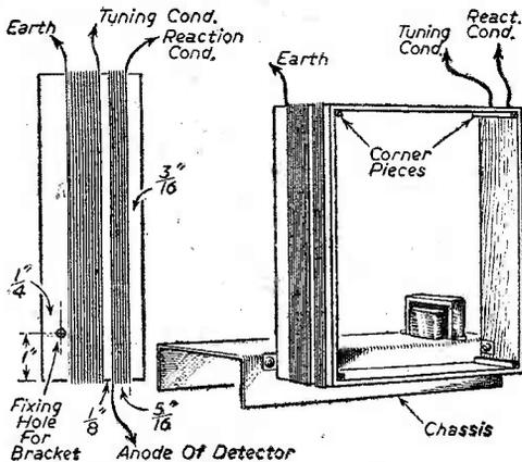
Fig. 2.—Details of the frame aerial.
