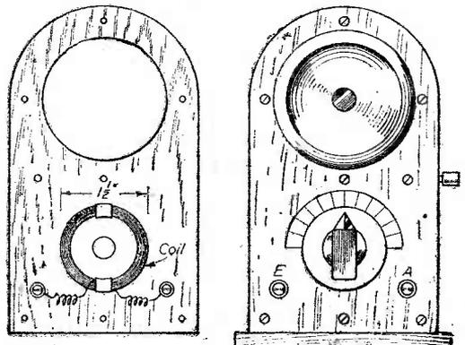
Fig. 2.—How the coil is connected, with front view of the set, showing smaller pointer knob and cardboard dial.
