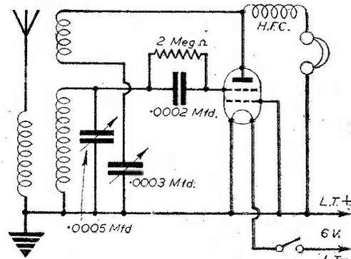
Fig. 21.—A one-valve Unidyne circuit.
