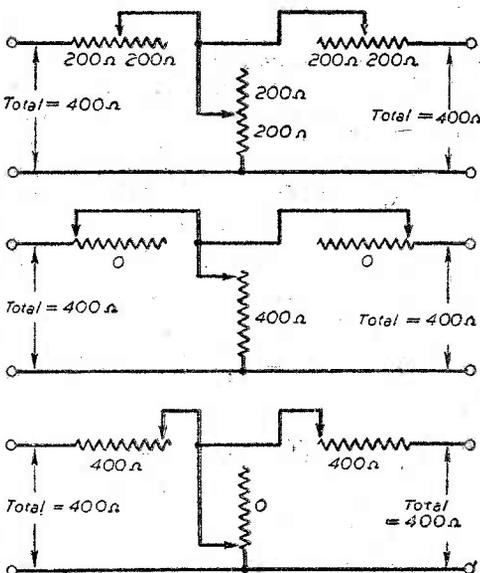
The circuit of the control at "full volume," "half volume" and "off."
