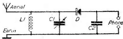
Fig. 4.—Theoretical circuit of the receiver.
