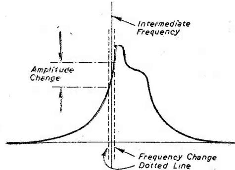
Fig. 4.—A diagrammatic representation showing how a misaligned I.F. transformer can produce a condition whereby a small change of frequency can cause a big change in amplitude.
