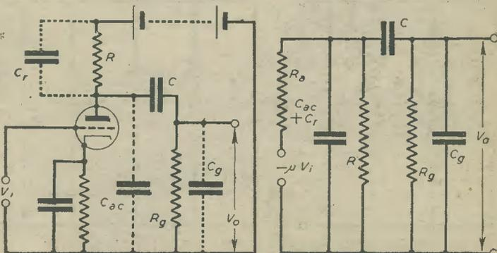
Fig. 3.—The practical resistance-coupled amplifier and its equivalent circuit.
