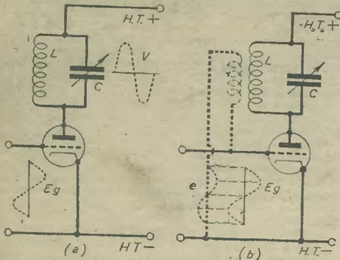
Fig. 1.—Showing how an H.F. amplifier can be "kept going" as an oscillator (b) if an e.m.f.  $e$  is injected back from anode to grid circuits in phase with  $E_g$ .
