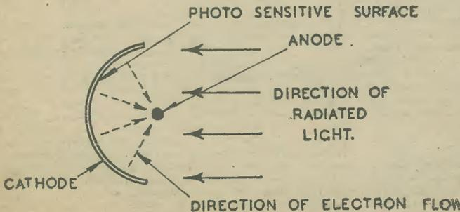
Fig. 1.—The principle of the photo-electric cell.
