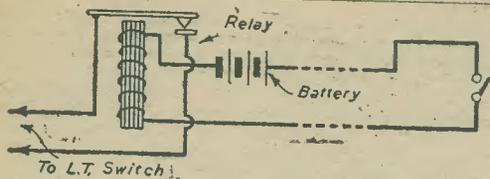
Fig. 4.—Where control at a distant point is required, a relay such as this should be used.
