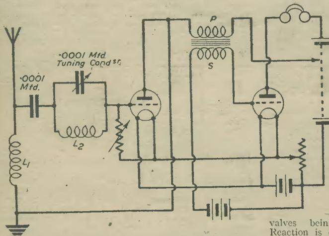
Fig. 5.—Showing a complete "N" circuit, with an L.F. amplifier added.
