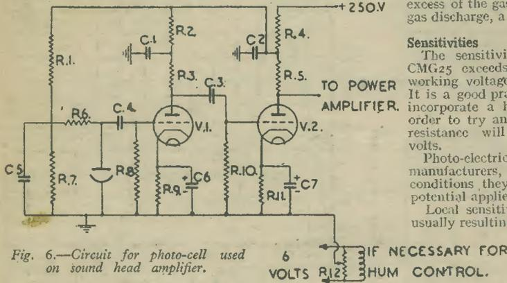
Fig. 6.—Circuit for photo-cell used on sound head amplifier.
