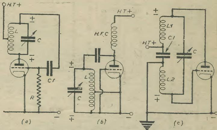
Fig. 6.—Forms of Hartley Oscillator, which show clearly how the e.m.f. returned to the grid is of opposite phase to the anode voltage.
