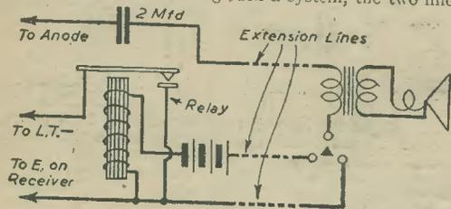
Fig. 5.—Complete extension control is obtained by this system.
