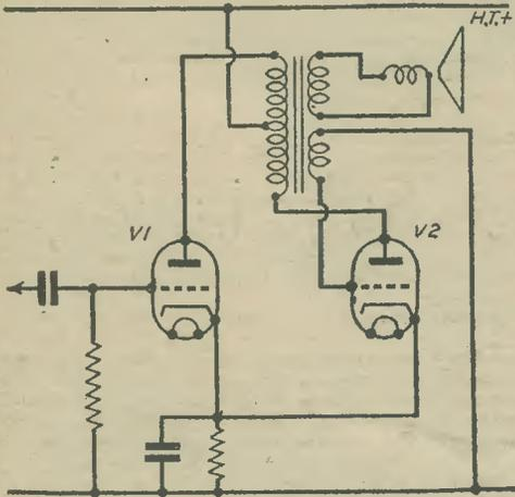
Fig. 1.—The output transformer with additional secondary winding to feed the second valve.
