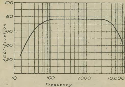
Fig. 4.—Frequency response curve of a typical amplifier.
