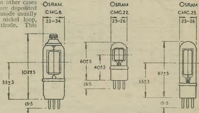
Fig. 2.—Typical designs of photo-electric cell having a rectangular-shaped cathode and rectangular wire loop for the anode.
