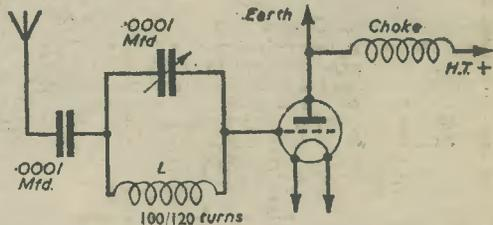
Fig. 3.—Correctly handled, this circuit is non-radiating.
