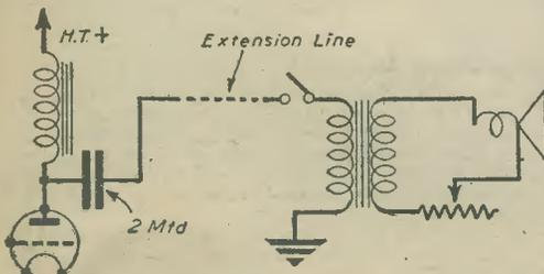
Fig. 2.—A volume control fitted at the extension point.
