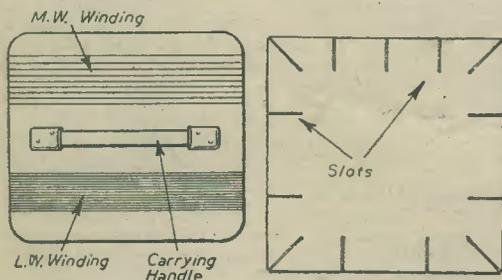
Fig. 6.—Top view of cabinet, showing position of aerial and carrying handle. Fig. 7.—Frame for winding a pancake aerial.
