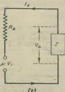
Fig. 2.—The simple equivalent circuit of the valve amplifier of Fig. 1.
