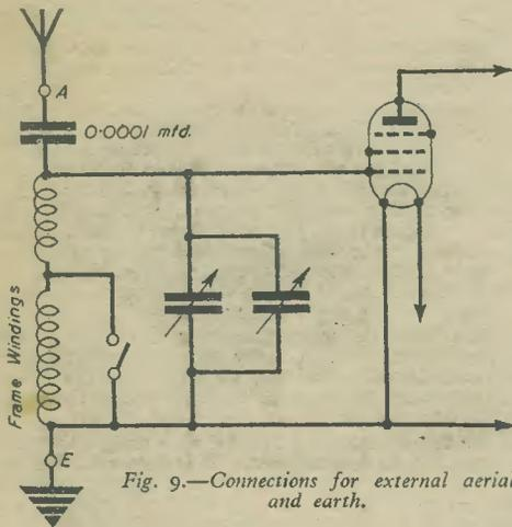
Fig. 9.—Connections for external aerial and earth.
