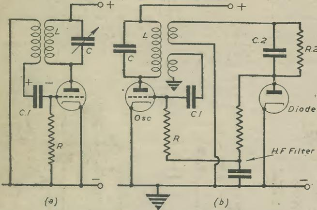
Fig. 3.—(a) Self-bias by grid condenser-leak. (b) Simplified circuit diagram showing one way of using a separate diode rectifier for control bias.
