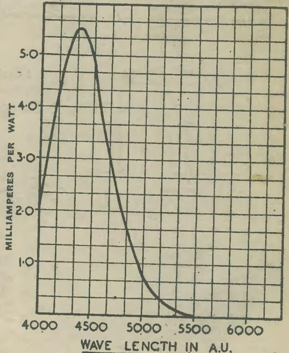
Fig. 5.—Average spectral sensitivity curve.
