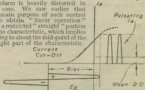
Fig. 5.—Class C operation: self-bias increases to about twice the current cut-off value.
