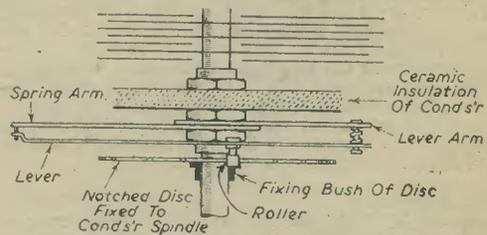
A locating device for bandspread tuning condensers (Mr. P. Redman).
