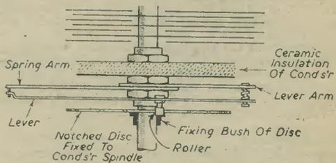
A locating device for bandspread tuning condensers (Mr. P. Redman).
