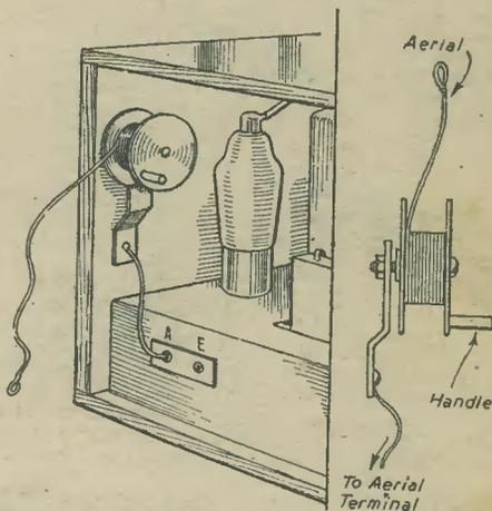
Fig. 6.—How a frame aerial may be added to an ordinary receiver.
