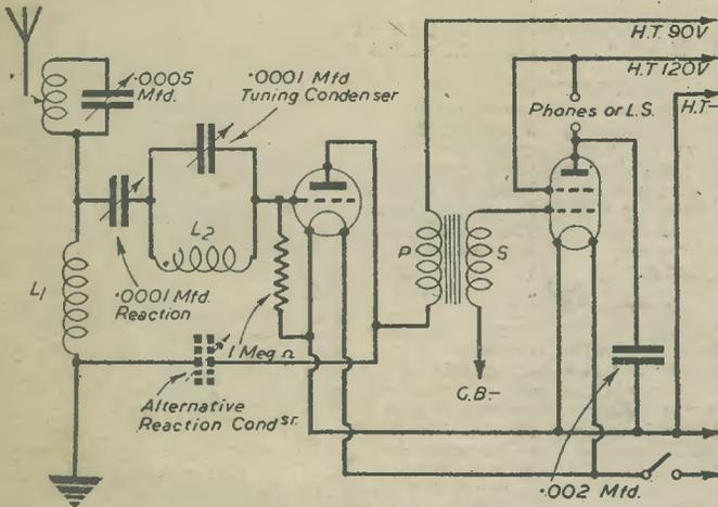
Fig. 6.—Fig. 5 modernised; care should be exercised that  $L_1$  and  $L_2$  are kept at right-angles.
