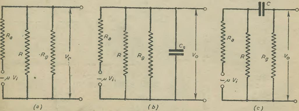
Fig. 5.—Equivalent circuit diagrams for the resistance-coupled amplifier for medium, high and low frequencies respectively.
