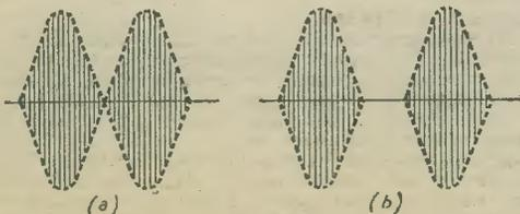
Fig. 4.—Illustrating "squegger oscillations."
