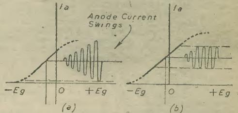
Fig. 2.—An oscillation will usually grow until the amplitude is restricted by the bends in the valve characteristic. (a). "Linear operation" (b) can be accomplished by amplitude control.
