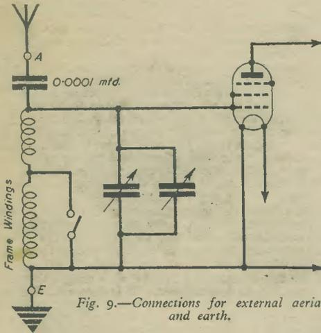
Fig. 9.—Connections for external aerial and earth.
