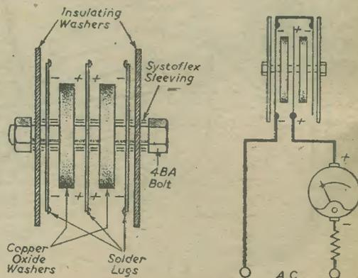
Details of the A.C. meter rectifier.
