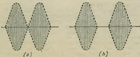
Fig. 4.—Illustrating "squegger oscillations."
