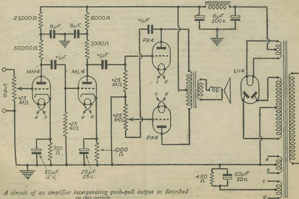
A circuit of an amplifier incorporating push-pull output as described in this article.
