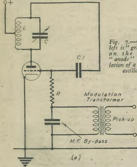
Fig. 7.—On the left is "grid," and on the right, "anode" modulation of a Class C oscillator.
