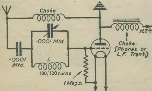
Fig. 4.—The choke connected between aerial and earth in this circuit is to prevent the break-through of strong signals.
