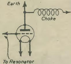
Fig. 2.—In this circuit the aerial resonates at the frequency of the grid.
