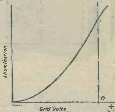
Fig. 19.—Due to non-linearity of the tube grid-brilliance characteristic the picture loses contrast in the dark regions.
