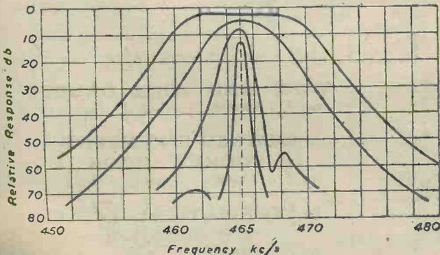
Fig. 1.—Typical I.F. selectivity curves of a modern high-grade receiver.
