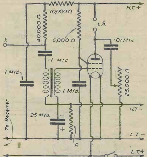
Fig. 2.—A parallel-fed transformer-coupled amplifier.
