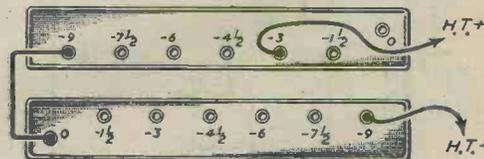
Fig. 6.—Connections for the two grid-bias batteries.
