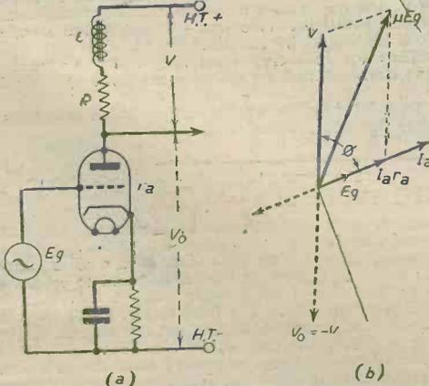
Fig. 6.—Vector diagram for load having resistance and inductive reactance.
