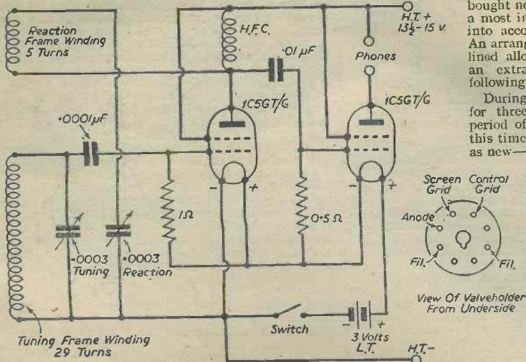
Fig. 1.—Theoretical circuit of the Portable, and Valveholder connections.
