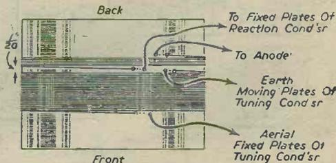
Fig. 3.—Details of the Coil.
