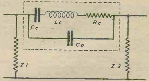
Fig. 4.—Theoretical representation of the circuit of Fig. 2.
