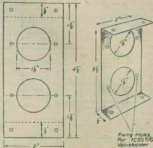
Fig. 4.—Valve mount details.
