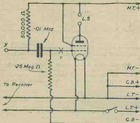
Fig. 1.—A simple amplifier stage using a tetrode valve.
