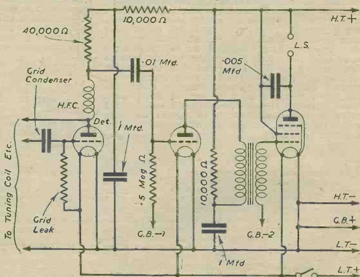
Fig. 3.—A three-stage amplifier with "mixed" couplings.
