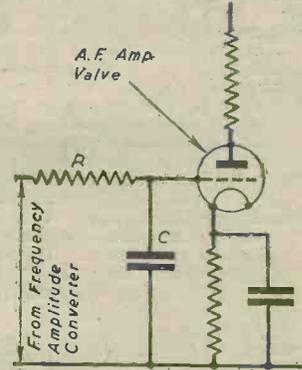
Fig. 2.—De-emphasis can be accomplished by a single top-cut filter, R and C.
