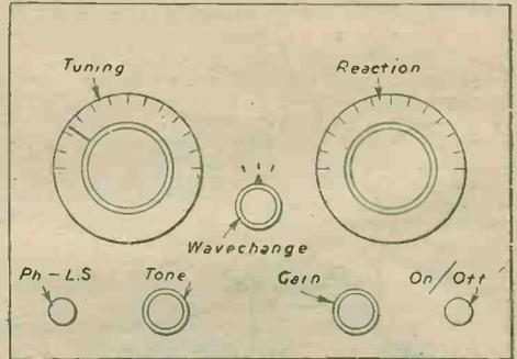
Fig. 5.—Layout of the panel controls.
