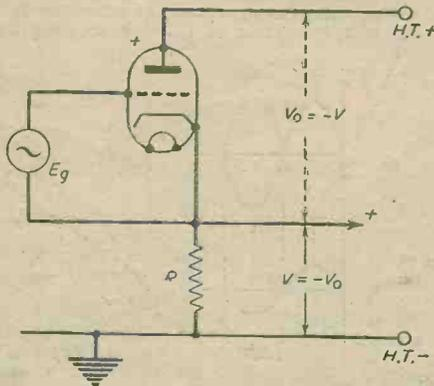
Fig. 3.—If the load resistance R were put on the cathode side, the output voltage would be  $V = -V_o$ . There is no phase-reversal such as exists across the valve.
