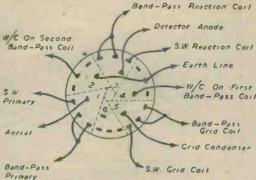
Fig. 4.—Details of the switch wiring.
