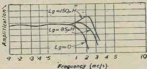
Fig. 14.—These curves show the amplification with various loads.
