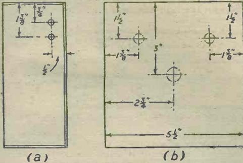
Fig. 2.—Cabinet side and front, with drilling details.
