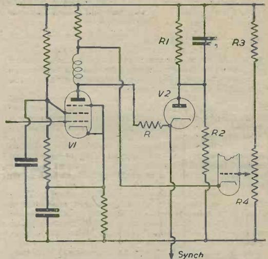
Fig. 26.—Another form of synch separator following an anode bend detector stage.
