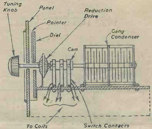
Fig. 6.—Automatic wave-change switching.
