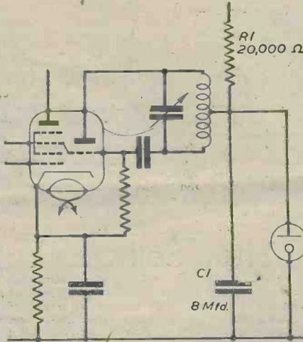
Fig. 3.—The use of a voltage stabiliser to prevent frequency variation caused by audio frequency feed-back or hum.
