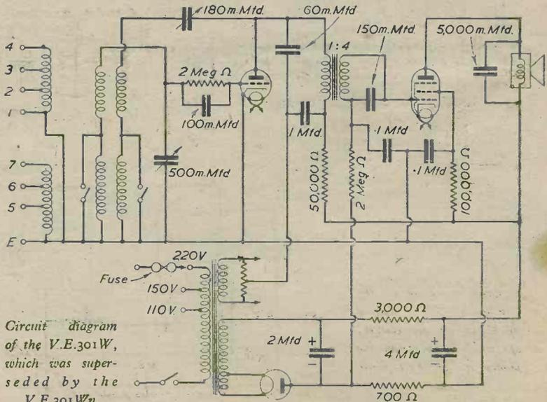
Circuit diagram of the V.E.301W, which was superseded by the V.E.301Wn.
