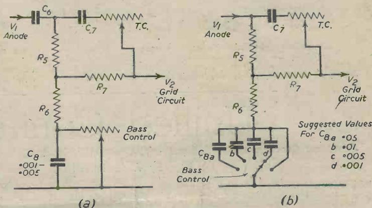
Fig. 6.—Alternative arrangements for variable "bass boost" as described in the text.
