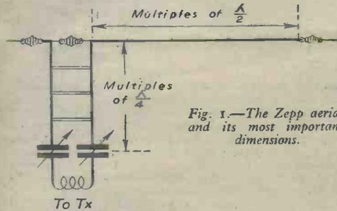
Fig. 1.—The Zepp aerial and its most important dimensions.
