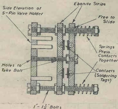
Constructional details of a switch plug for disconnecting the heater and smoothing condenser wiring on an A.C. receiver.—J. D. Lee (Leicester).
