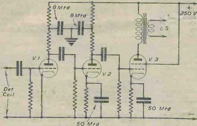
Fig. 1.—Standard L.F. amp. circuit with decoupling.
