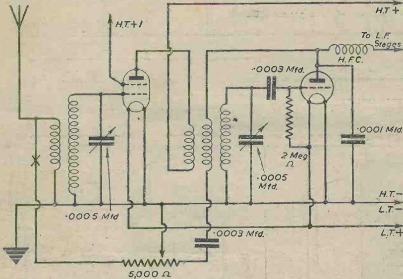
Fig. 1.—Combined reaction and H.F. input control.
