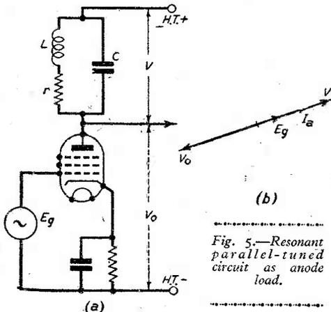
Fig. 5.—Resonant parallel-tuned circuit as anode load.
