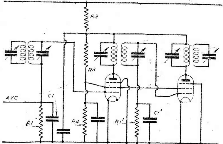
Fig. 4.—A similar circuit to Fig. 3, but R.C. coupling replaced by a tuned transformer; not often used, but illustrates more clearly the twin-stage action.
