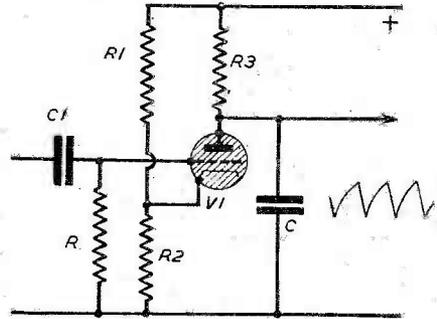
Fig. 34.—The basic gas-discharge circuit.
