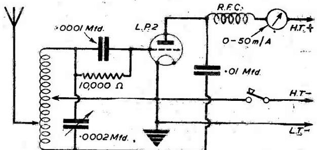
Fig. 1.—This simple transmitter uses the Hartley arrangement.
