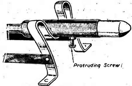
Keeping the soldering-iron in place.
