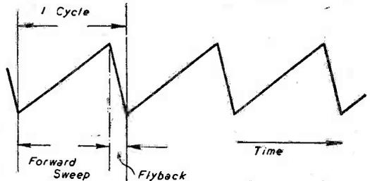
Fig. 33.—Sawtooth waveforms such as are applied to the tube deflector plates for production of a raster.
