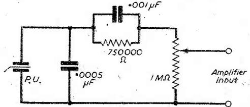
Fig. 5.—Compensating circuit for crystal pick-up.
