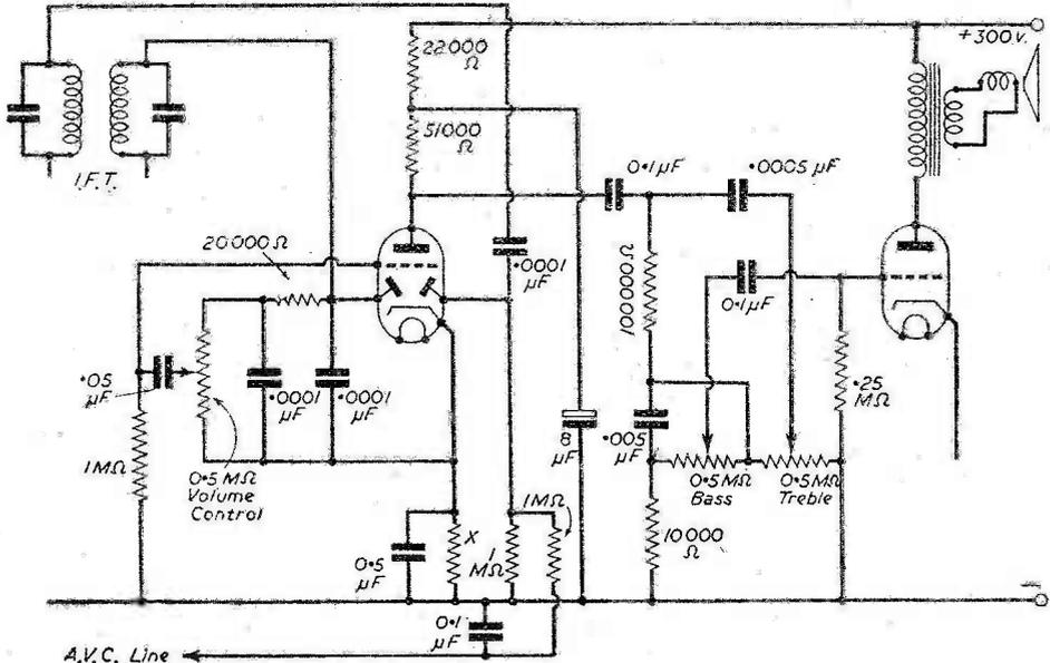
Fig. 11.—Detector, A.V.C. and tone control stage.
