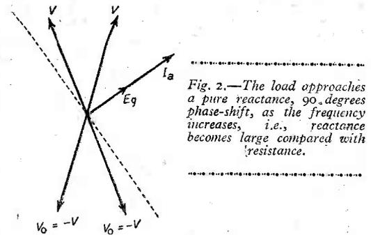
Fig. 2.—The load approaches a pure reactance, 90 degrees phase-shift, as the frequency increases, i.e., reactance becomes large compared with resistance.
