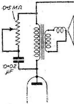
Fig. 12.—Simple treble attenuator.
