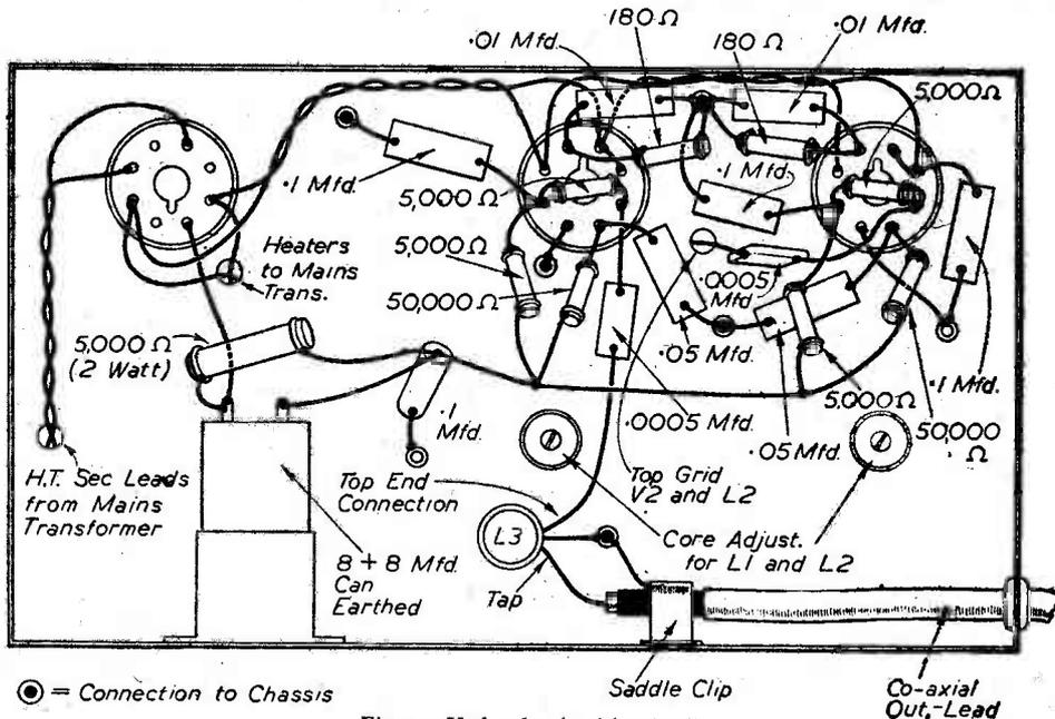
Fig. 4.—Under chassis wiring details.
