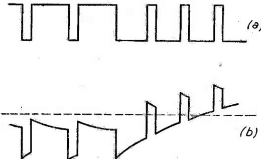
Fig. 31.—The effect of the frame separator circuit of Fig. 1 on the frame synch. pulses.
