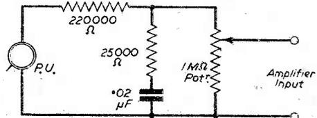
Fig. 4.—Bass boosting pick-up circuit.
