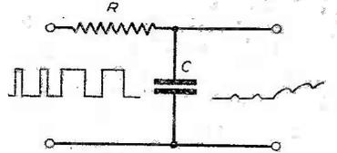
The effect of passing the line and frame synch. pulses through a differentiating circuit of the above nature is shown for even and odd frame endings in Fig. 27 (b) and (e) respectively.
