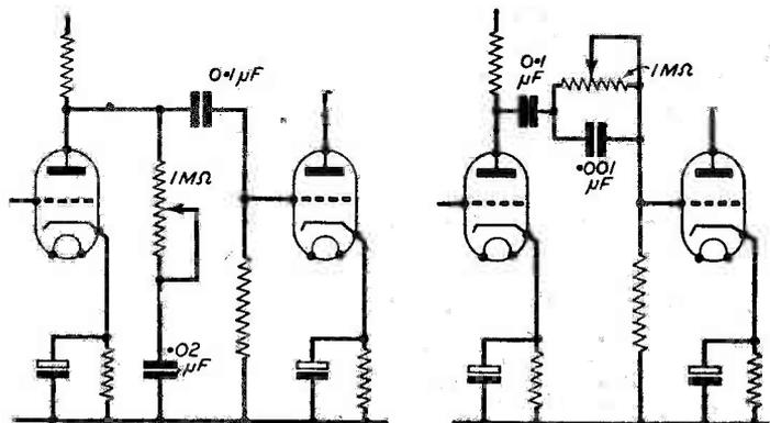
Fig. 3.—(a) Treble attenuator. (b)—right—Bass attenuator.
