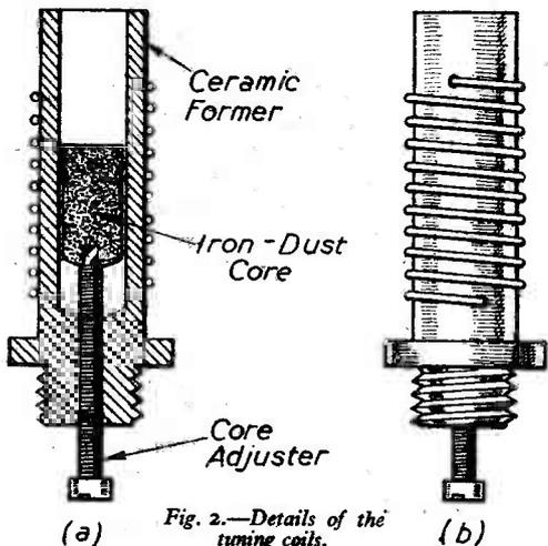
Fig. 2.—Details of the tuning coils.
