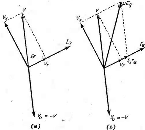
Fig. 3.—(a) The applied voltage  $V$ , across the load, is the vector sum of two 90 degree components,  $V_x$  and  $V_r$ . In (b), the internal voltage-drop  $I_a r_a$  is again added vectorially to  $V$ , giving the total equivalent generator e.m.f.,  $\mu E_g$ .
