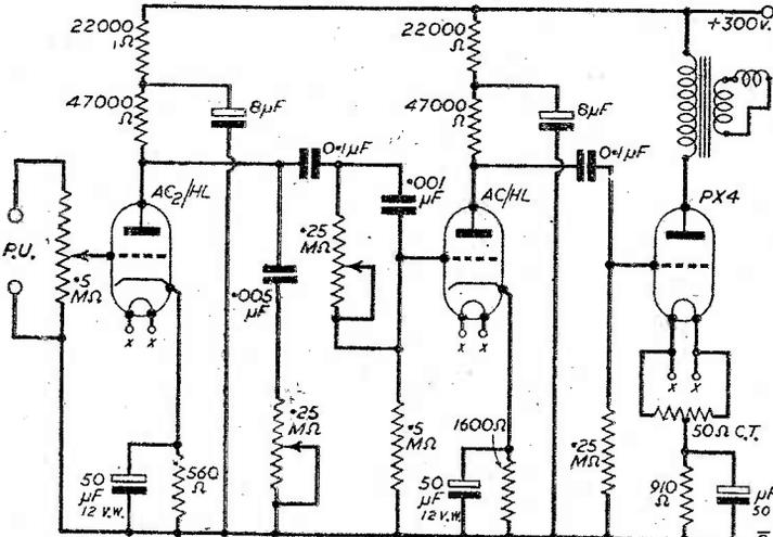
Fig. 7.—3-stage amplifier, with bass and treble attenuation.
