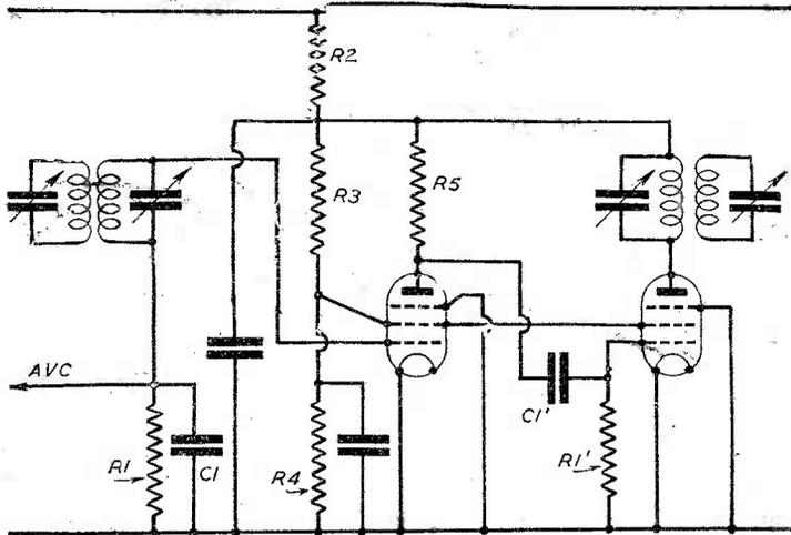
Fig. 3.—A two-stage amplitude limiter; compromise is not necessary as each stage performs its task under optimum conditions. Suggested values are:  $R_1$ —50,000 $\Omega$ ;  $C_1$ —90pfd.;  $R_1'$ —200,000 $\Omega$ ;  $C_1'$ —250 pfd.;  $R_5$ —5,000 $\Omega$  (approx.).
