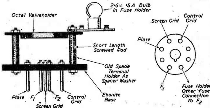
Adapting a standard valveholder to enable low-voltage valves to be used.
