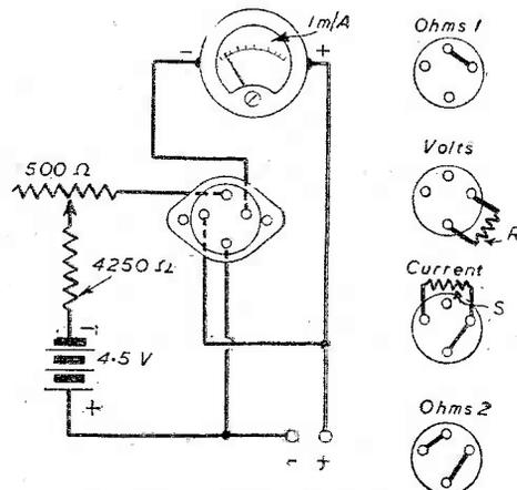
Circuit and plug-in attachments for the multi-meter.
