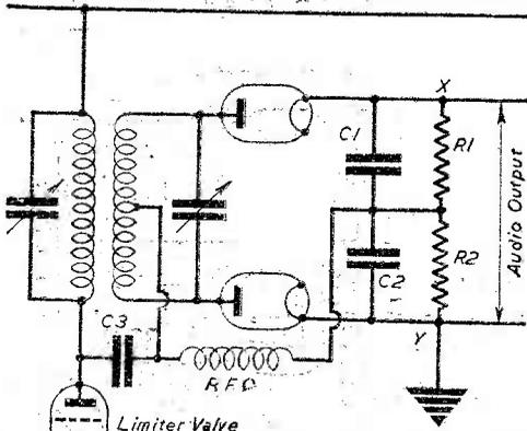
Fig. 6.—The phase-discriminator; frequency-amplitude converter; values are the same as for Fig. 5. The inductance of the radio frequency choke should be appropriate for intermediate frequency or be replaced by a resistance.
