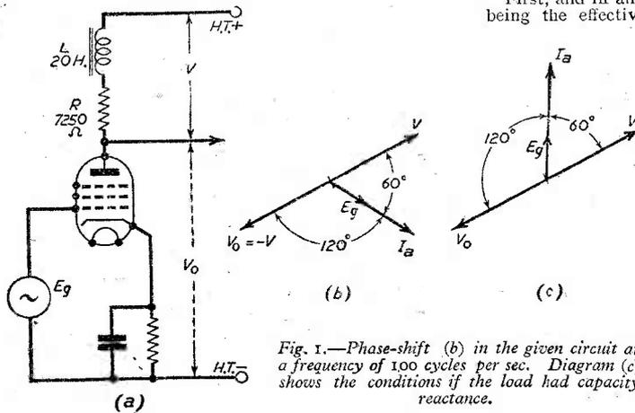
Fig. 1.—Phase-shift (b) in the given circuit at a frequency of 100 cycles per sec. Diagram (c) shows the conditions if the load had capacity reactance.
