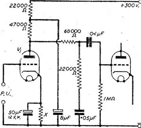
Fig. 6.—Bass boosting first stage (triode).
