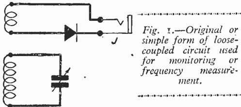
Fig. 1.—Original or simple form of loose-coupled circuit used for monitoring or frequency measurement.
