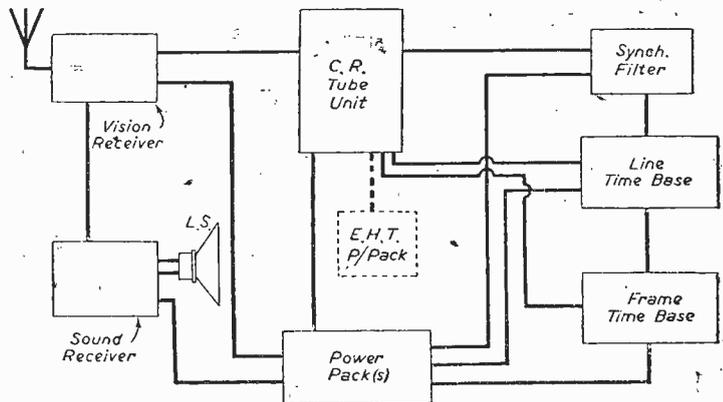
Diagram showing the general arrangement of a modern television picture and sound receiver.
