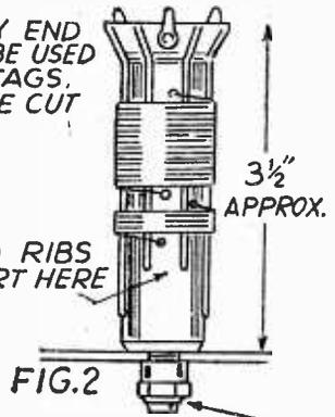
NOZZLE END AND CAP CUT OFF. END OF CAP IS THREADED, AND ACTS AS NUT, WHEN FIXING BELOW ALUMINIUM PANEL.
