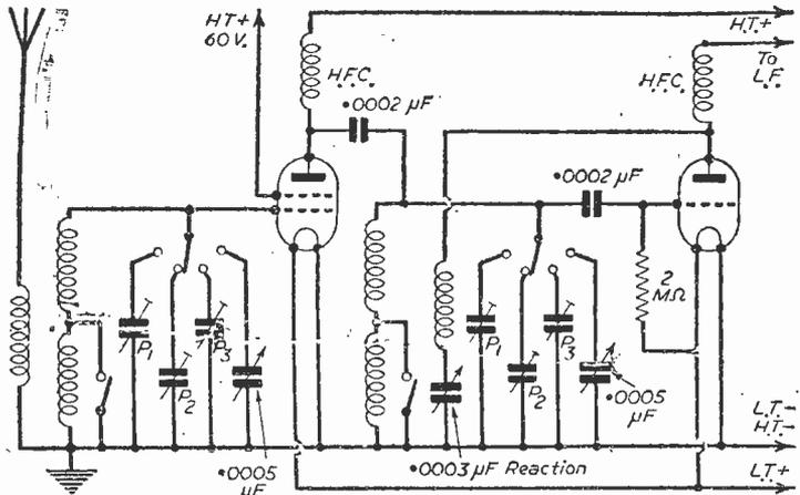
Fig. 2.—The same type of switch is used in this circuit, but manual tuning is provided and a reaction circuit is included.
