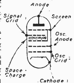
Fig. 2.—Electrode functions of a pentagrid.
