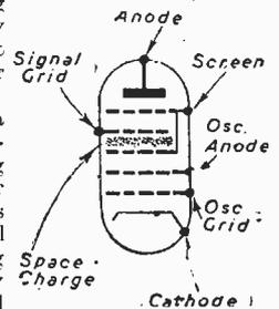
Fig. 2.—Electrode functions of a pentagrid.
