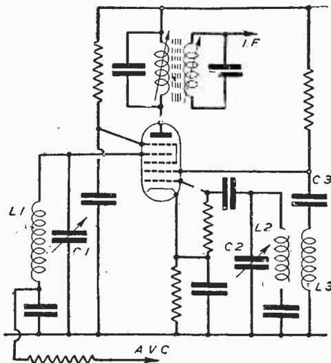
Fig. 1.—A typical modern frequency-changing stage.
