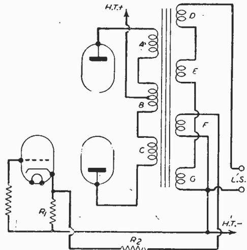
Fig. 2.—This method of providing feed-back should reduce phase shift.
