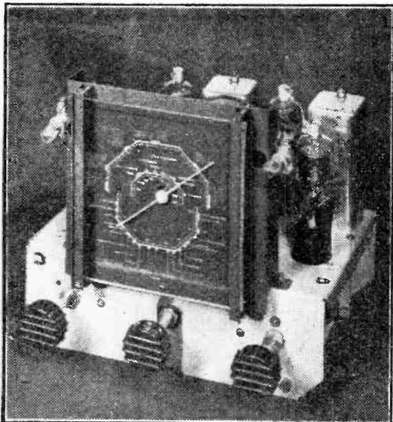
The R.M. "Radio Feeder," a three-waveband three-valve unit for addition to a standard power supply and amplifier.
