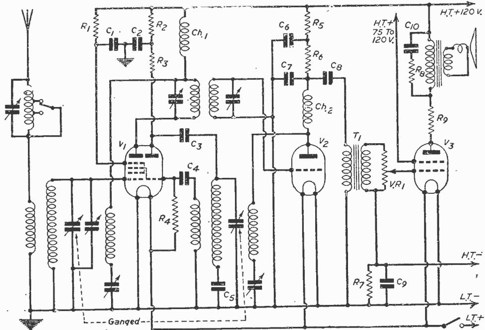
Fig. 2.—Battery version of a circuit on the lines of Fig. 1.
