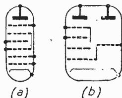
Fig. 3.—Showing (a) an octode, and (b) a triode-hexode type of frequency-changer.
