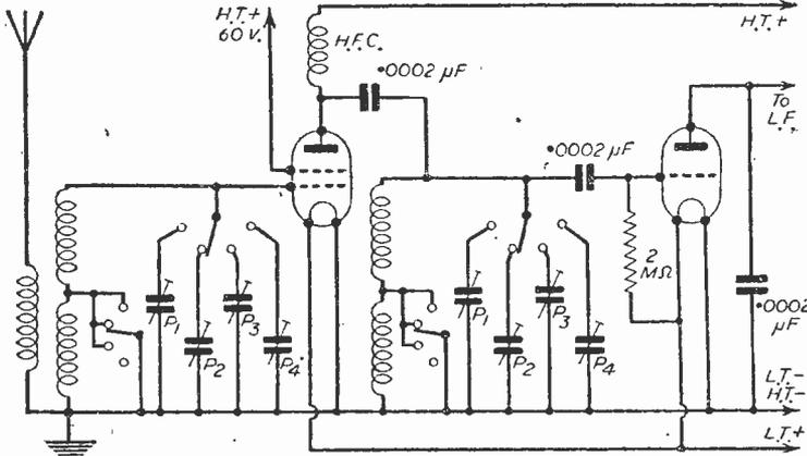
Fig. 1.—A simple two-valve with a rotary 4-position switch assembly to provide choice of four stations.
