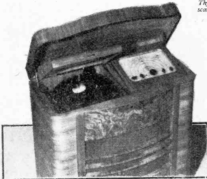
*The Eiber Conqueror, type K.129R, made by Dynatron, is fitted into a Regency cabinet, and as may be seen has a special lid for the record reproducing section, and a sloping panel on the radio side.*
