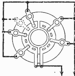
How to arrange the additional contact (shown by the broken lines above).
