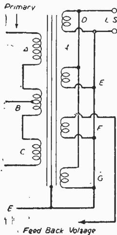
Fig. 1.—How section-alised windings may be arranged on a multi-ratio output transformer.
