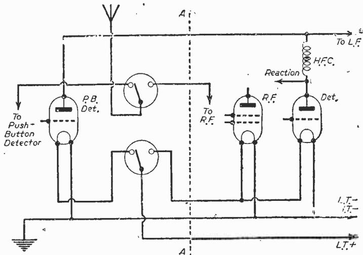
Fig. 6.—A simple method of adding push-button switching without interfering with normal circuit arrangements.
