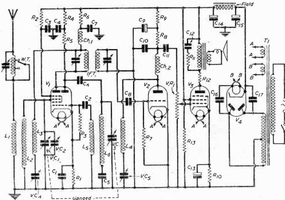
Fig. 1.—A.C. Mains Short-wave Three as described.
