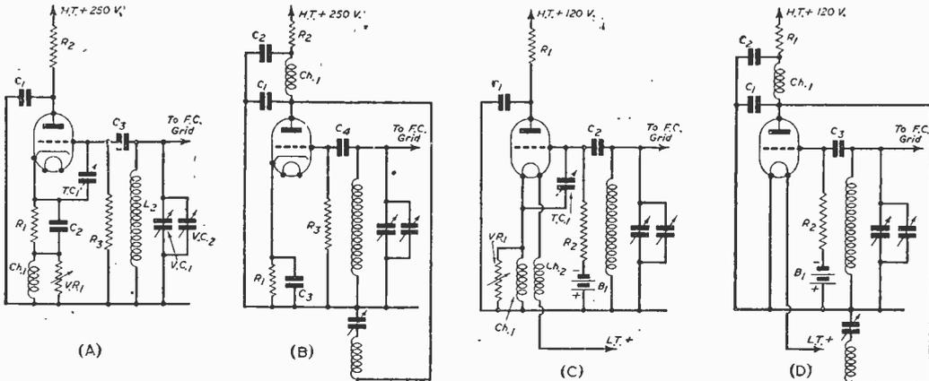
Fig. 3.—Electron-coupled cathode controlled reaction circuits.
