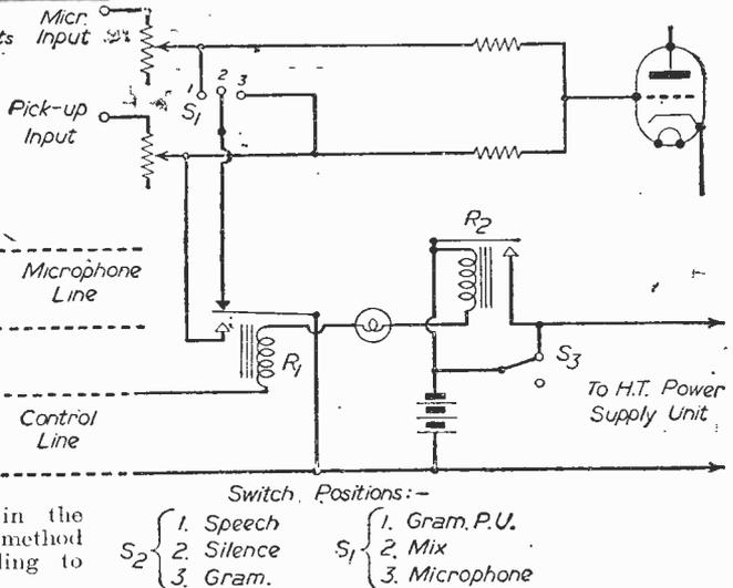
Fig. 2.—Battery-operated equipment may be switched as shown here.
