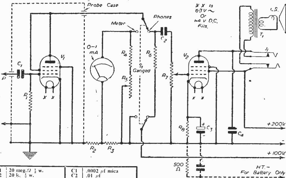
Fig. 1.—Theoretical circuit of the Signal Tracer.
