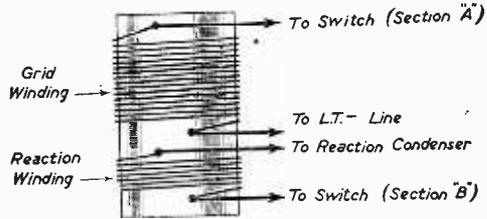
Fig. 5.—Coil winding and connection details.
