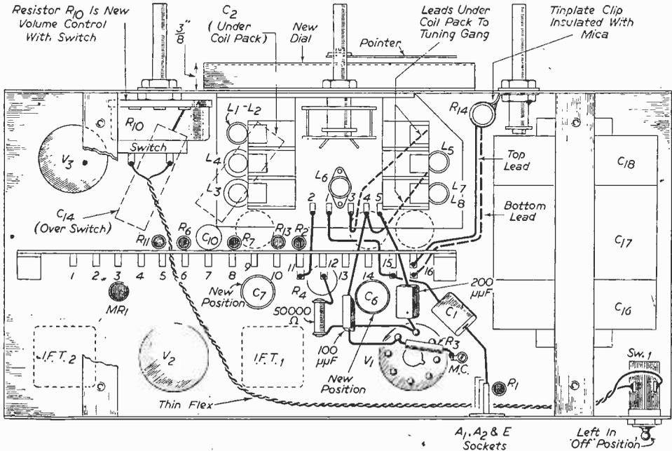
Fig. 3.—Under-chassis view showing coil pack in position. Dotted lines at tags 9, 14 and 16 on sub-panel show original position of C.7, C.6 and resistor R.14.
