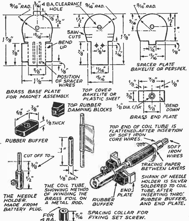
Fig. 1.—Main features of the pick-up.
