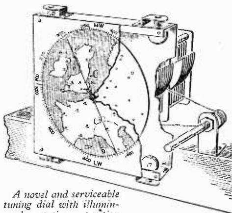
A novel and serviceable tuning dial with illuminated station position identification.
