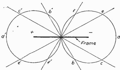
Fig. 1.—A typical frame aerial and the field plotted round it.
