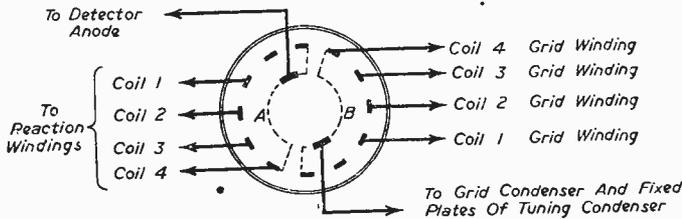
Fig. 4.—Details of connections to the switch.
