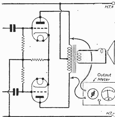
Fig. 4.—Measuring Output of a Push-pull Circuit.
