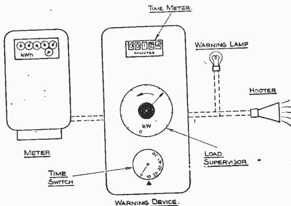
Diagram showing the method of arranging the warning device.
