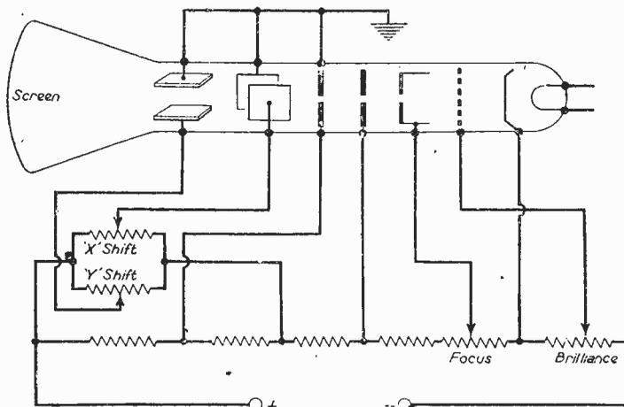
Fig. 1.—C.R.T. shift network, showing method of arranging X and Y shift controls.
