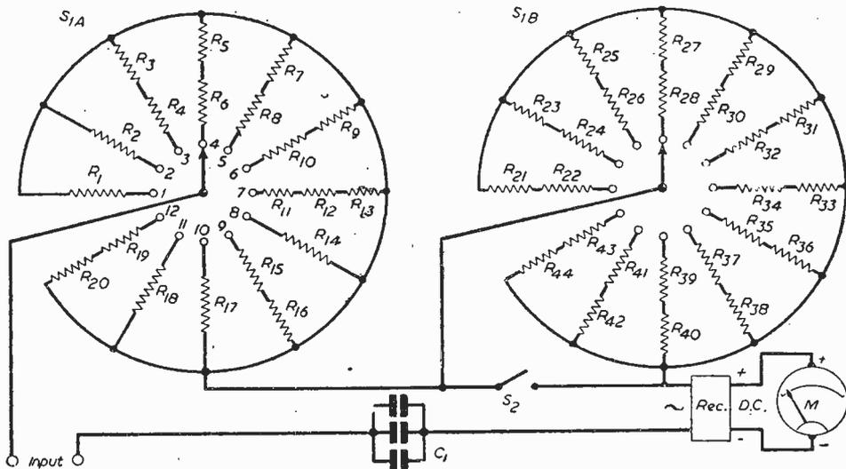
Fig. 2.—Circuit Diagram of the Output Meter described in this article.
