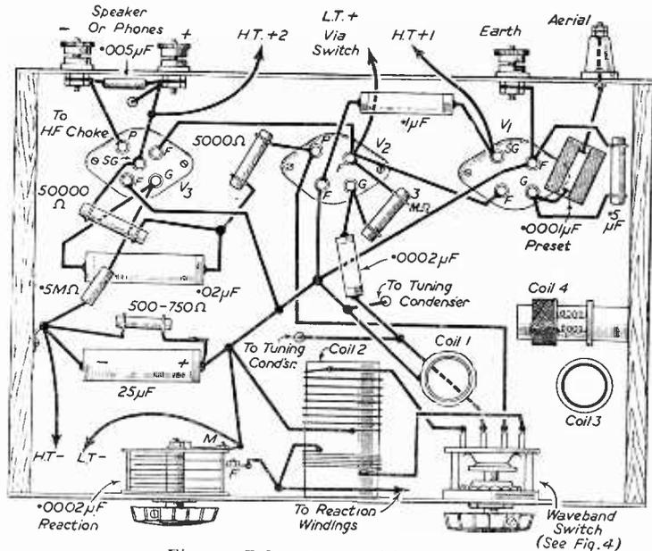
Fig. 3.—Below-chassis wiring details.
