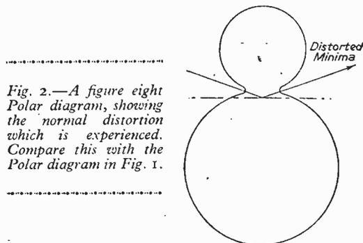
Fig. 2.—A figure eight Polar diagram, showing the normal distortion which is experienced. Compare this with the Polar diagram in Fig. 1.
