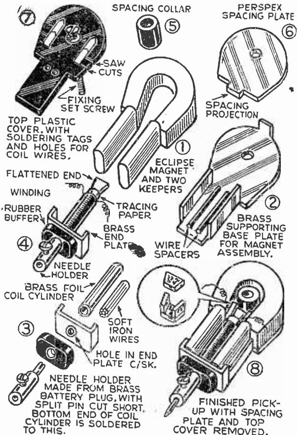
Fig. 2.—Main assembly details.
