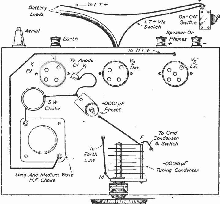
Fig. 2.—Above-chassis wiring details.
