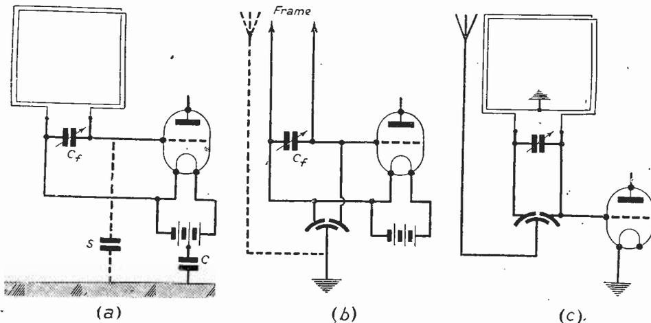
Fig. 3.—Three methods of correcting a circuit to avoid what is known as the "vertical effect."
