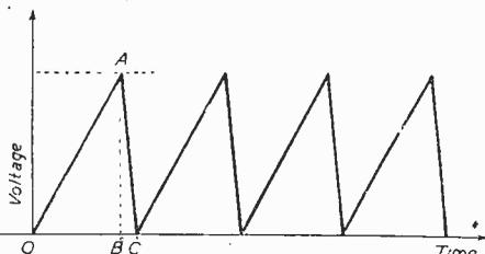
Fig. 2.—Linear time-base waveform, where OA equals the sweep, and BC is the flyback time.
