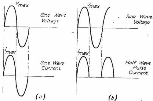
Fig. 4.—In an ordinary A.C. circuit, (a),  $V/I =$  a Resistance,  $R = V_{max}/I_{max}$ , where  $V$  and  $I$  are R.M.S. values, and  $V_{max}$  and  $I_{max}$  peak values. If the voltage is a sine-wave, but the current intermittent half-waves as in (b), does  $V_{max}/I_{max}$  still mean the resistance  $R$ ? Actually, it is a pulse load value.
