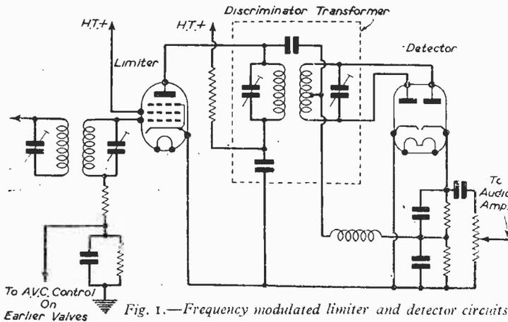
Fig. 1.—Frequency modulated limiter and detector circuits.
