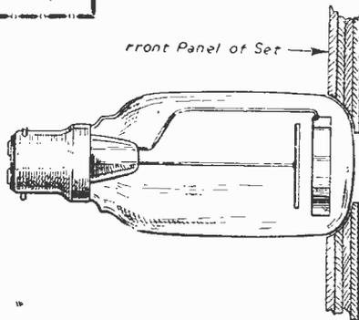
Using a Neon as a Polarity Indicator.
