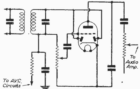
Fig. 2.—Conventional amplitude-modulated detector circuit which can be compared with Fig. 1.
