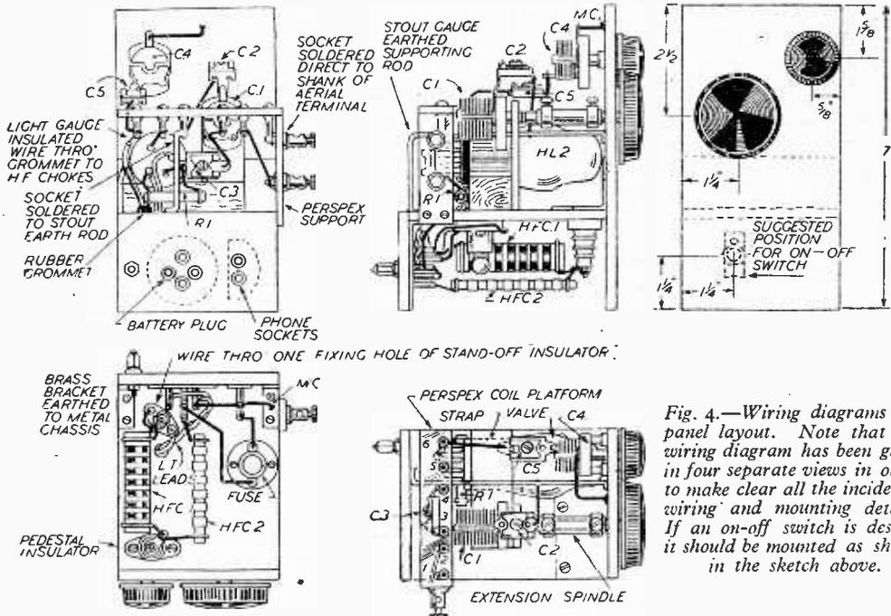
Fig. 4.—Wiring diagrams and panel layout. Note that the wiring diagram has been given in four separate views in order to make clear all the incidental wiring and mounting details. If an on-off switch is desired it should be mounted as shown in the sketch above.
