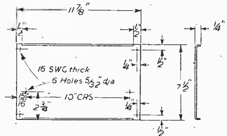
Fig. 3.—Details of the panel.
