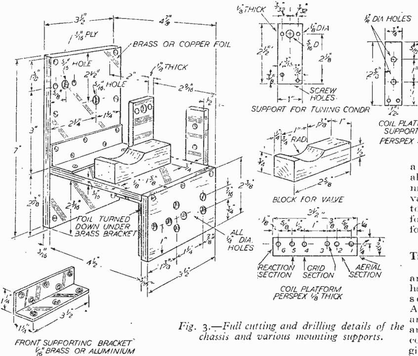
Fig. 3.—Full cutting and drilling details of the chassis and various mounting supports.
