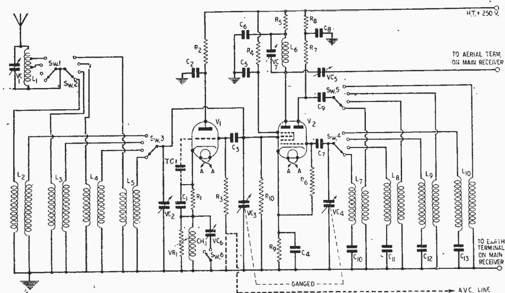
Fig. 1.—Theoretical circuit of the converter unit.
