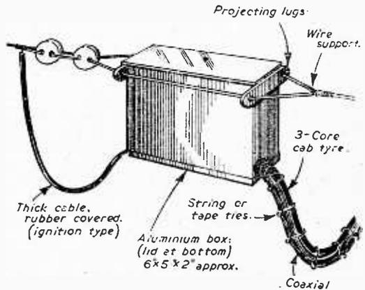
Fig. 1.—The completed Antistatic Aerial Unit shown mounted on the aerial.
