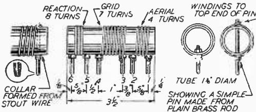
Fig. 5.—Full details of the coil unit.
