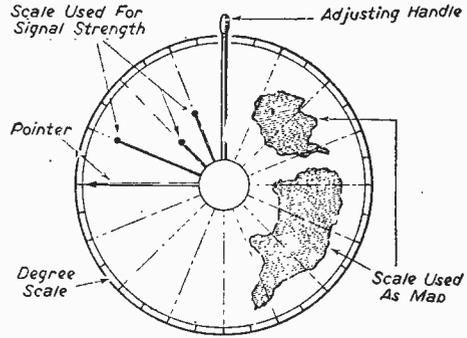
Fig. 7.—A plan of the Frame scale. This may be used for recording signal strengths on the inner portion. A map may be drawn centred on the frame and the relative distances marked off radially. The frame should be sited as high as possible and well away from earthed objects.
