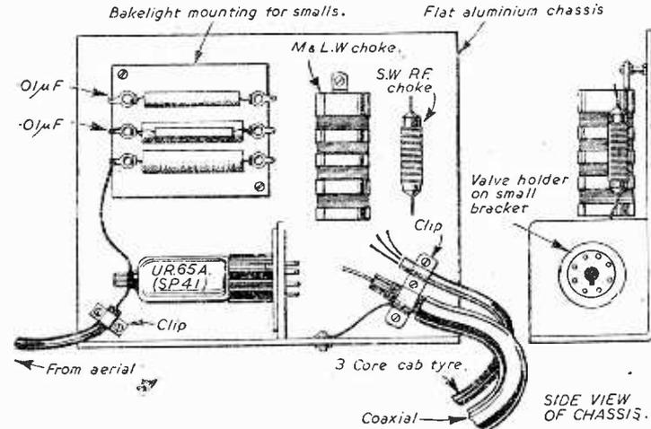
Fig. 3.—Layout of the component and an indication of the wiring of the aerial unit.
