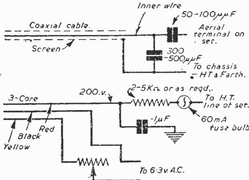
Fig. 4.—Circuit of the "house end" of the unit.
