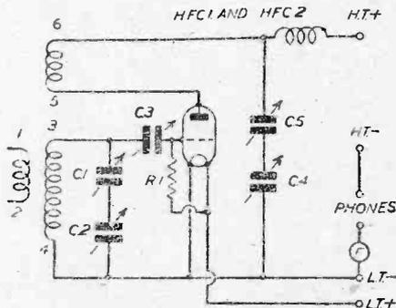
Fig. 2.—Theoretical circuit of the short-wave receiver.
