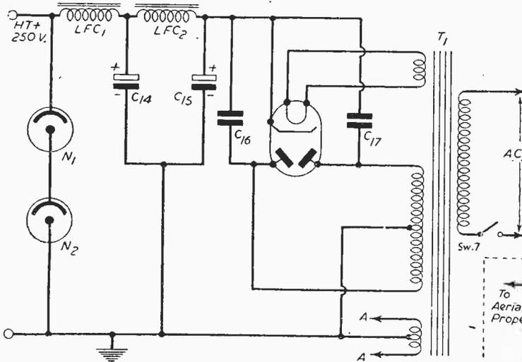
Fig. 2.—Circuit of the stabilised power pack.
