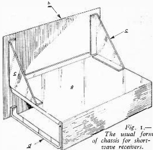
Fig. 1.—The usual form of chassis for short-wave receivers.
