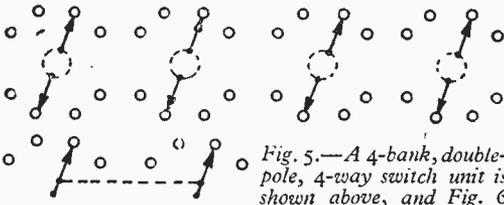
Fig. 5.—A 4-bank, double-pole, 4-way switch unit is shown above, and Fig. 6 an alternative method of showing the separate banks.
