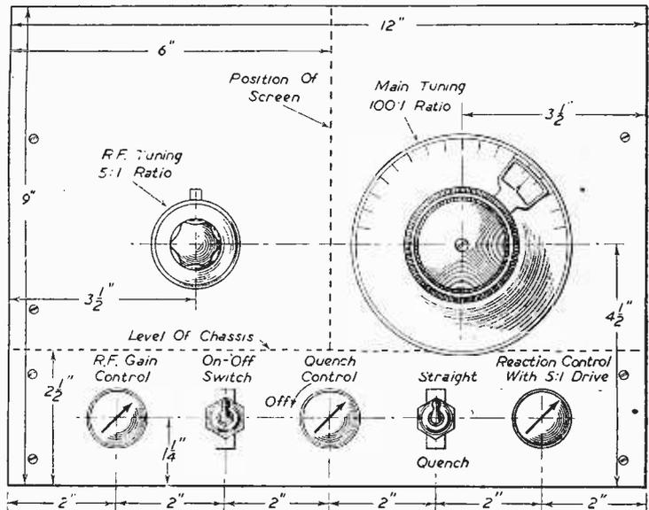
Fig. 3.—Layout and drilling dimensions of the panel.
