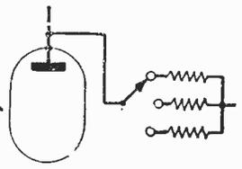
Fig. 3.—A simple circuit application of the multi-contact switch.
