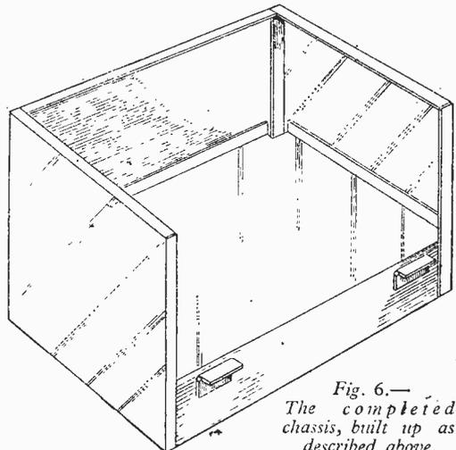
Fig. 6.—The completed chassis, built up as described above.
