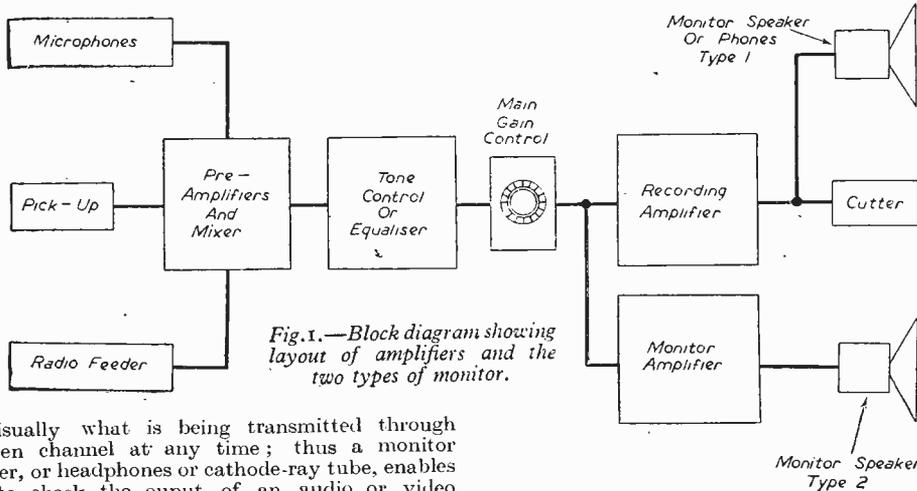
Fig. 1.—Block diagram showing layout of amplifiers and the two types of monitor.
