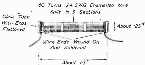
Fig. 8.—Constructional details of the low-resistance filament chokes.
