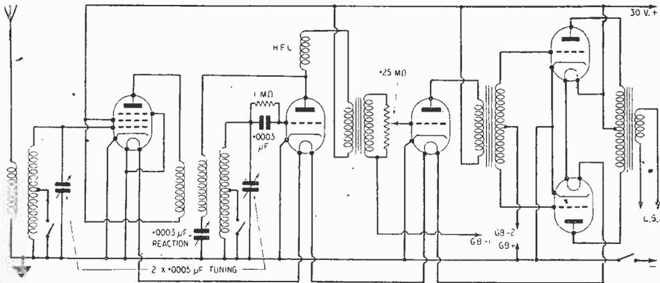
Fig. 1.—A circuit for a receiver for 30-volt operation. -
