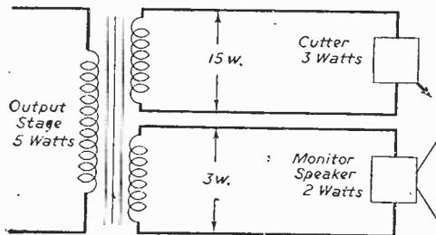
Fig. 3 (b).—Recording cutter and monitor are fed from individual windings, each taking a fixed percentage of output power (see text).
