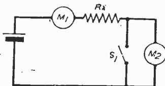
Circuit arrangement for measuring meter resistance.
