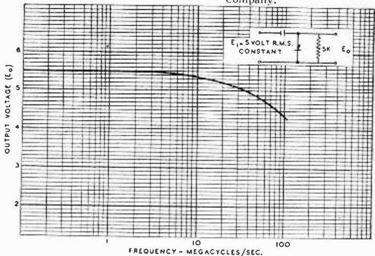
Fig. 3.—Typical frequency response characteristics of the rectifier.
