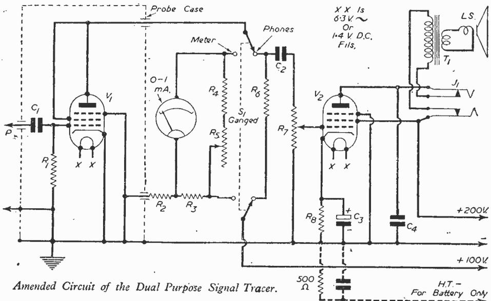
Amended Circuit of the Dual Purpose Signal Tracer.
