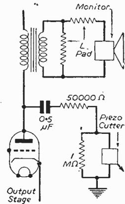
Fig. 6.—For piezo recorder. Transformer secondary matches monitor speaker; L pad removed for playback.
