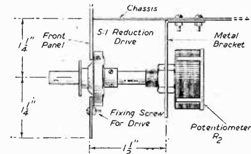
Fig. 9.—The above illustration shows method of mounting and dimensions for the slow-motion reaction control drive.
