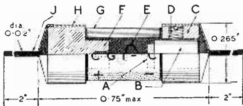
Fig. 1.—Half-section of germanium crystal rectifier, type CG.
