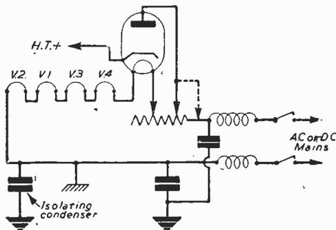
Fig. 4.—A more detailed circuit for A.C. or D.C. mains supplies showing the inclusion of H.F. filtering arrangements.
