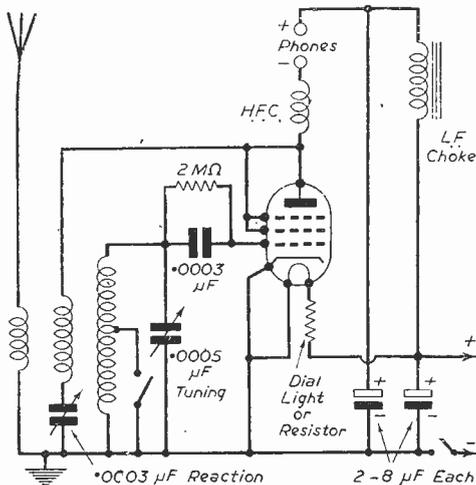
Fig. 3.—A 1-valve circuit showing position of H.T. smoothing and voltage-dropping resistor.
