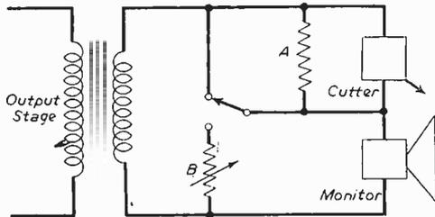
Fig. 5.—Record/playback circuit. With 15 ohm cutter, secondary and speaker, A is 10-15 ohms and maximum value of B is 25-30 ohms.
