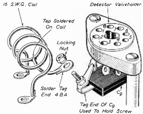
Fig. 5.—Details of the coil-mounting for the detector stage, showing the soldered cathode tap and method of connecting the tap direct to the valveholder.
