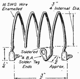
Fig. 10.—An example of the 4-turn detector coil and full data for all coils required to cover from 27 to 90 Mc/s.
