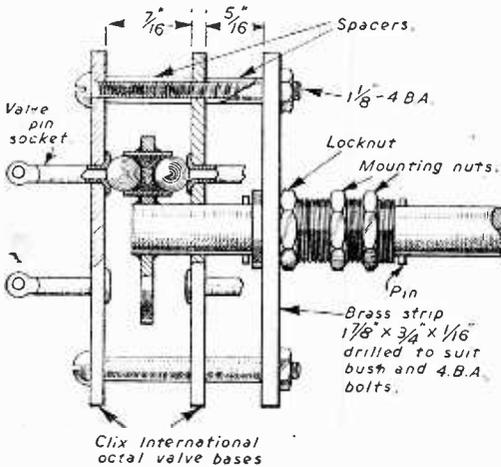
Main details of a rotary switch.
