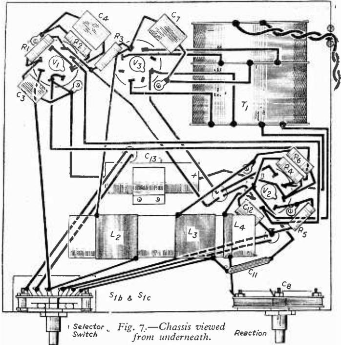
Fig. 7.—Chassis viewed from underneath.
