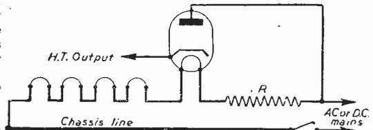
Fig. 3.—The above diagram shows the basic voltage, L.T. and H.T., supply arrangement for A.C. or D.C. mains supplies.
