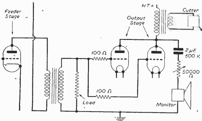
Fig. 4.—Monitor is connected to primary of output stage via blocking condenser and high resistance that serves as volume control.
