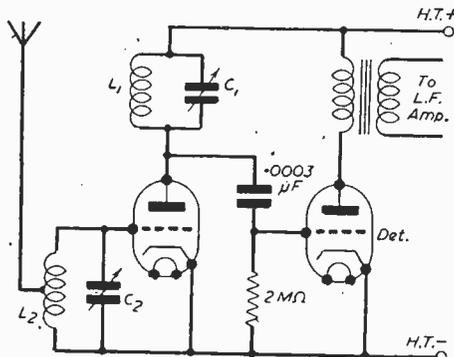
Fig. 3.—As an experiment, it is instructive to try an H.F. stage consisting of a triode with anode and grid tuned-circuits. It provides an object lesson in "H.F. instability!"
