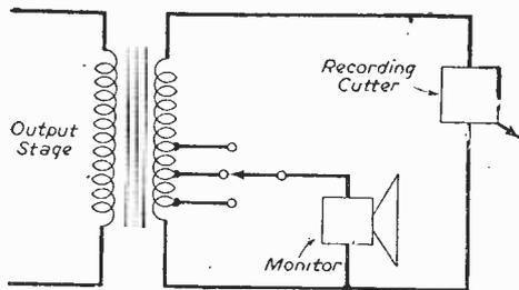
Fig. 3 (a).—Monitor speaker is fed from tapings on the secondary of output transformer.
