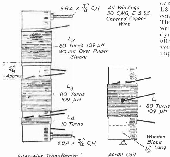
Fig. 2.—Details of the home-made coils.
