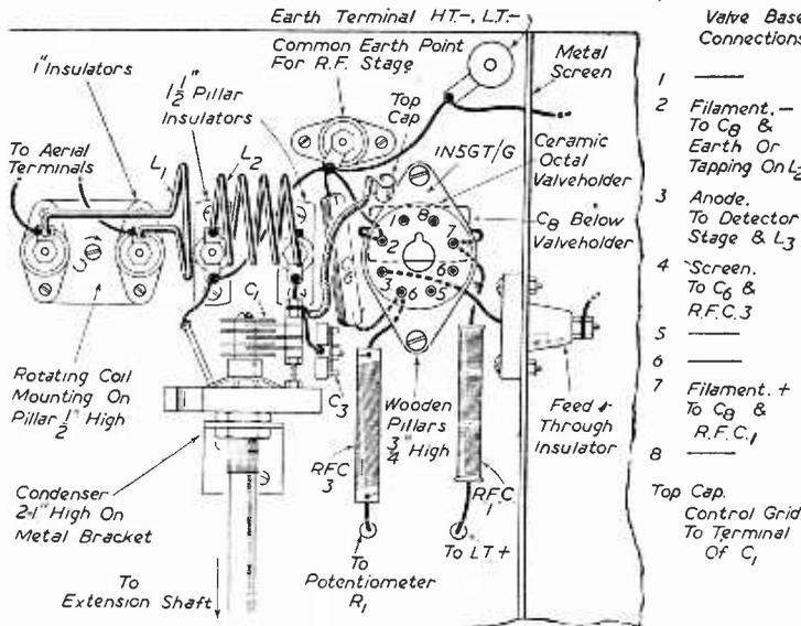
Note:—When R.F. Stage Is Regenerative, Pin No 2 On Valve Goes To The Tapping On L<sub>2</sub> And Not To Earth. Valve Pins Viewed From Top.
