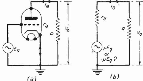
Fig. 2.—By "forgetting the H.T.," we get these "abstractions"—pure A.C. circuits—of the actual valve circuit 1a. But they fail completely to represent the voltage conditions of Fig. 1, since the relative "signs" of  $V$  and  $V_o$  depend upon the fixed D.C. potential of the + H.T. line. There is nothing remotely resembling the true conditions in purely "A.C. equivalents."
