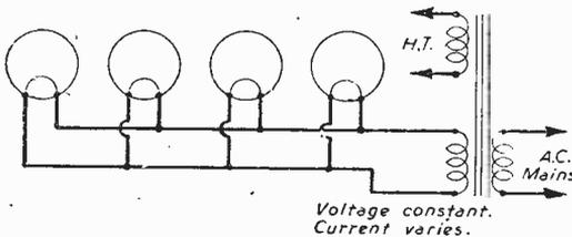
Fig. 1.—This is the normal A.C. heater-fed arrangement.
