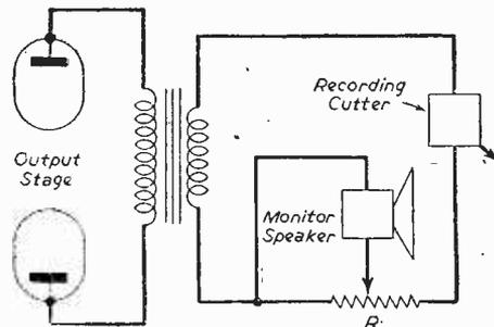
Fig. 2.— $R$  is varied to give comfortable monitor volume. For 15 ohm cutter and 15 ohm secondary,  $R$  is 5 ohms, with 3 ohm monitor speaker.
