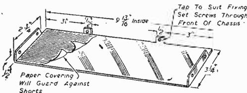
Fig. 11.—Note the use of a paper covering to avoid the risk of short circuits.
