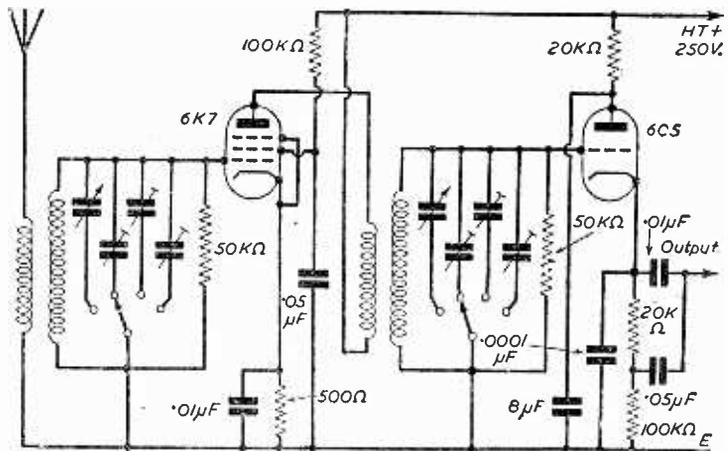
Fig. 5.—Extended-response tuner, with Kunde cathode-follower output. Coils and trimmers are as for Fig. 4.
