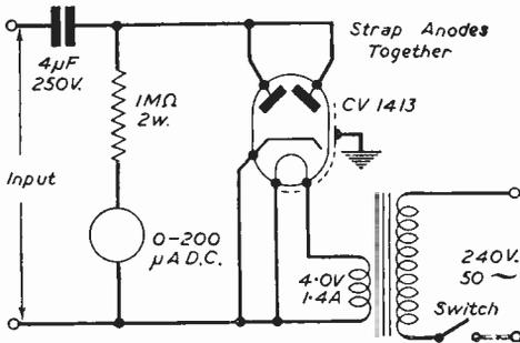
Fig. 1.—Circuit of the peak valve voltmeter.
