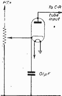
Fig. 2.—A noise-suppressor for incorporation across the input to the picture tube.
