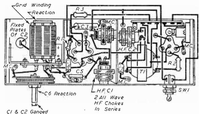
ment, but there is ample space available for most makes of the small type component. The chassis depth of 2 in. of course limits the size one way, but if the size of the transformer used prevents the inclusion of H.F. choke 2, this latter might be substituted by a  $\frac{1}{2}$ -watt resistance of about 10,000 ohms without too much loss of reaction smoothness. Note the grid stopper resistance, R.2.
