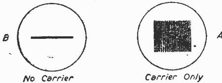
Fig. 10.—Typical oscillograms, showing carrier waveform.
