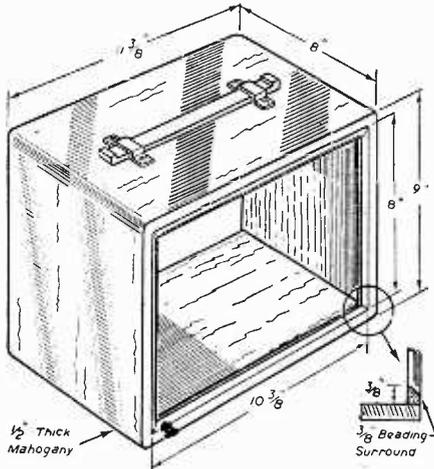
Fig. 10.—Dimensions of the containing case.
