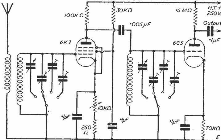
Fig. 4.—General purpose tuner, using plate rectification. Coils may be Wearite PHF2 or similar. Trimmers and ganged switches permit pre-setting of a number of tunings.
