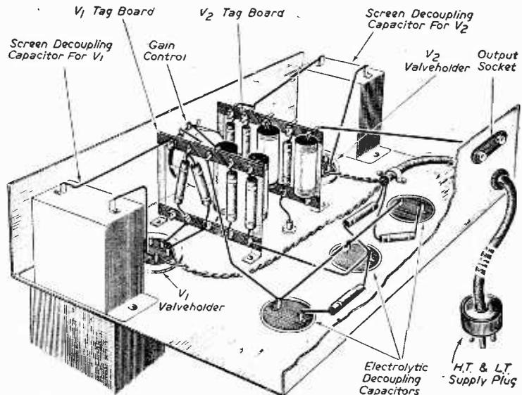
Fig. 4.—Underneath view of the suggested layout.
