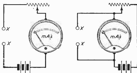
Fig. 1.—(Left) Basic series-connected ohmmeter, and Fig. 2 (right), Basic shunt-connected ohmmeter.
