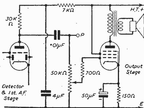
Fig. 2.—Last two stages of commercial receiver. Taking the output between point P and Earth provides an AF signal of 3 to 5 volts. See Fig. 3 for method of coupling.
