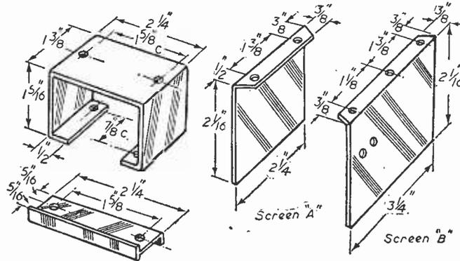
Fig. 6.—Details of the speaker platform and sub-panel screens.
