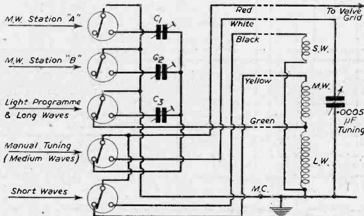
Fig. 2.—Theoretical circuit with coils and tuning condenser.
