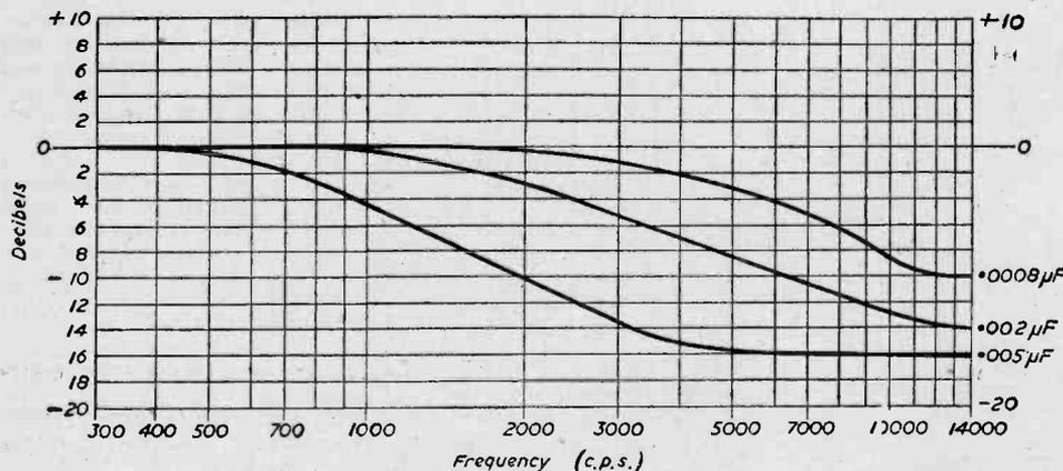
Fig. 3.—The top-cut response curve.
