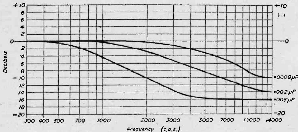
Fig. 3.—The top-cut response curve.
