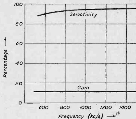
Fig. 7.—Variation of voltage gain and selectivity factors for R.F. transformer with high inductance primary winding.
