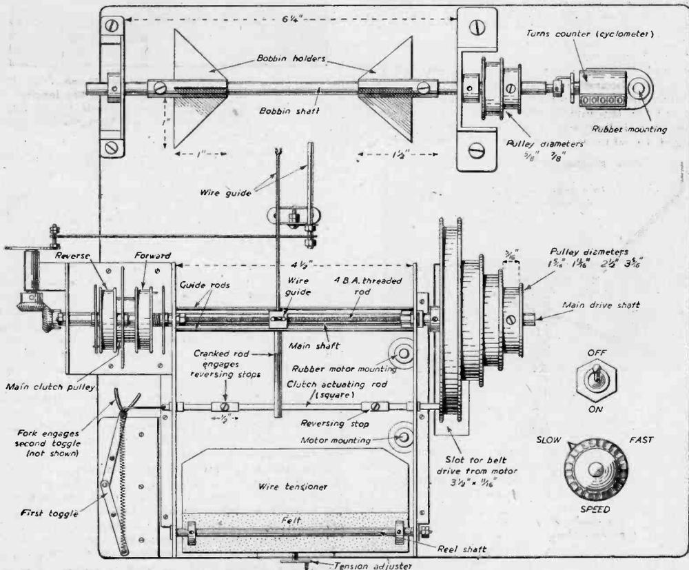
Fig. 1.—A plan of the machine with all parts identified.
