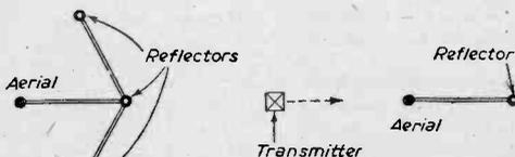
Fig. 3.—(Left) Multiple reflector for bad reception areas, and Fig 4 (right) theoretical relationship between aerial, transmitter and reflector.
