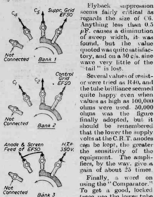
Fig. 4.—Details of Time-box frequency switch and cut-off circuit.
