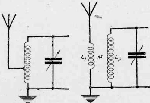
Fig. 2.—Circuit of a tapped-coil aerial coupling. Fig. 5.— Mutual-inductance aerial coupling circuit.
