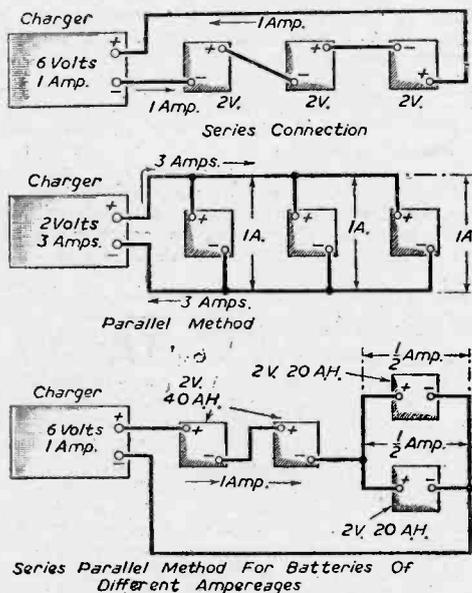
Fig. 7.—Various methods of connecting batteries.
