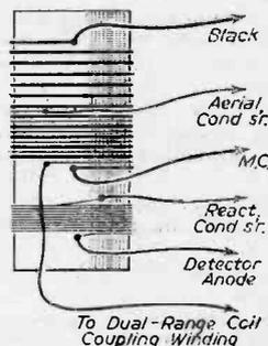
Fig. 5.—Details of a suitable short-wave coil.
