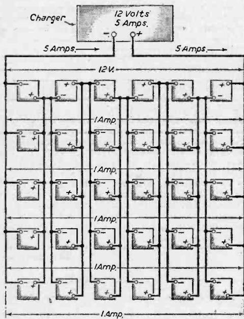
Fig. 9.—Another method of connecting thirty two-volt cells.
