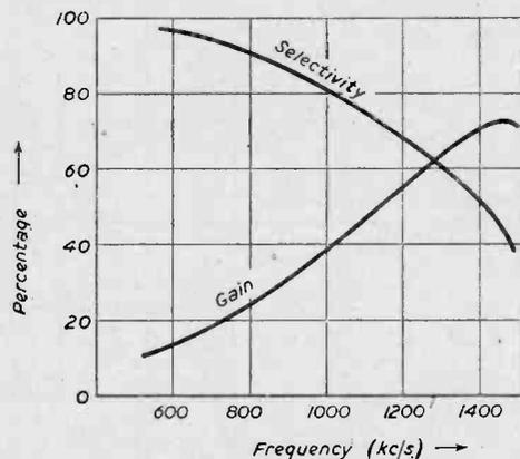
Fig. 6.—Variation of voltage gain and selectivity factors for R.F. transformer with low inductance primary winding.
