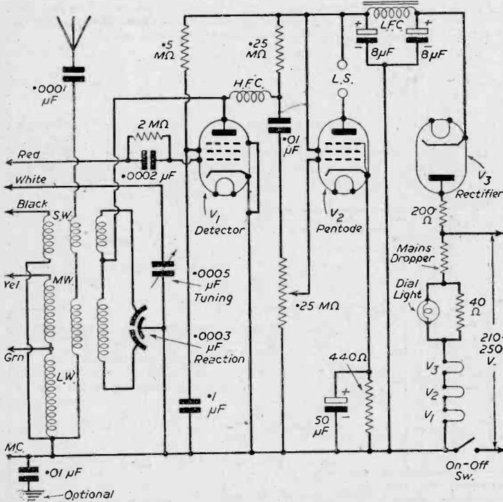
Fig. 4.—A complete 2-valve mains circuit.
