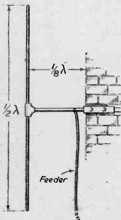
Fig. 1.—A standard dipole showing main details.
