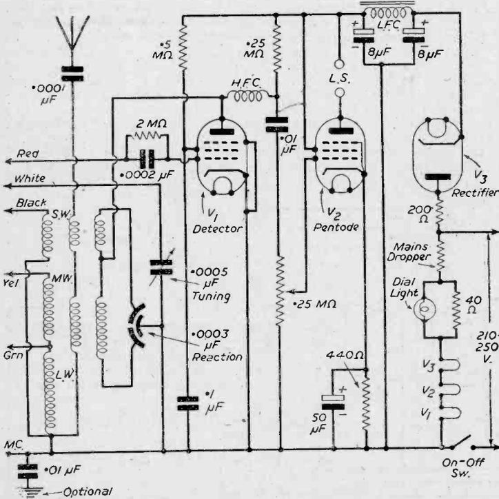
Fig. 4.—A complete 2-valve mains circuit.
