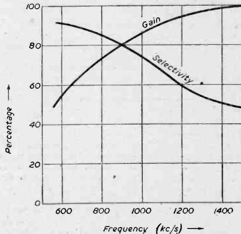
Fig. 3.—Variation of gain and selectivity with frequency for a tapped-coil aerial coupling.
