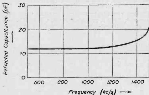
Fig. 4.—Variation of reflected capacitance with frequency for tapped-coil aerial coupling.
