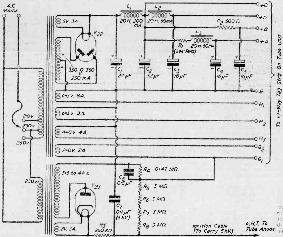
Fig. 1.—Theoretical circuit of the power pack, with terminal references.
