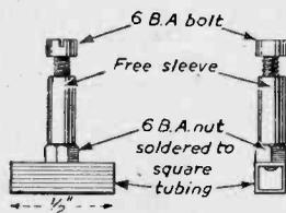
Fig. 3.—Details of construction of the reversing stops.
