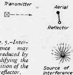
Fig. 5.—Interference may be reduced by modifying the position of the reflector.
