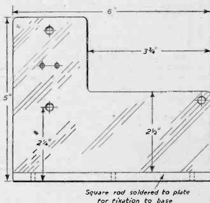
Fig. 2.—Shape and size of the sideplates. Two are needed.
