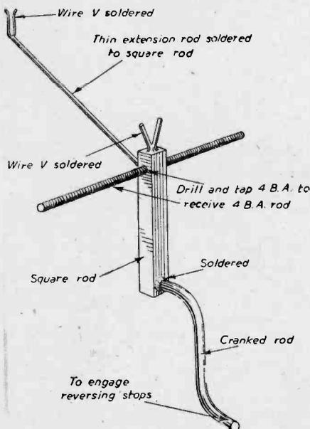
Fig. 4.—Make-up details of the wire guide.
