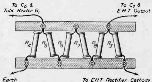
Fig. 3.—How to arrange the EHT bleeder to provide a long leakage path.
