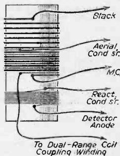
Fig. 5.—Details of a suitable short-wave coil.
