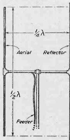
Fig. 2.—A dipole with reflector. Spacing may be reduced to one-eighth wavelength.
