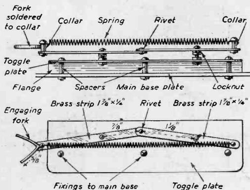
Fig. 5.—The first toggle seen in plan and elevation.
