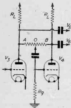
Fig. 2.—Circuit of the "floating" paraphase inverter used in this amplifier.
