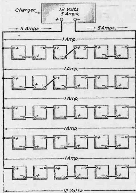
Fig. 8.—One method of connecting thirty two-volt cells.
