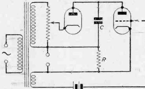
Fig. 2.—A diode acting as a discharge source.
