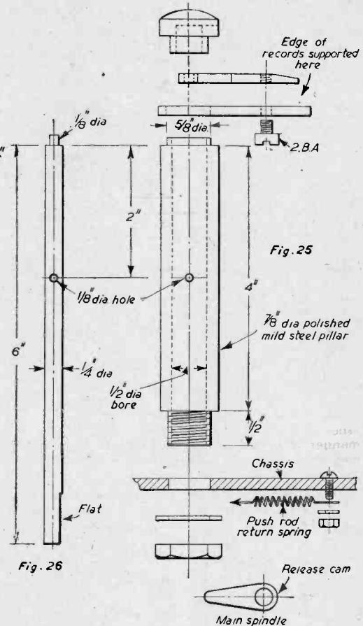
Figs. 25 and 26.—Record supporting pillar assembly.
