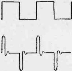
Fig. 15.—A rectangular pulse and its form after application to a circuit of this type shown in Fig. 14(a).
