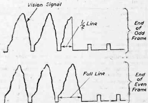
The characteristic of the signal and synchronising pulses.—Not to scale.
