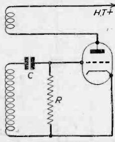
Fig. 3(a).—Simple reaction circuit.
