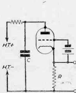
Fig. 1.—Simple thyatron circuit.
