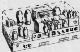
2 RF Stages. Tuneable Oscillator. 4 I.F.s. staggered from 9.5—13.5 mcs. Det. and output stages. Extra circuits that can be modified for Time bases. A total of 17 valves.
