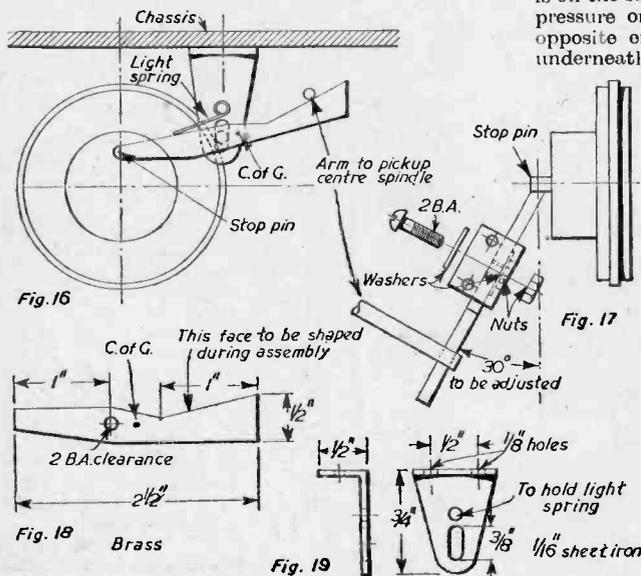
Figs. 16 to 19.—Details of the trip lever and bracket.
