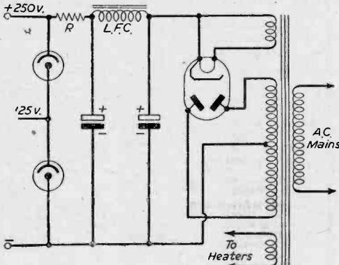
Fig. 4.—Two stabilised outputs are given by this arrangement.
