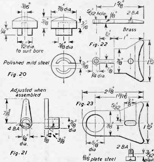
Figs. 20 to 23.—The record release components.
