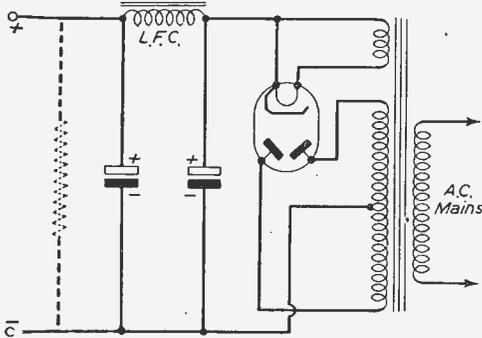
Fig. 1.—Standard power pack circuit.
