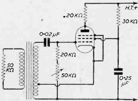
Fig. 4.—Simple Hartley oscillator circuit.
