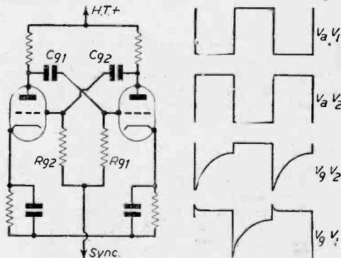
Fig. 5(a) and (b).—Multivibrator circuit and representative waveforms.
