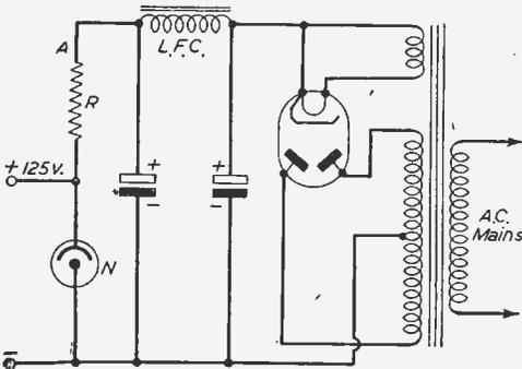
Fig. 2.—A stabilised tapping point.
