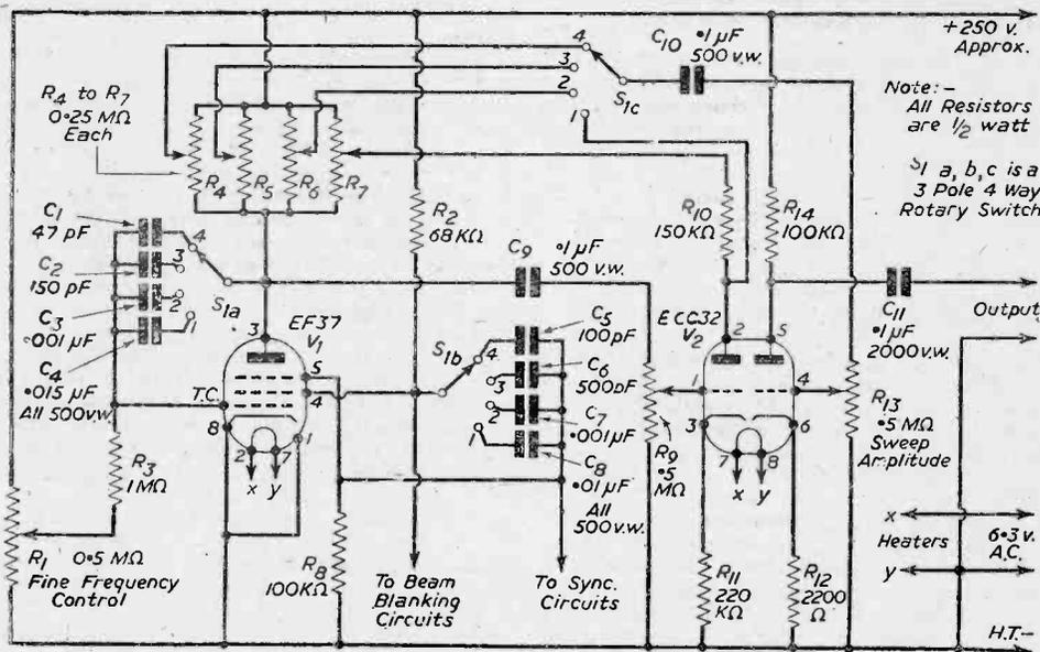
Fig. 2.—Circuit of the Improved Miller Timebase
