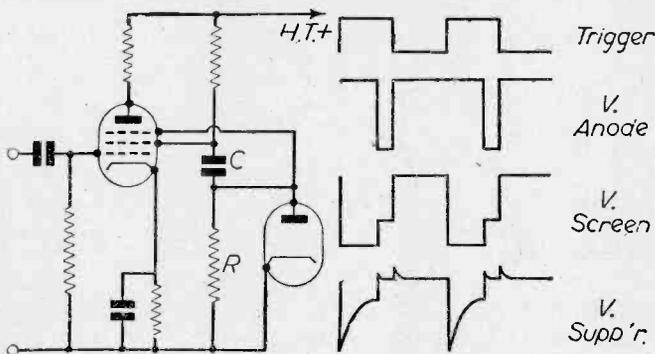
Figs. 7(c) and (d).—An alternative circuit of a triggered transitron and its waveforms.
