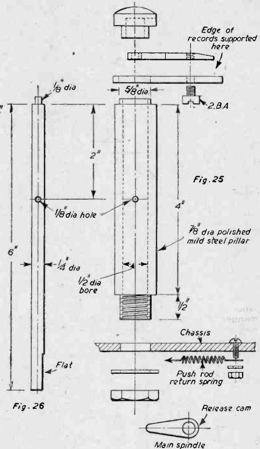
Figs. 25 and 26.—Record supporting pillar assembly.
