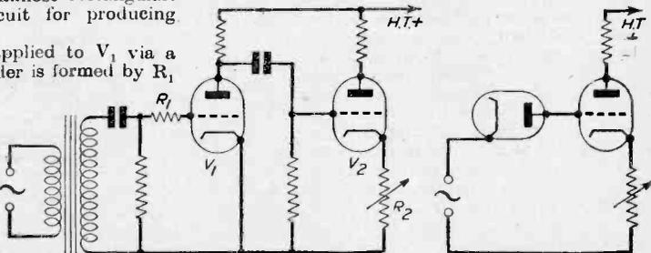
Fig. 9.—Circuit for producing rectangular pulses.
