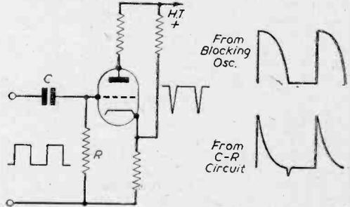
Figs. 12 and 13.—Effects of biasing, and a shaping circuit.
