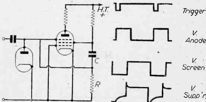
Fig. 7(a) and (b).—Triggered transistor and its waveforms, HD 3110
