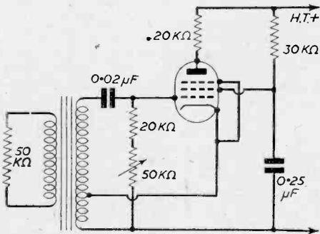
Fig. 4.—Simple Hartley oscillator circuit.
