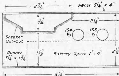
Fig. 2.—Chassis cutting and drilling details.
