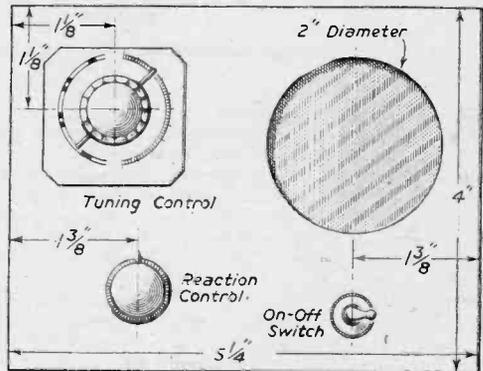
Fig. 3.—Panel lay-out.
