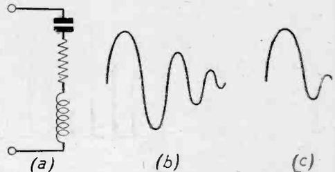
Fig. 14.—Circuit consisting of L, C and R, and the resultant damped output.
