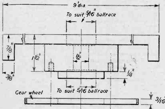
Fig. 24.—Turntable details (aluminium).
