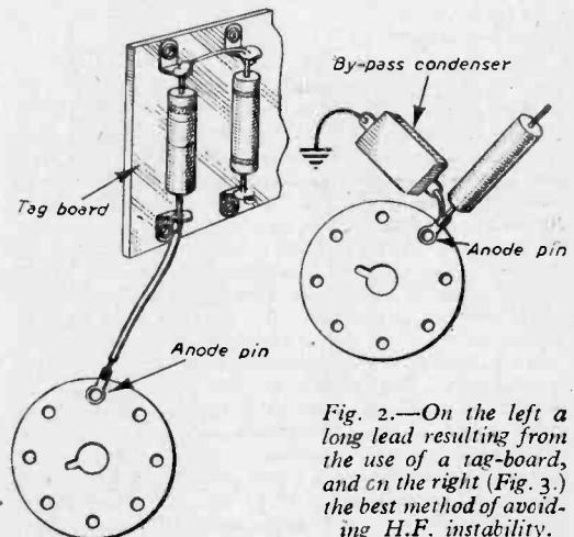
Fig. 2.—On the left a long lead resulting from the use of a tag-board, and on the right (Fig. 3.) the best method of avoiding H.F. instability.
