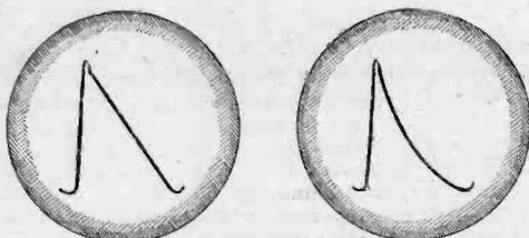
Fig. 1—(a). The ideal Miller Timebase voltage sweep and (b) (left) non-linearity at low frequencies.
