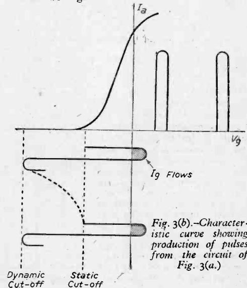
Fig. 3(b).—Characteristic curve showing production of pulses from the circuit of Fig. 3(a.)
