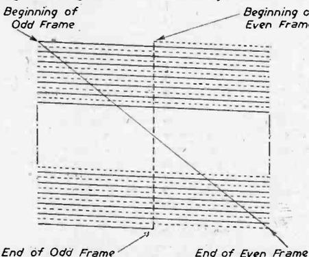
How a normal raster is built up by the interlacing method.
