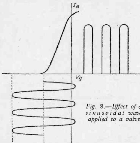
Fig. 8.—Effect of a sinusoidal wave applied to a valve.
