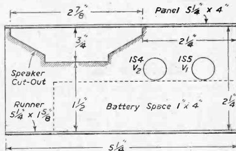
Fig. 2.—Chassis cutting and drilling details.
