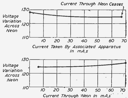
Fig. 3 (a) and (b).—Graphs showing effect of stabilisation.
