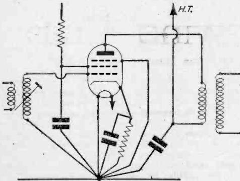
Fig. 1.—Circuit diagram indicating a common earthing point in an H.F. stage.
