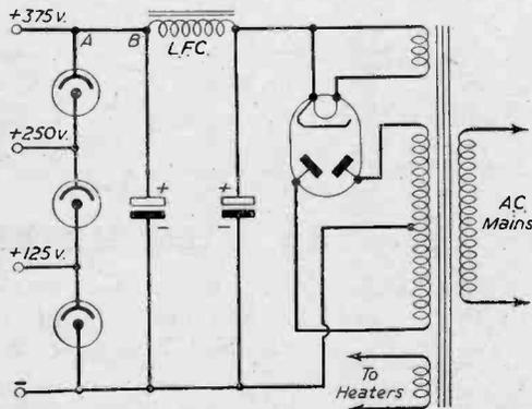
Fig. 5.—How three stabilised outputs may be obtained.
