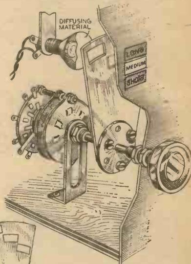
A novel panel lighting device, using only one bulb.
