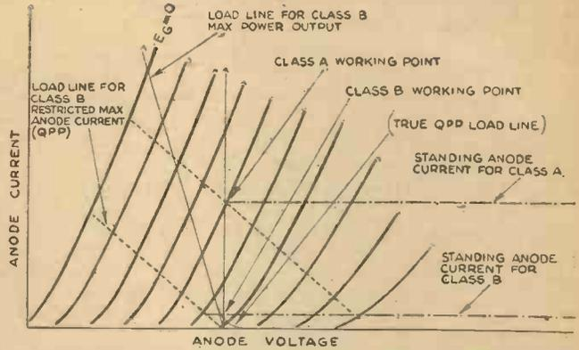
Fig. 5.—Comparison between Class A and two alternative applications of Class B, the one alternative for maximum economy in average anode current ("Q.P.P."), and the other alternative for maximum power output (low impedance loading "Class AB1")
