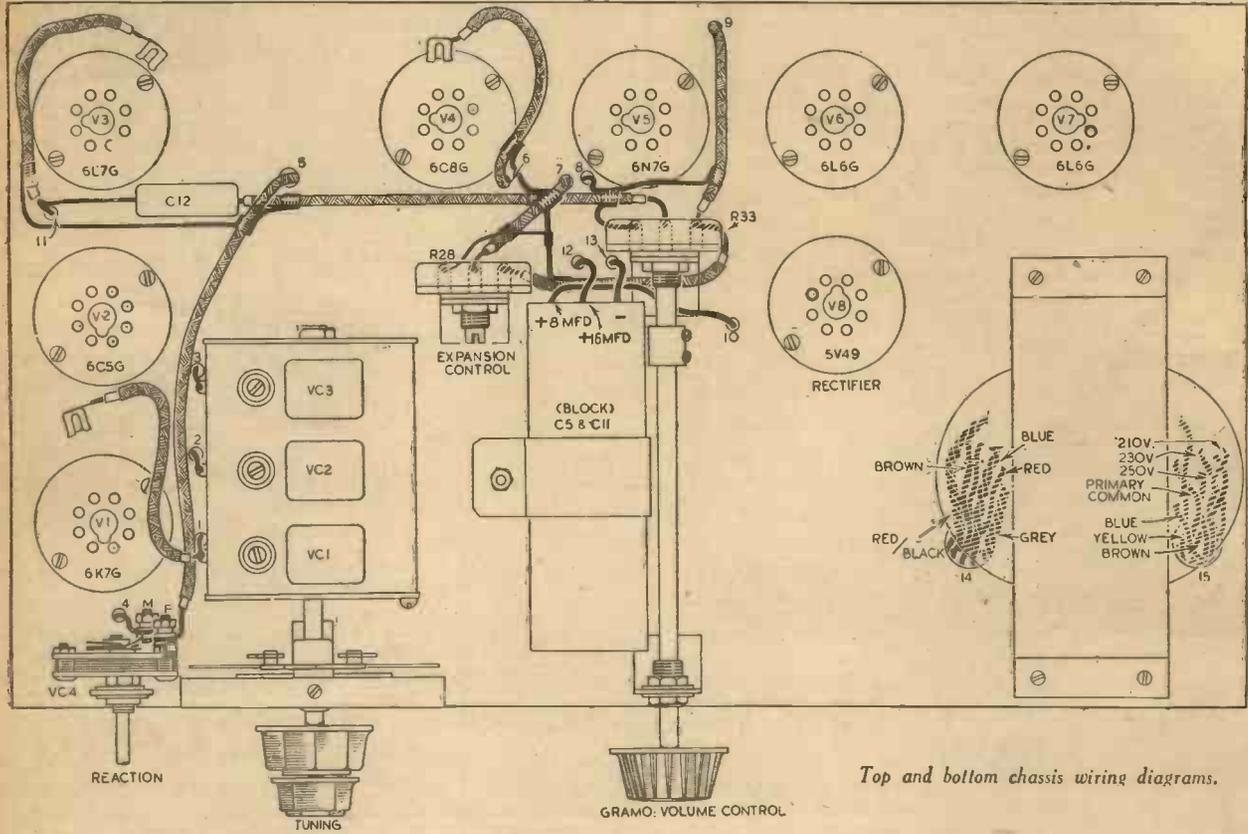
Top and bottom chassis wiring diagrams.
