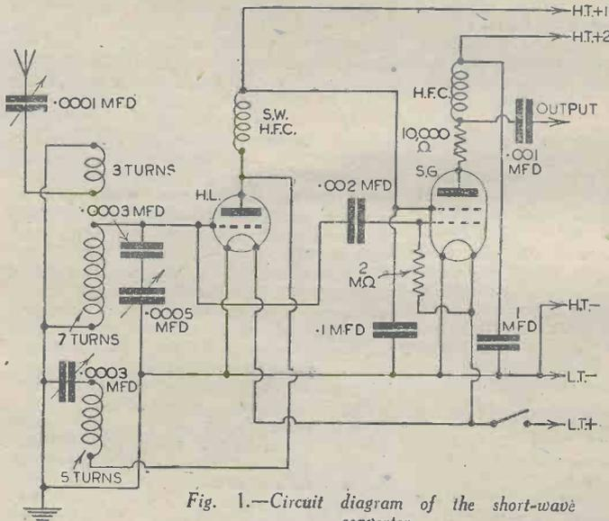
Fig. 1.—Circuit diagram of the short-wave converter.
