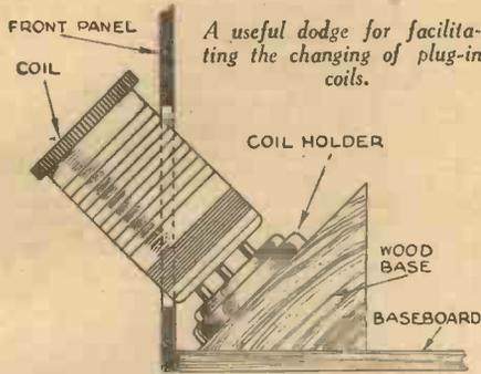
in the front or side of the set and to screw the coil holder on to a wooden mount in the position shown. The top of the coil then protrudes at the front or side of the receiver, whichever arrangement suits best. This allows the coil to be changed without difficulty, but needless to say it applies only to plug-in coils.—A. COOK (Ayr).
