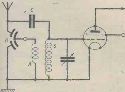
Circuit diagram incorporating a differential condenser for controlling volume.
