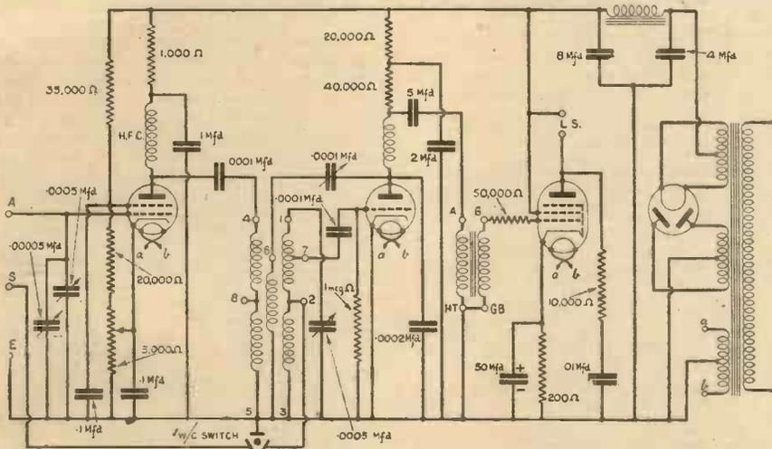
Fig. 1.—A suitable theoretical circuit for the transportable. Other types of coil could be used.
