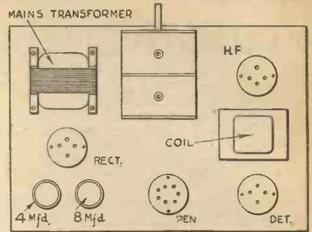
Fig. 2.—A suggested layout, showing how the mains equipment is located to one side of the chassis away from the coil.
