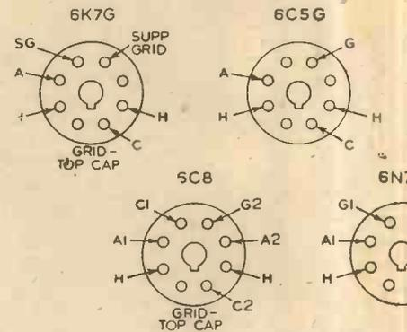
Fig. 2.—Pin connections for the valves. Note
