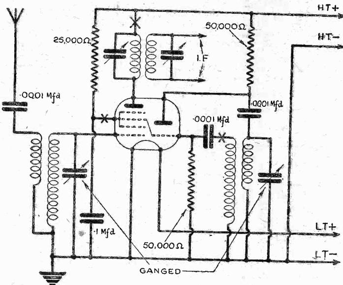
Fig. 3.—In the case of the triode-hexode frequency-changer one grid is common to both portions of the valve. This type of frequency-changer circuit is coming into increasing use for all-wave and short-wave receivers.
