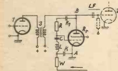
Fig. 1.—Basic circuit of the electrical auto-tone-control arrangement.
