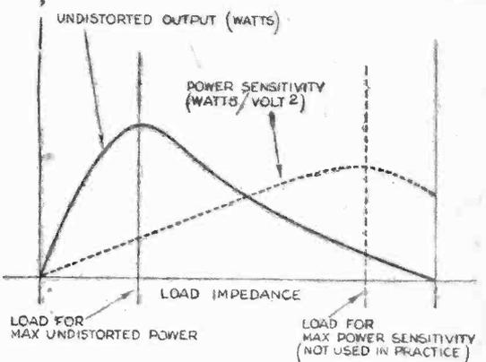
of the input signal by the complete output stage. To be comprehensive, this must also take into account the characteristic of the loudspeaker, which may vary over a very wide range depending on the nature of its design.
