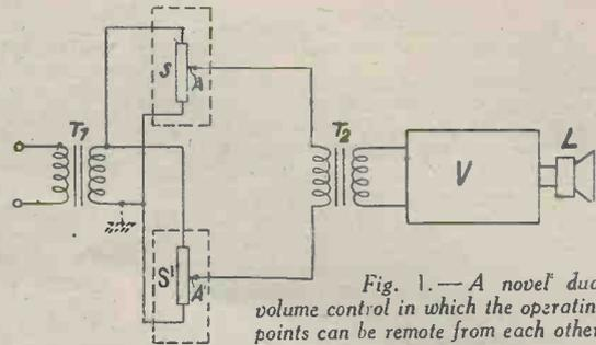
Fig. 1.—A novel dual volume control in which the operating points can be remote from each other.
