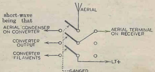
Fig. 2.—Diagram of connections for a three-pole anti-capacity switch.
