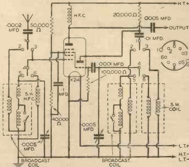
The basic circuit diagram and, inset, connections to one side of the S.212 rotary switch. Connections are duplicated on the other side.
