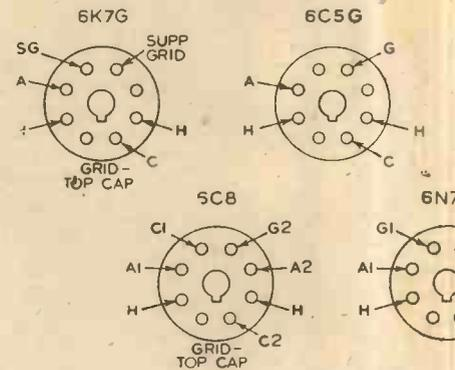
Fig. 2.—Pin connections for the valves. Note
