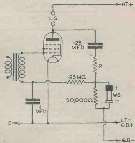
Fig. 2.—A "standard" H.T. economiser circuit incorporating a Westector. Suitable values for resistor R are given below.
