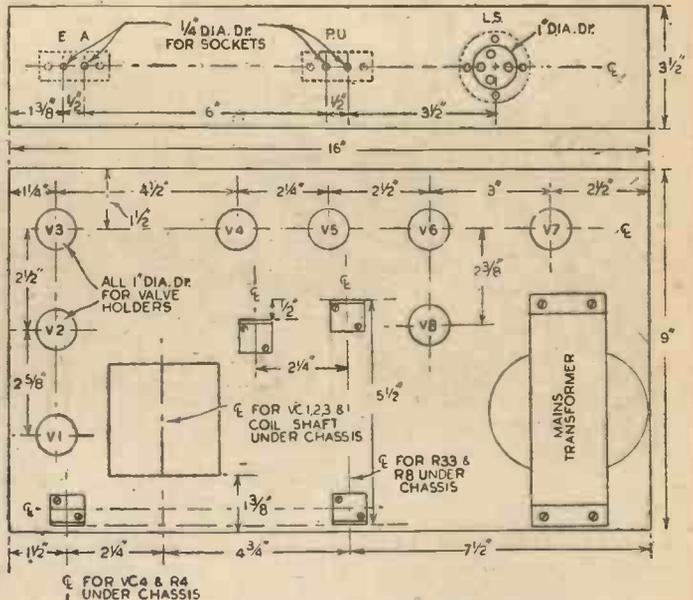
Fig. 4.—Chassis construction and drilling details.
