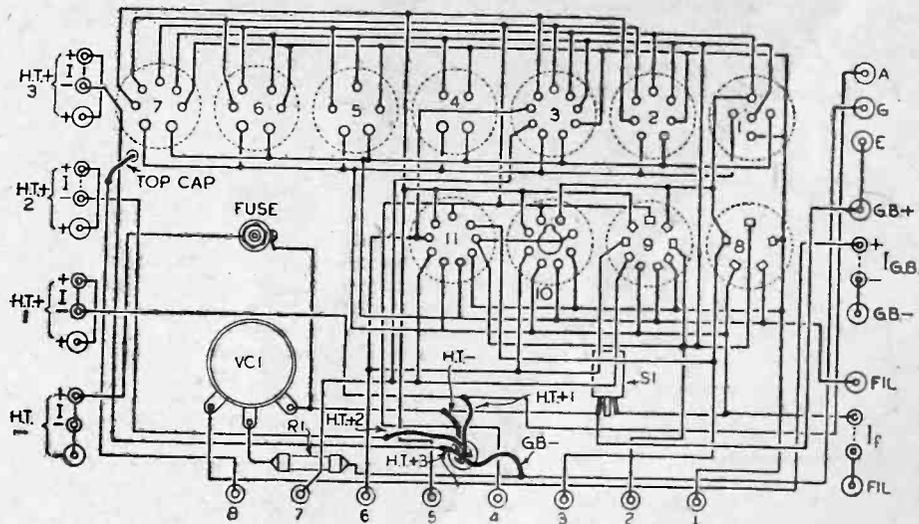
Fig. 2. Wiring diagram of the universal valve-tester.
