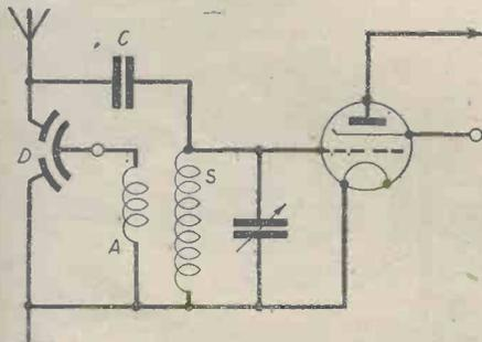
Circuit diagram incorporating a differential condenser for controlling volume.
