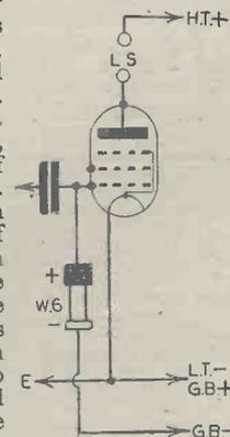
Fig. 3.—A simplified H.T. economiser arrangement suitable for use with an R.C.C. stage.
