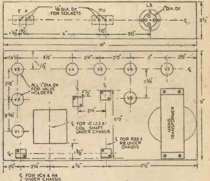
Fig. 4.—Chassis construction and drilling details.
