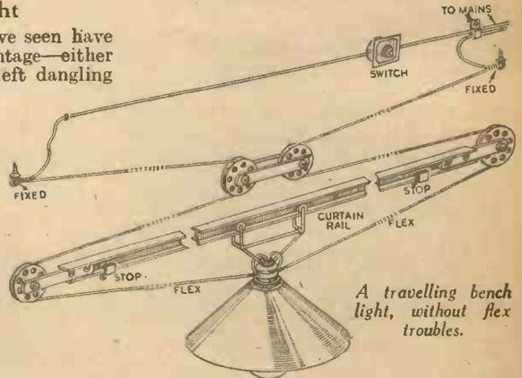
rail is obtainable at any sixpenny stores, as well as the pulley runners; the other items required are 1 1/2 in. grooved pulleys, and some 1/16 in. strip brass. The lamp is hung on to the pulley runners by means of a short length of fairly stiff wire formed into a triangular loop. Rail stops (optional, but recommended) are fitted at each end of the rail to prevent "overrunning" the ends. The ends of the flex wires are fixed to either wall, as indicated.—E. WILLIAMS (Llanely).
