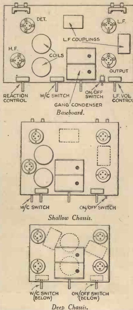
These plan diagrams show how a basic layout can be used for baseboard construction, or for chassis of different proportions.
