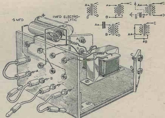
A plug and socket switching unit for transformers used for testing purposes.
