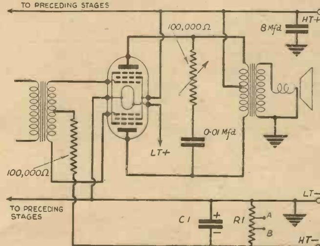
Fig. 6.—"Q.P.P." stage with "automatic" grid-bias. Bias is produced by the flow of H.T. current through the resistance  $R_1$  via the filament circuit. Various values of bias may be tapped from  $R_1$  for the preceding valves. The electrolytic condenser  $C_1$  must be at least 50 mfd. capacity.  $C_1$  smoothes out considerably the variation in current through  $R_1$  due to change in output volume level.
