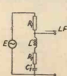
Fig. 6.—Illustrating the resonance short-circuit feature.
