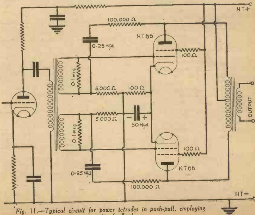
Fig. 11.—Typical circuit for power tetrodes in push-pull, employing negative feedback.
