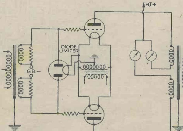
Fig. 5.—Signal voltage limiting circuit for use with power triodes in class AB1 push-pull, showing the diode.
