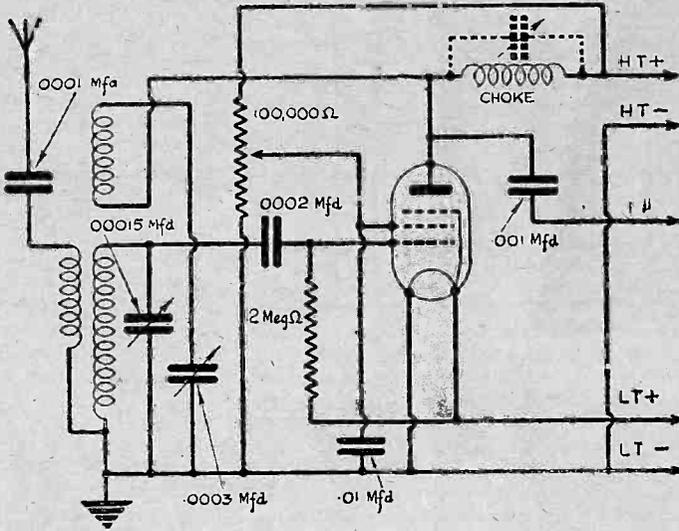
a short-wave converter, has an H.F. pentode or similar valve wired in a circuit similar to that of a single-valve regenerative receiver.
