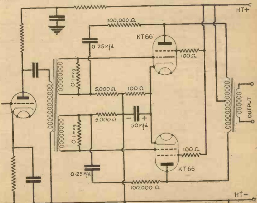
Fig. 11.—Typical circuit for power tetrodes in push-pull, employing negative feedback.
