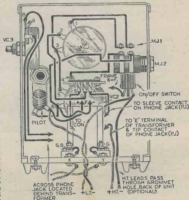
Fig. 4.—Layout of components and wiring diagram.
