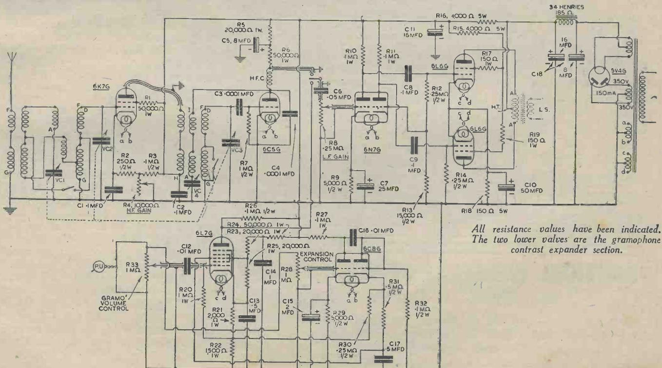
All resistance values have been indicated. The two lower valves are the gramophone contrast expander section.
