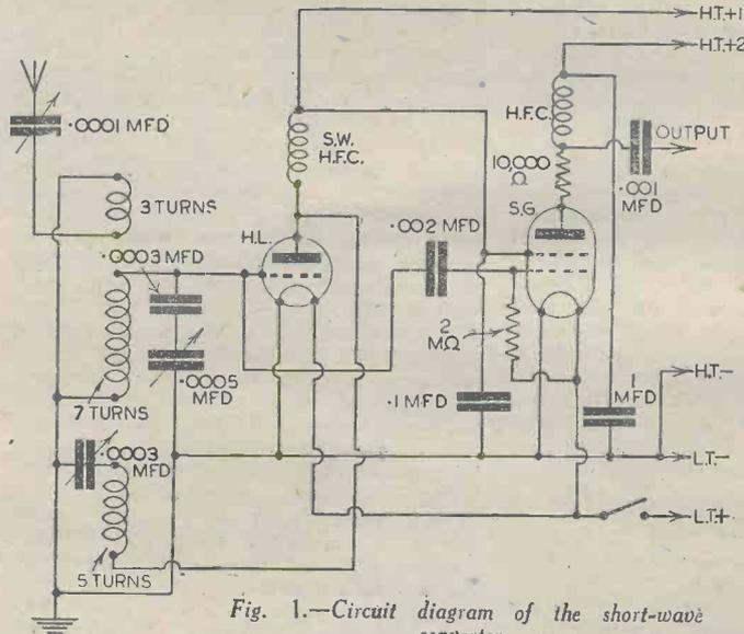
Fig. 1.—Circuit diagram of the short-wave converter.
