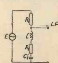
Fig. 6.—Illustrating the resonance short-circuit feature.
