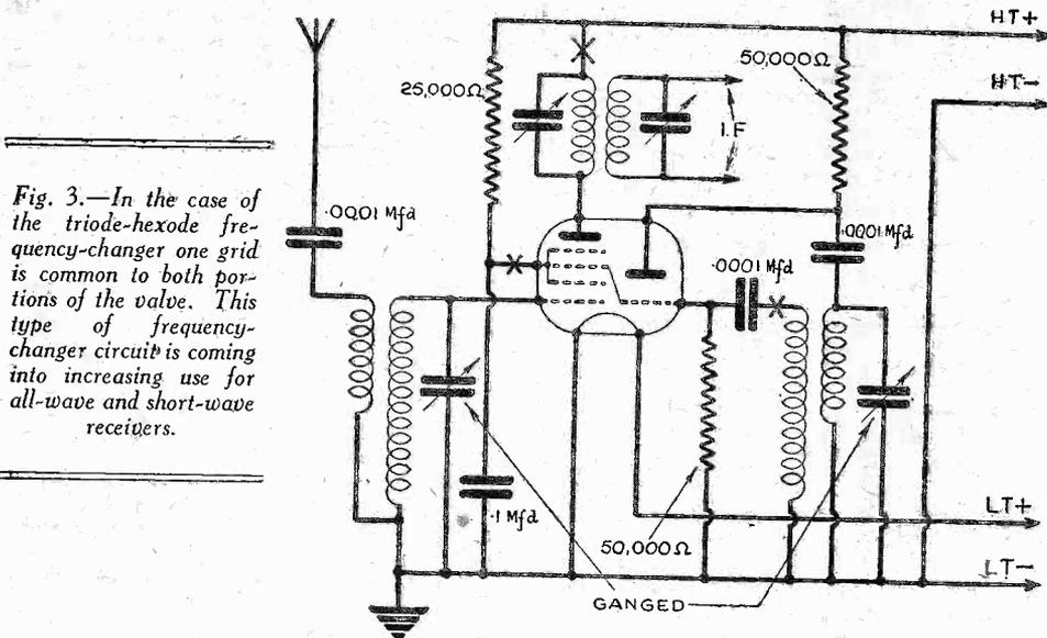
Fig. 3.—In the case of the triode-hexode frequency-changer one grid is common to both portions of the valve. This type of frequency-changer circuit is coming into increasing use for all-wave and short-wave receivers.
