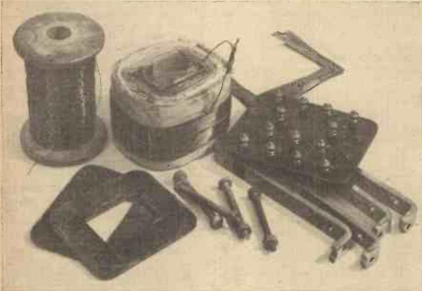
Parts of a commercial mains transformer which has been dismantled to show construction. Note insulation between layers of windings.
