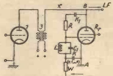
Fig. 5.—The use of a series resonance circuit.
