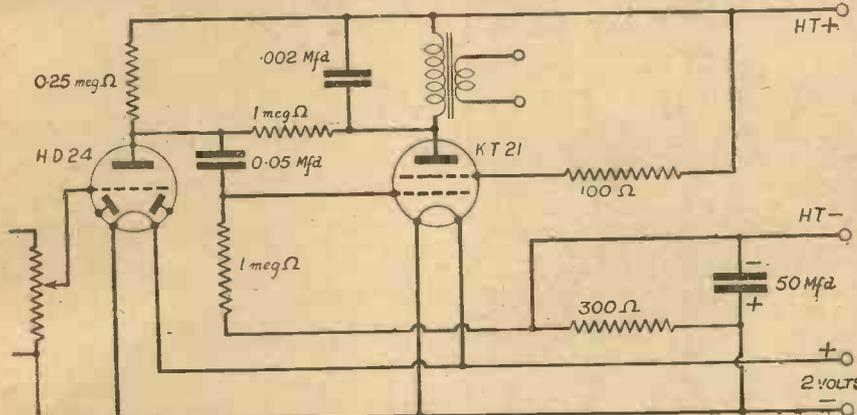
Fig. 10.—Typical circuit for a 2-volt battery power tetrode employing negative feedback.
