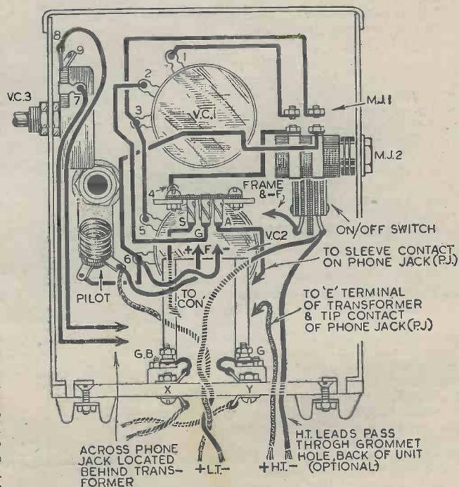
Fig. 4.—Layout of components and wiring diagram.
