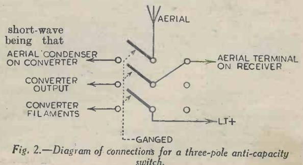
Fig. 2.—Diagram of connections for a three-pole anti-capacity switch.
