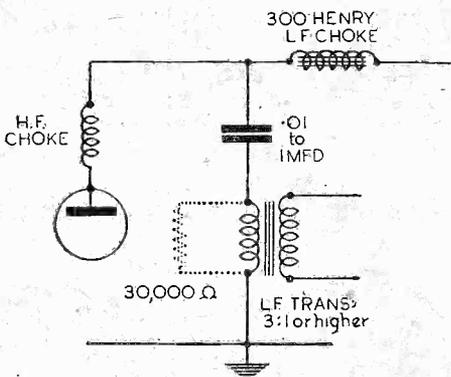
Fig. 2.—Anode circuit and L.F. coupling for high-impedance detector valves.
