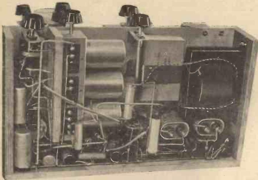
Fig. 1.—Underside, showing position of components and wiring. Note method of mounting the coil unit.
