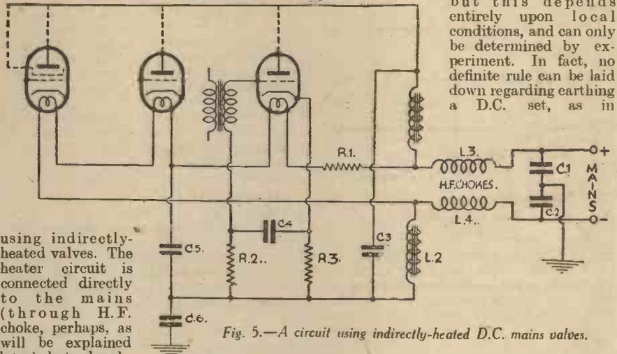
Fig. 5.—A circuit using indirectly-heated D.C. mains valves.
