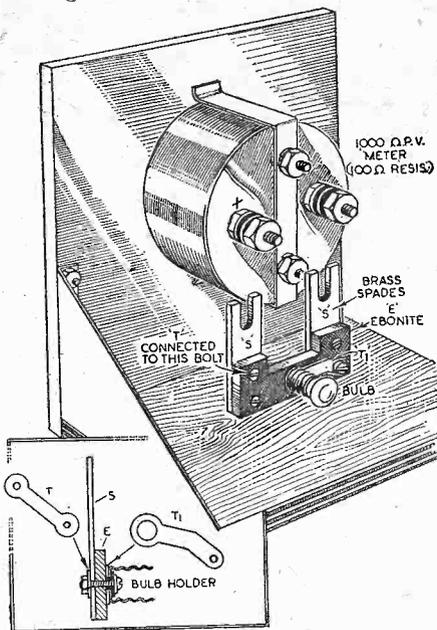
A method of using a torch bulb as a meter shunt.
