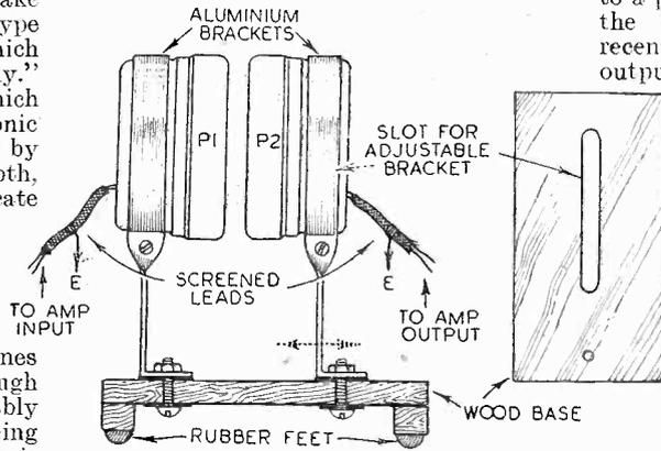
Fig. 1.—The first step in the development of the oscillator.
