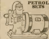
**PETROL ELECTRIC GENERATING SETS** for Lighting and Charging. Half h.p. DIRECT COUPLED. 150 watts D.C., 1,300 r.p.m., 2-stroke water-cooled 1-cyl. Engine, magneto ignition. On bedplate with 30 volts 5 amps. Dynamo. £12. 75 Larger size 1 kW. Petrol Electric Sets. 500 watts. 2-stroke water-cooled 1 h.p., 1 cyl. engine on bedplate direct-coupled to 50/70 volts 10 amps. D.C. Dynamo, magneto ignition, fuel and oil tank. £16.
