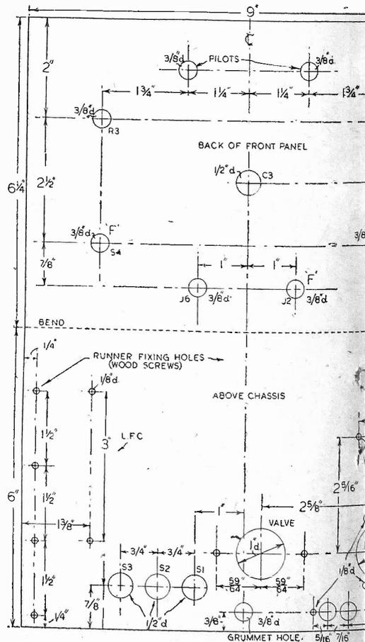
Fig. 4.—Drilling dimensions of the chassis
