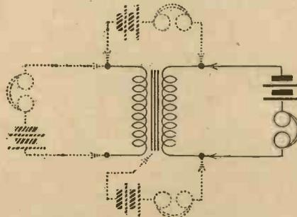
Method of testing a faulty transformer
