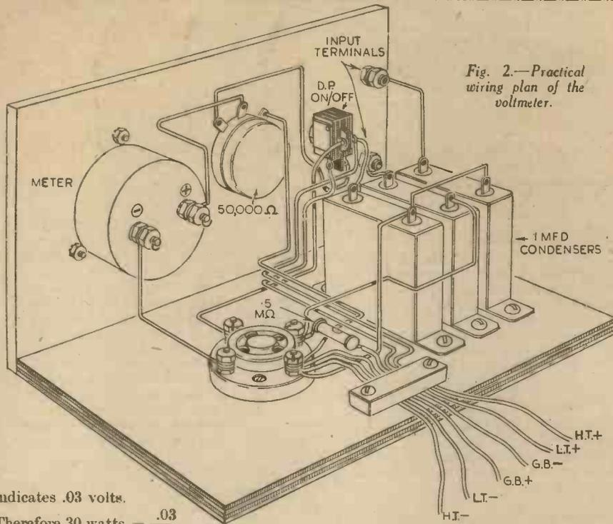
Fig. 2.—Practical wiring plan of the voltmeter.
