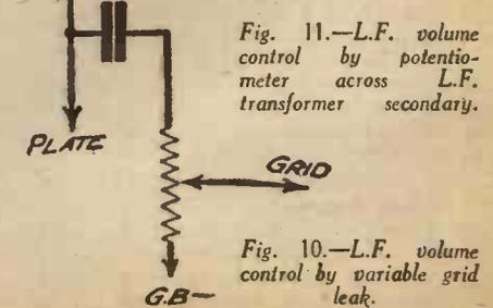
Fig. 10.—L.F. volume control by variable grid leak.
