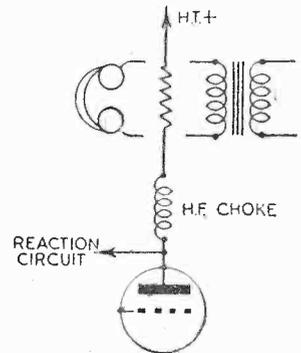
Fig. 2.—Typical anode circuit indicating the components which are found there. This explains the reasons for threshold howl.
