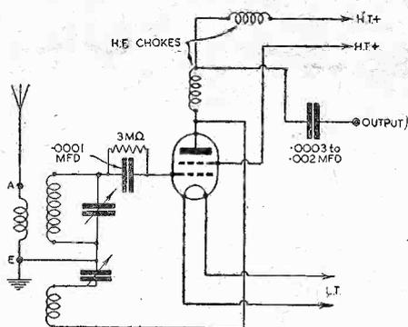
Fig. 2.—Similar arrangement to Fig 1, but using a pentode.
