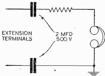
Fig. 1.—One method of 'phone isolation, with high impedance extension.
