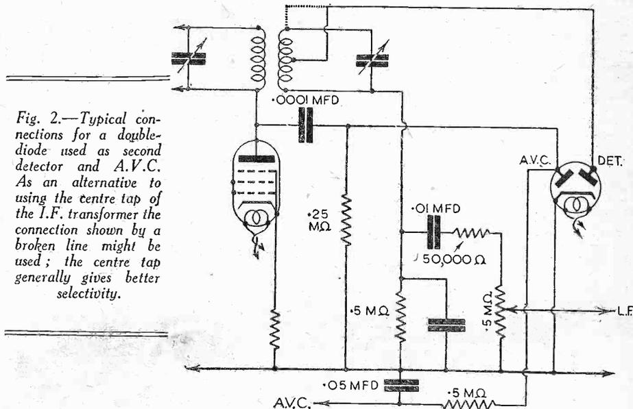
Fig. 2.—Typical connections for a double-diode used as second detector and A.V.C. As an alternative to using the centre tap of the I.F. transformer the connection shown by a broken line might be used; the centre tap generally gives better selectivity.
