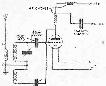
Fig. 1.—Simple reacting scheme using a triode.
