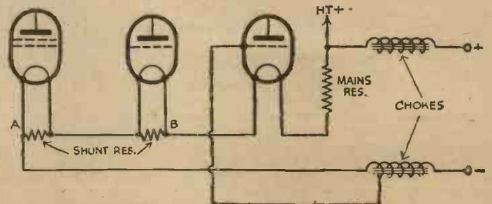
Fig. 3.—The filaments of D.C. valves are wired in series.
