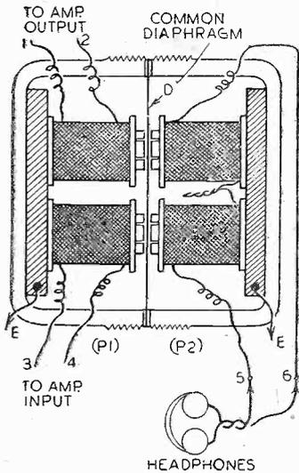
Fig. 3.—Two earpieces combined to provide a similar effect to Fig. 1.
