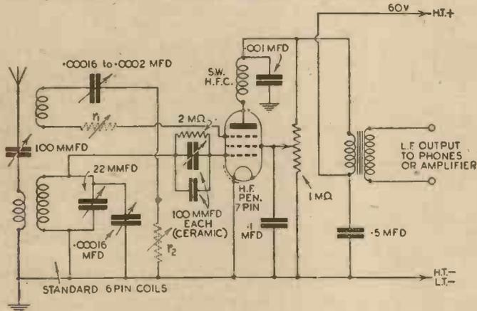
Fig. 1.—Circuit diagram showing in skeleton form the theory of the suppressor-grid system of reaction.
