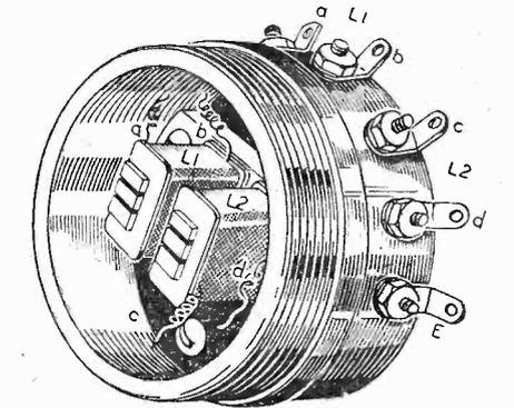
Fig. 2.—How the earpiece was split up and provided with terminals in a further stage of development.
