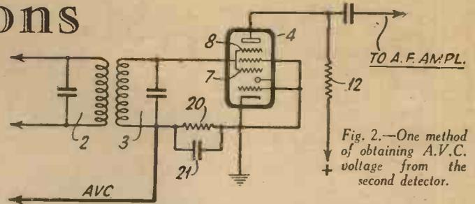
Fig. 2.—One method of obtaining A.V.C. voltage from the second detector.
