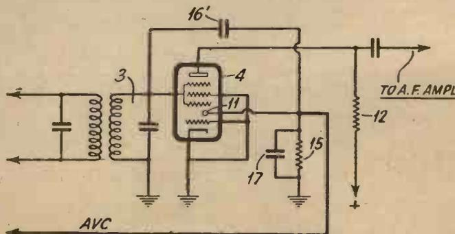
Fig. 3.—In this arrangement the I.F. currents are fed through condenser 16.
