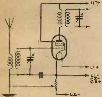
Fig. 4.—Theoretical circuit for battery variable-mu valves.
