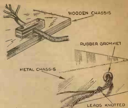
Fig. 2.—Methods of anchoring flex leads to prevent them from being pulled away from the chassis.
