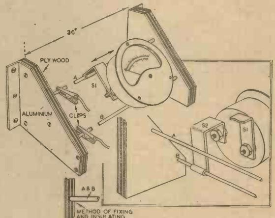
This sliding meter rack facilitates testing work.
