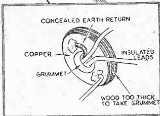
A useful wiring hint for combined wood and metal chassis.
