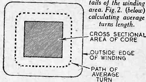
Fig. 1.—(Left) Details of the winding area. Fig. 2. (below) calculating average turns length.
