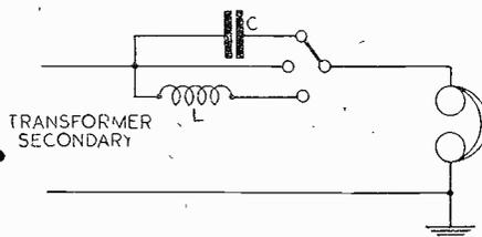
Fig. 4.—Simple type of tone control for use in conjunction with Fig. 2.
