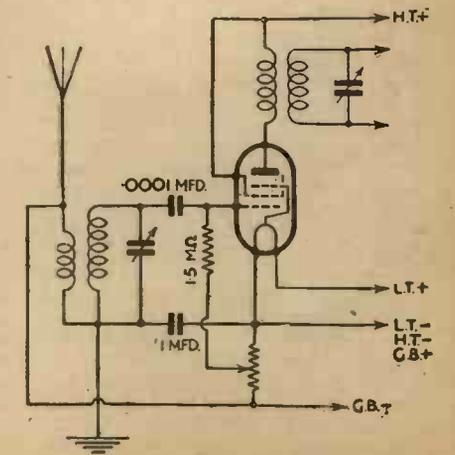
Fig. 6.—A still better form of volume control—combined variable-mu and aerial damping.
