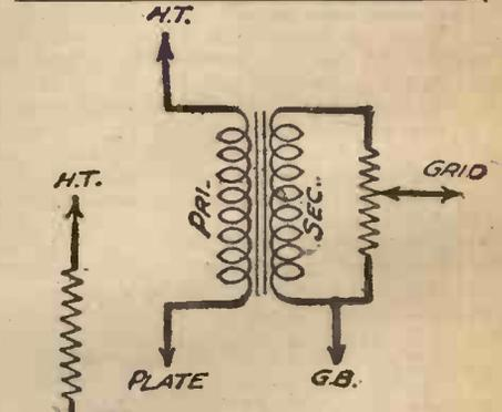
Fig. 11.—L.F. volume control by potentiometer across L.F. transformer secondary.
