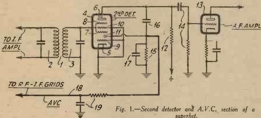
Fig. 1.—Second detector and A.V.C. section of a superhet.
