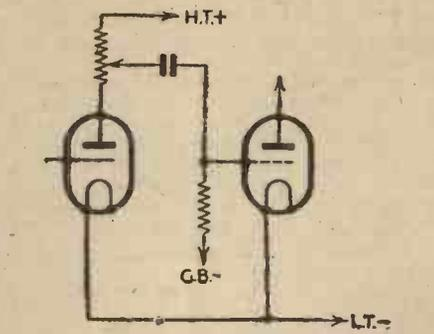
Fig. 9.—L.F. volume control by variable anode resistance.
