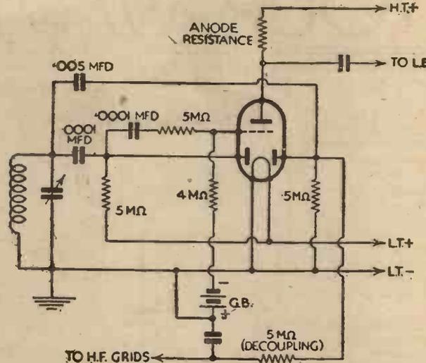
Fig. 7.—Simple A.V.C. for a battery set using double-diode triode.
