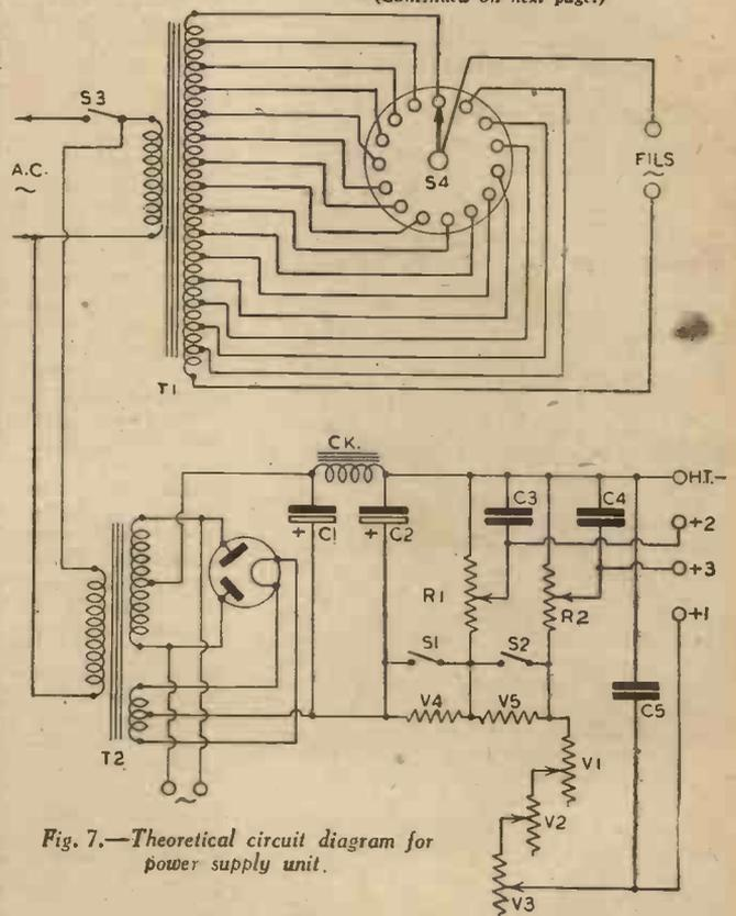
Fig. 7.—Theoretical circuit diagram for power supply unit.
