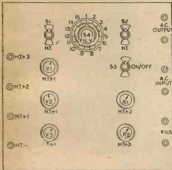
Fig. 6.—Panel layout for the power supply unit. The size of the panel can be made to suit requirements.
