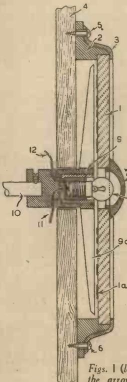
Figs. 1 (left) and 2 (right) show the arrangement of the edge-lighted dial.
