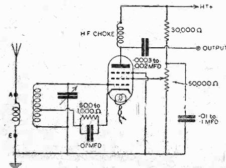
Fig. 3.—A mains circuit using resistance-controlled reaction.
