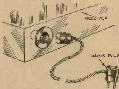
Fig. 3.—"Live" mains connectors should always be insulated. Connectors with open pins or sockets should be "dead" when removed.
