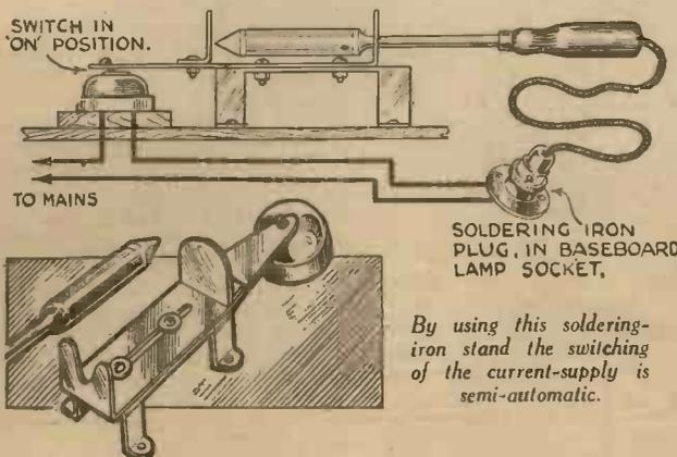
By using this soldering-iron stand the switching of the current-supply is semi-automatic.
