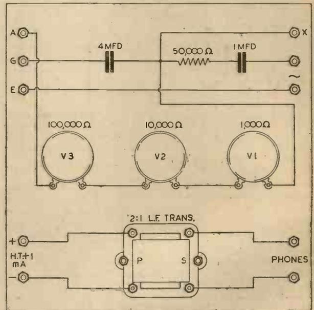
Figs. 4 and 5.—Front view of panel, and wiring diagram of the bridge unit.
