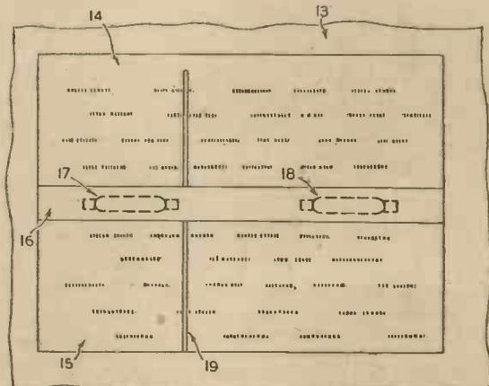
are illuminated by total reflection of light within the glass. The strip 16 is readily detachable to permit access to the lamps from the exterior of the cabinet.
