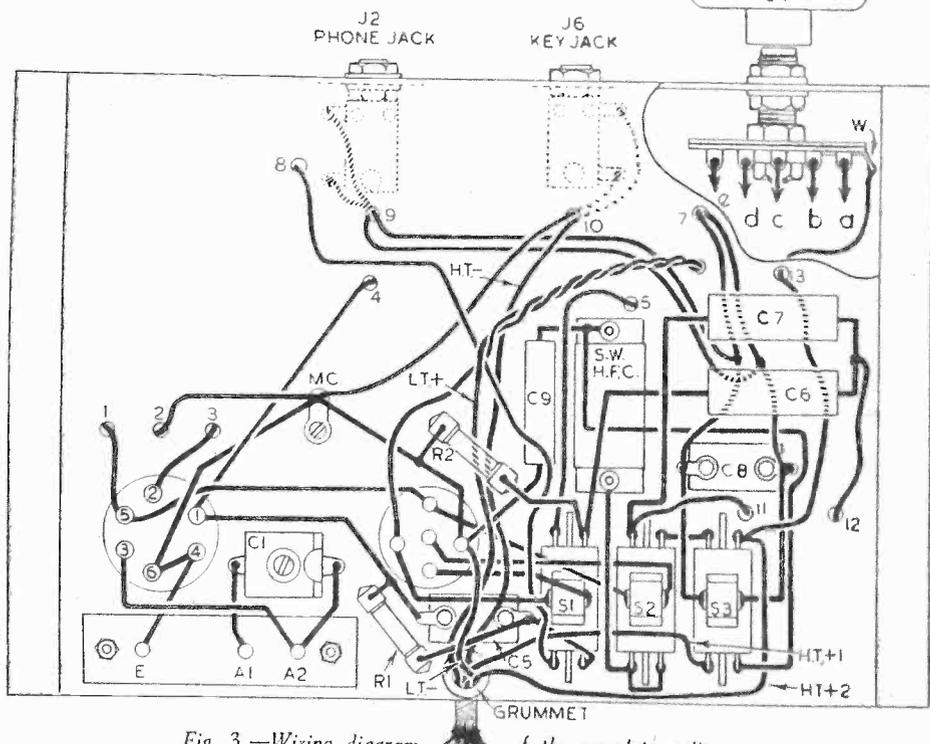
Fig. 3.—Wiring diagram of the complete unit.
