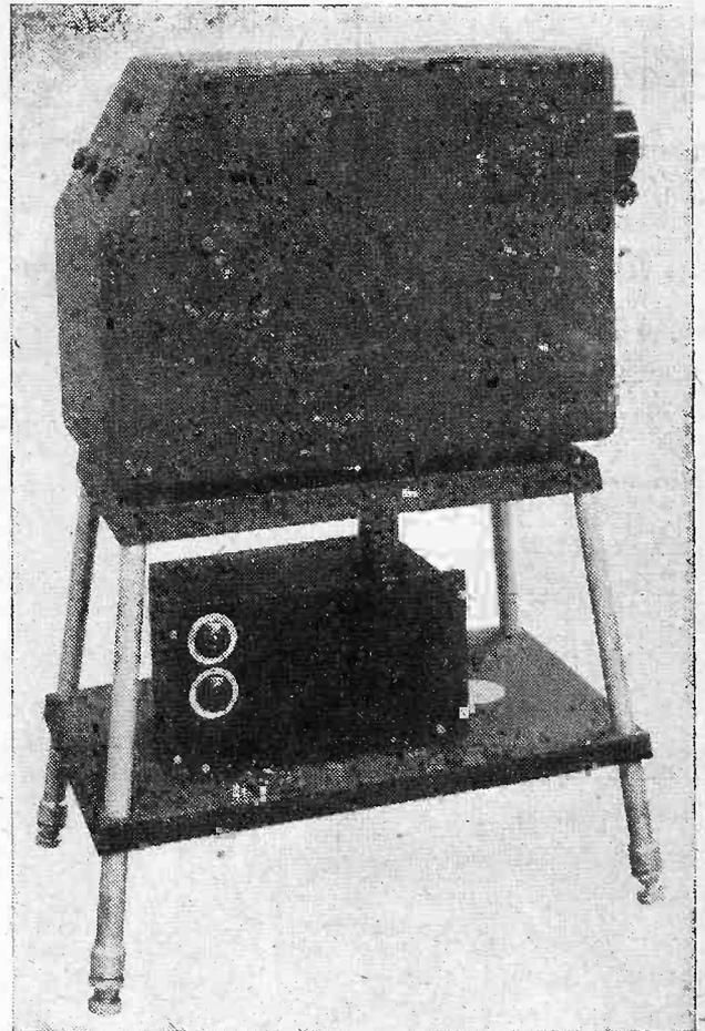
A good example of a compact big-screen television which is suitable for small halls for signal rediffusion.
