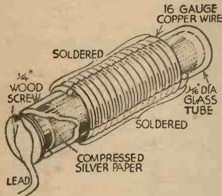
A novel method of making small tubular condensers.
