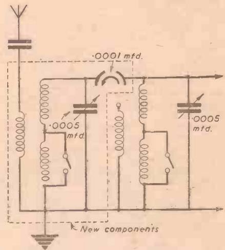
Fig. 3.—A simple form of "top capacity" band-pass coupling by adding a second tuning circuit and small coupling condenser.
