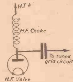
Fig. 1.—The position of the choke in a standard H.F. stage.
