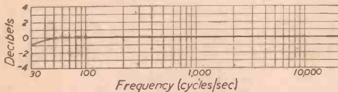
Fig. 1.—Response curve (practically "straight line") for a high-fidelity amplifier.
