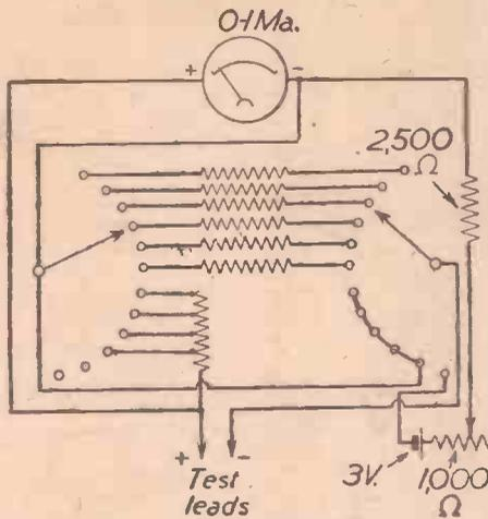
Fig. 1.—Theoretical circuit of the 12-range meter.
