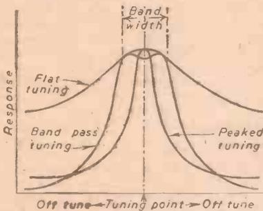
Fig. 1.—These familiar curves show the effect of using different tuning systems. When tuning is flat a wide audio-frequency range is covered, but interference is probable; with peaked tuning the reverse is the case; band-pass allows quality to be combined with selectivity.
