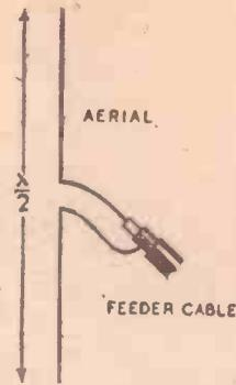
Fig. 2. — Current feeding with a dipole aerial.
