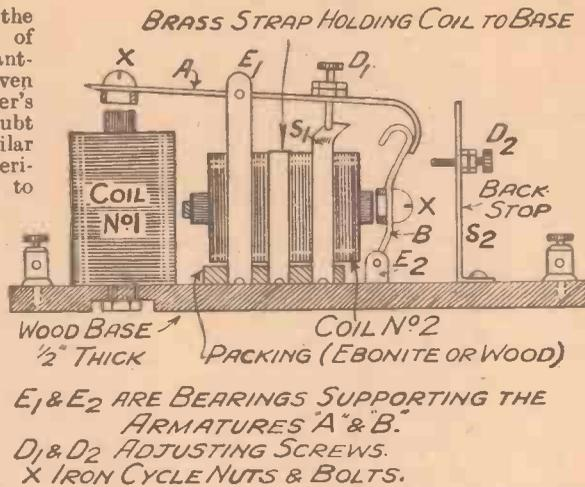
Fig. 1.—Completed relay showing armature "B" attracted, and relay in closed position after No. 2 coil has been momentarily energised. L.T. circuit is then closed and L.T. current then flows up the bottom armature to top armature through bearings to set.
