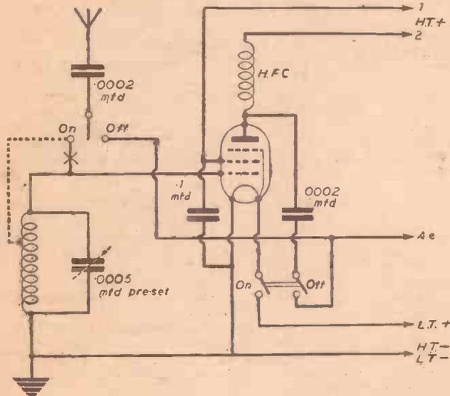
Fig. 1. (Left)—Circuit of a simple pre-tuned H.F. amplifier for use with a Det.-L.F. type of receiver.
