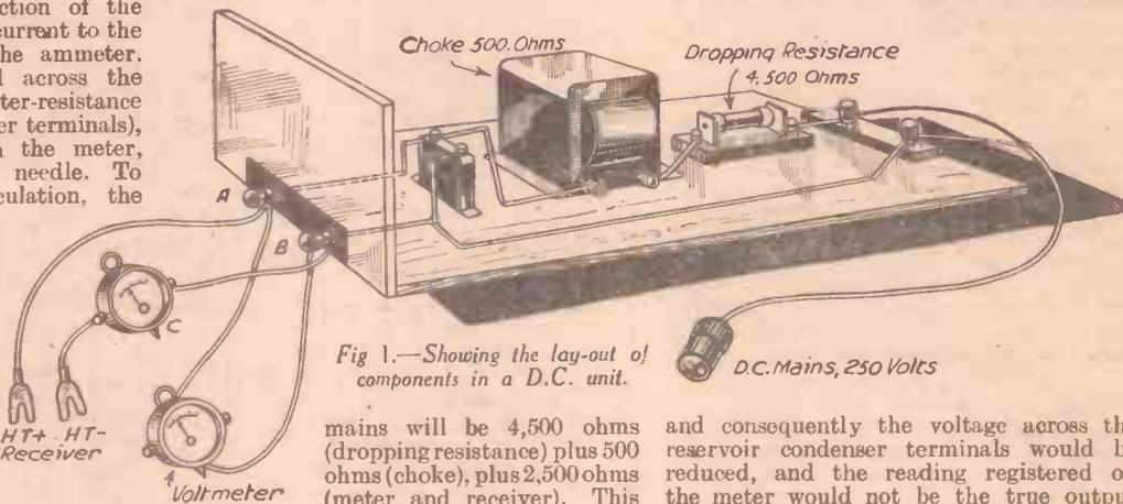
Fig. 1.—Showing the lay-out of components in a D.C. unit.
