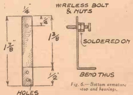
Fig. 6.—Bottom armature stop and bearings.
