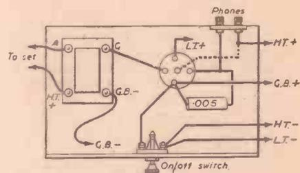
Fig. 2.—The practical arrangement for Fig. 1. A pentode valve can be used if desired.
