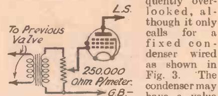
Fig. 4.—When instability is due to fitting a new high-amplification valve, a volume control should be connected between the L.F. transformer and the grid of the valve.
