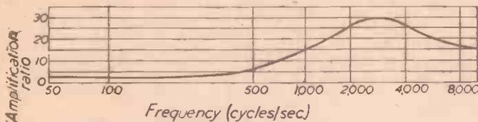
Fig. 4.—This transformer curve is of different form from that shown in Fig. 2, since frequency is plotted against amplification ratio.
