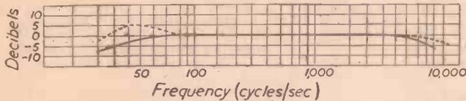
Fig. 2.—Curve for a well-known parallel-fed L.F. transformer. Broken lines show how the curve can be modified by changing circuit constants as explained in the text.
