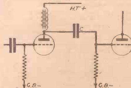
Fig. 3.—L.F. choke used for L.F. coupling purposes.
