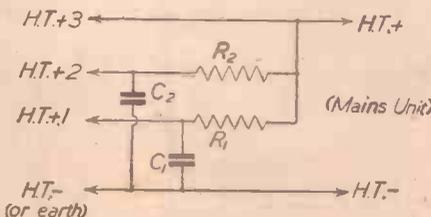
Fig. 4.—How to arrange for the decouplers shown in Fig. 3, so that they may be included between the receiver and mains unit.
