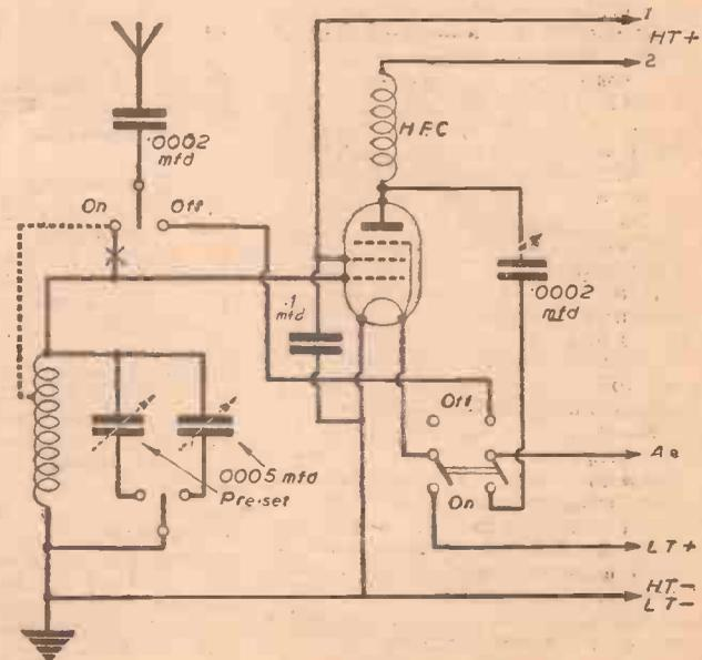
The above remarks apply particularly to a "straight" set already having an H.F. stage. When a detector-L.F. type of receiver is used it will probably be considered worth while to add an H.F. amplifier which can easily be switched into circuit when signal strength is temporarily reduced—this is done by the B.B.C. in the interests of national security, as has been announced on various occasions.
