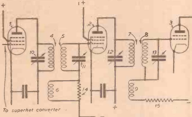
Fig. 1.—The early stages of a standard superhet.
