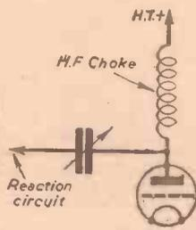
Fig. 3.—The standard reaction H.F. choke.
