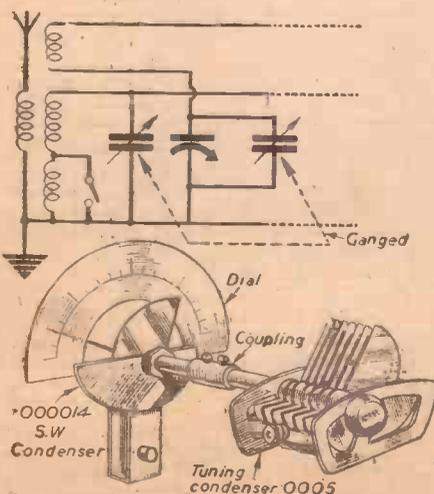
Circuit diagram and pictorial view of a simple unit for preventing oscillation.
