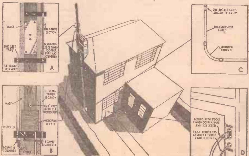
Fig. 4.—Illustrating important points in one form of aerial and feeder installation.
