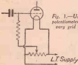
Fig. 1.—Using a potentiometer to vary grid bias.
