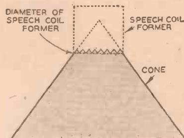
Fig. 4.—Cut off the apex of the cone for a speech-coil mounting.
