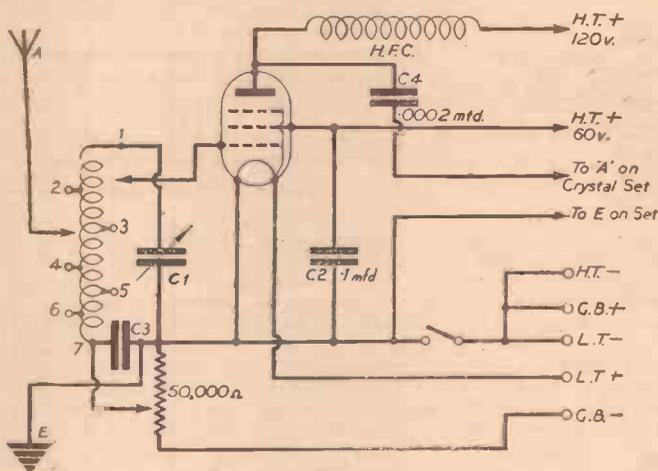
Fig. 1.—An efficient H.F. stage having a wide range of application. An ordinary S.G. valve can be used if so desired.
