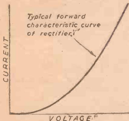
Fig. 1.—Curve of a normal Westector.
