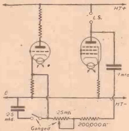
Fig. 1.—A negative feed-back arrangement where control of feed-back is provided by a variable resistor. A ganged switch is used to cut out the negative feed-back when desired.
