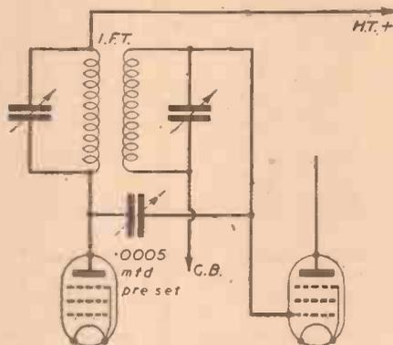
Fig. 4.—"Top-capacity" coupling applied to an I.F. transformer.
