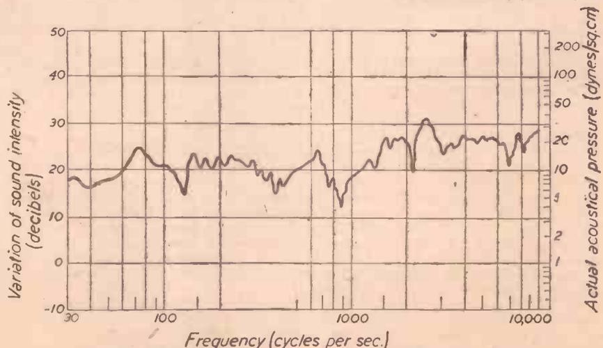
Fig. 3.—A scientific method of plotting a response graph for a high-grade loudspeaker. This is more "detailed" than usual, for in most cases the graph is drawn as a smooth curve.
