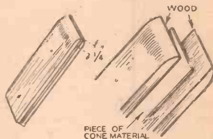
Fig. 7.—A novel tool for turning the cone edge for fixing purposes.
