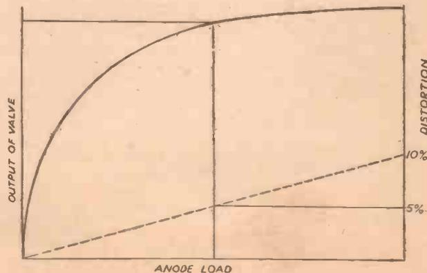
Fig. 2.—This curve shows the relation between output and load with the addition of distortion curves.
