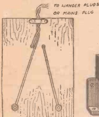
Fig. 2.—The wiring connections underneath the test board.
