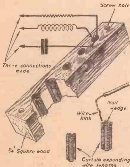
A method of making quick temporary connections.
