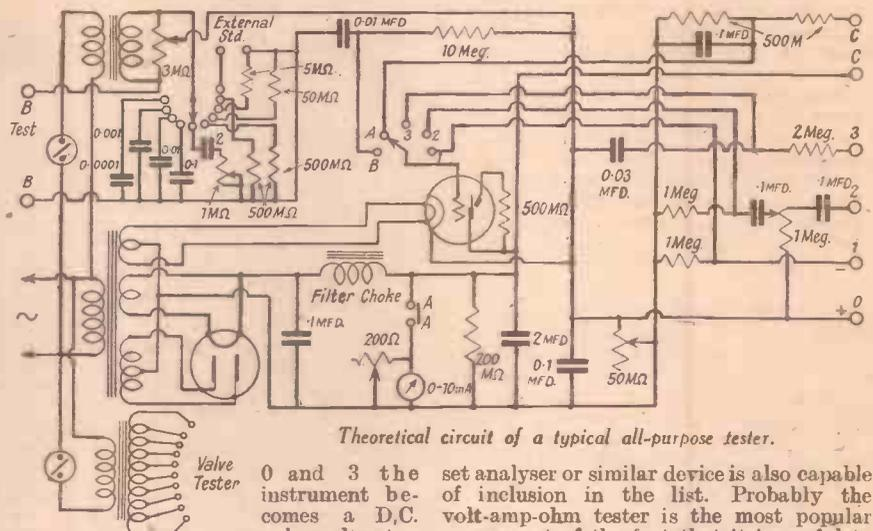
Theoretical circuit of a typical all-purpose tester.
