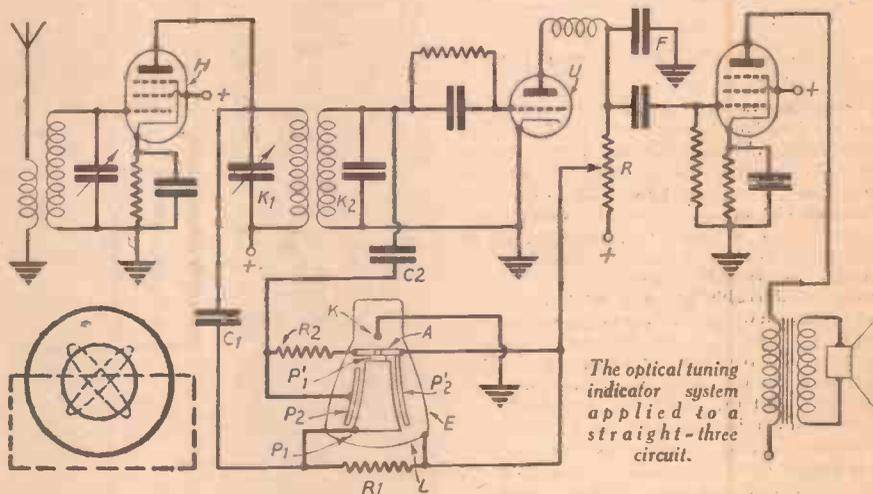
The optical tuning indicator system applied to a straight-three circuit.
