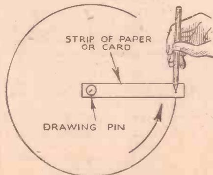
Fig. 5.—Marking out a circle when large compasses are not available.
