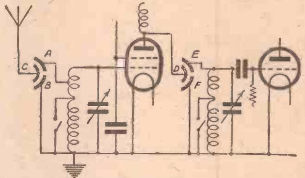
Fig. 7.—Differential condensers used as volume and selectivity controls.
