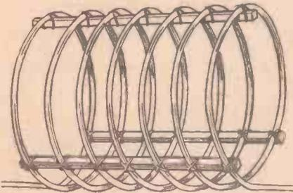
Fig. 1.—A very simple form of self-supporting coil for short-wave working.
