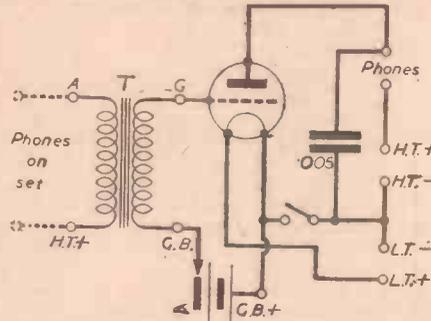
Fig. 1.—When 'phones are to be used, this single valve amplifier will give adequate output.
