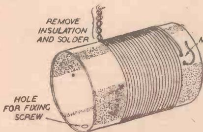
Fig. 2.—Shows how the tapping loops are formed and how the ends of the winding are anchored.
