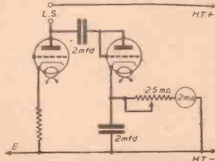
Fig. 3.—A simple output meter, for which an old triode is used as rectifier.
