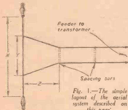
Fig. 1.—The simple layout of the aerial system described on this page.
