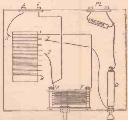
Fig. 3.—A suitable layout and wiring fed to specified parts. M indicates the moving vanes of the tuning condenser.
