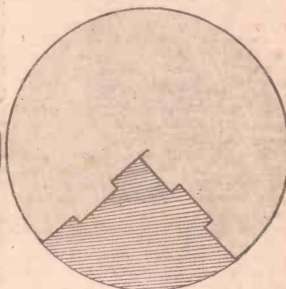
Fig. 3.—A lapped joint is preferred by some constructors.
