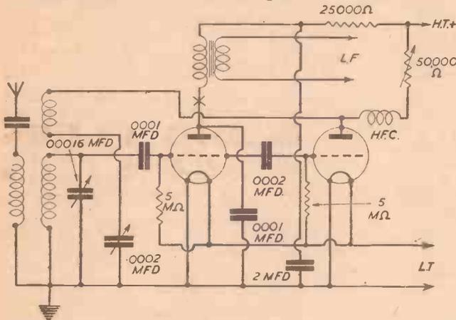
ative circuit proves the most satisfactory short-wave detector, but nevertheless there are many other systems that deserve attention and which provide ample scope for experiment. One of these is illustrated in Fig. 1. The arrangement is by no means novel, but there are probably many readers who have not tried it. As may be seen, there are two triode valves, and these are virtually in parallel.
