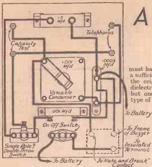
Fig. 1.—Wiring diagram of the simple capacity tester.
