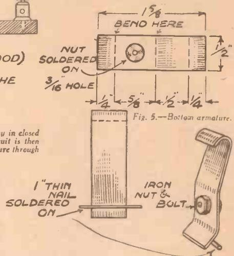
through coil No. 2 the bottom armature is attracted to the core, and in doing so knocks against the top armature and lifts it up. The top armature acts as a kind of latch, and immediately drops back over the bottom armature, and effectively locks it
