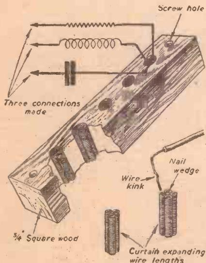
A method of making quick temporary connections.
