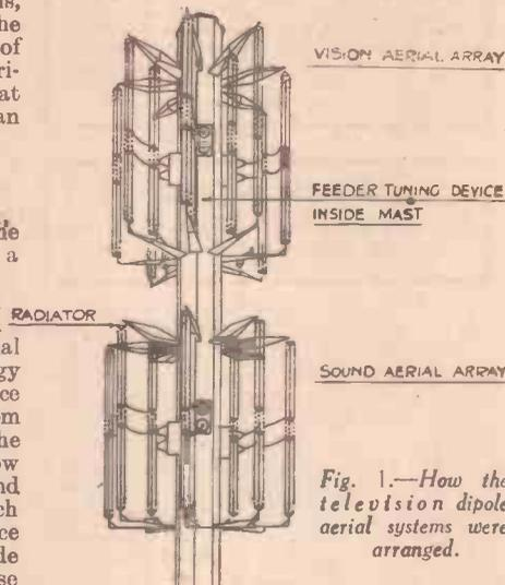
Fig. 1.—How the television dipole aerial systems were arranged.
