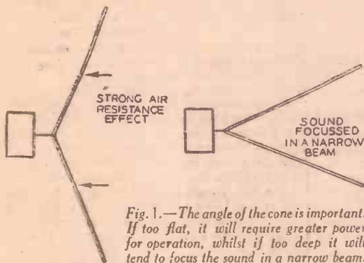
Fig. 1.—The angle of the cone is important. If too flat, it will require greater power for operation, whilst if too deep it will tend to focus the sound in a narrow beam.
