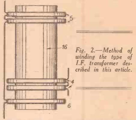
Fig. 2.—Method of winding the type of I.F. transformer described in this article.
