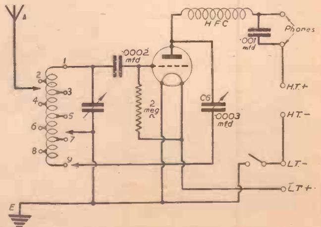
Fig. 3.—How the original coil can be used to form a very efficient one-valver.
