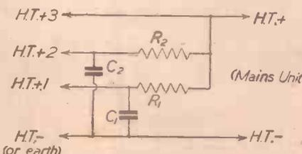
Fig. 4.—How to arrange for the decouplers shown in Fig. 3, so that they may be included between the receiver and mains unit.
