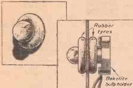
A novel method of mounting pilot bulbs on a panel
