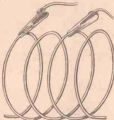
Fig. 3.—Tapping points may be obtained by means of crocodile clips.
