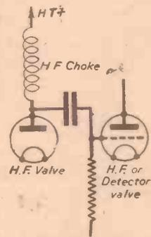
Fig. 2.—Aperiodic H.F. coupling includes a choke as shown here.
