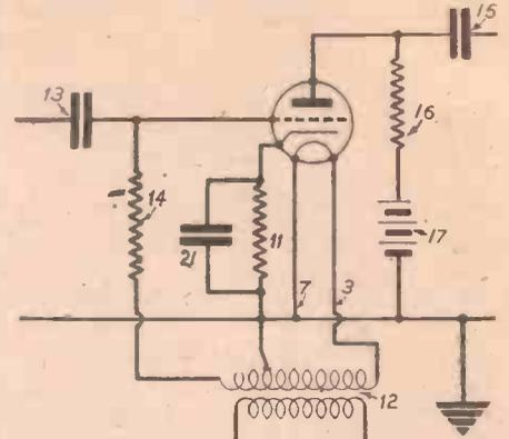
Fig. 3.—Modified circuit showing how hum may be prevented by the special heater and cathode arrangement.
