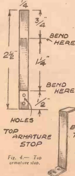
Fig. 4.—Top armature stop.
