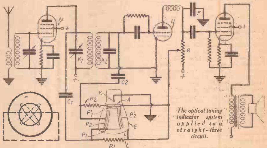
indicated in broken line (or may be prevented from being effective), so that it is possible to determine directly the sense of the detuning from the lateral shift of the visible parts of the ellipse.
