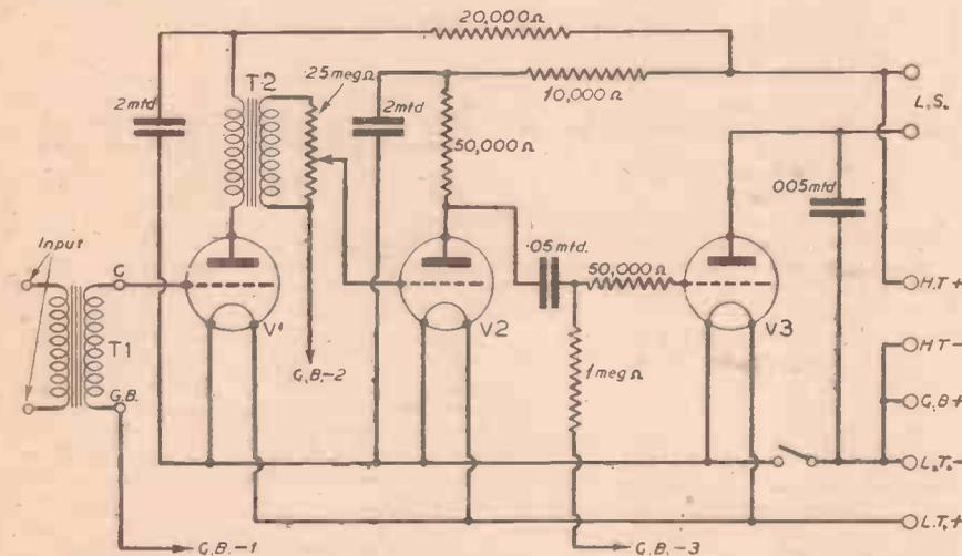
Fig. 3.—A circuit capable of giving ample loudspeaker results from a crystal set input.
