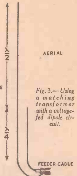
Fig. 3.—Using a matching transformer with a voltage-fed dipole circuit.
