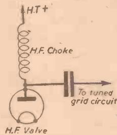
Fig. 1.—The position of the choke in a standard H.F. stage.
