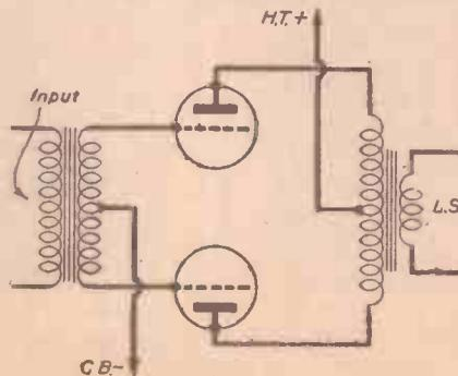
Fig. 2 (Left).—Circuit diagram for a standard push-pull output stage.
