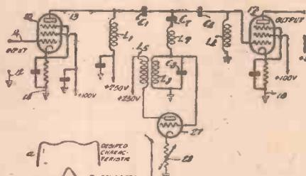
Fig. 3 (Above)—A modified network including a shunt circuit.
