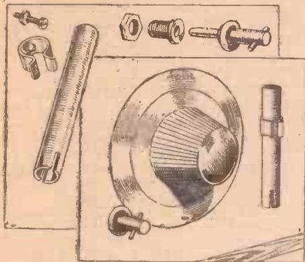
Details of a novel slow-motion control device.
