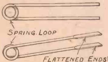
A handy pair of tweezers made from a piece of springy wire.
