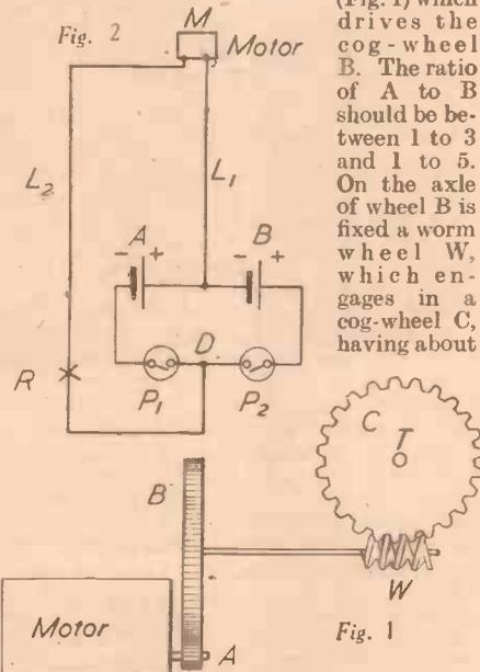
A simple motor-driven remote-control arrangement.
