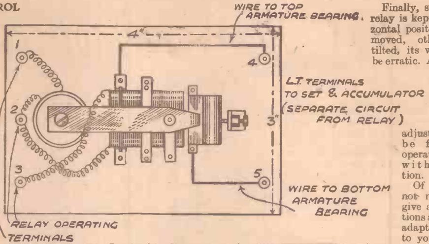
Figs. 8 and 9.—Showing wiring and circuit to relay.
