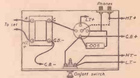
Fig. 2.—The practical arrangement for Fig. 1. A pentode valve can be used if desired.
