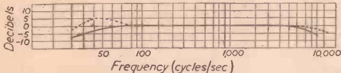
Fig. 2.—Curve for a well-known parallel-fed L.F. transformer. Broken lines show how the curve can be modified by changing circuit constants as explained in the text.
