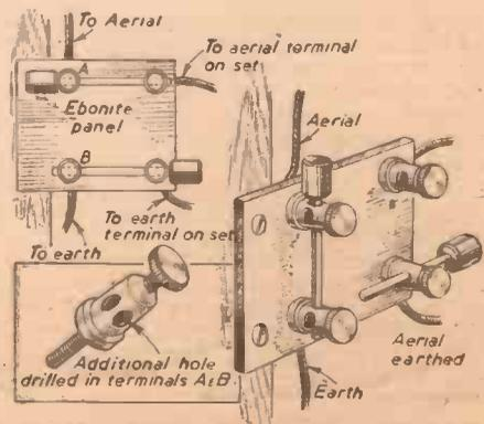
Details of a simple aerial and earth switching arrangement.
