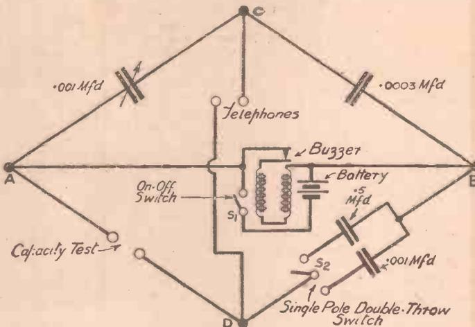
Fig. 2.—Theoretical circuit diagram.
