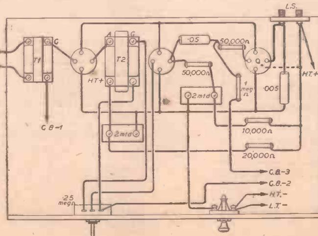
Fig. 4.—The complete wiring and layout for the three-valve amplifier shown in Fig. 3.
