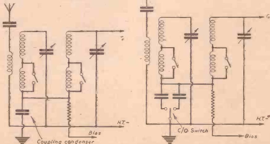
Fig. 2.—A "bottom-capacity" band-pass circuit can be modified to give two alternative band widths by fitting two condensers of different value and a change-over switch.
