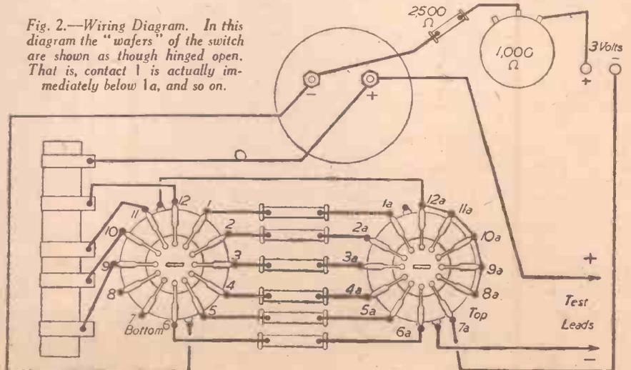
Fig. 2.—Wiring Diagram. In this diagram the "wafers" of the switch are shown as though hinged open. That is, contact 1 is actually immediately below 1a, and so on.
