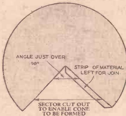
Fig. 2.—Marking out the cone. Note the angle of the cut-out section.
