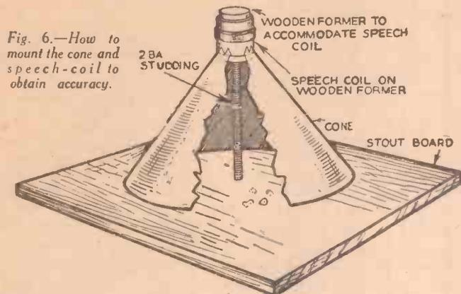
Fig. 6.—How to mount the cone and speech-coil to obtain accuracy.
