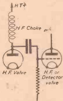
Fig. 2.—Aperiodic H.F. coupling includes a choke as shown here.
