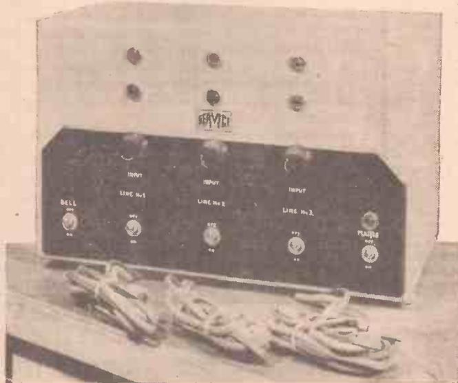
The E.M.I. Service Intermittent Fault Test Device.
