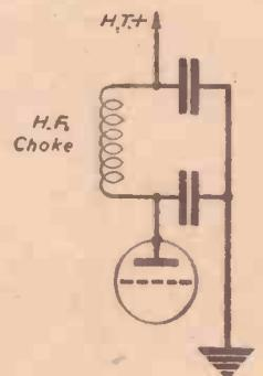
Fig. 3 (Right).—An efficient H.F. filter arrangement.
