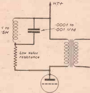
Fig. 5.—A similar arrangement to Fig. 4, but designed for transformer coupling.
