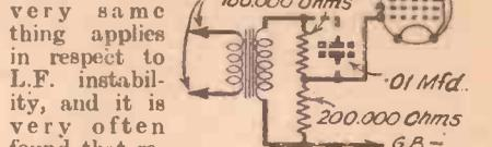
Fig. 5.—The amplification of an L.F. stage can easily be reduced by using the connections shown above, and explained in the text.
