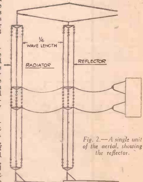
Fig. 2.—A single unit of the aerial, showing the reflector.
