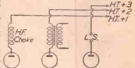
Fig. 2.—A skeleton standard 3-valve circuit showing normal anode connections.
