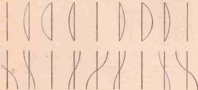
Fig. 1.—Showing the current and voltage changes for one complete cycle in a dipole aerial.
