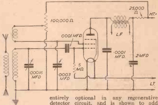
Fig. 2.—This circuit is comparable with that shown in Fig. 1, but an H.F. pentode acts as a double triode valve.
