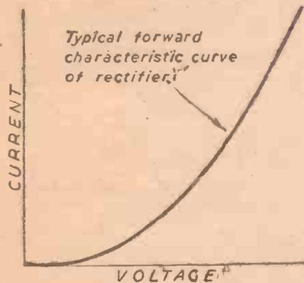
Fig. 1.—Curve of a normal Westector.
