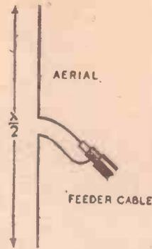
Fig. 2.—Current feeding with a dipole aerial.
