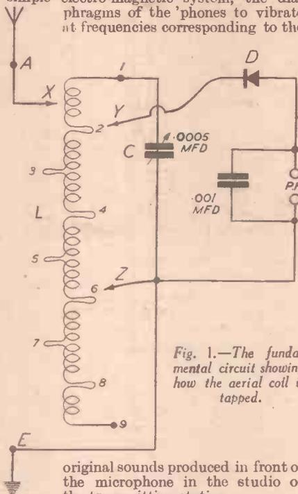
Fig. 1.—The fundamental circuit showing how the aerial coil is tapped.
