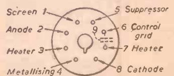
Fig. 1.—Octal valve base showing electrode connections.
