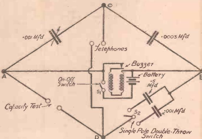
Fig. 2.—Theoretical circuit diagram.
