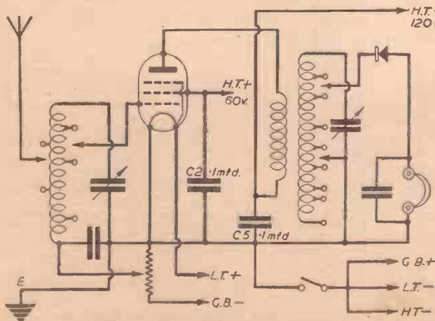
Fig. 2.—The H.F. transformer system of inter-valve coupling is shown in this circuit.
