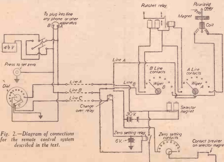
Fig. 2.—Diagram of connections for the remote control system described in the text.
