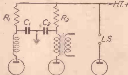
Fig. 3.—The arrangement of Fig. 2, plus decouplers
