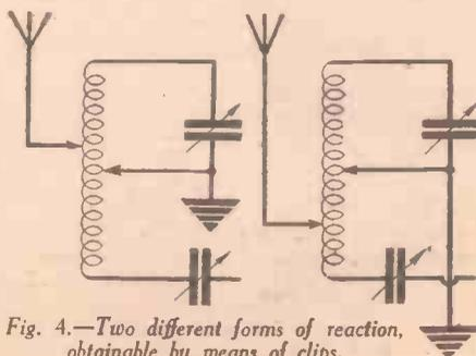
Fig. 4.—Two different forms of reaction, obtainable by means of clips.
