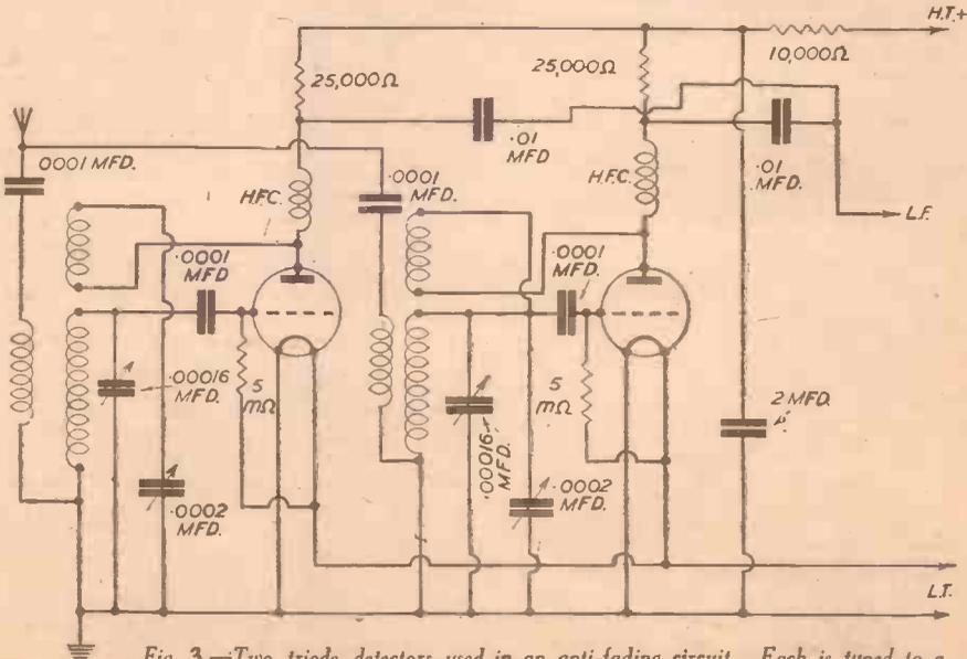
Fig. 3.—Two triode detectors used in an anti-fading circuit. Each is tuned to a different wavelength on which the same programme is being radiated.
