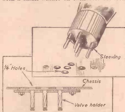
A novel method of fitting sub-chassis valveholders
