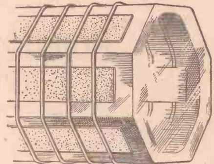
Fig. 2.—Here a solid former is used for the preliminary coil winding. It is afterwards removed.
