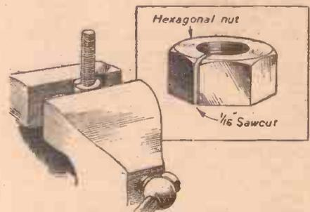
An effective clamp for holding screwed rods in a vice.
