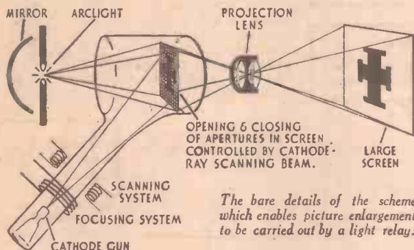
The bare details of the scheme which enables picture enlargement to be carried out by a light relay:
