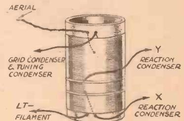
Coil connection details for the Gas-mask Box Receiver.
