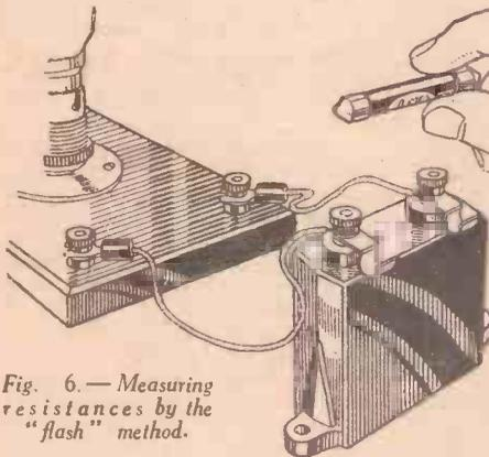
Fig. 6.—Measuring resistances by the “flash” method.
