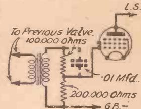
Fig. 5.—The amplification of an L.F. stage can easily be reduced by using the connections shown above, and explained in the text.
