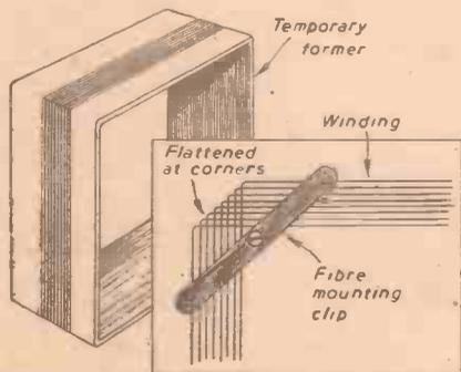
Fig. 2.—A compact frame aerial may be made by winding the wire on a temporary former and then flattening the corners.
