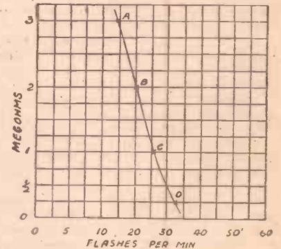
Fig. 7.—The curve used for finding the value of resistances.
