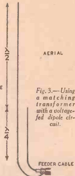
Fig. 3.—Using a matching transformer with a voltage-fed dipole circuit.
