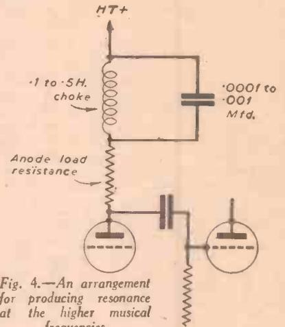
Fig. 4.—An arrangement for producing resonance at the higher musical frequencies.
