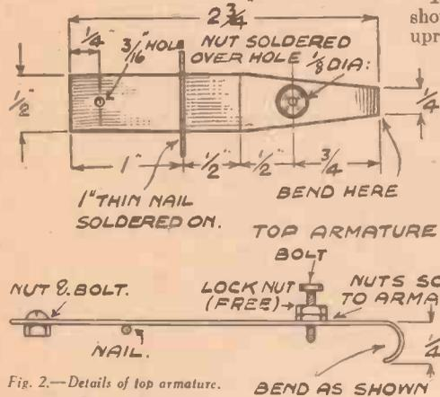
Fig. 2.—Details of top armature.
