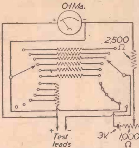
Fig. 1.—Theoretical circuit of the 12-range meter.
