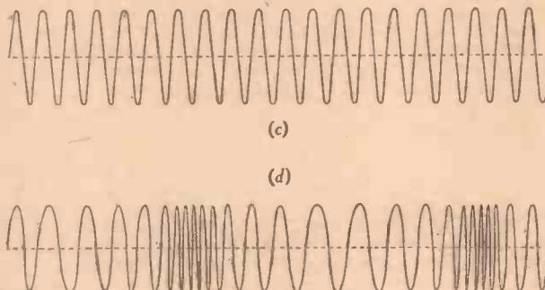
(c) is the carrier and audio wave combined in Amplitude Modulation, whilst (d) is the same combination in Frequency Modulation.
