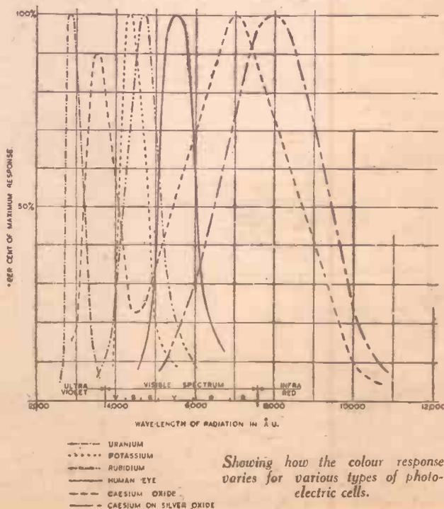
Showing how the colour response varies for various types of photo-electric cells.
