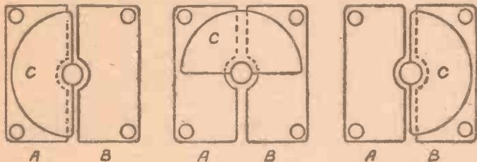
Fig. 2.—Plan of the vanes of a differential condenser, showing three different settings of the condenser.
