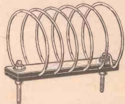
Fig. 5.—How to arrange for plugging in the coil.
