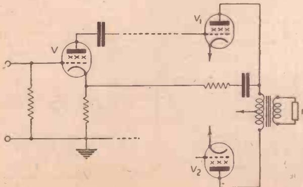
Fig. 1.—Standard push-pull amplifier with feedback taken from the primary of the output transformer.
