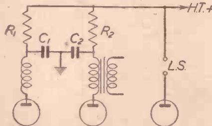
Fig. 3.—The arrangement of Fig. 2, plus decouplers
