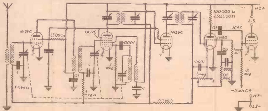
Fig. 2.—Diagram of superhet for the new 1.4 volt valves.
