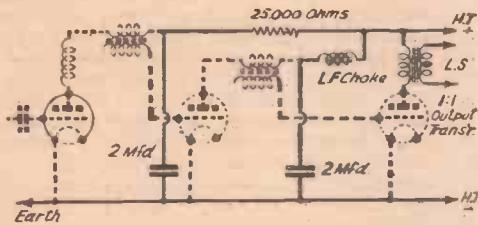
Fig. 1.—Theoretical diagram showing how the detector and subsequent L.F. valves can most easily be decoupled. The decoupling components and wiring are shown by full lines.
