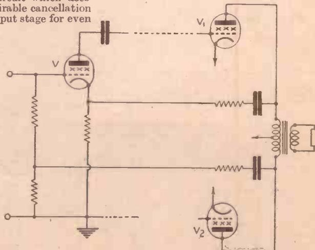
Fig. 2.—Additional feedback is provided in this circuit—balancing out even harmonics.
