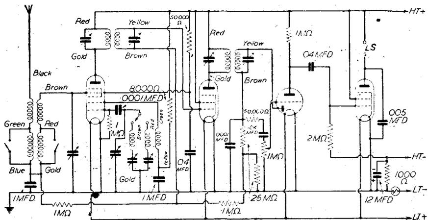
Theoretical circuit of the receiver, with colour-coded references for the coils.
