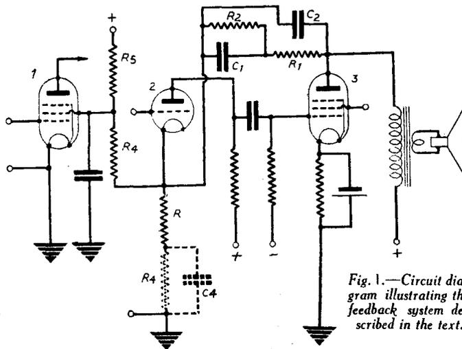
Fig. 1.—Circuit diagram illustrating the feedback system described in the text.
