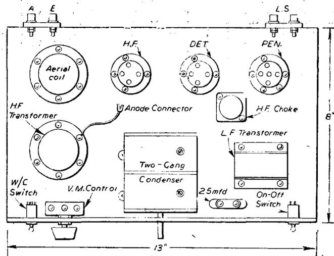
Fig. 2.—A suitable general layout for a set incorporating a circuit of the type shown in Fig. 1. It will be seen that reasonable compactness is aimed at, without making access to component terminals difficult. The chassis layout shown in Fig. 3 is usually to be preferred.
