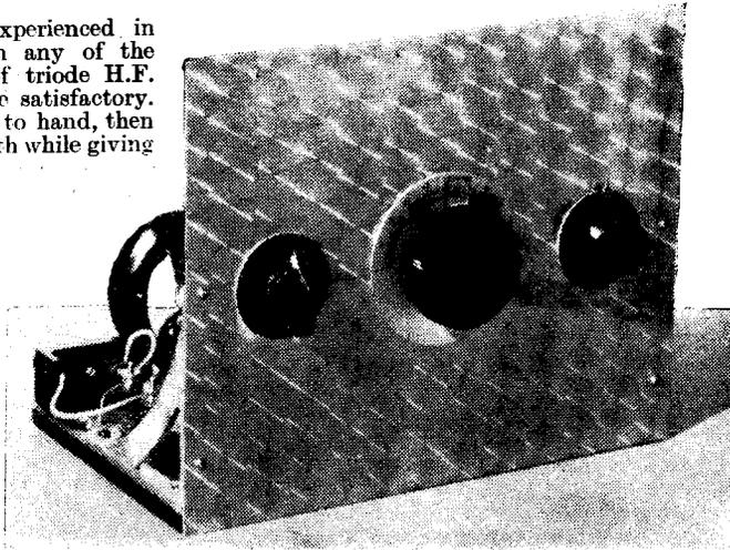
The clean panel layout is emphasised in this illustration, the centre control being that of the band-spreader, the tank being on the left and the reaction control on the right.
