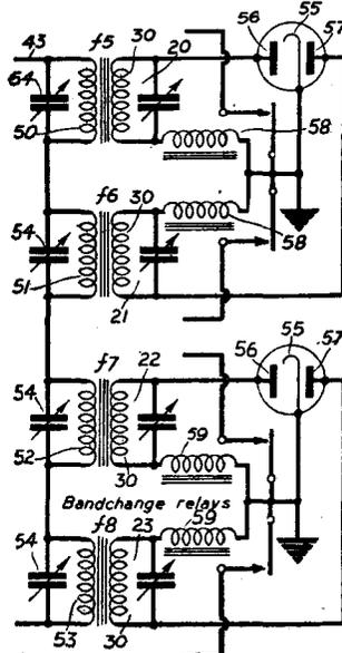
Fig. 3.—A more sensitive arrangement for the receiver.
