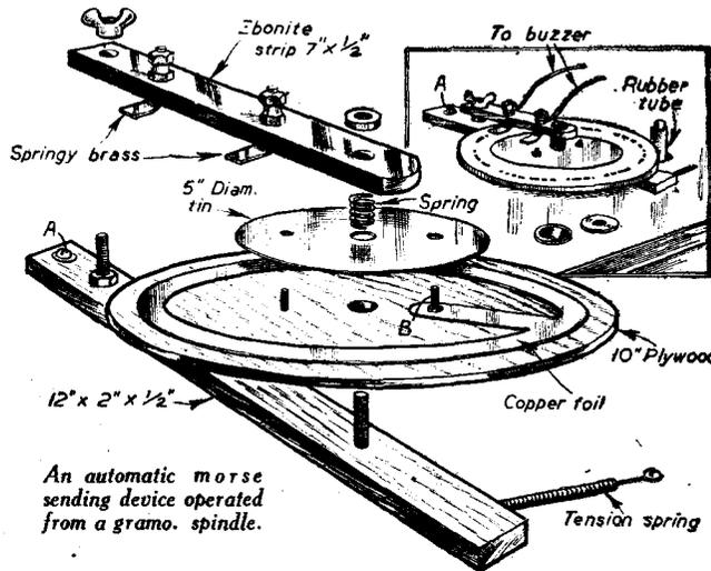
An automatic morse sending device operated from a grammo. spindle.
