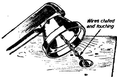
Radiogram reproduction was found to "cut-out" sometimes while the gramophone was in use due to short-circuit of the pick-up leads where they passed through the motor board.
