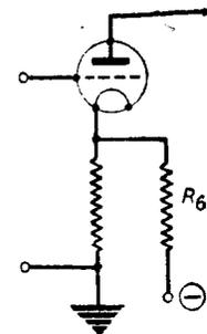
Fig. 3.—Current back-coupling by means of a cathode resistance.
