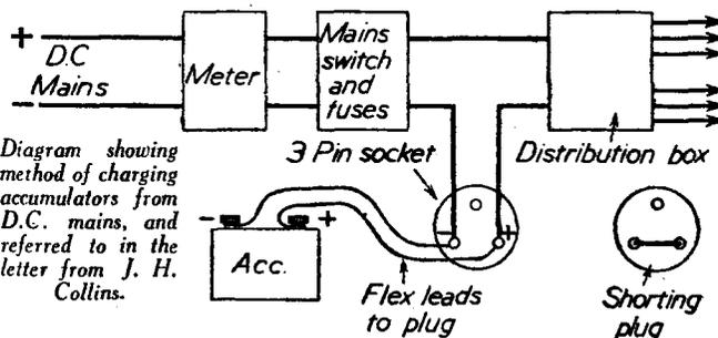
Diagram showing method of charging accumulators from D.C. mains, and referred to in the letter from J. H. Collins.
