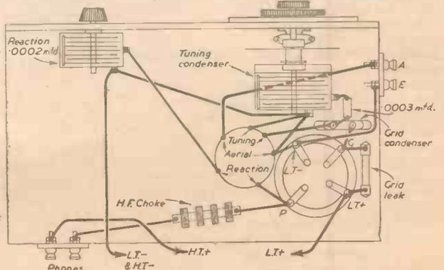
This plan shows how the constructor has endeavoured to keep H.F. leads as short as possible. Ample space is left for an L.F. stage.
