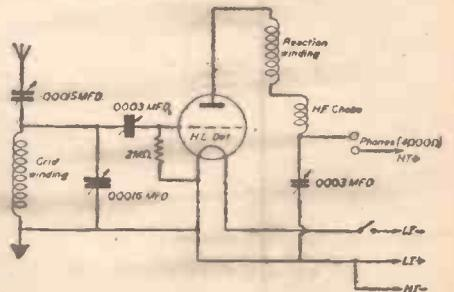
Circuit diagram of a "super" one-valver, described by P. Dickerson, of Fritton.
