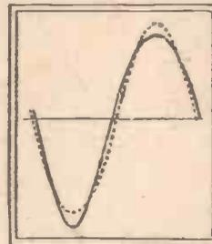
Fig. 4.—The result of combining the two curves, showing how the introduction of second harmonic alters the shape of the pure sine curve.
