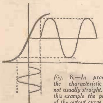
Fig. 8.—In practice the characteristic is not usually straight. In this example the peaks of the output curve are flattened. This means the production of a strong third harmonic.
