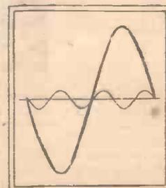
Fig. 5.—Sine curves representing the fundamental and a third harmonic.
