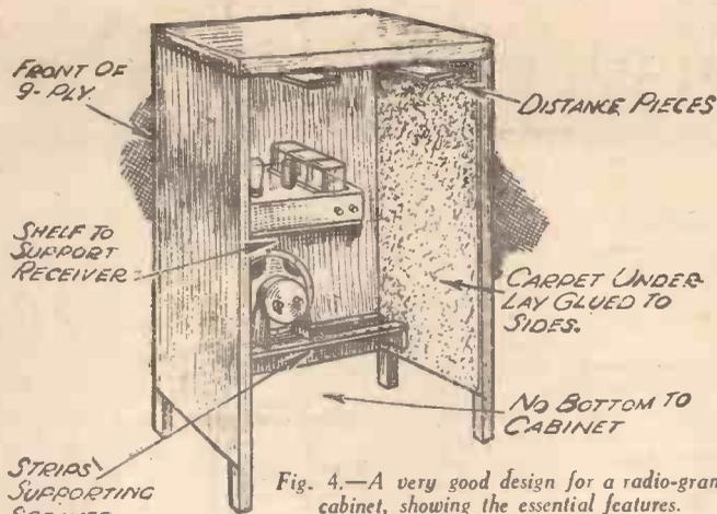
Fig. 4.—A very good design for a radio-gram cabinet, showing the essential features.
