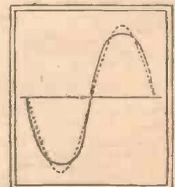
Fig. 6.—The effect of the third harmonic is to flatten the peaks of the fundamental curve.
