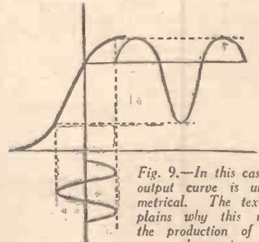
Fig. 9.—In this case the output curve is unsymmetrical. The text explains why this means the production of even harmonics.
