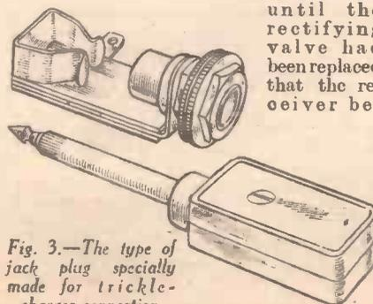
Fig. 3.—The type of jack plug specially made for trickle-charger connection.
