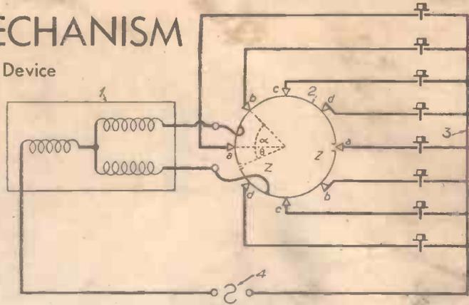
The general arrangement of an automatic wave-changing system employing commutator switching devices.
