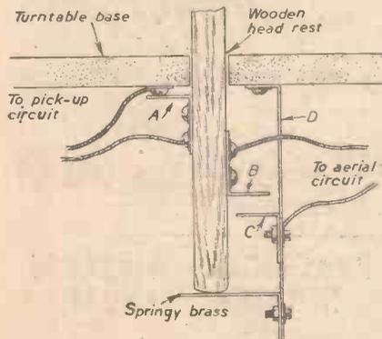
A device for automatically switching in a pick-up as soon as the arm is lifted off the rest.
