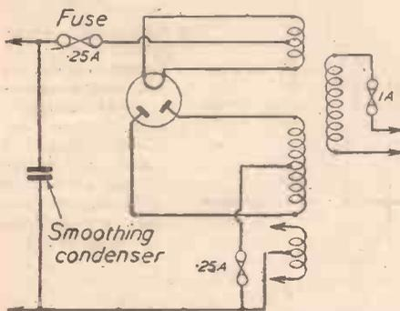
Fig. 1.—Alternative positions for a safety fuse in the rectifier circuit. The fuse in the mains lead should be used in addition. Indicated values are approximate only, and depend largely on the rectifier output.
