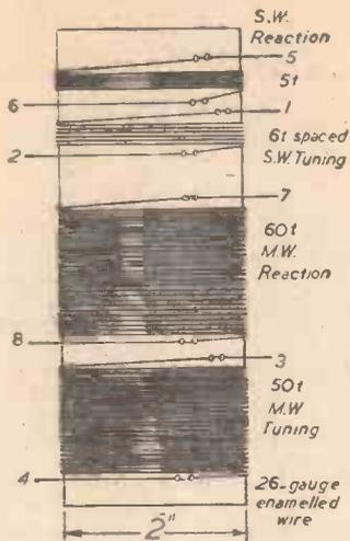
Fig. 1.—Details of a suitable short and medium-wave coil shown approximately to scale, assuming the use of 26-gauge enamelled wire. The length of the former should be about 5in., or 6in. if 24-gauge wire is used.
