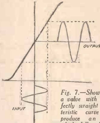
Fig. 7.—Showing how a valve with a perfectly straight characteristic curve would produce an output which followed faithfully the wave-form of the input and would, therefore, contain no harmonics.
