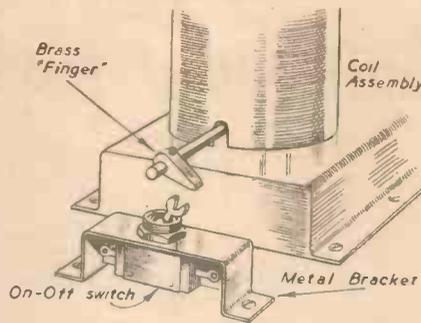
Fig. 4.—A method of operating a toggle on-off (battery or mains) switch from the spindle of built-in wave-change switches.
