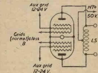
Fig. 6.—A novel modification of a Q.P.P. valve.
