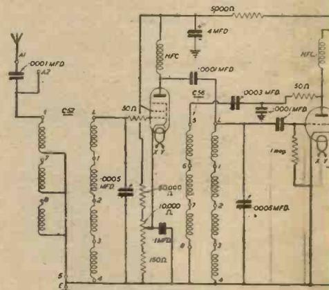
Theoretical circuit diagram of the A.C. Four-wave receiver, with some components omitted to avoid complications when
