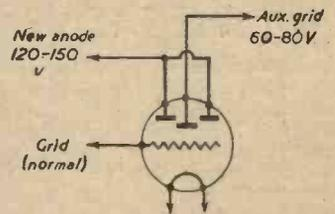
Fig. 4.—Method of utilising a double-diode valve to operate as a screened-grid valve.
