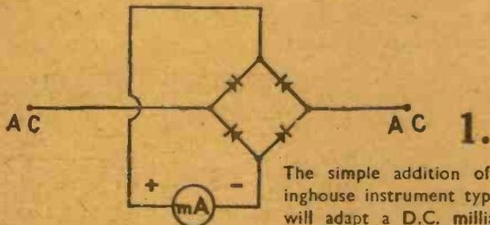
1. The simple addition of a Westinghouse instrument type rectifier will adapt a D.C. milliammeter to read A.C. milliamps with 11 per cent. higher full scale range.
