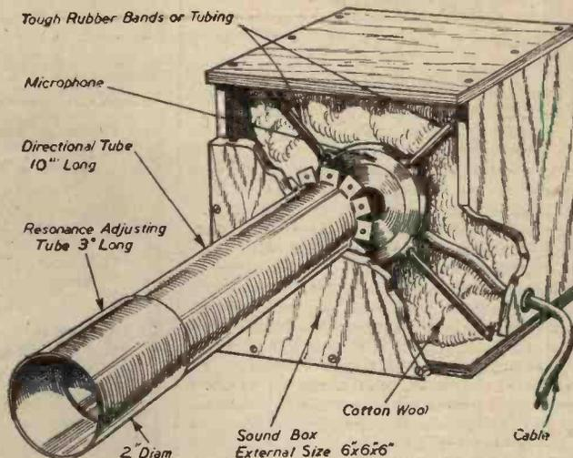
Fig. 2.—Part sectional view showing construction of sound box and directional resonator tube.
