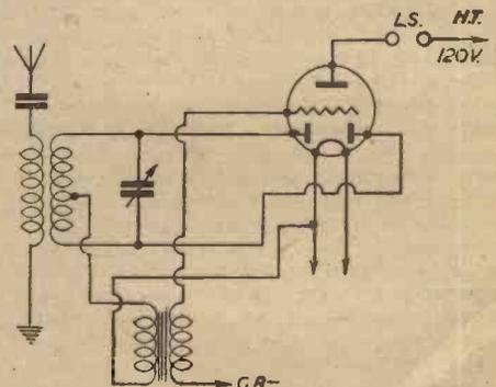
Fig. 7.—Method of modifying a double-diode-triode valve.
