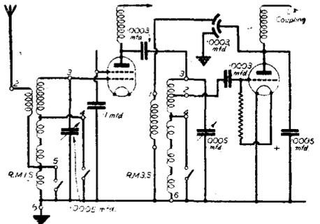
Fig. 3.—An efficient S.G. Three can be built around these types.
