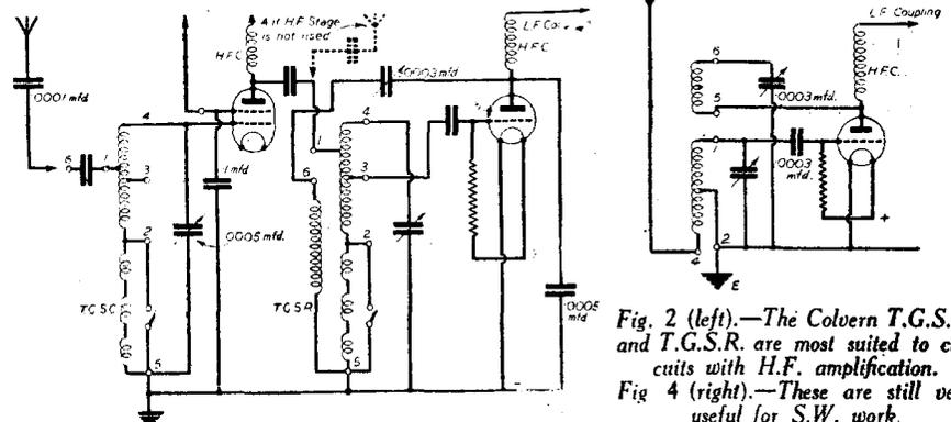
Fig. 2 (left).—The Colvern T.G.S.C. and T.G.S.R. are most suited to circuits with H.F. amplification.
