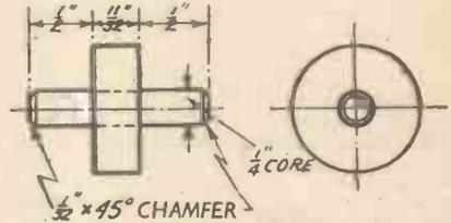
Fig. 4.—Details of Alnico bobbins.
