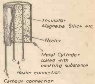
Fig. 11.—An indirectly heated cathode.
