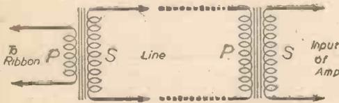
Fig. 6.—Matching of a ribbon microphone.
