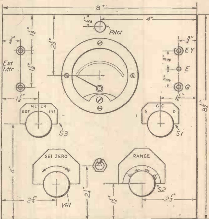
Fig. 4.—Panel layout and drilling measurements.
