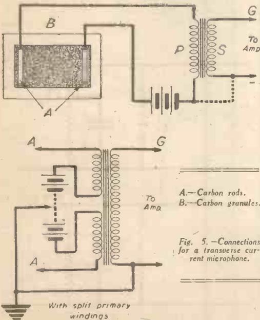
Fig. 5.—Connections for a transverse current microphone.
