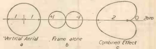
Fig. 3.—Principle of the cardioid response curve.
