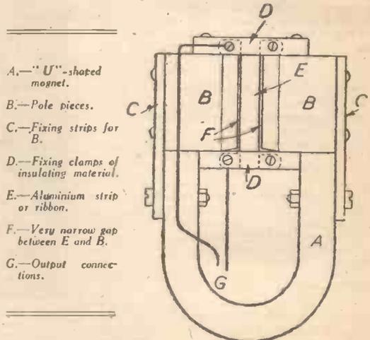
Fig. 2.—Details of a ribbon microphone.
