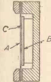
Fig. 3.—Section of a high-impedance microphone.
