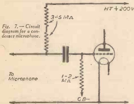
Fig. 7.—Circuit diagram for a condenser microphone.
