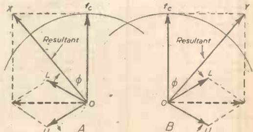
Fig. 5.—Vectors for an FM transmission.
