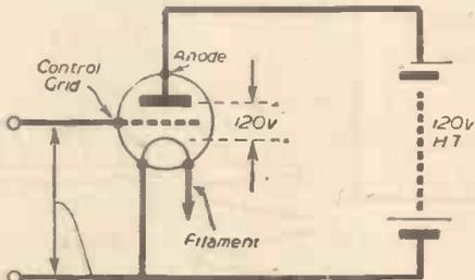
Smaller PD acting through this smaller space can have the same effect as the 120v through anode/filament space
