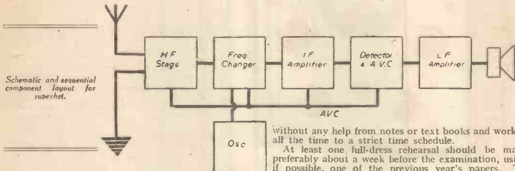
Schematic and sequential component layout for superhet.
