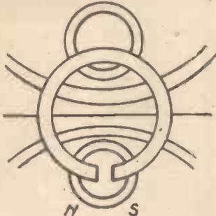
Fig. 5.—Diagram indicating leakage by atmospheric paths.
