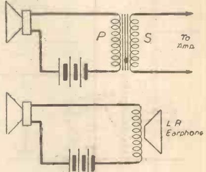
Fig. 4.—Connections for carbon microphones.
