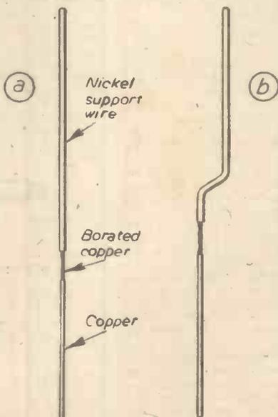
Fig. 2 (a).—Straight foot-wire. (b) Cranked foot-wire.
