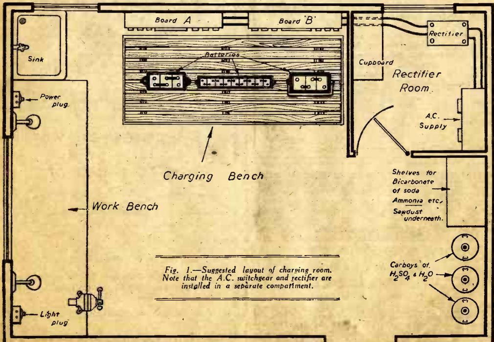
Fig. 1.—Suggested layout of charging room. Note that the A.C. switchgear and rectifier are installed in a separate compartment.
