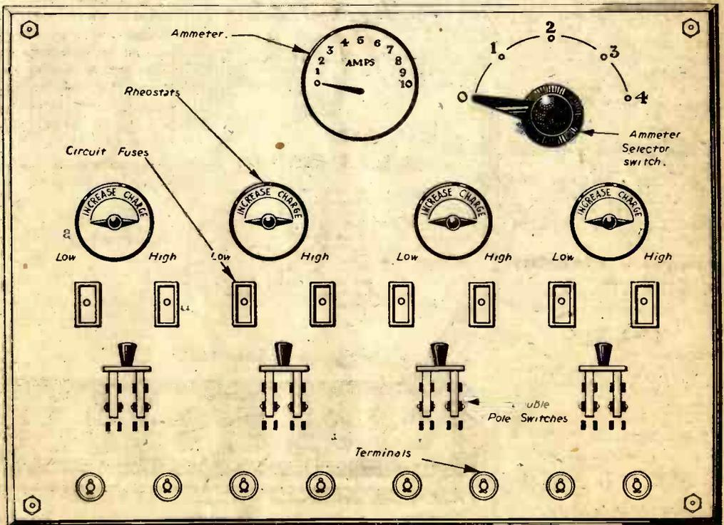
Fig. 3.—A four-circuit charging panel.
