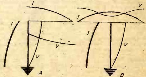
Fig. 72.—A, "Inverted L" aerial. B, "T" type aerial.
