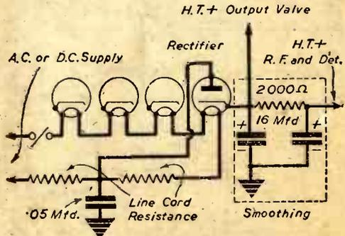
Fig. 2.—A typical H.T. smoothing circuit as used in midget A.C./D.C. receivers.
