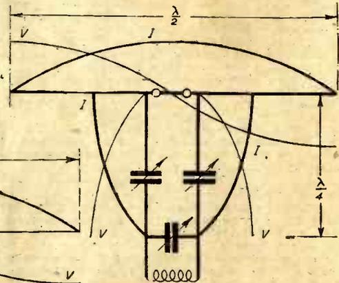
frequency can be adjusted by variation of its capacity or inductance. The main difference between an aerial and a tuned circuit (closed) is that whilst the aerial is designed for maximum radiation, the tuned circuit necessitates minimum radiation.
