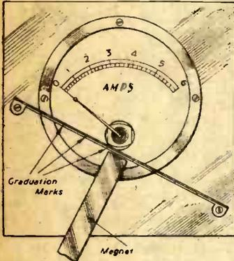
A simple Magnetometer.
