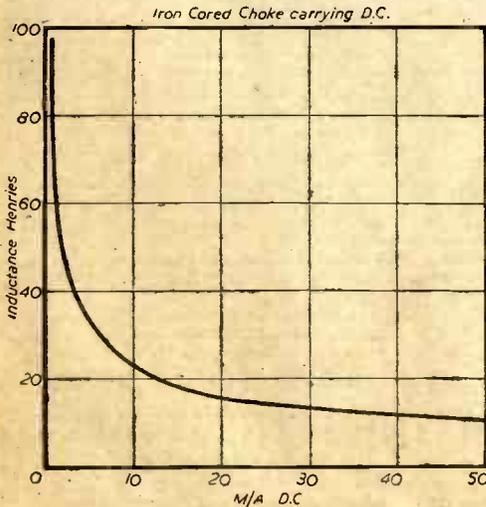
Fig. 1.—Curve showing the relationship between the D.C. component and inductance of an iron cored choke.
