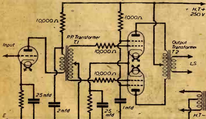
Fig. 1.—A tetrode push-pull stage following a triode amplifier. The latter may be the triode portion of a double-diode triode.
