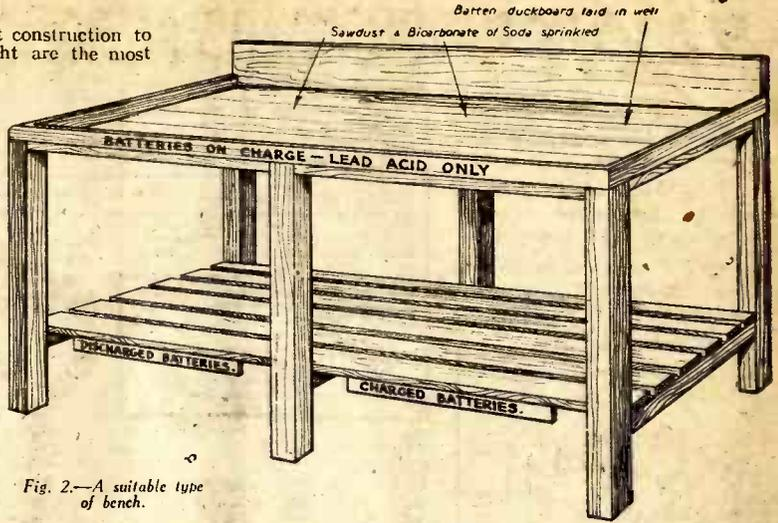
Fig. 2.—A suitable type of bench.
