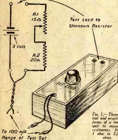
Fig. 1.—Theoretical and practical forms of a small unit to measure resistances from 1 ohm to 2,000 ohms.
