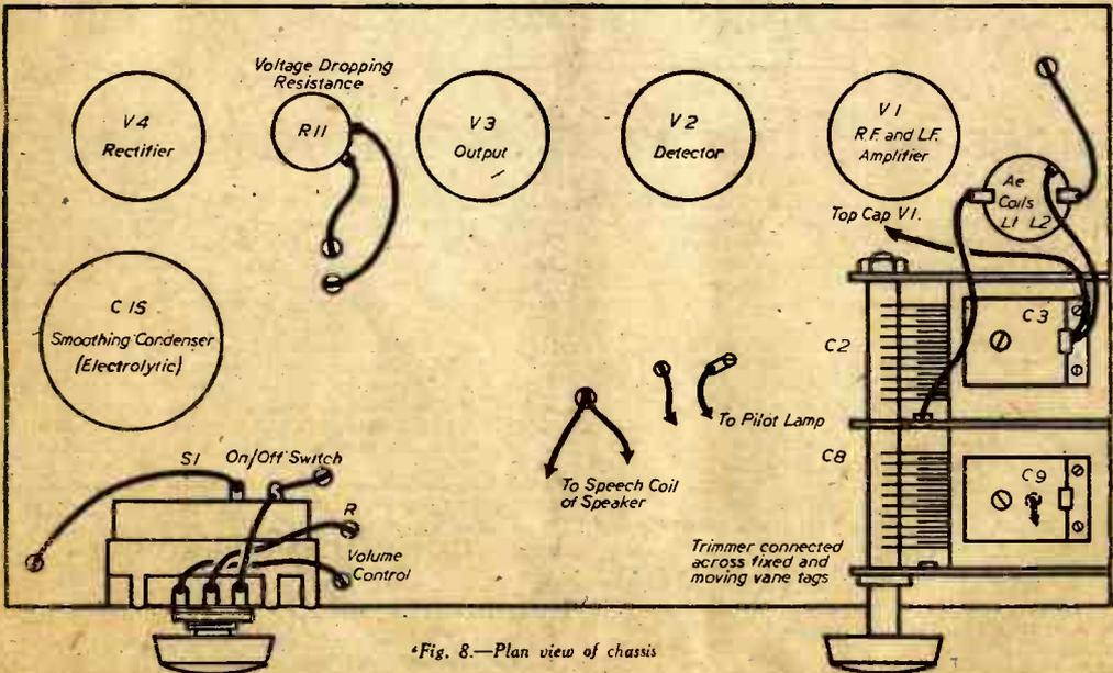
\*Fig. 8.—Plan view of chassis
