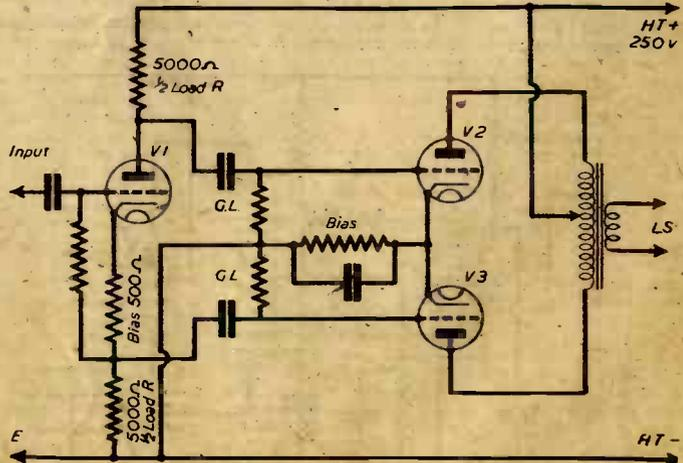
Fig. 4.—Outline circuit of a paraphase amplifier, where valve V1 takes the place of a push-pull transformer, and acts as a phase-splitter, while V2 and V3 behave as normal push-pull valves. The values shown are purely nominal, and are intended primarily to show that resistors of equal value are used in anode and cathode circuits.
