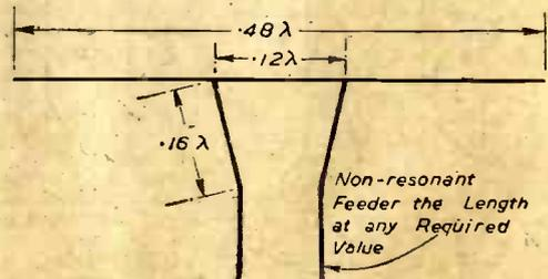
Fig. 77.—The use of a non-resonant feeder with a  $\lambda/2$  (approx.) dipole.
