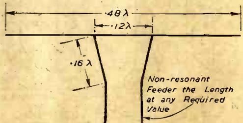
Fig. 77.—The use of a non-resonant feeder with a  $\lambda/2$  (approx.) dipole.
