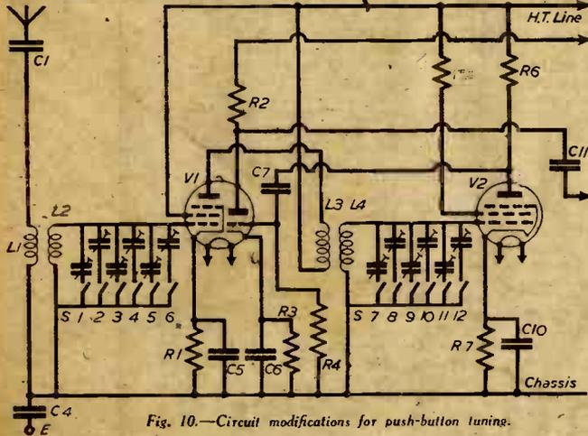
Fig. 10.—Circuit modifications for push-button tuning.
