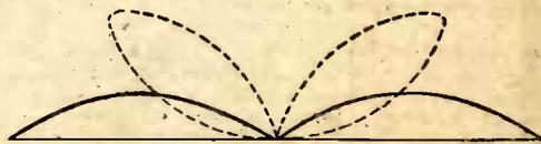
Fig. 79.—The effect of earth conductivity upon a  $\lambda/2$  aerial.
