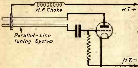
Fig. 3.—Resonant or parallel-line tuning, which is most satisfactory for use with ultra-short and micro-waves.
