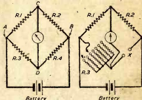
Fig. 2.—Basic circuit of the Wheatstone Bridge.
