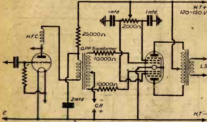
Fig. 3.—A Q.P.P. stage following a leaky-grid detector.
