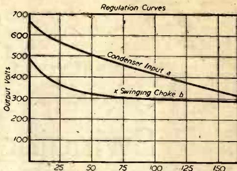
Fig. 4.—Regulation curves of two types of power pack.
