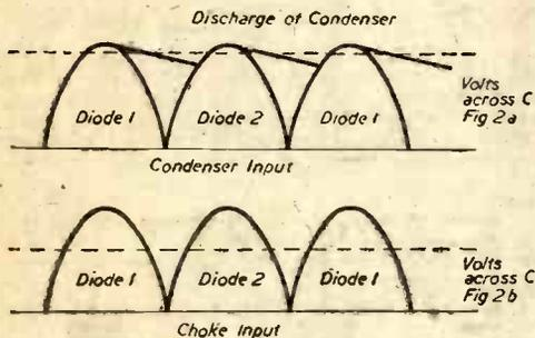
Fig. 3.—Output voltage waveforms of a full-wave rectifier with condenser and choke output.
