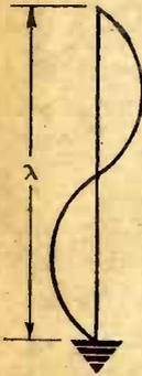
Fig. 73.—(Left) Cancellation of radiation when aerial length is a multiple of  $\lambda$ .
