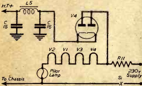
Fig. 9.—(Above) Modifications for low anode voltage values.
