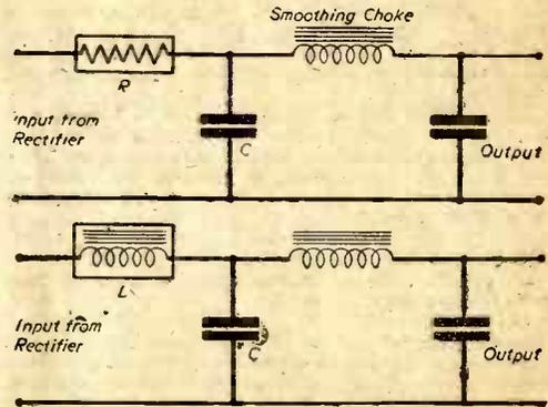
Fig. 2.—(a) (upper) Zero inductance is represented by R—the D.C. resistance of the windings. (b) (lower) The same choke shown as an inductance, L.
