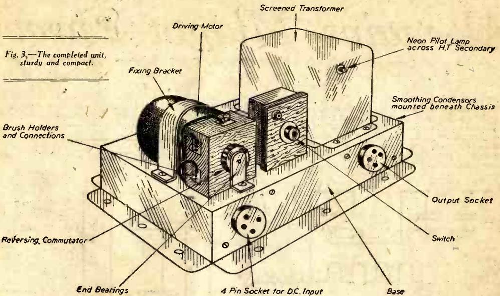
Fig. 3.—The completed unit, sturdy and compact.
