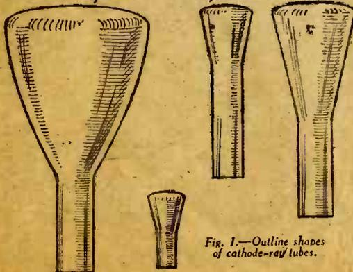
Fig. 1.—Outline shapes of cathode-ray tubes.
