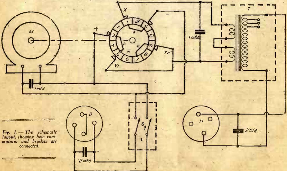
Fig. 1.—The schematic layout, showing how commutator and brushes are connected.
