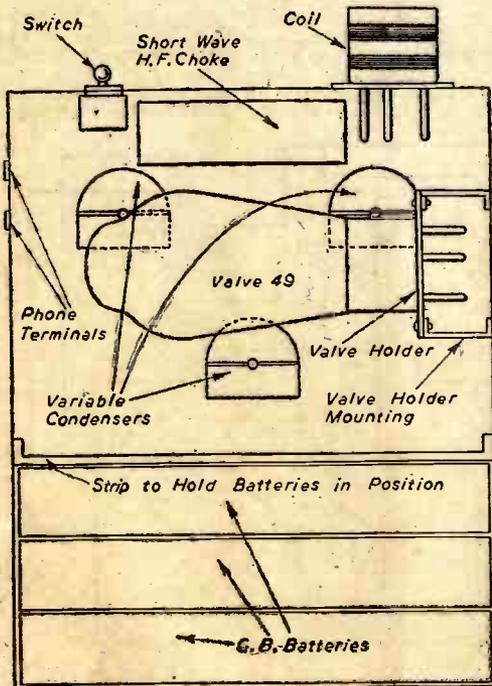
Fig. 3.—Rear view of the interior of the receiver, showing how the valve is mounted.
