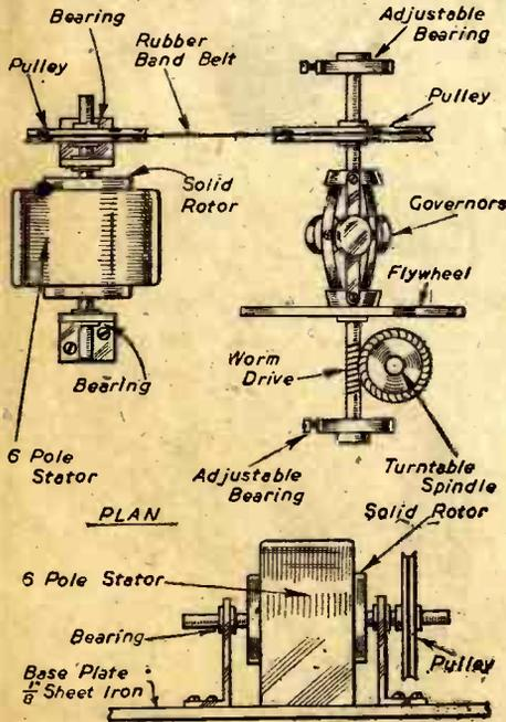
A converted cycle dynamo used as a gramophone motor.
