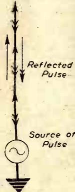
Fig. 69.—Reflection of voltage pulse.
