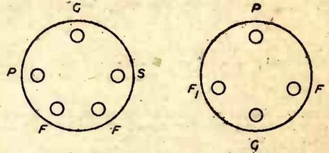
Fig. 4 (Left).—The pin connections for the 49 valve holder. (Right) Those applying to the coil and holder. The view of the valve holder is the underside but that of the coil holder is upperside.
