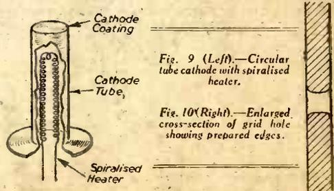
Fig. 9 (Left).—Circular tube cathode with spirals heater.
