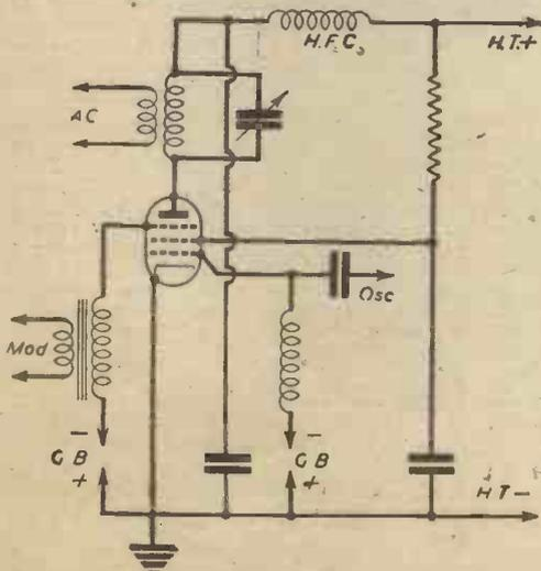
Fig. 5.—How suppressor-grid modulation may be applied to an R.F. amplifier.
