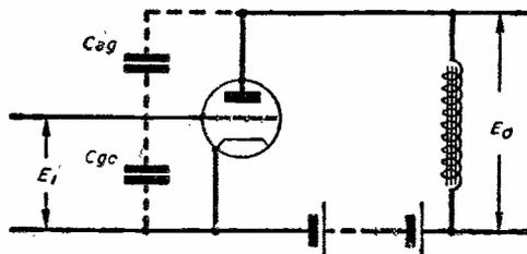
Fig. 2.—The anode load in this instance is an L.F. choke and is therefore reactive.
