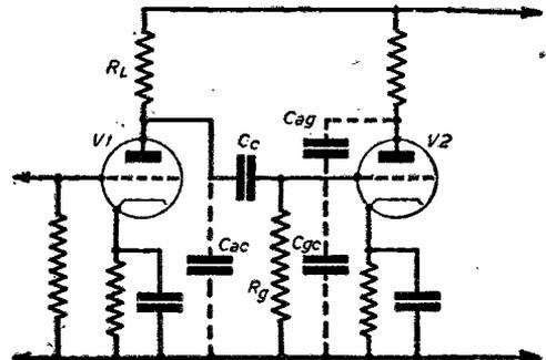
Fig. 8.—A typical resistance capacity coupled A.F. amplifier.
