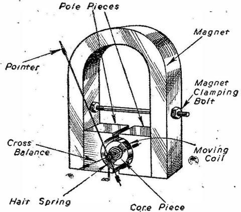
Fig. 1.—Diagrammatic view of a moving coil meter.
