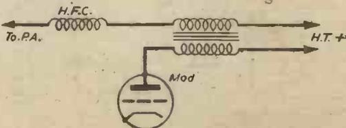
Fig. 2.—A method of matching the modulator to the P.A. by using an iron-cored transformer.
