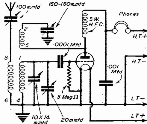
Fig. 3.—Theoretical circuit of DX 1-valver.
