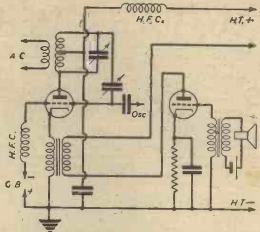
Fig. 4.—Cathode modulation. The modulator output is used to vary both grid bias and anode voltage.
