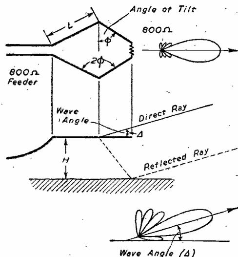
Fig. 2.—These diagrams show a rhombic aerial in plan and elevation, whilst the horizontal and vertical polar diagrams indicate the general radiation pattern.
