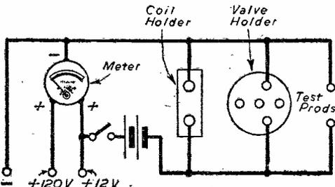
Front view of finished tester, and diagram of connections.
