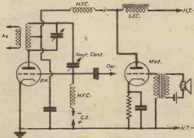
Fig. 1.—Simple anode or choke modulation of a Class C R.F. amplifier.
