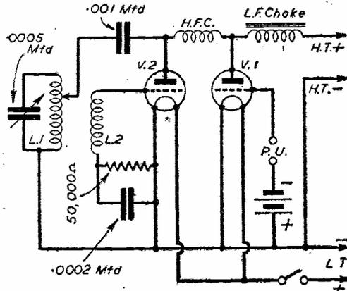
Fig. 6.—Circuit suitable for pick-ups with small output.
