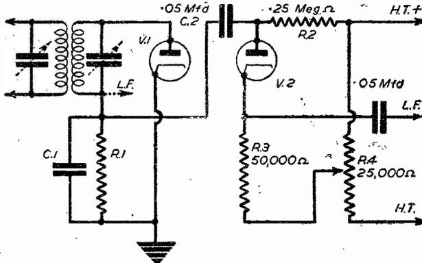
Fig. 3. (Left).—A noise-suppression circuit used between the second detector ( $V_1$ ) and L.F. amplifier of a superhet receiver.
