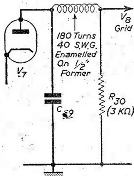
Fig. 2. — Modified diode filter on the vision unit.
