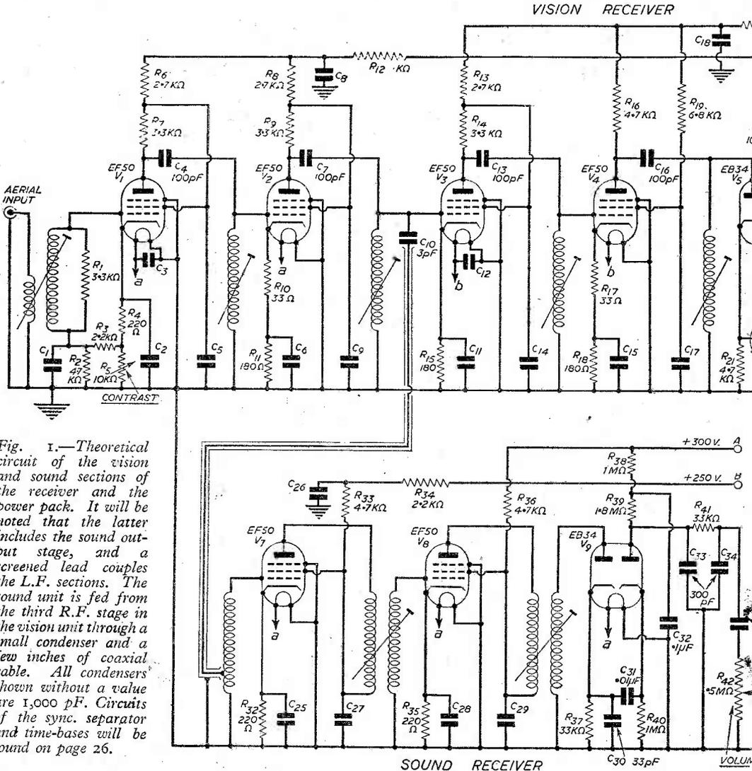
*Fig. 1.—Theoretical circuit of the vision and sound sections of the receiver and the power pack. It will be noted that the latter includes the sound output stage, and a screened lead couples the L.F. sections. The sound unit is fed from the third R.F. stage in the vision unit through a small condenser and a few inches of coaxial cable. All condensers shown without a value are 1,000 pF. Circuits of the sync. separator and time-bases will be found on page 26.*
