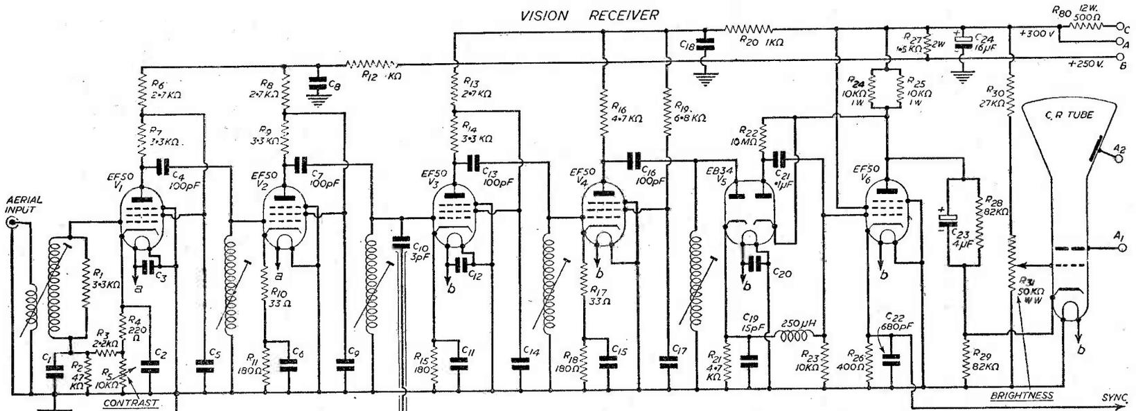
Fig. 1.—Theoretical circuit of the vision and sound sections of the receiver and the power pack. It will be noted that the latter includes the sound output stage, and a screened lead couples the L.F. sections. The sound unit is fed from the third R.F. stage in the vision unit through a small condenser and a few inches of coaxial cable. All condensers shown without a value are 1,000 pF. Circuits of the sync. separator and time-bases will be found on page 26.
