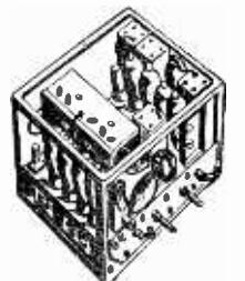
**VIBRATOR PACK 21.** The vibrator pack designed to supply the above unit and its associated transmitter. It can be fitted beneath the receiver and form a neat self-contained set. Output of 150 v. at 40 mA, which is sufficient for most small receivers, is obtained from 6 v. input. ONLY 19.6.
