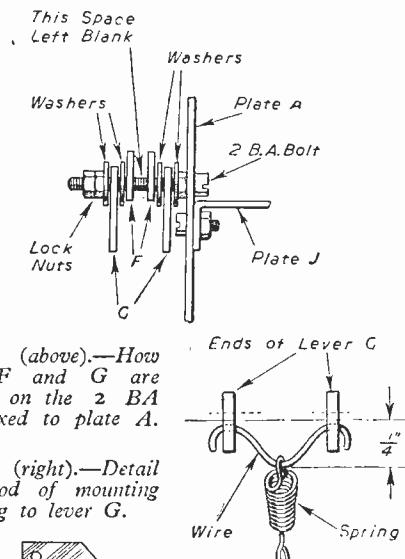
Fig. 17 (above).—How levers F and G are mounted on the 2 BA screw fixed to plate A.
