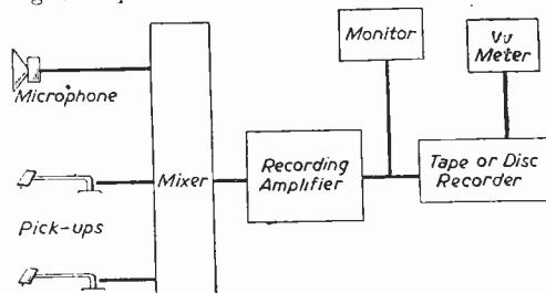
Fig. 2.—Block diagram representing equipment for recording either (on disc) composite effects, such as voices plus crowd noise plus band playing, or (on tape) sound track to be synchronised with cine film.
