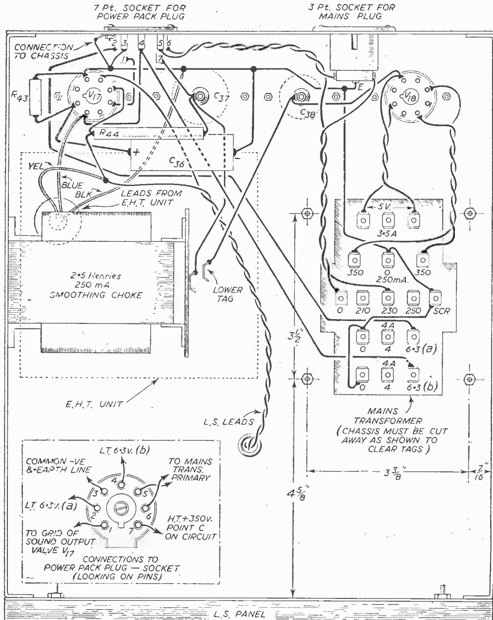
Fig. 4.—Wiring diagram of the power supply and audio output stage.
