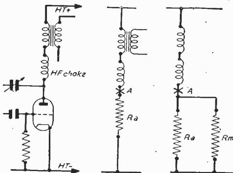
Fig. 1.—Theoretical and equivalent circuits of a single valve stage.
