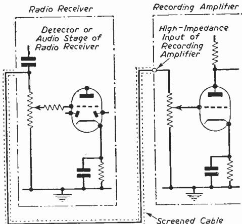
Fig. 1.—Method of connecting radio receiver to recording amplifier to record radio material. Note: The output stage of the radio receiver may be used to monitor the programme material. Variation of the radio volume control will not affect the recording circuit.
