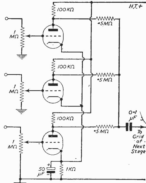
Fig. 4.—Circuit of three-channel input mixer. Channels are completely independent, and more may be added, in parallel, if required. Values used are general purpose triodes, such as 6C5, 6J5. Types containing two triodes in one envelope, such as 6N7, 6SN7, 6SC7, can be used more economically.
