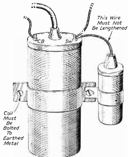
Fig. 5.—Suppressor condenser connected to ignition coil.
