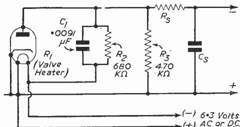
Fig. 5.—A practical version of Fig. 3 with component values.
