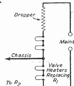
Fig. 6.—Showing a method of replacing  $R_1$  by valve heaters.
