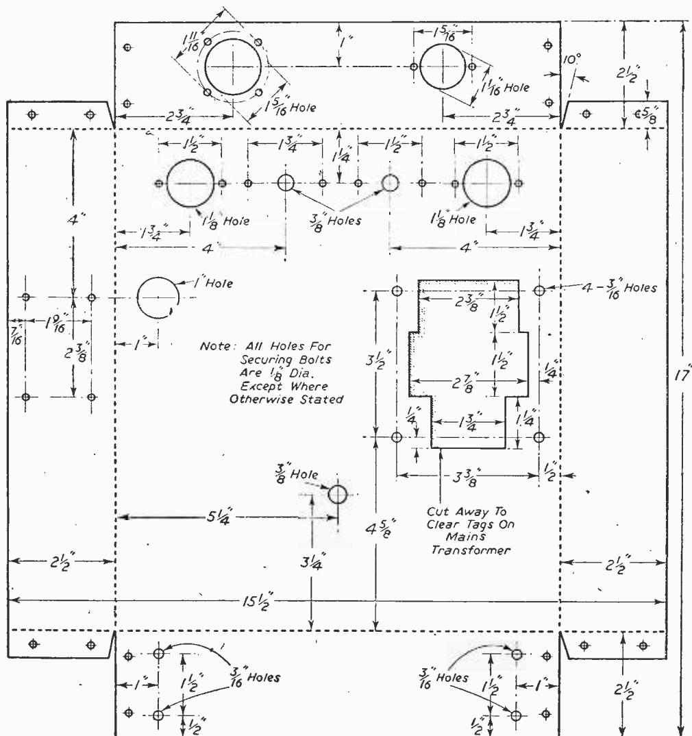
Fig. 3.—Cutting and drilling data for the chassis of the mains unit.
