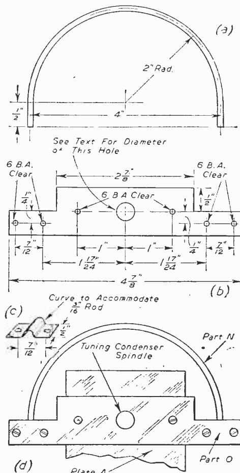
Fig. 20 (a), (b) and (c).—Warning light mechanism, and parts N and O. (d) Appearance of semi-circular contact mounting when assembled. The brass saddles holding parts N and O together are mounted behind part O.
