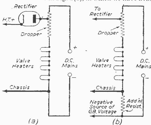
Fig. 2 (a).—Skeleton diagram of a typical supply circuit for an A.C./D.C. receiver.
