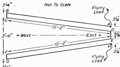
Fig. 1.—Layout and dimensions of the aerial.
