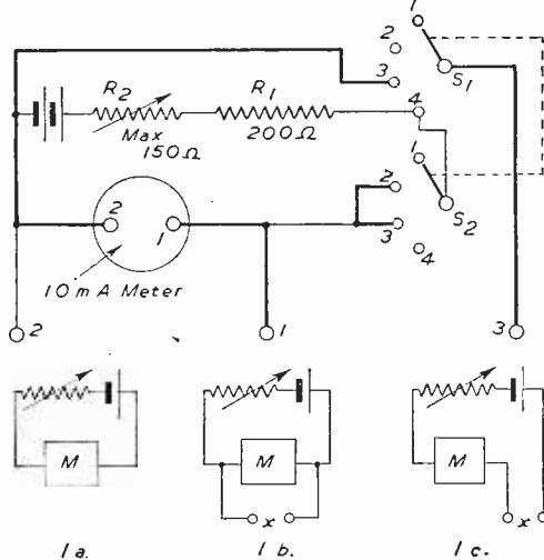
Fig. 1—Theoretical circuit of the test meter.
