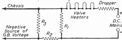
Fig. 4.—Simplified version of Fig. 3, showing how that circuit functions on a D.C. mains supply.
