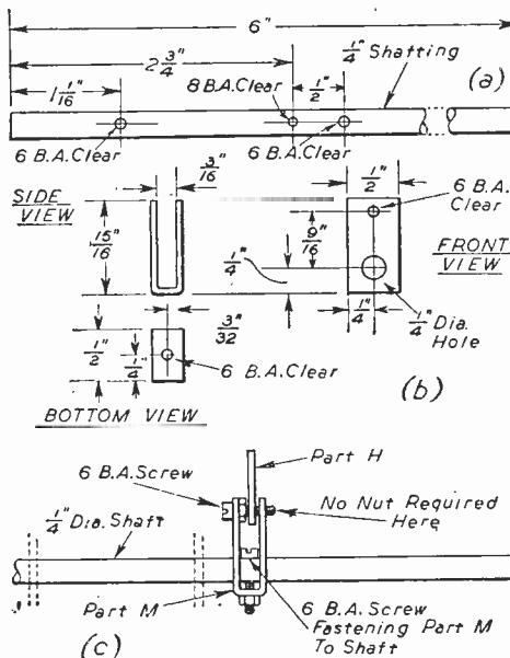
Fig. 15. (a) and (b).—Details of shafting, and its mount. (c) How part M is fixed to the lin. spindle.
