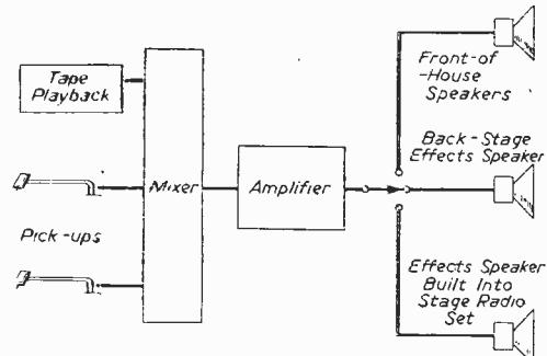
Fig. 3.—Typical theatre set-up, capable of providing effects from tape, disc, or both, and interval music from disc. All speakers must be generously rated to avoid overloading.
