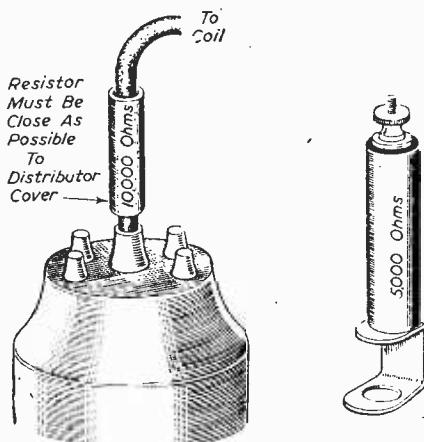
Fig. 4 (left).—Suppressor resistor in main ignition H.T. lead.
