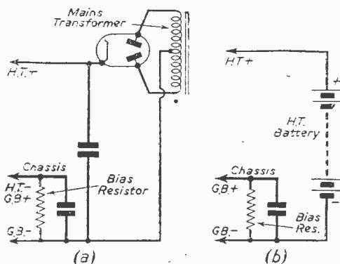
Figs. 1 (a) and (b).—How "automatic" bias may be obtained from A.C. and battery-operated equipment.
