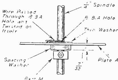
Fig. 19.—Detail of method used to fix  $\frac{1}{4}$  in. spindle to plate A.
