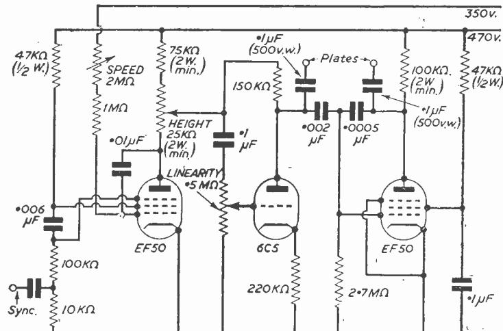
Note: All Capacitors Except The  $\text{0.1}\mu\text{F}$ 's Must Be Mica
