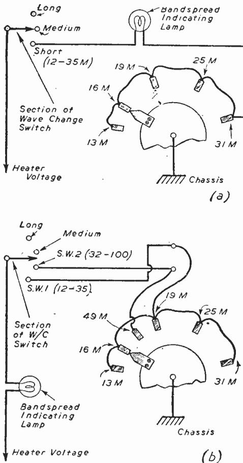
Fig. 23.—(a) and (b). Various methods of connecting the fixed contacts and bandsread indicating lamps to obtain different effects.
