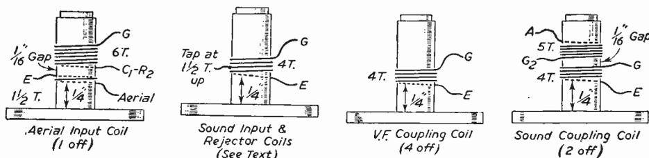
Fig. 1.—Details of the coils for Sutton Coldfield. Wire used is 28 S.W.G.
