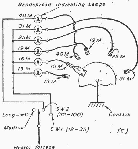
Fig. 23.—(c). Further method of connecting the contacts.
