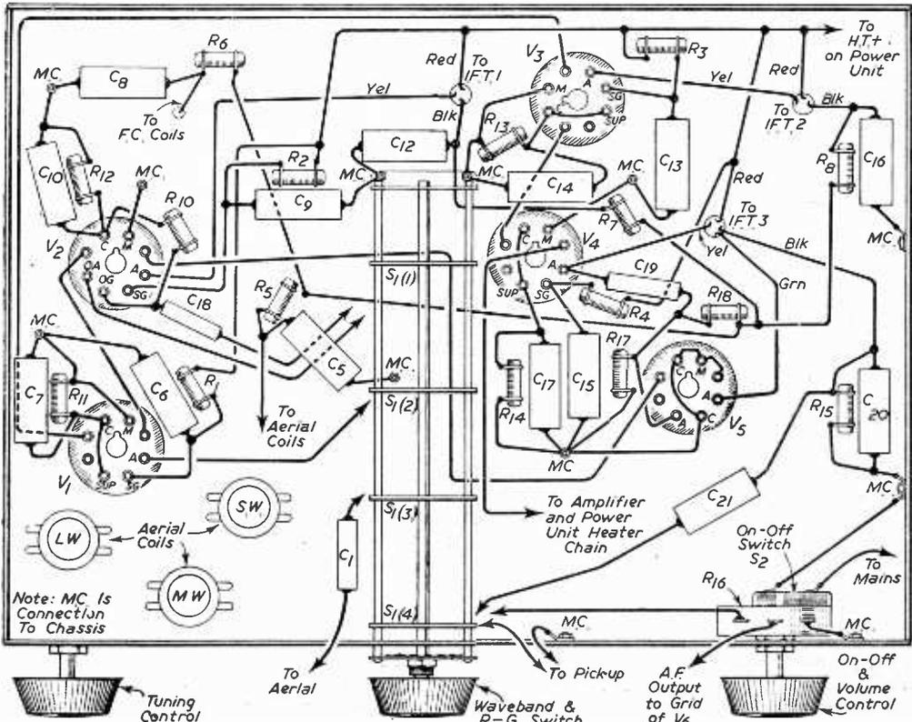
Fig. 3.—Wiring details of the receiver section. The amplifier portion will be dealt with next month.
