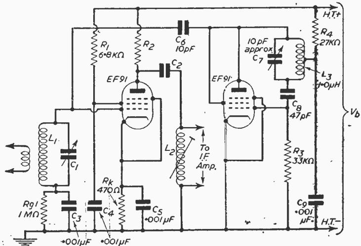
Fig. 1.—Typical television mixer circuit.
