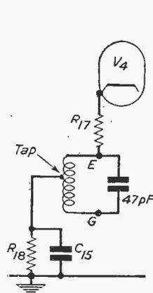
Fig. 2.—Position of the rejector coil in the cathode circuit of V4.
