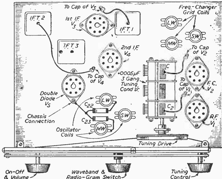
Fig. 2.—Chassis layout of the receiver section.
