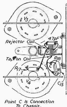
Fig. 3.—Actual position of the rejector coil on the chassis side runner.
