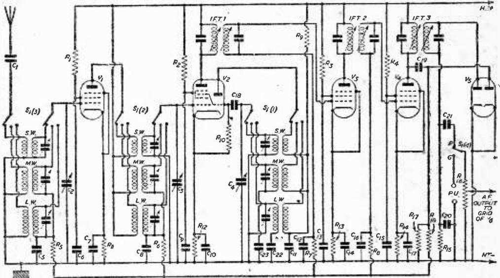
Fig. 1.—Theoretical circuit of the receiver.
