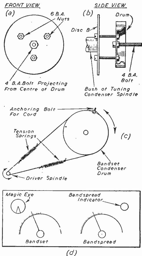
Fig. 22.—(a) and (b). How a drum for a cord drive may be fitted to the bandset tuning condenser. (c) A spring is fitted to both sides of the cord drive to avoid strain (see text). (d) Suggested dial layout for the unit.
