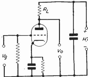
Fig. 4.—Single-stage voltage amplifier.
