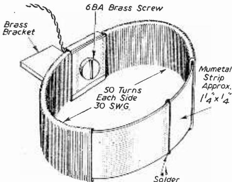
Fig. 1.—A simple record-playback head.
