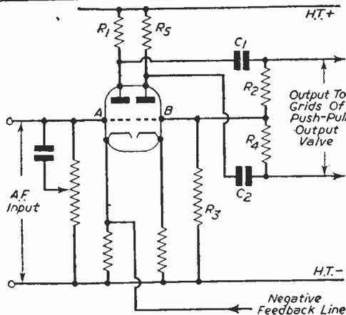
Fig. 2.—Basic circuit for phase inverter using a double triode.
