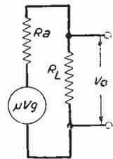
Fig. 5.—Equivalent circuit of Fig. 4.
