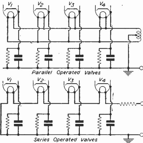
Figs. 1 and 2.—Note the possible difference of potential between heater and cathode of V4 in each case.
