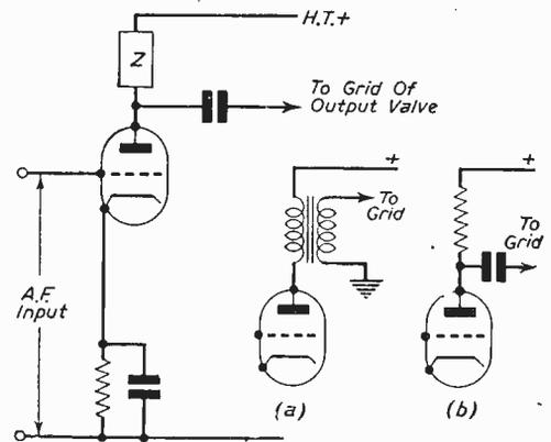
Fig. 1.—Basic circuit of triode amplifier, together with (a)—Transformer coupling, and (b)—Resistance-capacity coupling.
