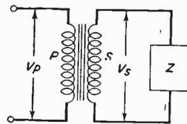
Fig. 8.—Standard transformer circuit.
