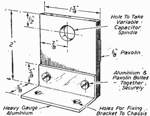
Fig. 5.—Bracket for condenser.
