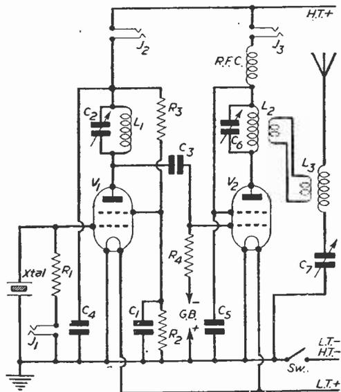
Fig. 1.—Theoretical circuit of the complete unit.
