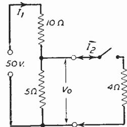
Fig. 1.—Simple potential divider circuit.
