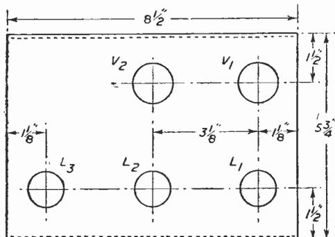
Fig. 2.—Chassis drilling data.
