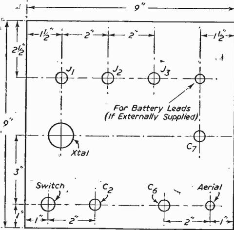
Fig. 4.—Details for panel drilling.
