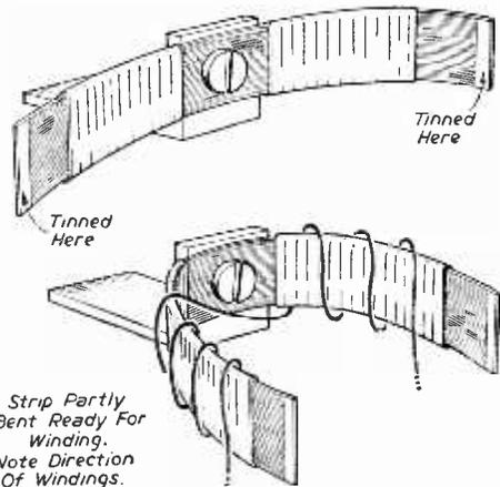
Fig. 2.—Details of construction of the head.
