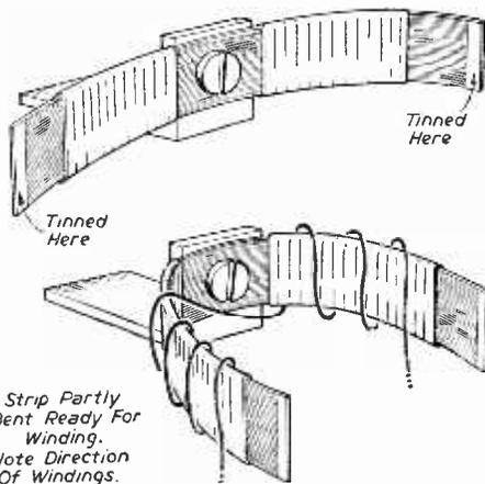
Fig. 2.—Details of construction of the head.
