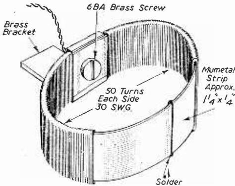
Fig. 1.—A simple record-playback head.
