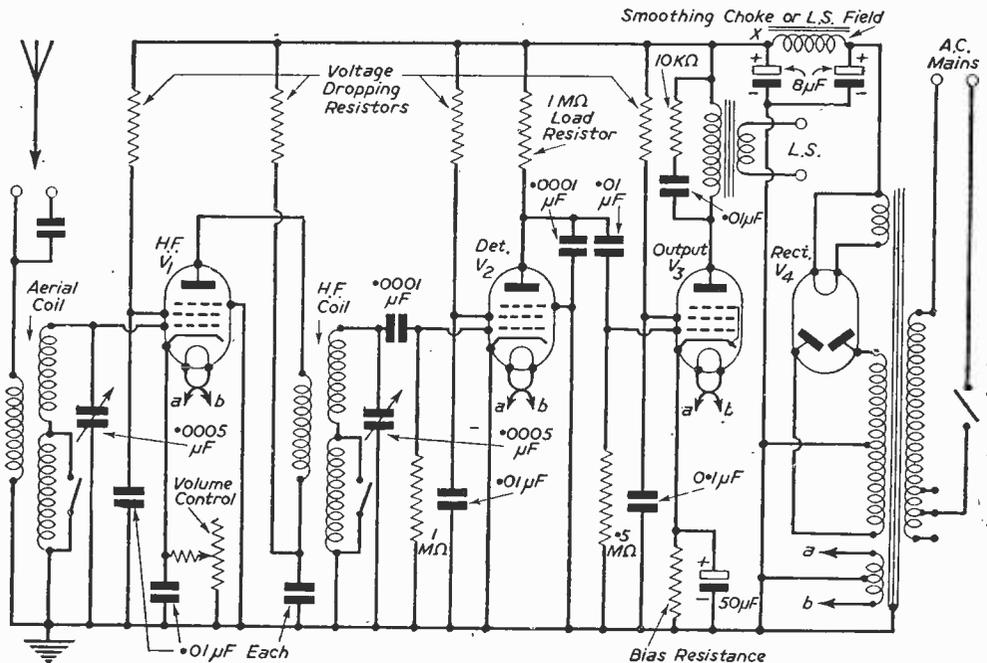
Fig. 1.—A suggested circuit for a simple 3-valve plus rectifier A.C. Mains Receiver. Details of design and the principles involved will be described in this series.
