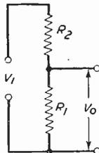
Fig. 3.—Potential divider circuit without values.
