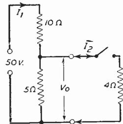
Fig. 1.—Simple potential divider circuit.
