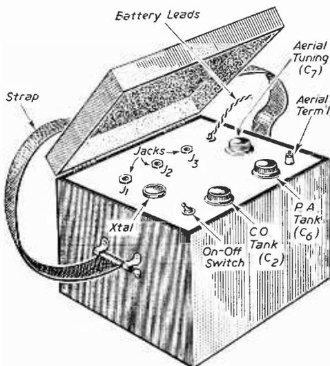
Fig. 3.—Appearance of finished unit.
