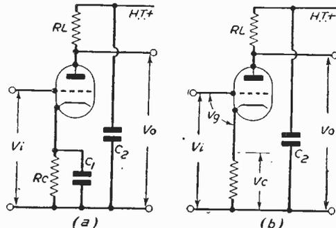
Fig. 2.—Simple amplifier and modification to introduce N.F.B.
