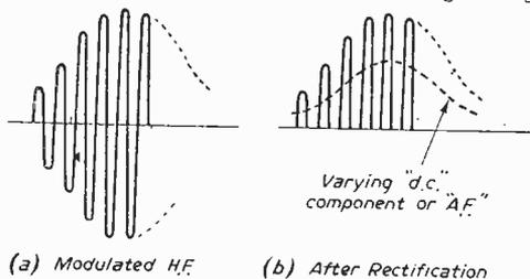
Fig. 6.—Rectification of a modulated signal. The D.C. component will now be varying at the frequency of the amplitude modulation.
