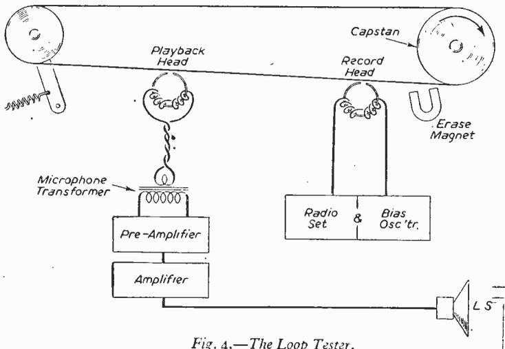
Fig. 4.—The Loop Tester.
