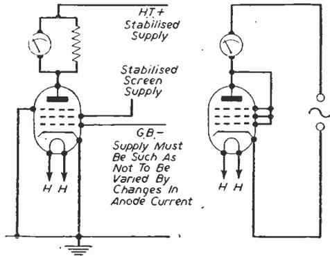
Fig. 3.—Heater supply must apply accurate potential across heater. This supply must give correct voltage for any current drawn. Care must be taken to prevent oscillation through arrangement of leads to electrodes.
