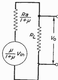
Fig. 7.—Equivalent circuit of Fig. 6.
