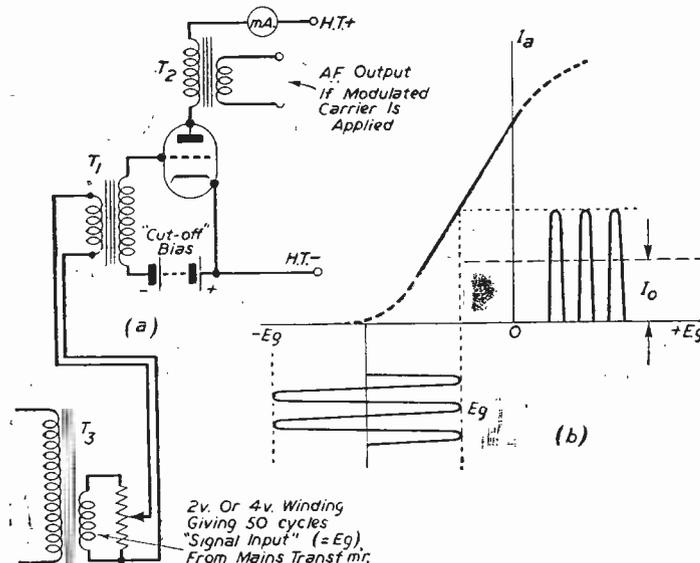
Fig. 5.—Demonstrating "Anode Bend" Detection with a Milliammeter.
