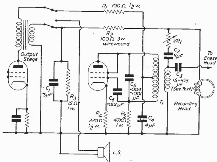
Fig. 3.—Oscillator and head circuit. The oscillator coil may be obtained from Wright and Weare, Judge Industries, etc.
