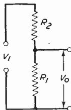
Fig. 3.—Potential divider circuit without values.
