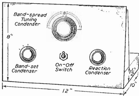
Fig. 3.—Panel and chassis panel mounting.
