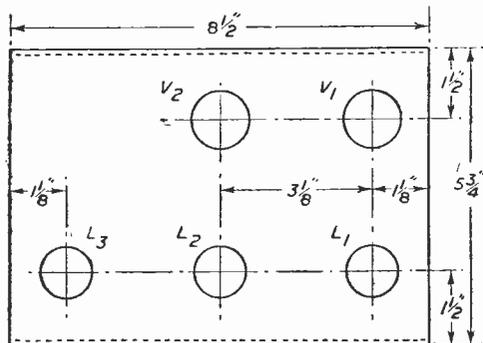
Fig. 2.—Chassis drilling data.
