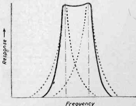
Fig. 5.—The response curve obtained by combining the response curves of two crystals in opposite phase—a band pass characteristic.
