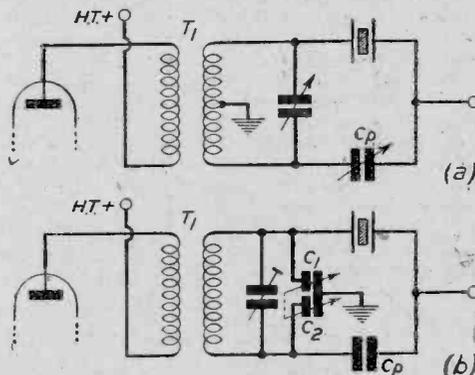
Fig. 2.—Showing the position of the phasing condenser  $C_p$  in the bridge. In (a) the centre-tap on the coil is earthed, and in (b) the rotor of the "opposed stator" condenser  $C_1 C_2$ .
