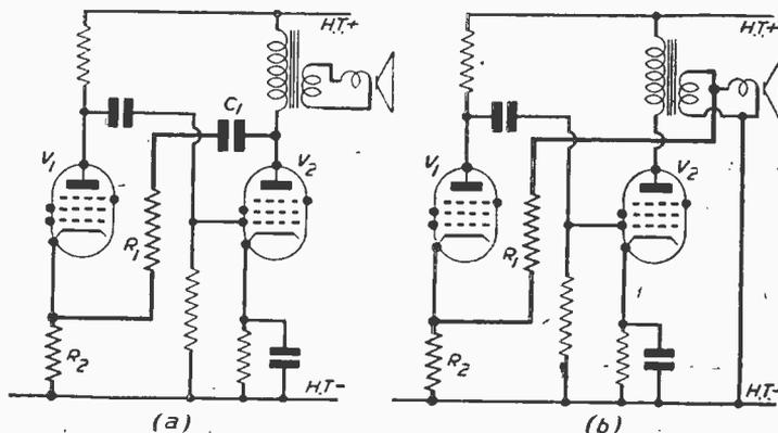
Fig. 4(a) and (b).—Two popular methods of applying feed-back in A.F. amplifiers.
