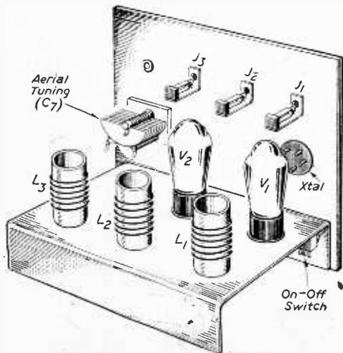
Fig. 6.—Rear view of the set showing coils in position.
