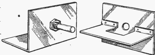
Figs. 1 and 2.—Simple chassis for superhet or straight units.
