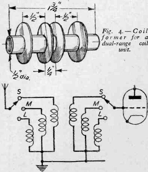
Fig. 4.—Coil former for a dual-range coil unit.
