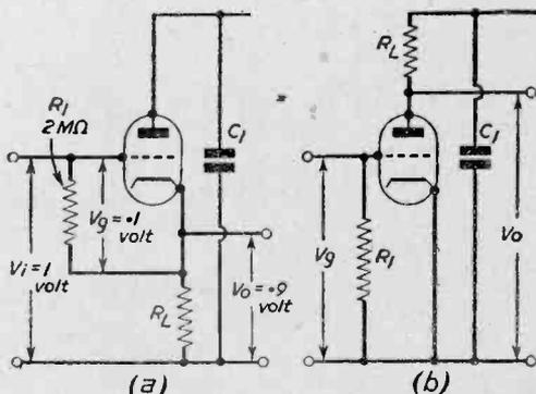
Fig. 7.—(a) A practical cathode—follower circuit, and (b) a simple amplifier, without feedback.
