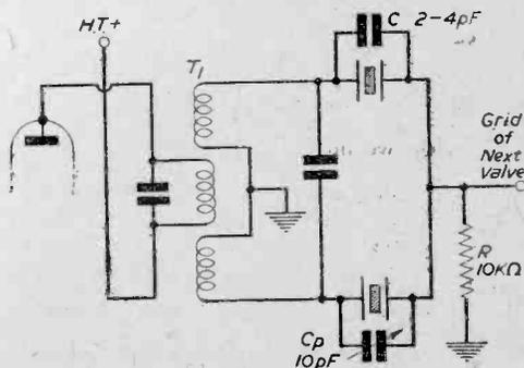
Fig. 6.—A band pass filter for C.W.  $C_p$  phasing condenser 10 pF.  $C$ , balancing condenser 2-4 pF.  $T_1$ , input transformer—secondary composed of two normal secondaries in series.  $R$ , 10,000  $\Omega$ .
