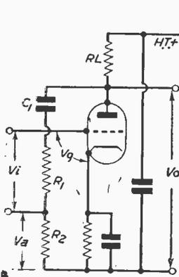
Fig. 3.—This circuit shows voltage feed-back.
