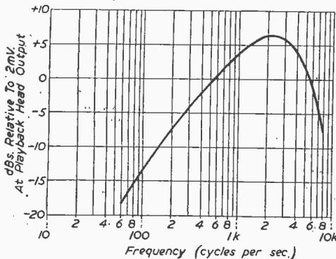
Fig. 4.—Response curve (uncompensated) of the G.E.C. Grade A tape.
