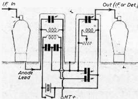
Fig. 4.—(b) One way of laying out the above circuit on a chassis.
