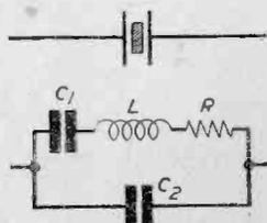
Fig. 1.—The quartz crystal resonator and its equivalent circuit.
