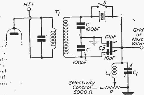
Fig. 4.—(a) A practical crystal gate circuit.
