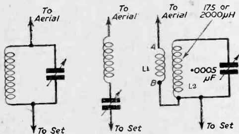
Figs. 1, 2 and 3.—Three simple wavetraps circuits, in which unwanted frequencies may be kept out of the receiver circuits.
