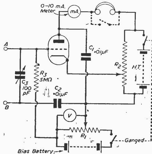
Circuit of the Valve Voltmeter
