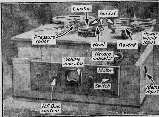
Fig. 1.—A typical home-made tape-recording and play-back unit with self-contained amplifier.
