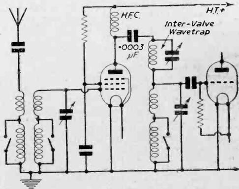
Fig. 4.—In this circuit the wavetraps is included in the H.F. coupling circuits.
