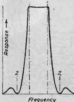
Fig. 7.—The effect obtained in a band-pass filter when the phasing condenser does not balance the capacity of the crystals in their holders. 2 Zero points are obtained. Compare with Figs. 3 (b) and 5.
