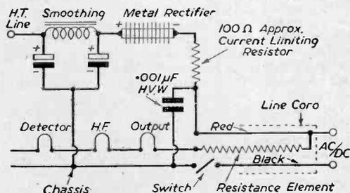
Fig. 2.—Circuit showing method of including a line-cord.
