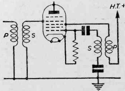
Fig. 5.—Simple frequency-changer stage.
