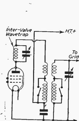
Fig. 5.—Another circuit in which the wavetrap is found between the H.F. and detector stages.
