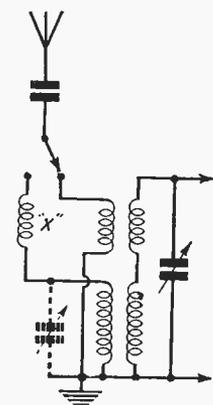
Fig. 6.—The use of an "anti-breakthrough" choke or coil is shown here.
