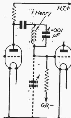
Fig. 7.—The trap circuit here is used to remove heterodyne whistles.
