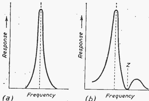
Fig. 3.—(a) Phasing condenser balancing out exactly capacity of crystal holder. (b) Response curve obtained when phasing condenser does not exactly balance the capacity of the crystal holder.
