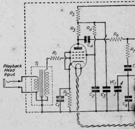
Fig. 2.—Theoretical circuit of a pre-amplifier for use in recorders. A list of components will be found on
