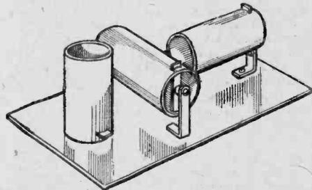
Fig. 7.—Three coils may be mounted as shown here to avoid interaction.
