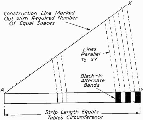
Fig. 2.—Diagram shows method of constructing a stroboscope for the rim of a turntable.
