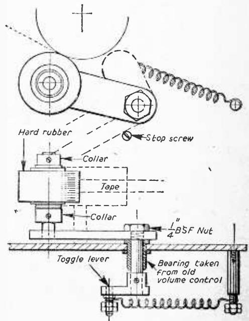
Fig. 2.—The pressure roller with toggle action.
