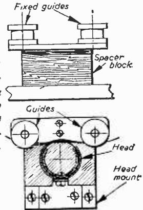
Fig. 4.—The recording head is mounted in a clamp made up from two strips of brass as shown in this plan and elevation.
