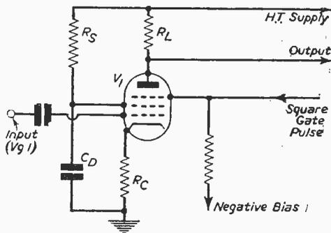
Fig. 3.—Basic "Gate" Circuit.
