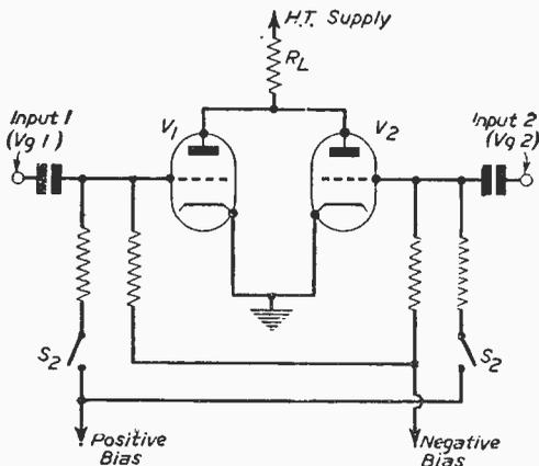
Fig. 1.—Basic Electronic Switch Circuit.
