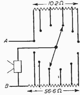
Fig. 3.—Wiring the resistances to a double-pole switch.
