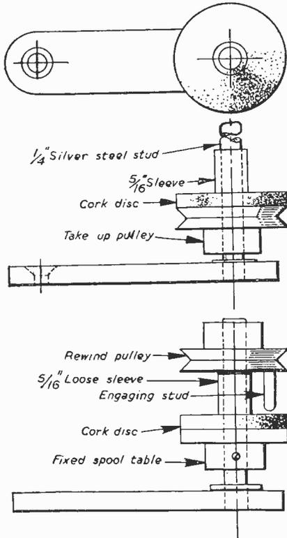
Fig. 3.—The feed-spindle with rewind pulley.
