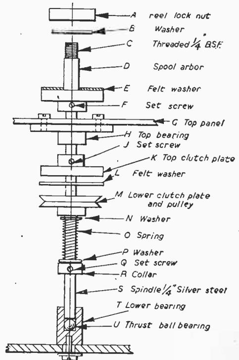
Fig. 7.—Full details of the take-up spindle.
