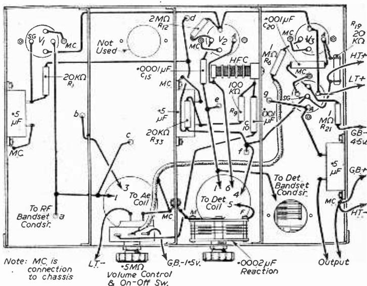
Fig. 4.—Below chassis wiring details.
