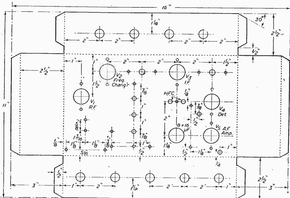
Fig. 2.—Drilling and cutting details of the chassis.
