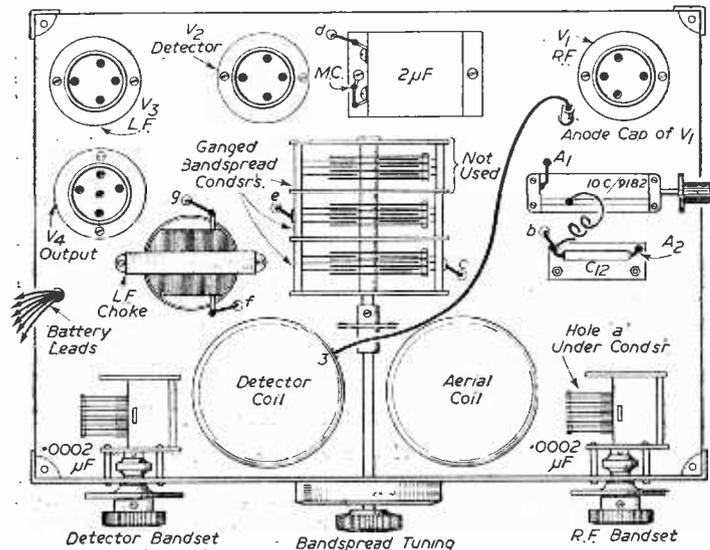
Fig. 3.—Above chassis layout and wiring details.
