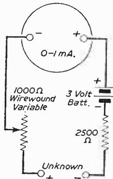
Fig. 8.—Circuit arrangement for an ohm-meter.
