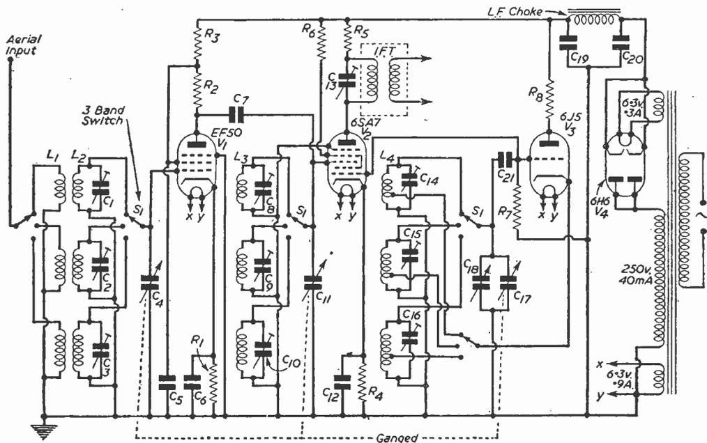
Fig. 1.—Theoretical circuit of the converter.
