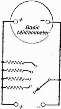
Fig. 7.—How shunts may be switched for multi-range milliammeters.
