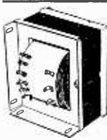
**Mains Transformers UPRIGHT-DROP THROUGH AS ILLUSTRATED. Two Types Only. No. 1: 250-0-250v., 80 mA., 0-4-6.3v., 5 amp. 0-4-5v., 2 amp. No. 2: Same, but 350v. Both 15/6, post 1/- for 1 to 3**
