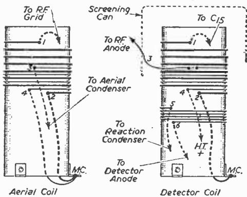
Note: MC. Is Connection To Metal Chassis
