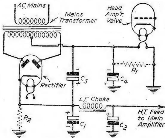
Fig. 3.—Another method of obtaining D.C. for the first valve.
