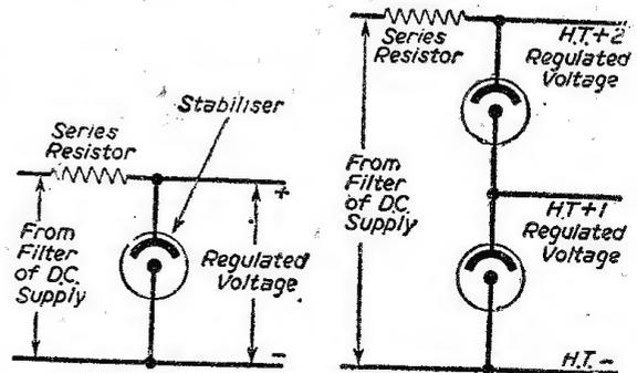
Fig. 1.—Circuit of straightforward stabiliser circuit.
