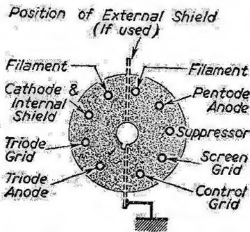
Fig. 2.—Details of valve base for the ECL80 valve.
