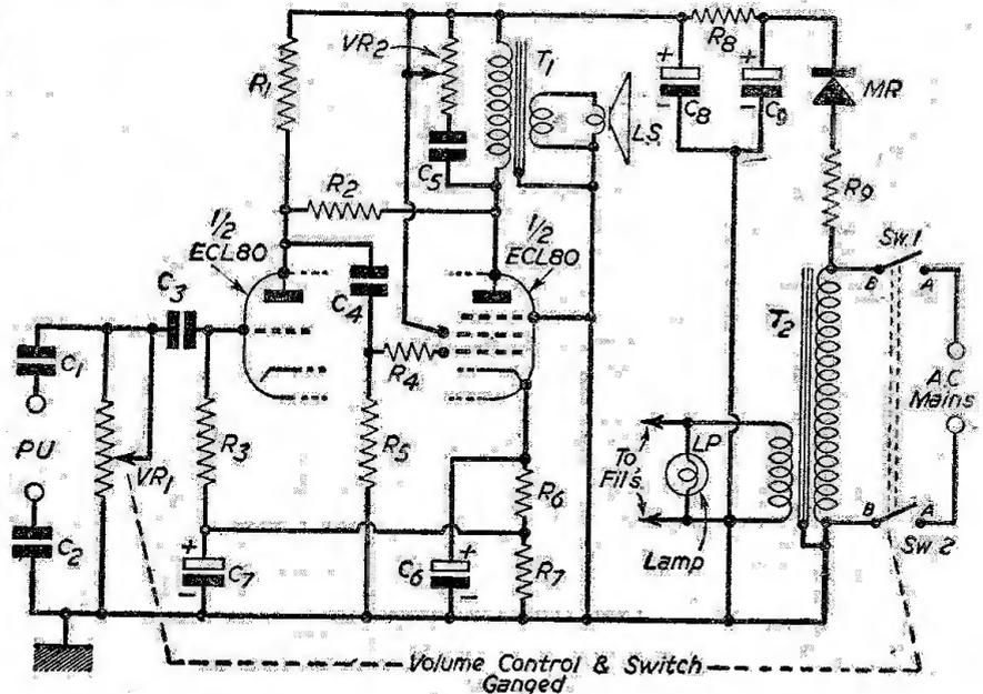
Fig. 1.—Theoretical circuit of the amplifier.
