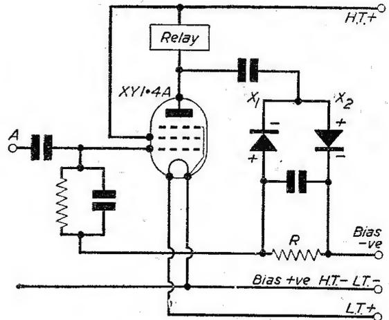
Fig. 2.—Final circuit of the A.F. stage.
