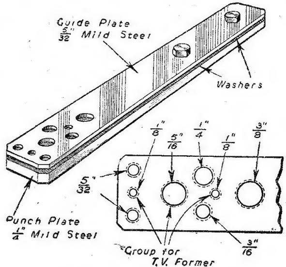
Details of construction of the punch.
