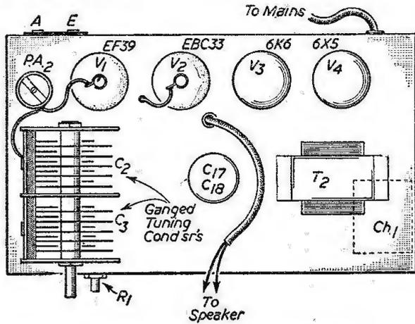
Fig. 2.—Layout of the receiver.
