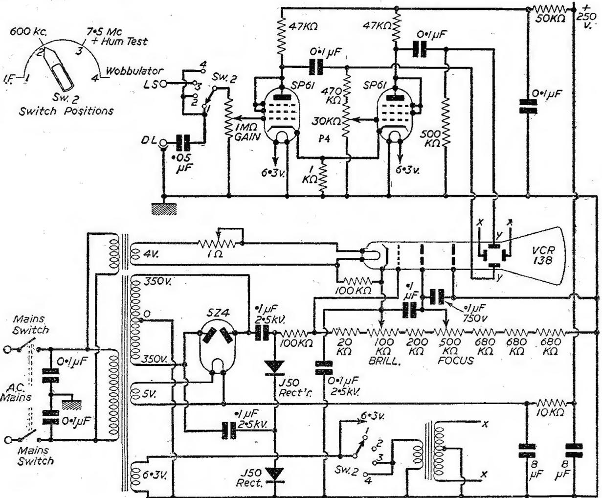
Fig. 2.—Tube and power supply circuits.
