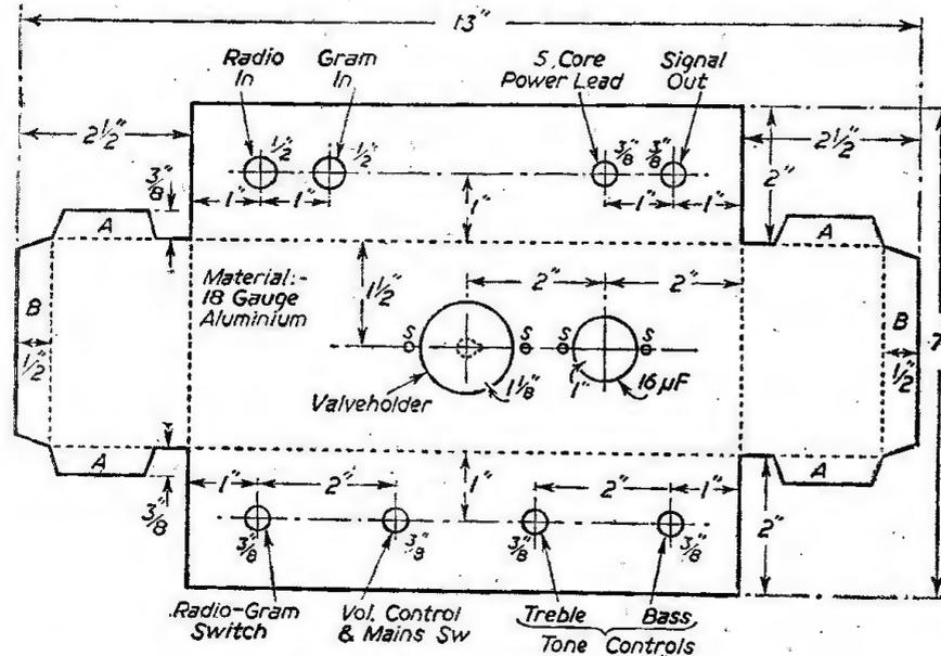
Fig. 2.—Chassis layout and drilling data.
