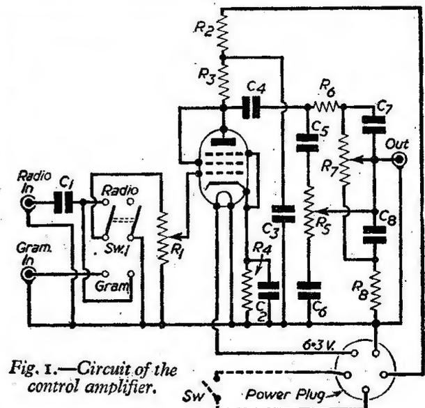
Fig. 1.—Circuit of the control amplifier.
