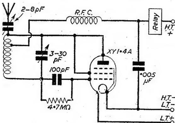
Fig. 1.—Detector stage of the receiver.
