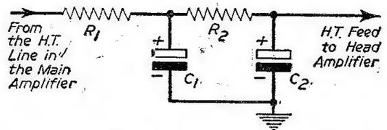
Fig. 2.—Circuit of the H.T. filtering.
