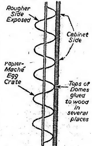
Fig. 1.—Method of fixing lining.
