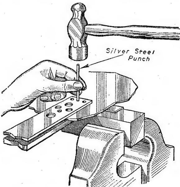
How the punch is used on the chassis.
